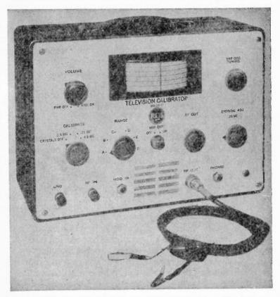
FIG. 19-Exterior view of R.C.A. type WR-39B television calibrator.
