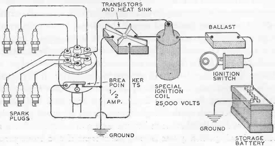
which flows through the points, especially at low speeds, overheats the points. The heat oxidizes and pits the points. Then the car does not start easily or run smoothly until the points have been replaced. If an engine is to be kept 100 per cent "tuned," the breaker points should be inspected or replaced (if necessary) every 2,000 to 5,000 miles.
