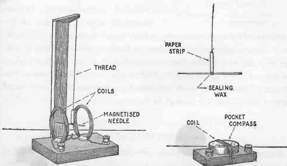
the wooden block or base. The thread should be fastened directly over the center of the coil. The paper strip and its needle swing in the center of the coil. The terminals of the coil are connected to two binding posts mounted on the base. When you use the gal-
