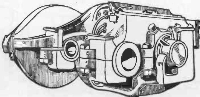
dynamo which is reversed, that is, instead of being driven by an engine or a turbine and generating an electric current it is fed with an electric current and used to drive machinery. In general construction there is but little difference between a dynamo and a motor, but there are differences in detail that make each machine better adapted to its own particular work.
