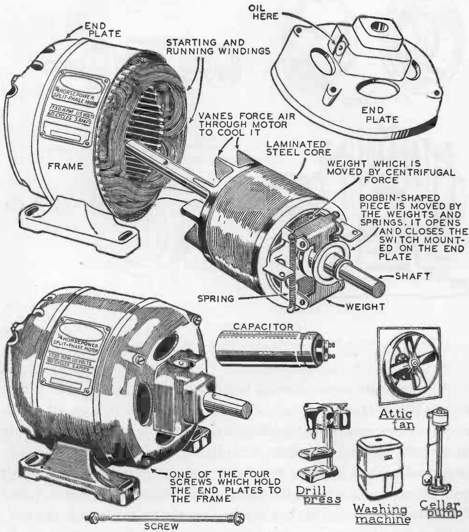
FRACTIONAL-HORSEPOWER CAPACITOR MOTOR
