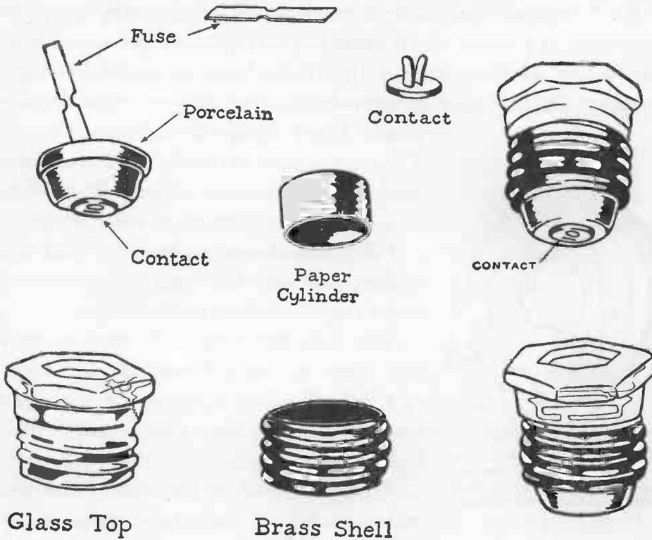
A FUSE PLUG SEPARATED INTO ITS PARTS
