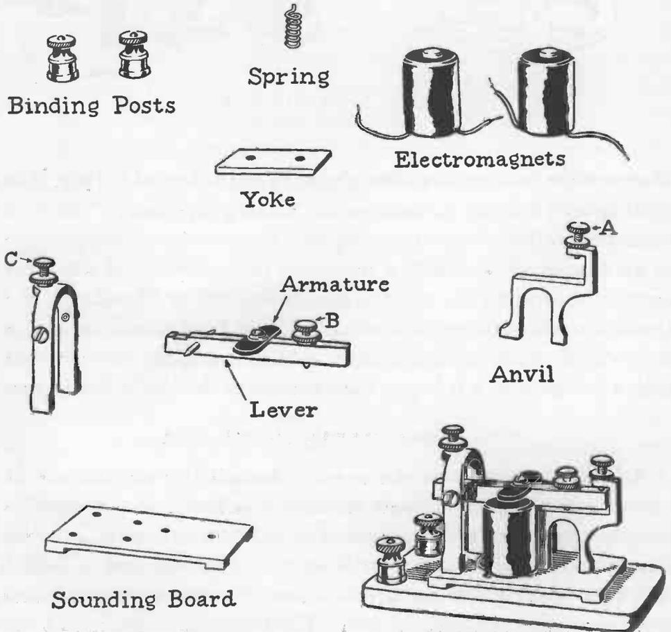
strikes the anvil and makes a click. When the key lever is released, the current flow ceases, the spring on the sounder pulls the lever up and it clicks against the top of the anvil.
