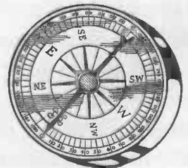
The magnetic compass which surveyors and hunters use on land to tell direction is almost as simple as the first one which the unknown inventor made. It is nothing more than a flat steel needle which has been magnetized and supported on a pivot at its center. The needle swings over a scale divided into degrees and also marked with the "points" of the compass. The needle and its scale are enclosed in a small case with a glass crystal like a watch.
