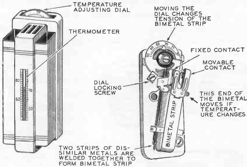
**A THERMOSTAT IS A SWITCH WHICH IS OPERATED BY CHANGES IN TEMPERATURE**
