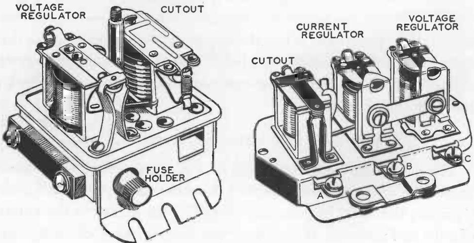
out of the field winding circuit in the generator. The regulators, together with the automatic cutout, are enclosed in a steel box mounted on top of the generator. Sometimes only a cutout and a voltage regulator are provided but many cars are equipped with a cutout, a voltage regulator and a current regulator.
