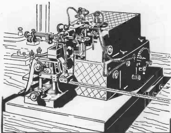
over an ocean cable. The current which travels through the cable when the key is pressed does not go to the other end instantly as it does over a telegraph line. It travels along like a wave. It takes one-fifth of a second for a signal to travel between Ireland and Newfoundland and then three seconds more for the current to gain its full strength. This makes a special device for receiving messages necessary.
