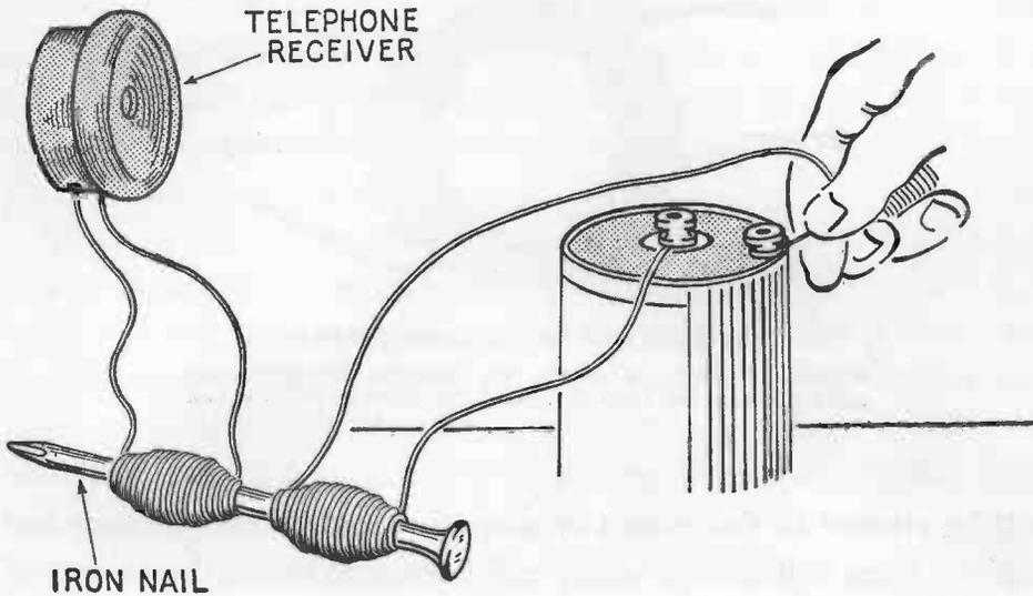
AN EXPERIMENT WITH ELECTROMAGNETIC INDUCTION
