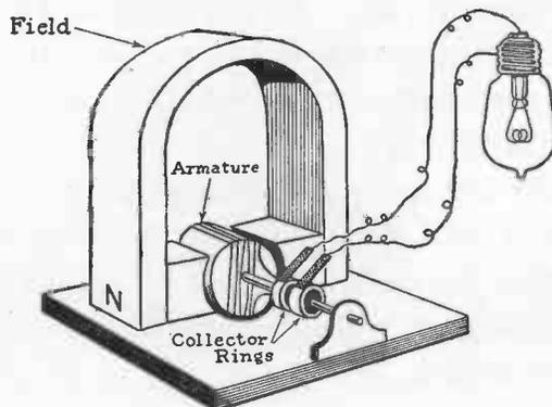
ulated rings (called collector rings) are mounted on the shaft and each connected to one end of the revolving armature coil. A little strip of thin copper or copper gauze (called the brushes) presses against each ring. The rings and the brushes lead the current out from the armature so that it may be employed for some useful work such as lighting a lamp.
