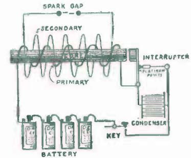
FIG. 157. — Diagram showing Essential Parts of Induction Coil.
