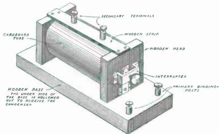
FIG. 166. — Completed Coil.
