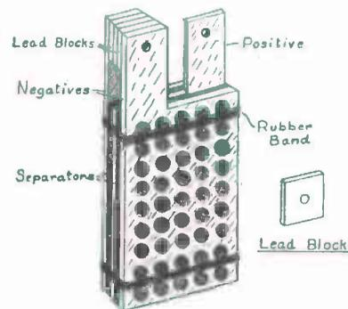
FIG. 73. — The Complete Element for a Storage Cell.
