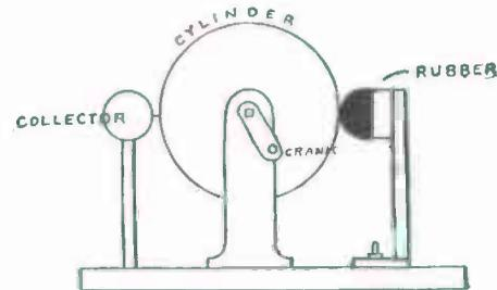
FIG. 29. — Front View of a Cylinder Electric Machine.
