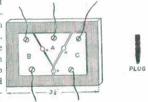
FIG. 100. — Home-made Lightning-Arrester.
