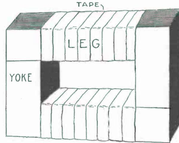
FIG. 181.—The Core, Assembled and Taped.
