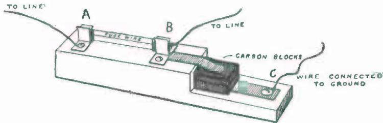
FIG. 101. — Lightning-Arrester for Telephone Wires.
