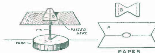
FIG. 21. — A Paper Electroscope.
