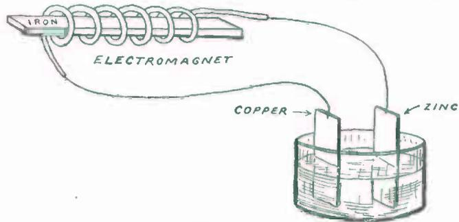
FIG. 83. — The Principle of an Electro-Magnet.
