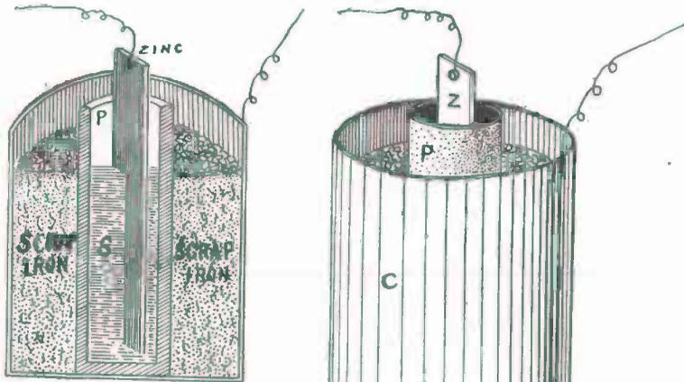
FIG. 67. — A Tomato-Can Cell; Sectional View.
