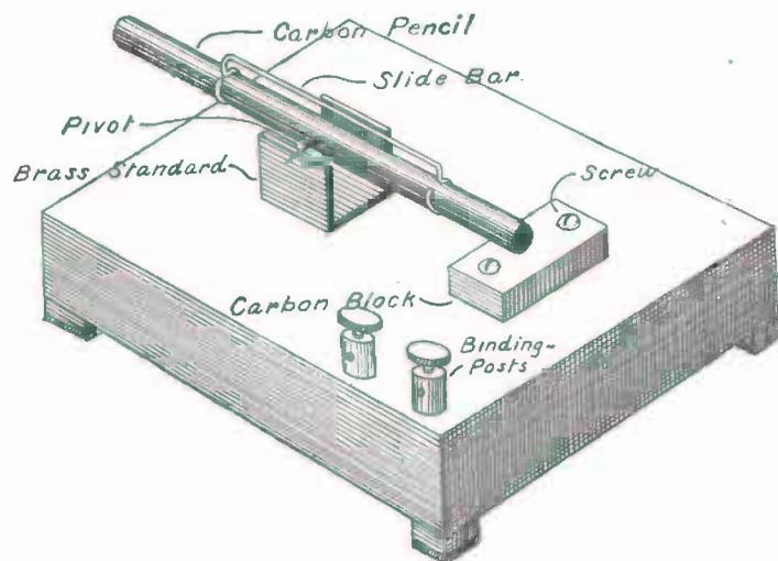
FIG. 144. — A Very Sensitive Form of Microphone, with which the Footsteps of a Fly can be heard.
