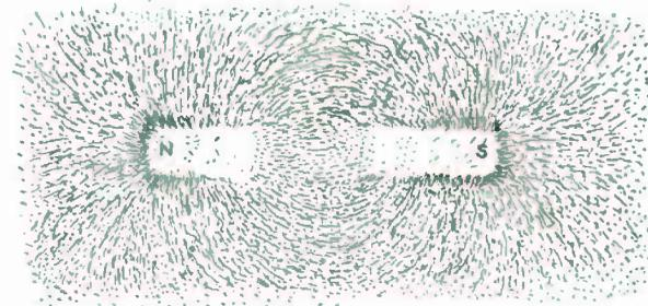
FIG. 13. — A Magnetic "Phantom," Showing the Field of Force about a Magnet.
