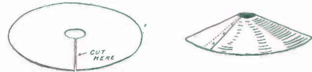
FIG. 293.—How the Reflector is made.
