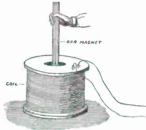
FIG. 86. — Showing how a Current of Electricity may be induced by a Bar Magnet and a Coil.
