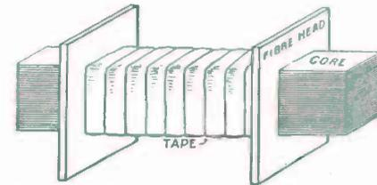
FIG. 184. — Leg with Heads in Position for Winding.
