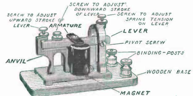
FIG. 131. — A Typical Telegraph Sounder, showing the Various Parts.
