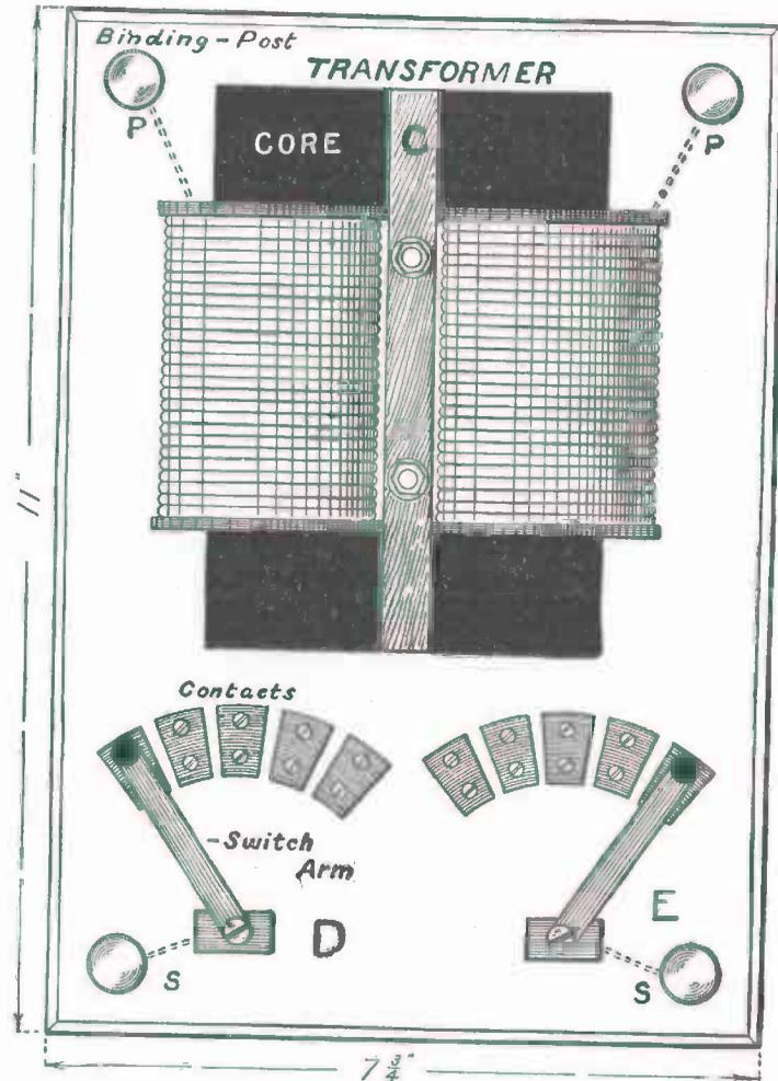
FIG. 191. — Top View of the Transformer.
