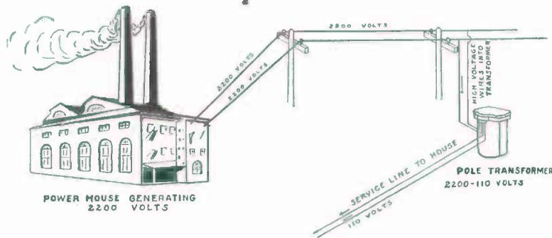
FIG. 176. — Alternating Current System for Light and Power.
