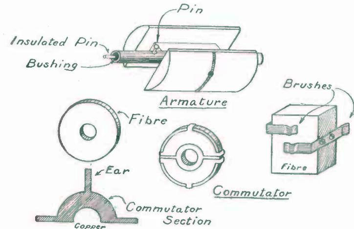
FIG. 253. — Details of the Armature, Commutator, and Brushes.
