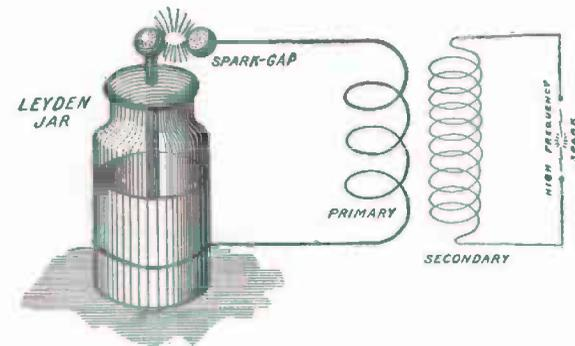
FIG. 317. — Illustrating the Principle of the Tesla Coil.
