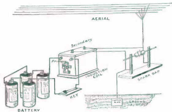
FIG. 194. — A Simple Transmitter.
