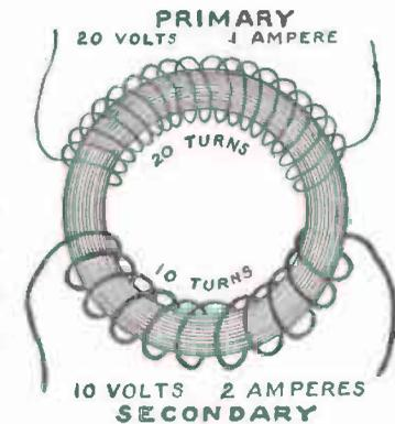
FIG. 179. — Step-Down Transformer.
