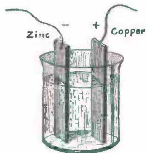
FIG. 52. — The Voltaic Cell.
