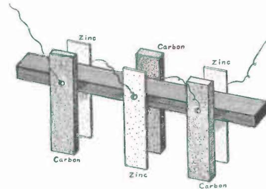
FIG. 63. — A Battery Element arranged for three Cells.
