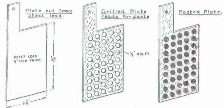
FIG. 71. — How to make the Plates for a Storage Cell.
