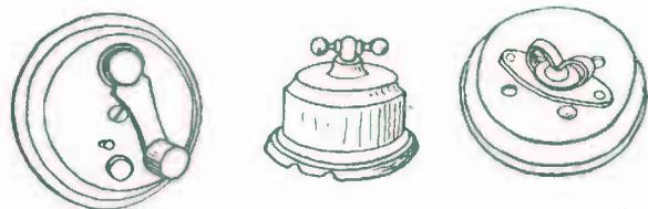
WOOD BASE SWITCH      SNAP SWITCH      CROWN SWITCH
