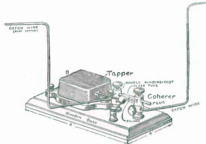
FIG. 233. — A Coherer and a Decoherer.
