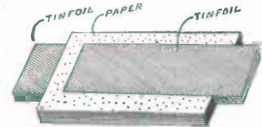
FIG. 215. — Building up a Fixed Condenser.
