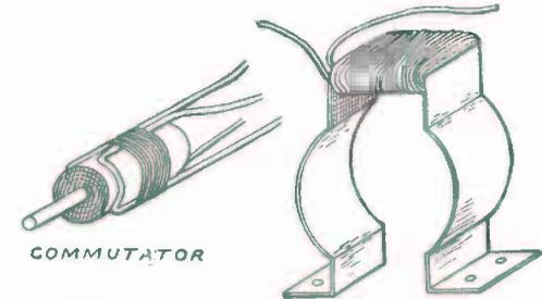
FIG. 246. — The Field and Commutator.
