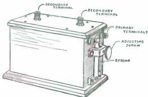
FIG. 221. — A Wireless Spark Coil.
