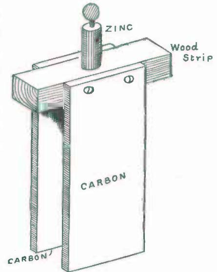
FIG. 61. — An Element made from two Carbon Plates and a Zinc Rod.
