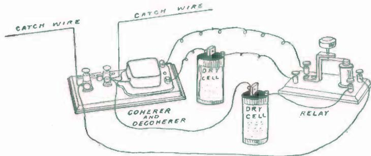
FIG. 236. — The Complete Coherer Outfit.
