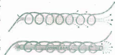
FIG. 82. — Showing how the Lines of Force "Leak" from a Coil of Wire, and how they are concentrated by an Iron Core.
