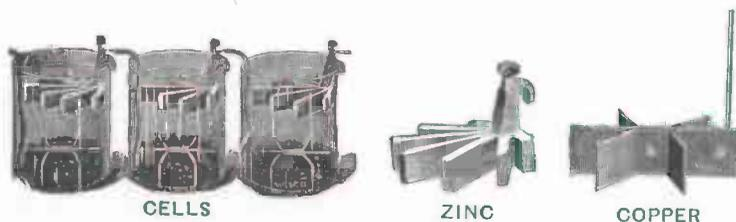
FIG. 75. — Gravity Cells.
