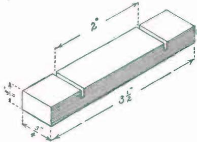
FIG. 272. — Details of a Wooden Tie.
