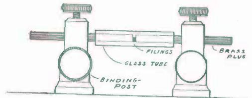
FIG. 234. — Details of the Coherer.
