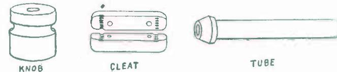
FIG. 90. — Porcelain Insulators to support Electric Light Wires.
