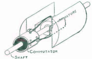
FIG. 258. — Diagram showing how to connect the Armature Winding to the Commutator.
