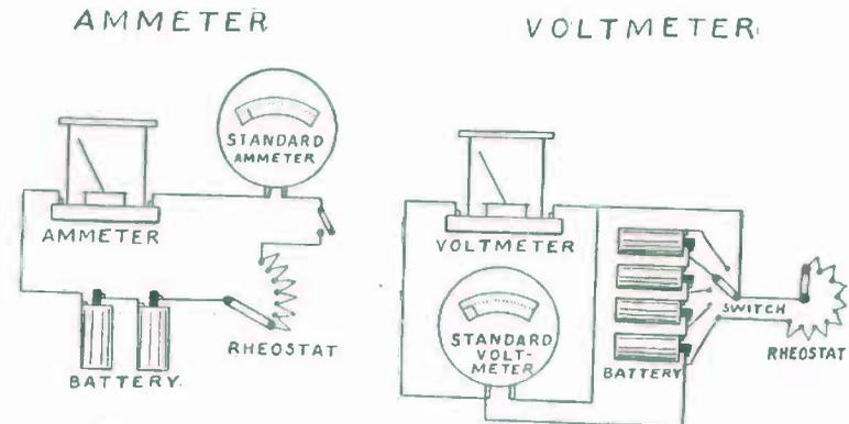
FIG. 109. — Circuits for Calibrating the Ammeter and Voltmeter.
