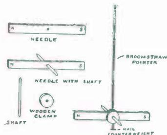
FIG. 103. — Arrangement of the Needle and Pointer.
