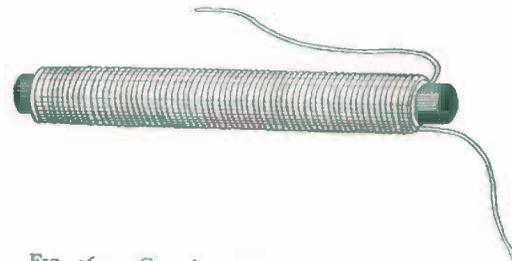
FIG. 160. — Complete Primary Winding and Core.
