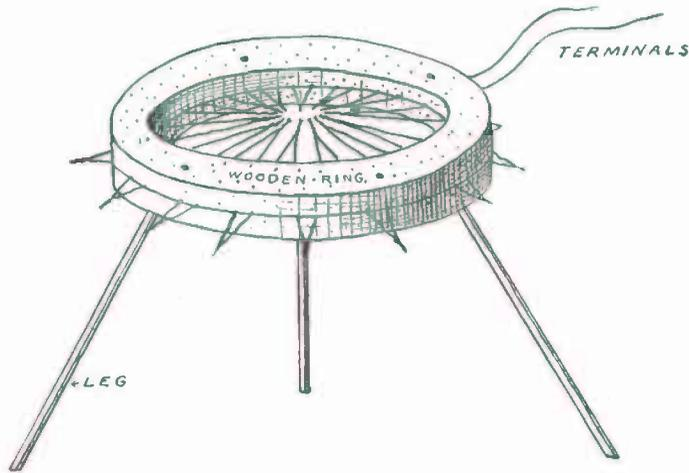
FIG. 305. — Complete Thermopile.
