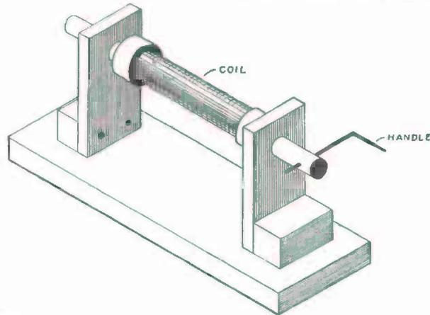
FIG. 162. — Simple Winding Device for winding the Secondary.
