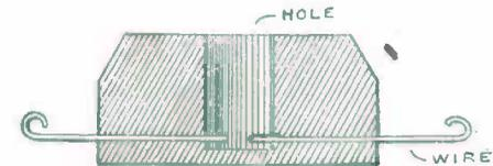
FIG. 46. — A Wooden Mortar for Igniting Gunpowder.
