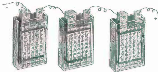
FIG. 74. — A Battery of Home-Made Storage Cells.
