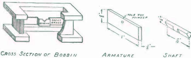
CROSS SECTION OF BOBBIN      ARMATURE      SHAFT
