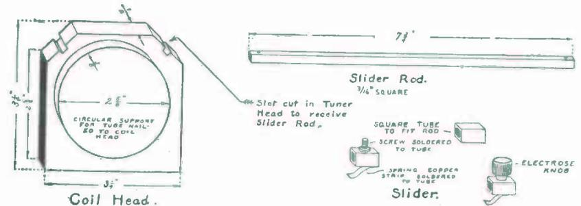
FIG. 201. — Details of the Tuning Coil.
