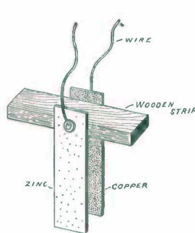
FIG. 53. — The Elements of Simple Voltaic Cell.
