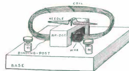
FIG. 111. — Galvanoscope.
