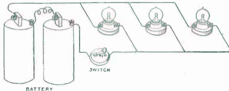
FIG. 287. — How Lamps are Connected in Multiple.
