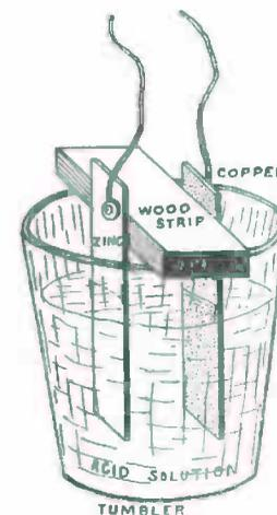
FIG. 54. — A Home-Made Voltaic Cell.
