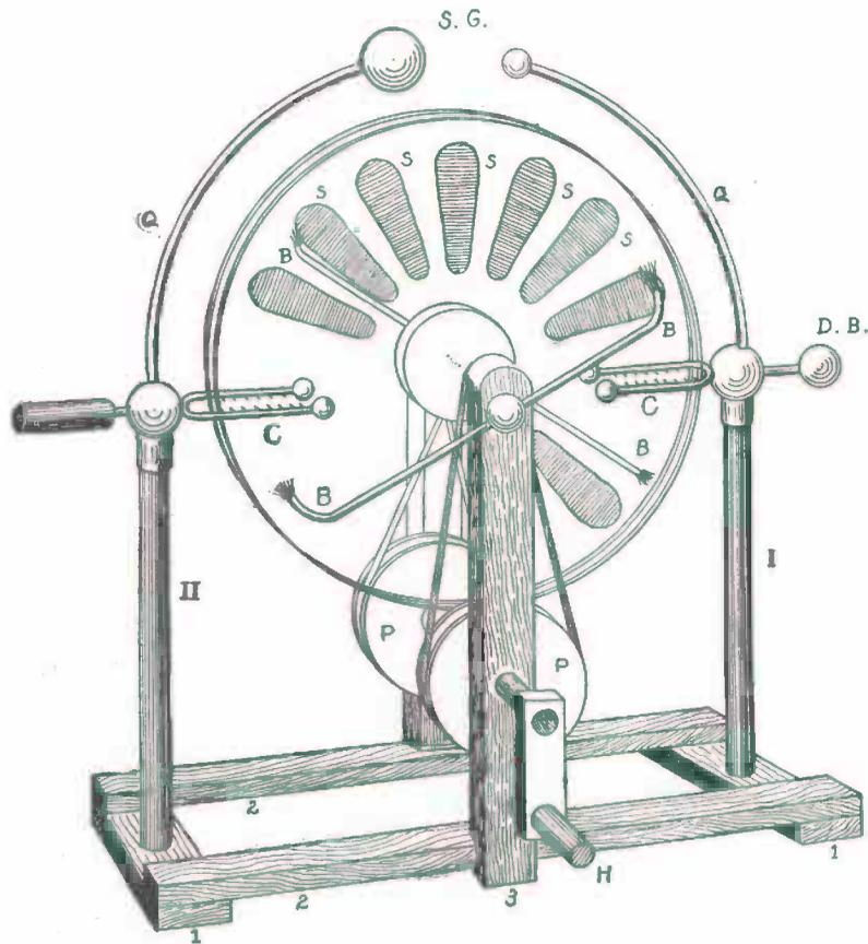
FIG. 44. — The Complete Wimshurst Electric Machine. B B B B, Brushes. C C, Combs. D B, Discharge Ball. I I, Glass Rods. H, Handle. Q Q, Quadrant Rods. S S S S S, Sectors. S G, Spark-Gap. P P, Driving-Wheels.
