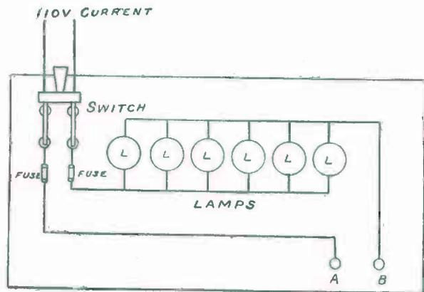
FIG 312. — Top View of Lamp Bank, showing how the Circuit is arranged.
