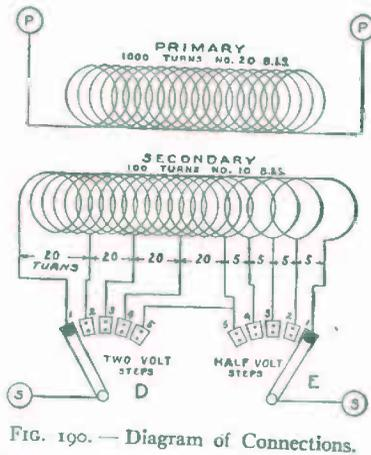
FIG. 190. — Diagram of Connections.
