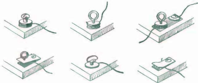
FIG. 93. — Home-made Binding-Posts.
