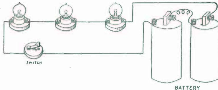
FIG. 288. — How Lamps are Connected in Series.
