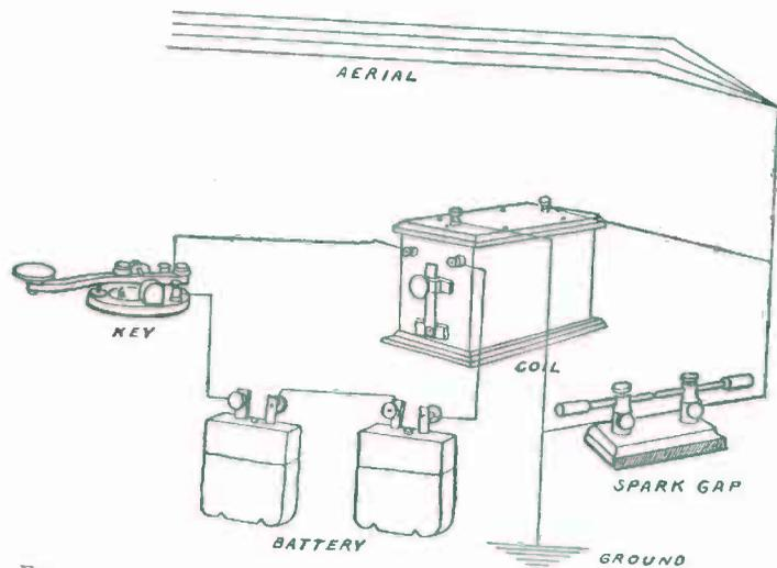
FIG. 223. — Diagram showing how to connect a Simple Transmitter.
