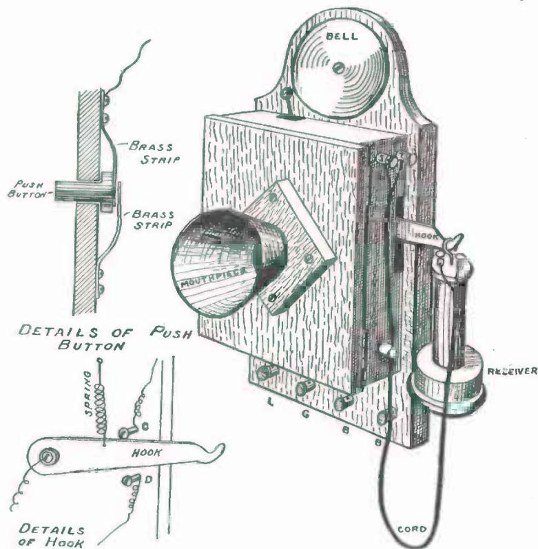
FIG. 149. — A Complete Telephone Instrument.
