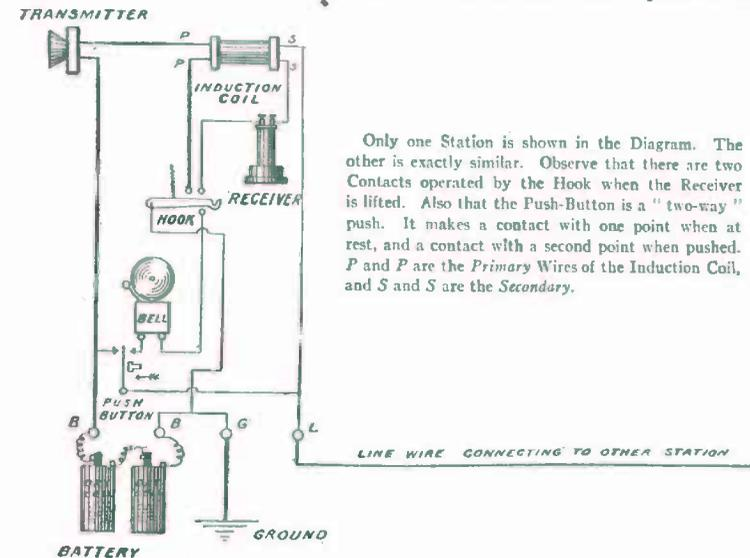
Only one Station is shown in the Diagram. The other is exactly similar. Observe that there are two Contacts operated by the Hook when the Receiver is lifted. Also that the Push-Button is a "two-way" push. It makes a contact with one point when at rest, and a contact with a second point when pushed. P and P are the Primary Wires of the Induction Coil, and S and S are the Secondary.
