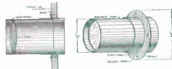
FIG. 307. — How the Lens is Arranged and Mounted.
