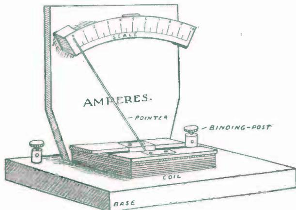
FIG. 105. — The Completed Meter.
