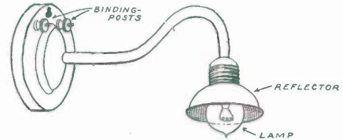
FIG. 290. — A Lamp Bracket for Miniature Lighting.
