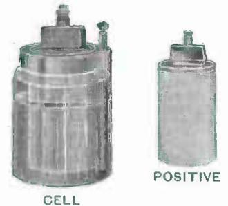
FIG. 56. — A Leclanche Cell, showing the Porous Cup.
