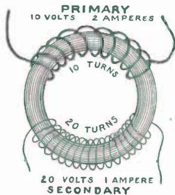
FIG. 178. — Step-Up Transformer.
