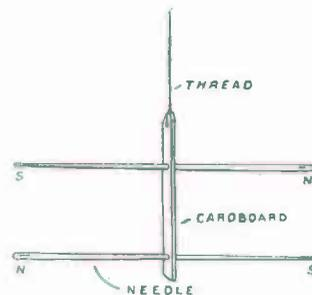
FIG. 113. — Astatic Needles.
