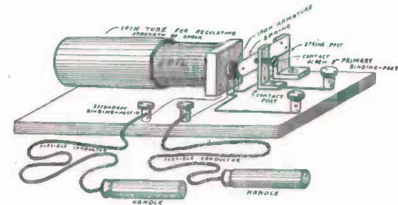
FIG. 156. — Completed Medical Coil.
