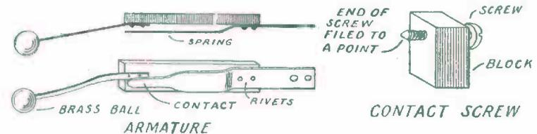
FIG. 120. — Details of the Armature, and Contact Screw.
