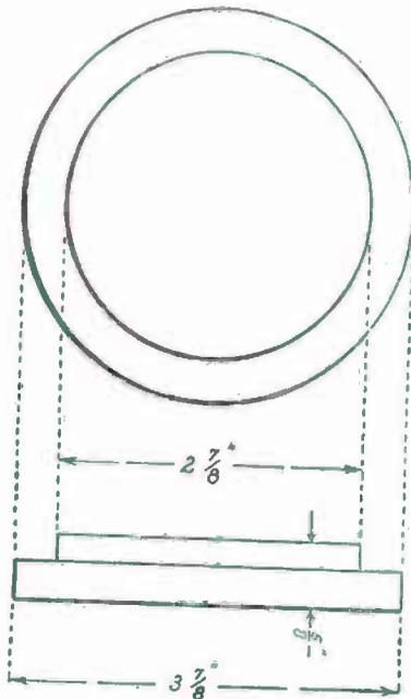
FIG. 320. — The Secondary Head.
