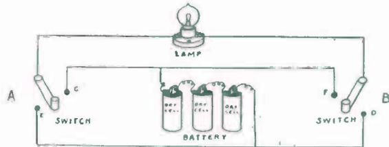
FIG. 289. — Three-way Wiring Diagram.
