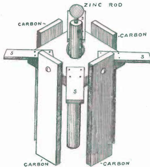
FIG. 62. — A Method of Mounting four Carbon Plates.
