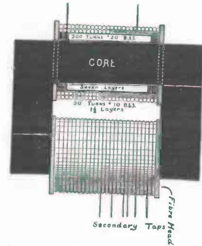
FIG. 186. — The Transformer completely Wound and ready for Assembling.
