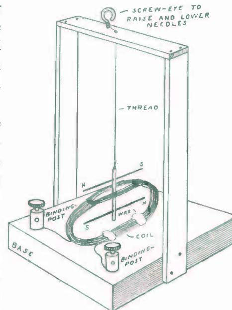
FIG. 112. — Astatic Galvanoscope.
