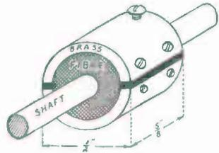
FIG. 257. — Details of the Commutator.
