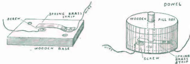
FIG. 123. — Two Simple Push-Buttons.
