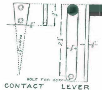
FIG. 188. — Details of the Switch Parts.
