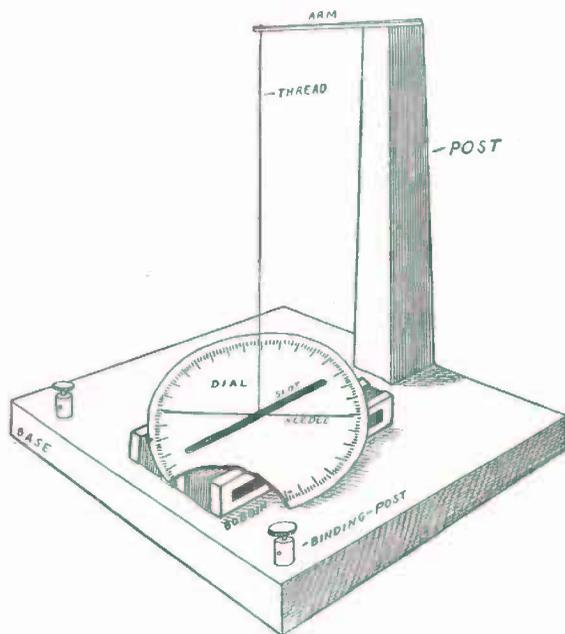
FIG. 115. — Completed Astatic Galvanometer.
