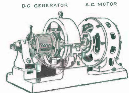
FIG. 177. — Motor Generator Set for changing Alternating Current to Direct Current.
