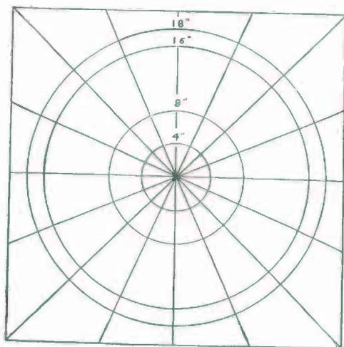
FIG. 34.— Paper Pattern for laying out the Plates.
