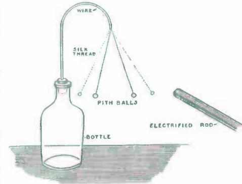
FIG. 23. — A Double Pith-Ball Electroscope.
