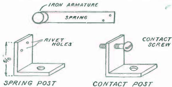
FIG. 155. — Details of Interrupter for Medical Coil.
