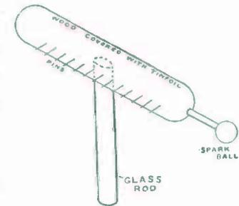
FIG. 32. — The Prime Conductor or Collector.
