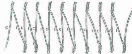
FIG. 303. — How the Copper Wires (C) and the German Silver Wires (I) are twisted together in Pairs.
