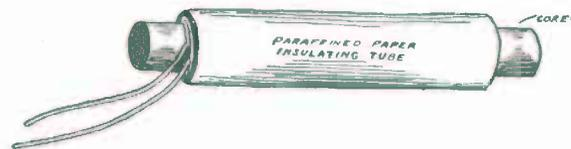
FIG. 161. — The Primary covered with Insulating Layer of Paper ready for the Secondary.
