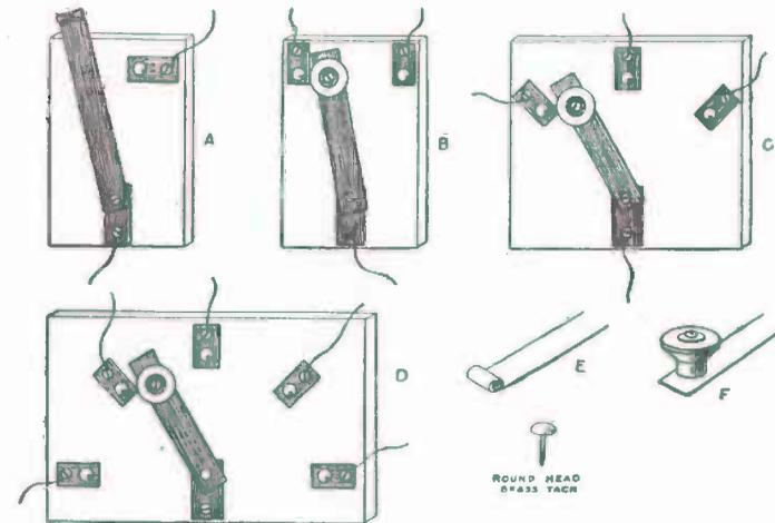
FIG. 95. — Simple Switches.
