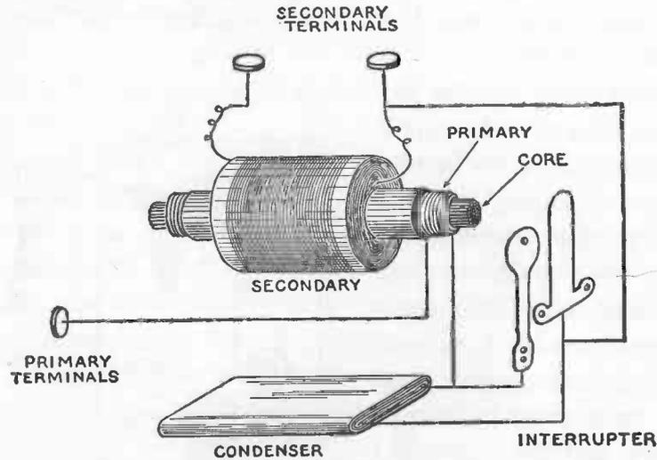
INSIDE THE MODEL "T" SPARK COIL
