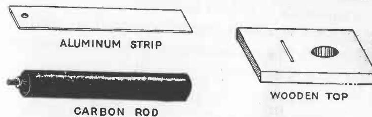
PARTS FOR AN ELECTROLYTIC RECTIFIER CELL
