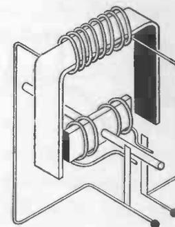
The field of a shunt motor is wound with more turns and with finer wire than a series motor of the same size. It is connected so that part of the current goes through the field and part through the armature. In a series motor all of the current that goes through the field also passes through the armature.
