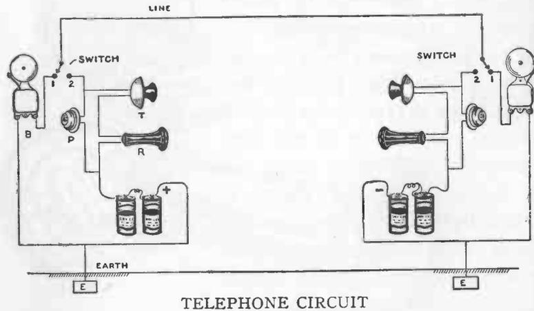
Notice that the positive terminal of one battery and the negative of the other are connected to earth. 1 is the "Ring" position of the switch and 2 the "Talk" position. *B* is a doorbell, *P* a push button, *T* the transmitter and *R* a telephone receiver.
