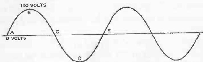
A PICTURE OF A SINGLE-PHASE ALTERNATING CURRENT
