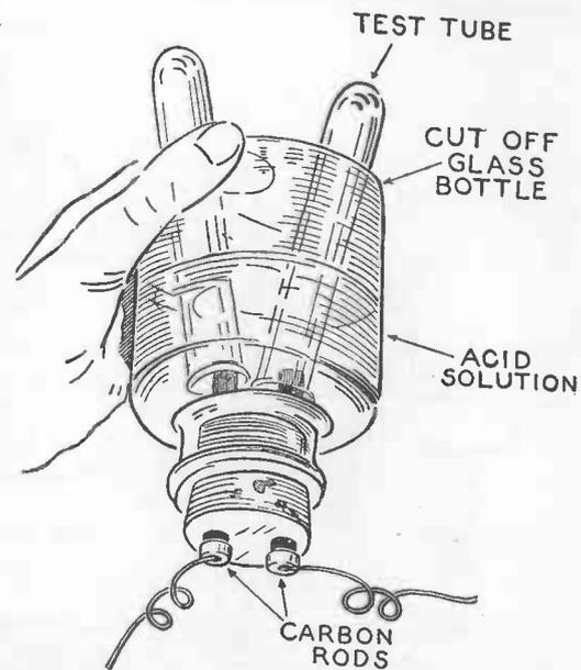
SIMPLE APPARATUS FOR PRODUCING OXYGEN AND HYDROGEN AND COLLECTING IN TEST TUBES
