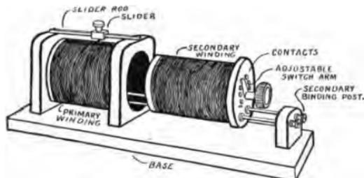
FIG. 91.—Loose coupled tuning coil.
