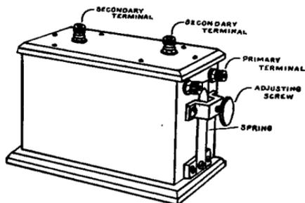
FIG. 35.—Induction coil for wireless telegraph purposes.
