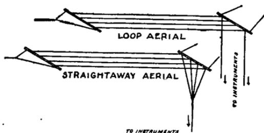
FIG. 23.—Diagram showing the difference between "loop" and "straightaway" aeriels.
