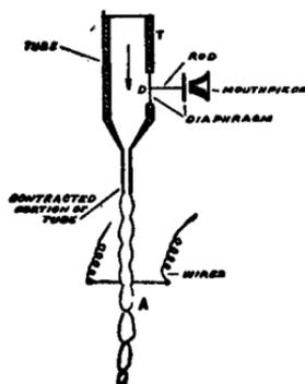
FIG. 148.—The Majorana wireless telephone transmitter.
