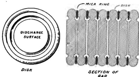
FIG. 53.—Quenched spark gap.
