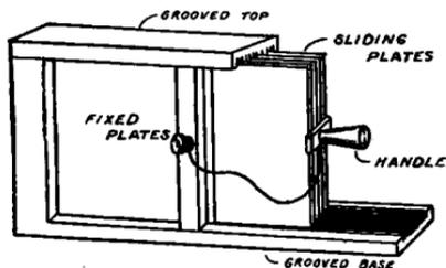
FIG. 84.—Sliding plate variable condenser.
