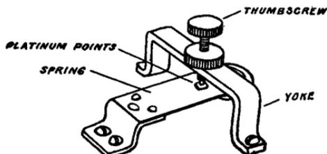
FIG. 37.—Interrupter for induction coil.
