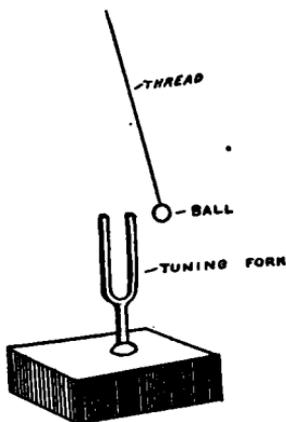
FIG. 123.—Experiment showing sounding bodies are in vibration.
