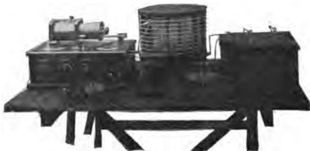
FIG. 99.—Complete receiving and transmitting outfit.
