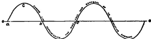
FIG. 41.—Diagram representing alternating current.
