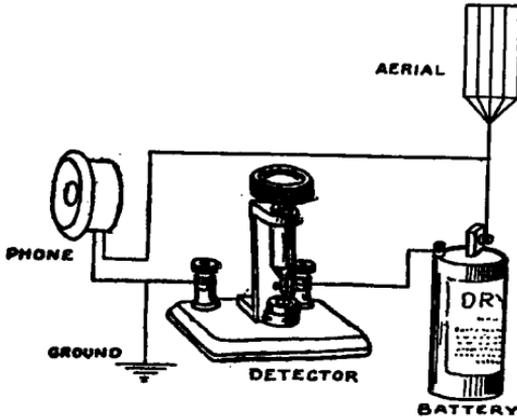
FIG. 73.—Electrolytic detector in circuit.
