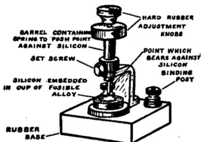
FIG. 71.—Silicon detector.
