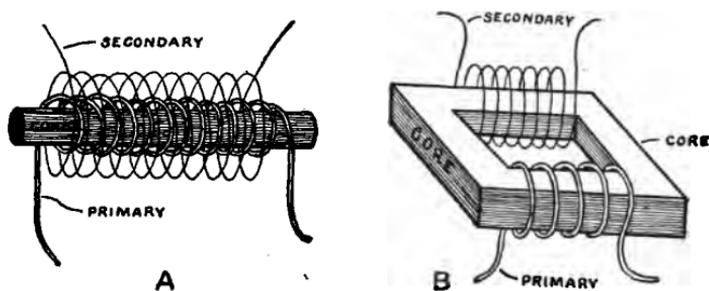
FIG. 39.—Open and closed core transformers.
