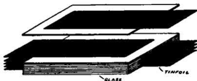
FIG. 46.—Diagram showing construction of condenser.
