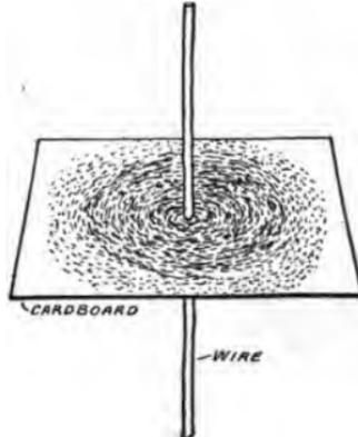
FIG. 32.—Magnetic phantom formed by wire carrying current.
