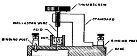
FIG. 72.—Electrolytic detector.
