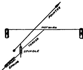
FIG. 89.—The principle of the hot-wire ammeter.
