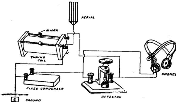
FIG. 79.—Diagram showing fixed condenser in circuit.
