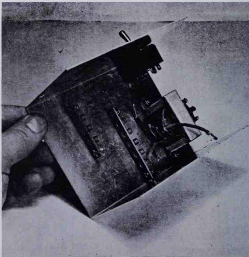
Fig. 9-2. Mounting the terminal strips, switch, and transformer.
