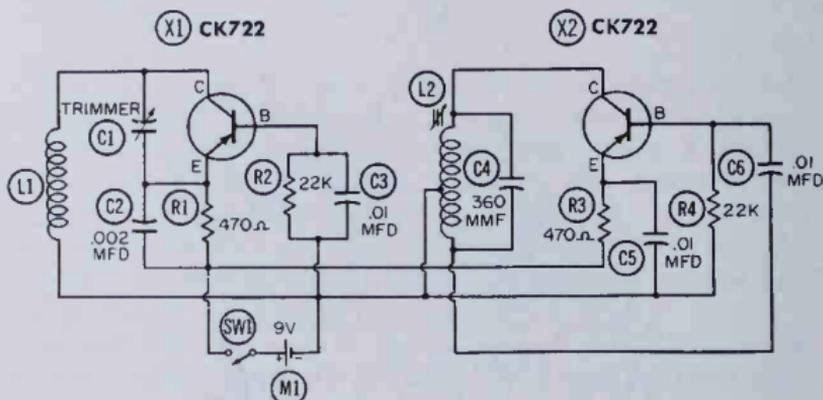
Fig. 7-3. Schematic diagram.
