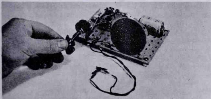
Fig. 8-1. The finished flip-flop circuit board.
