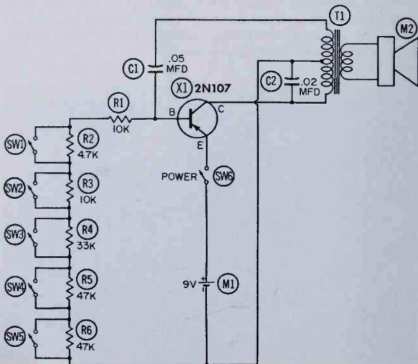
Fig. 9-6. Schematic diagram.
