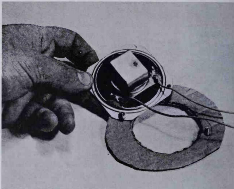
Fig. 11-8. Preparing the speaker mounting.
