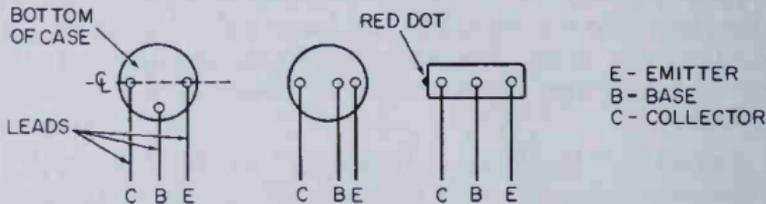
Fig. 1-2. How to identify transistor leads.
