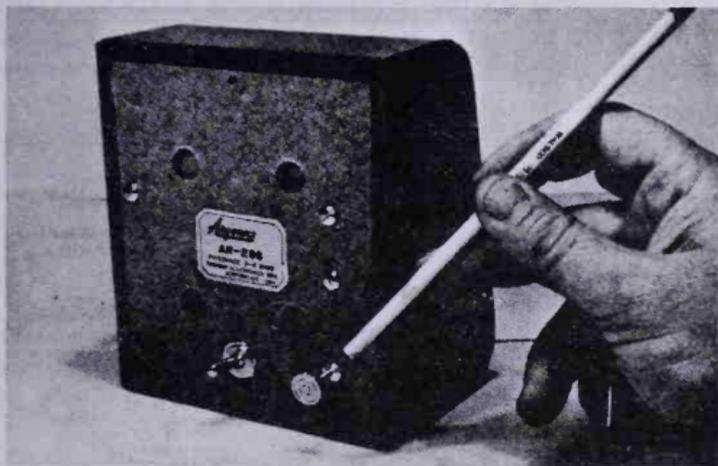
Fig. 6-6. Location of coil knob and control switch.
