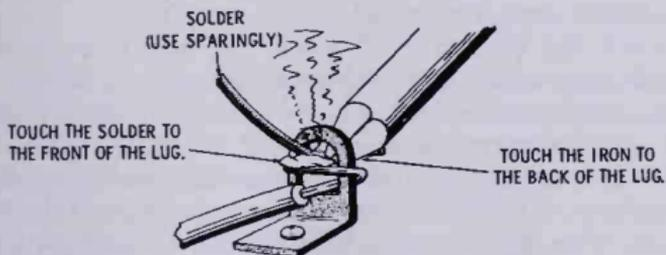
Fig. 1-4. Touch solder to the heated joint, not to the iron.
