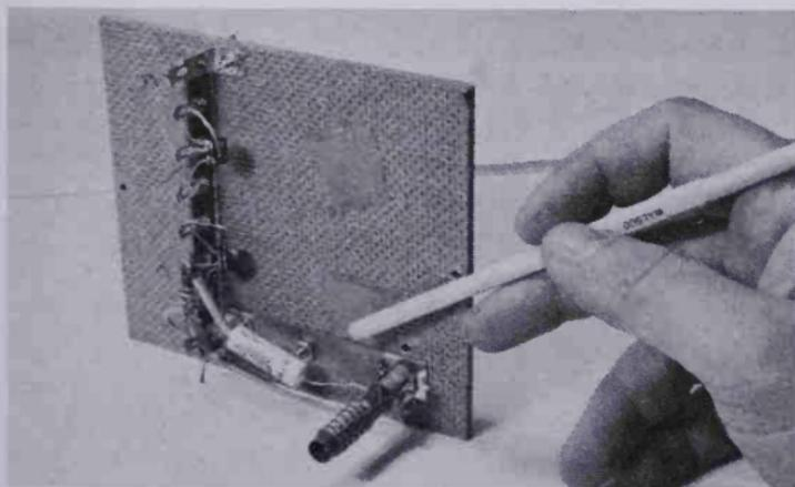
Fig. 6-3. Mounting the coil.
