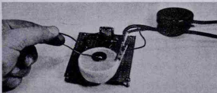
Fig. 3-1. The completed lemon-juice oscillator.
