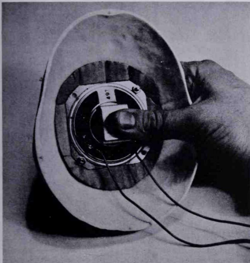
Fig. 11-9. Mounting the speaker.
