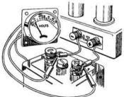
Fig. 85 .- The correct way to test the voltage of an accumulator is while it is under load, that is, while it is connected to the set and switched on.
