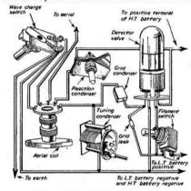
Fig. 63.—A typical detector stage in pictorial form.
