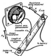
Fig. 79.—A practical arrangement of the simple bridge shown by Fig. 78.
