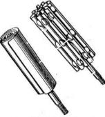
Fig. 50.—Two typical anode designs used in electrolytics.
