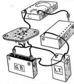
Fig. 88.—Set-up for taking valve measurements.
