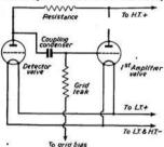
Fig. 67 .- Theoretical circuit of an R.C. coupling.
