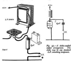
There are two types of output filters—the output choke and the transformer.
