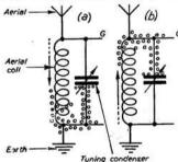
Fig. 59 (a) and (b).—Diagram illustrating the flow of electric currents in the aerial circuit of a vector. The electrons first flow to one end of the tuning circuit as at (a), and then to the other end, as at (b).
