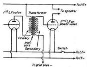
Fig. 70.—Theoretical circuit of transformer-coupled stage. valve, and what
