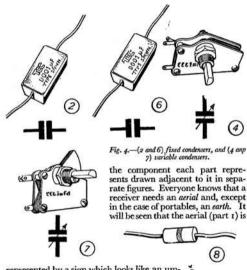
represented by a sign which looks like an umbrella that is blown inside out, and the earth (part 13) by a series of parallel lines gradually · diminishing in length so that they form an inverted cone. There are many types of aerial, both indoor and outdoor and, in the case of portable receivers, frame aerials which are
