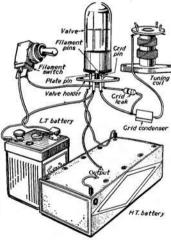
Fig. 65.-Battery connections.
