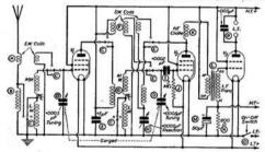
Fig. 73.-Theoretical circuit of a modern three-valve receiver.
