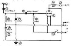
Fig. 1.—Circuit diagram of a simple one-volver for medium wavebands only. A fictorial diagram of the receiver built from this circuit is given on fage 17 Where crossing lines are connected by a dot, they are to be joined by solder, or connected to a terminal.
