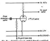
Fig. 69.—Grid-bias may be applied through a grid-leak.
