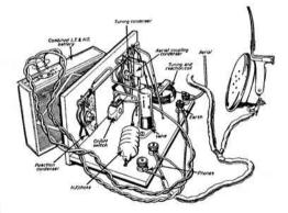
Fig. 10.—Pictorial wiring diagram of circuit shown by Fig. 1. Some of the wiring is underneath the baseboard, which is fixed to the band about an inch from the bottom edge to clear the value holder sockets.
