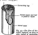
Direct Anode Bypass Condenser, ·0001-·0005 µF.
