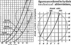
Figs. 86 and 87 .- (Left) The grid-volts anode curve. (Right) An enlarged view of the circled section.
