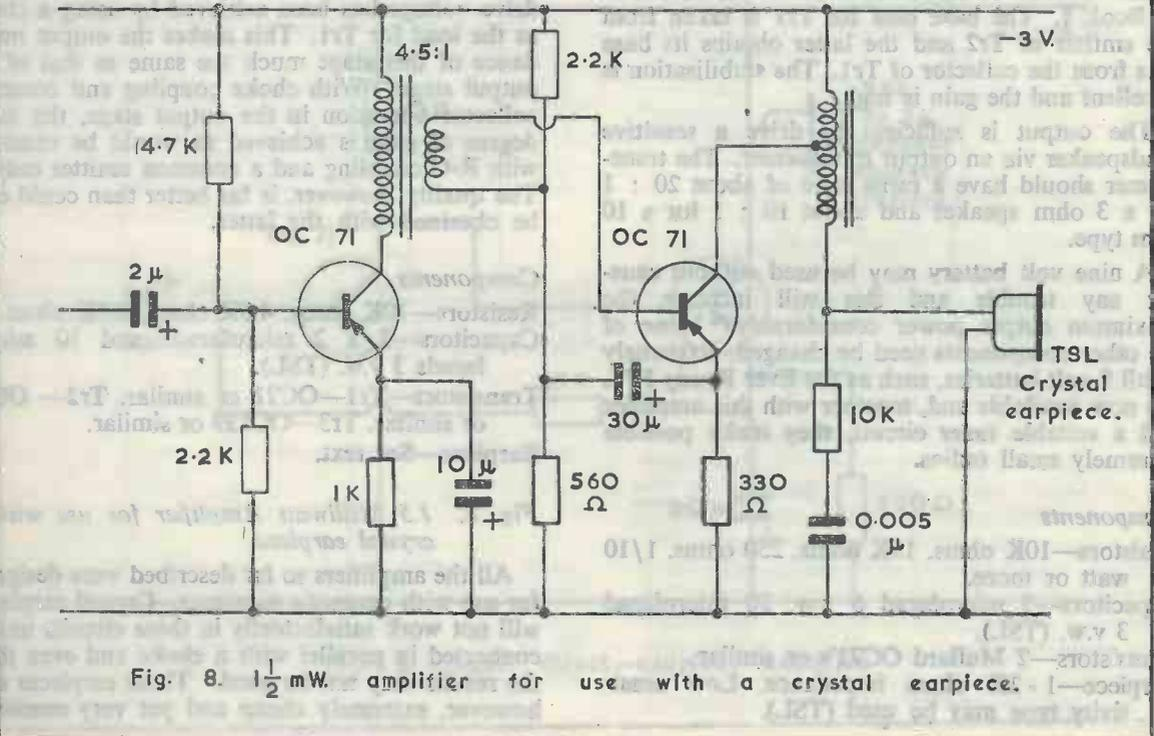
Fig. 8. 1/2 mW amplifier for use with a crystal earpiece.
