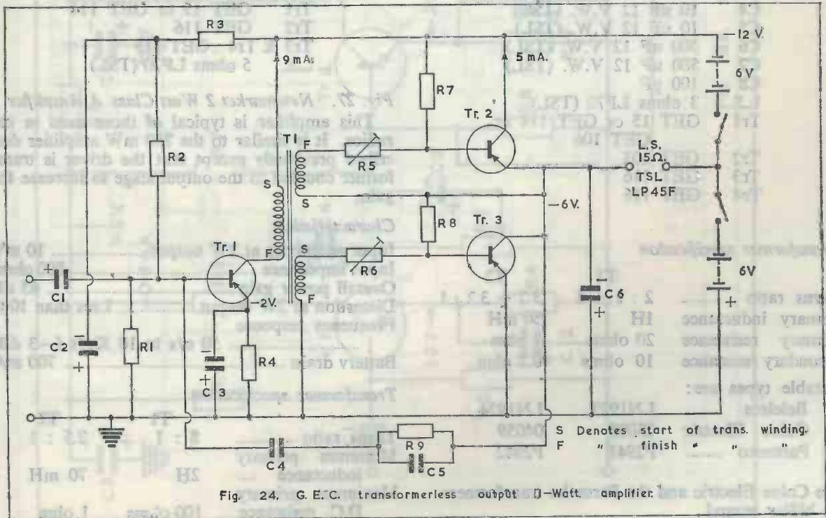
Fig. 24. G.E.C. transformerless output 1-Watt amplifier.
