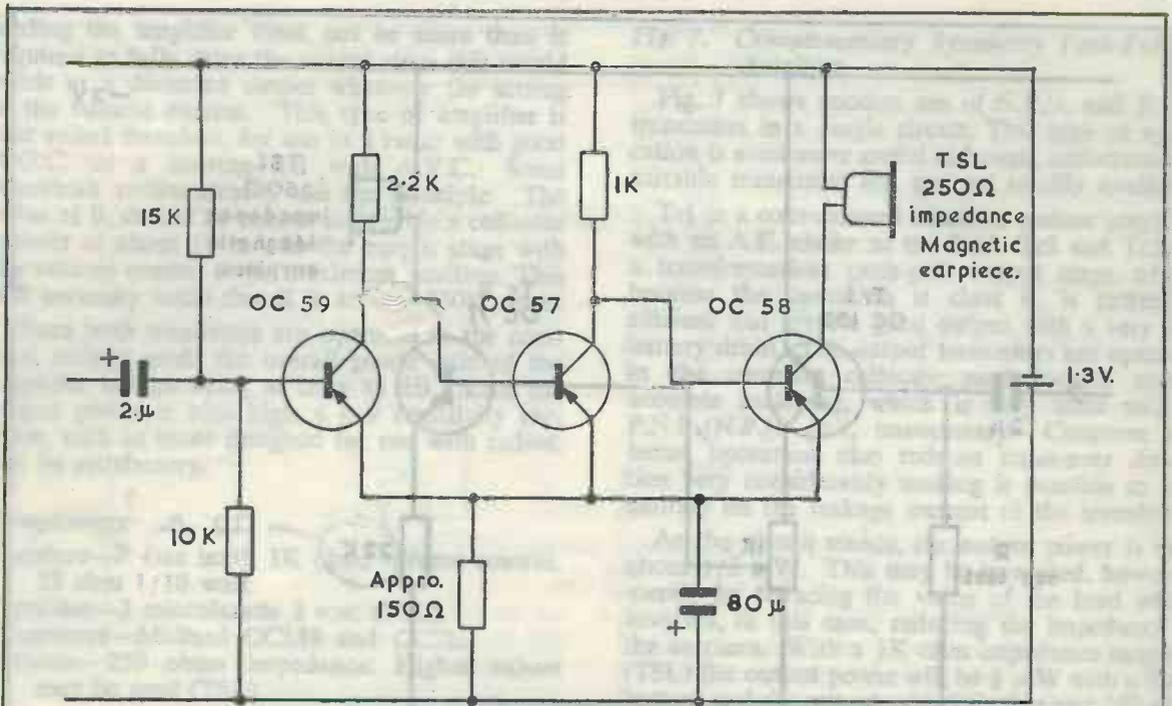
Fig. 3. A 2 mW. directly coupled amplifier.
