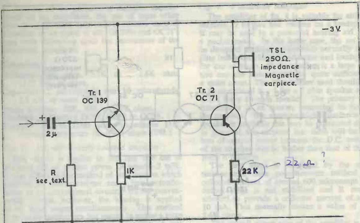
Fig. 5. Direct coupled amplifier with low battery drain.
