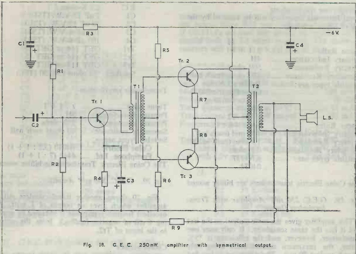
Fig. 18. G. E. C. 250mW. amplifier with symmetrical output.
