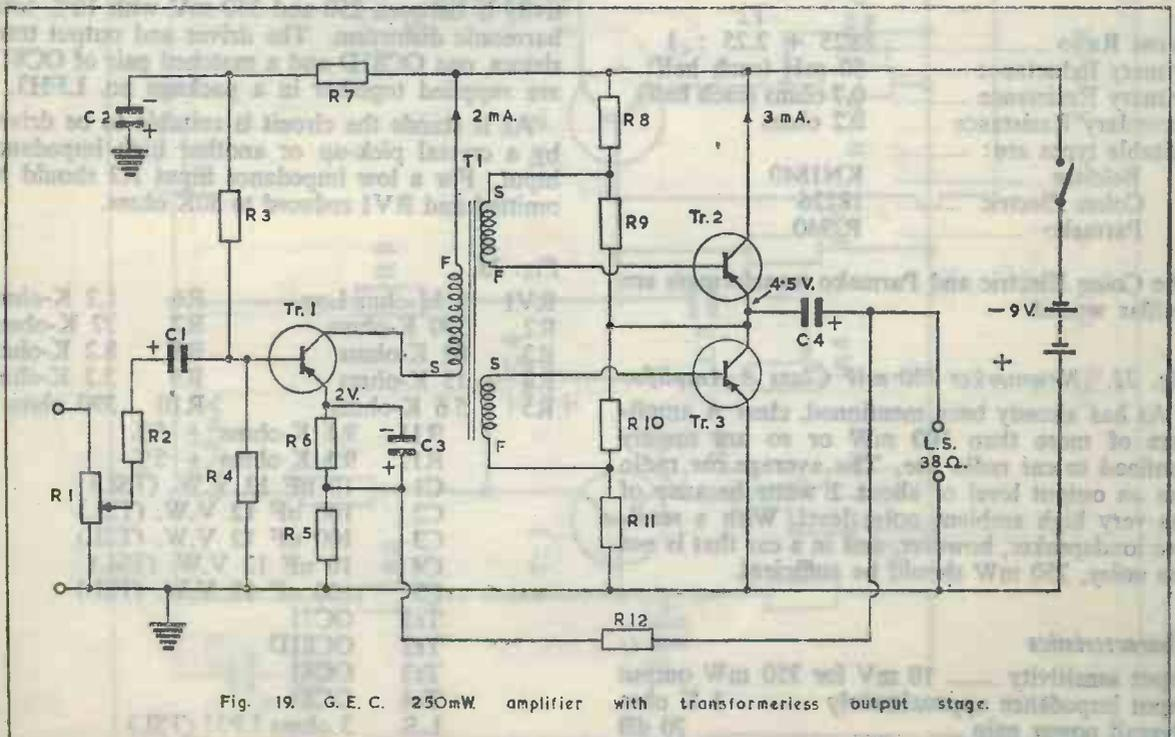
Fig. 19. G. E. C. 250mW amplifier with transformerless output stage.
