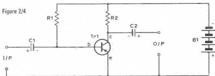
Note in our circuit of figure 4 that the capacitors are electrolytics. This is an indication that the circuit is intended to amplify low frequencies, such as audio frequencies (abbreviated to a.f.).
