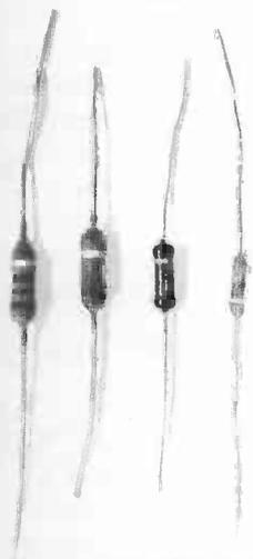
Figure 1/3 small fixed resistors
