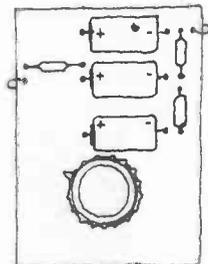
In this chapter we are going to build a two-transistor audio amplifier. In order to make the most use of our components, the amplifier has been designed especially so that it will allow you to plug the simple crystal receiver into it and thus amplify the signals sufficiently for them to be heard on a small loudspeaker. The amplifier may further be used with the other two receivers described later on.
