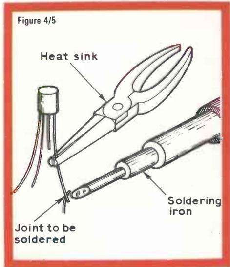
junctions can ruin the transistor. The wiring-in of transistors should therefore be left to the very last, as it is all too easy to touch the leads with the soldering iron accidentally when soldering in another component. To safeguard against damaging the transistor we use a 'heat shunt', so called because it 'shunts' some of the heat away from the transistor.
