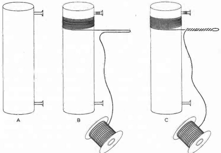
**Soldering** The copper wire is insulated by the coating of enamel, so when you want to solder it you must first remove the enamel coating. For this it is best to use a small piece of emery cloth, although sand paper will do at a pinch. Gently draw the wire between the sides of the abrasive; this will expose the bright copper underneath. Make sure that there is no enamel left on the wire where you
