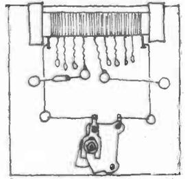
This type of receiver is just about the simplest and cheapest there is. It is practically foolproof too, since a mistake in the wiring will simply prevent the set from functioning properly, but it will not damage any of the components. The wiring fault will usually show itself as (a) the receiver not working at all or (b) the receiver functioning at greatly reduced volume.
