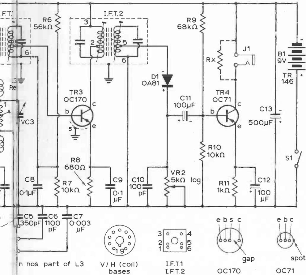
which plug into the jack socket J1. A separate on/off switch S1 breaks the positive lead to the battery when the set is off. Capacitor C13 is used from the negative supply rail to earth to short to earth any a.c. signals which might find their way on to the supply line.
