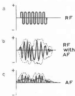
In figure 2a we have a symbolic drawing of a radio wave. It is simply an r.f. wave. A Morse signal consists of a wave like this, the wave being interrupted or broken up into dots and dashes. In figure 2b we have an r.f.
