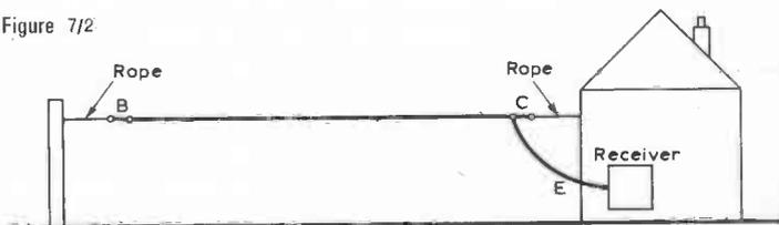
The length from the post or tree to the insulator can be rope, preferably weather-proofed. This also applies to the length from the other insulator to the house. Fifty feet is quite a good length to start with. It is best to keep it in a straight line but if not, try bending it around the garden. It will still work and you can bend it different ways to see which layout gives the best reception.
