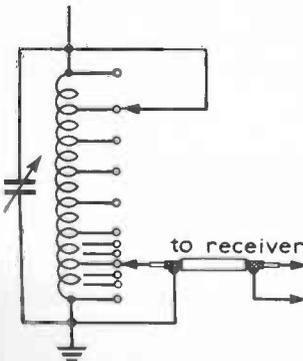
It is sometimes useful to add a capacitor as in figure 5. In this case the capacitor can be varied or tuned as well as the inductance. This coil and/or capacitor combination used in this way is called an Aerial Tuner Unit or a.t.u. It may be used with longwire aerials or verticals and a practical circuit is shown in figure 6. This coil is wound exactly as for the simple crystal set, but there are more tapping points. The capacitor could be  $300\mu\text{F}$ .
