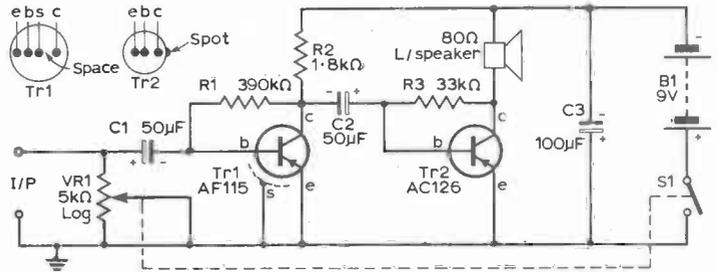
doesn't short out any of the resistor VR1, and thus all the signal is fed into the amplifier, corresponding to maximum volume. Capacitor C1 will allow the a.c. signal to pass on, but will prevent any d.c. passing which might upset the voltage on the base of transistor Tr1. Note that this capacitor is an electrolytic and must be connected the right way round. The positive end will either be marked with a + sign, or will have a red dot.
