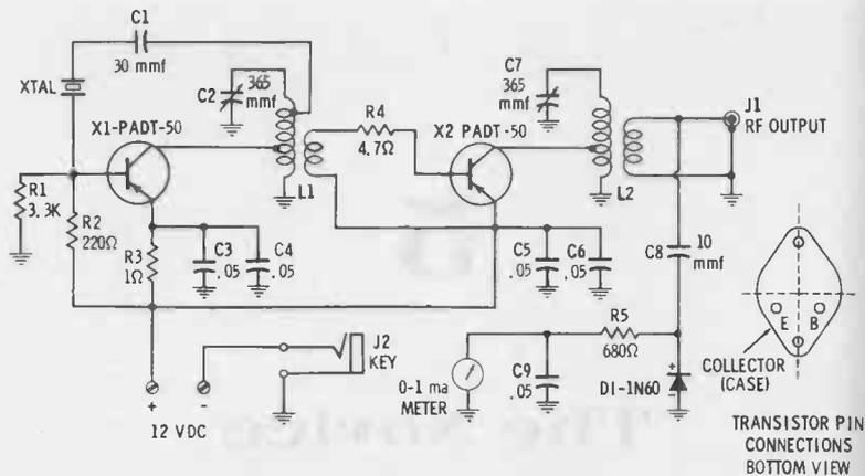
Fig. 5-1. Schematic of the "Novice Powerhouse" transmitter.
