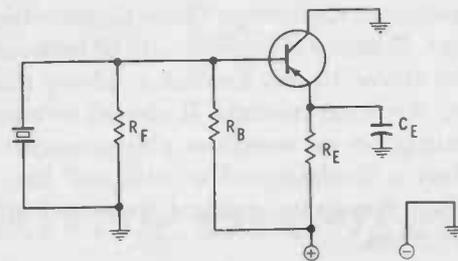
Fig. 2-24. Unusual transistor oscillator circuit.
