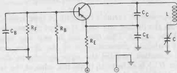
Fig. 2-15. Alternate Clapp oscillator circuit.
