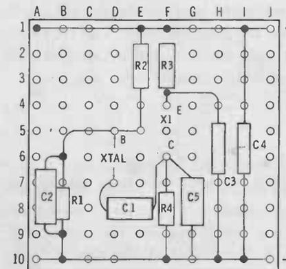
Fig. 3-3. Layout of the crystal checker.
