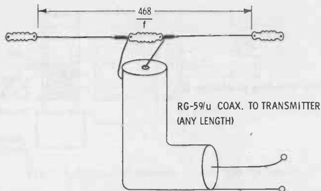
Fig. 3-12. Suggested antenna for the "CB Cyclone."
