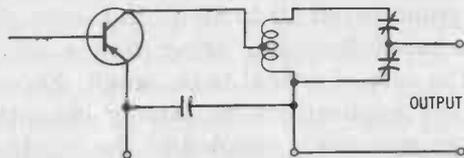
Fig. 4-6. Tapped coil for output impedance matching.
