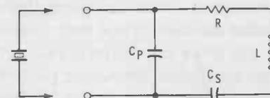
represent the mechanical vibration characteristics of the crystal. These three components will exhibit a low impedance at one frequency, which is determined primarily by the physical dimensions of the quartz and which, in turn, determines its vibrating characteristics. This point is called the series-resonant frequency of the crystal.
