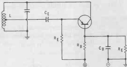
Fig. 2-9. Common-base Hartley oscillator.
