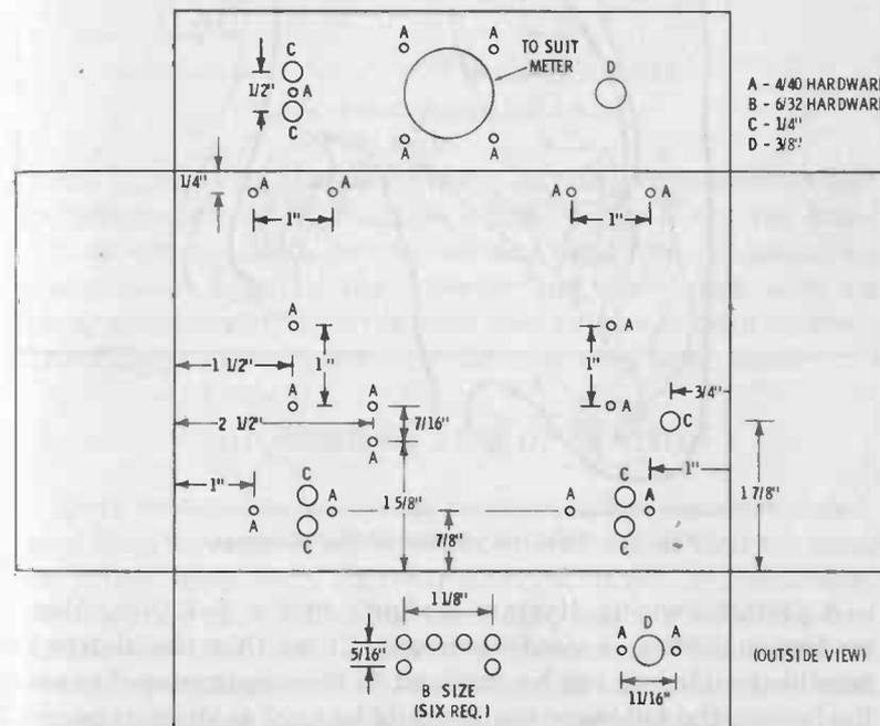
Fig. 5-3. Chassis layout for Novice Powerhouse transmitter.
