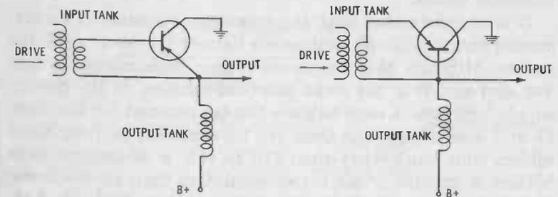
(A) Common emitter, grounded collector.
