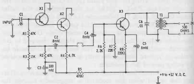
Fig. 6-9. Schematic diagram for the high-impedance microphone preamplifier and modulator.
