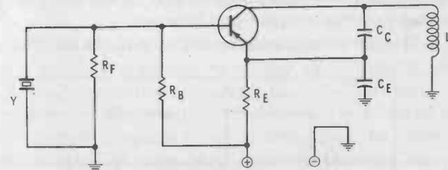
Fig. 2-21. Alternative version of Colpitts, crystal controlled.
