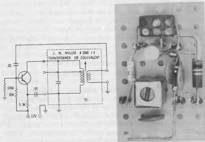
Fig. 2-6. Practical circuit of a tickler-coil oscillator.
