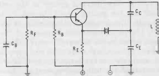
Fig. 2-20. Crystal-controlled version of the Colpitts oscillator.
