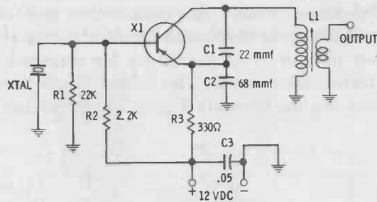
Fig. 3-8. Schematic diagram of the "CB Cyclone."
