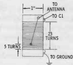
Fig. 4-10. Winding details for L1 in Fig. 4-8.
