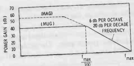
Fig. 1-8. High-frequency characteristics of typical transistor.
