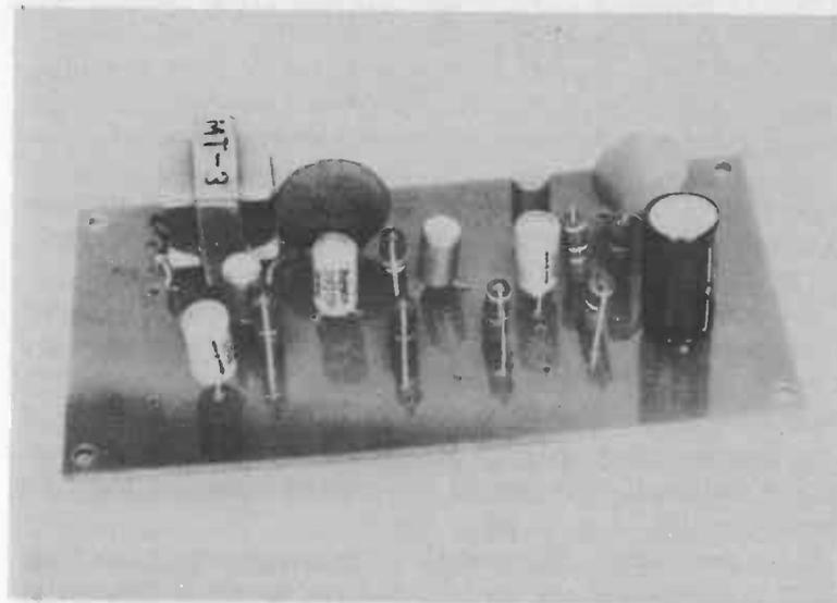
Fig. 6-11. Completed low-power modulator.
