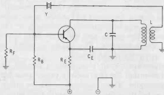
Fig. 2-18. Crystal-controlled version of a tickler-coil oscillator.
