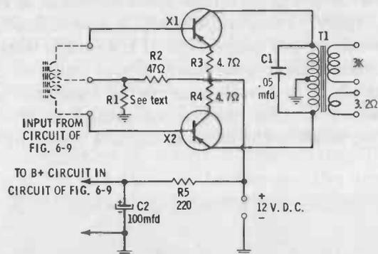
Fig. 6-12. Schematic of the half-watt modulator.
