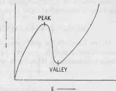
Fig. 7-4. EI characteristic curve of a typical tunnel diode.
