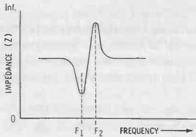
Fig. 2-17. Impedance-versus-frequency curve of a crystal.
