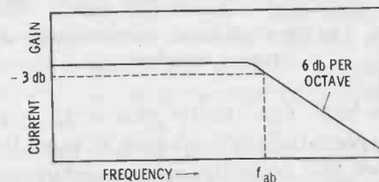
Fig. 1-7. Alpha-cutoff frequency curve.
