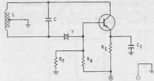
Fig. 2-19. Crystal-controlled equivalent of a Hartley oscillator.
