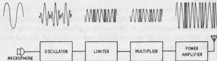
Fig. 6-2. Waveforms found in a typical FM transmitter.
