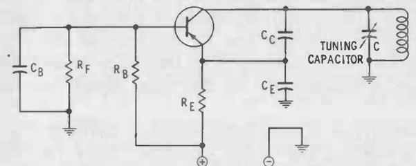
Fig. 2-13. Colpitts with tuning capacitor.
