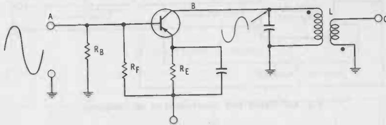
Fig. 2-4. PNP RF-amplifier circuit.
