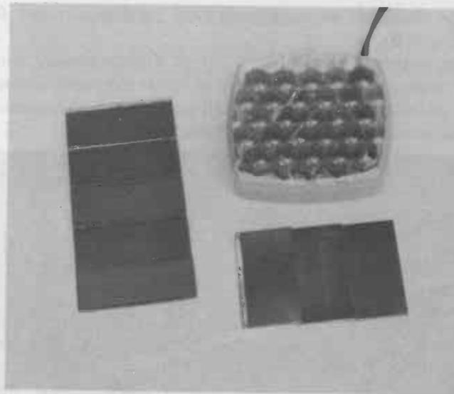
Fig. 7-8. Light-power solar cells.
