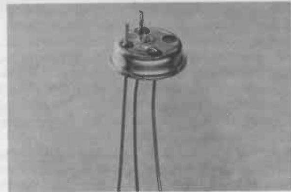
Fig. 1-3. Construction of a typical transistor.
