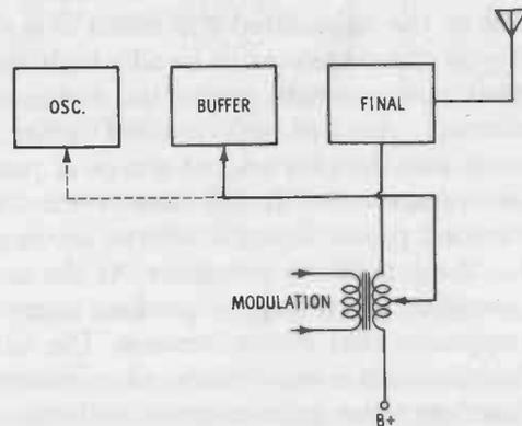
Fig. 6-7. Preferred method of modulating both driving and final stages.
