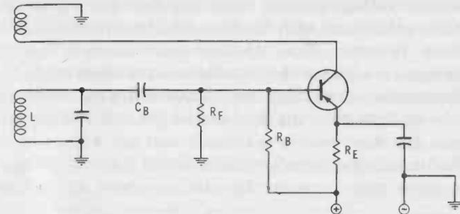
Fig. 2-7. Alternate tickler-coil oscillator circuit.
