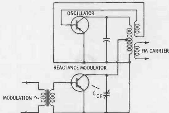
Fig. 6-1. A basic reactance-modulated oscillator circuit. Bias and voltage omitted for simplicity.
