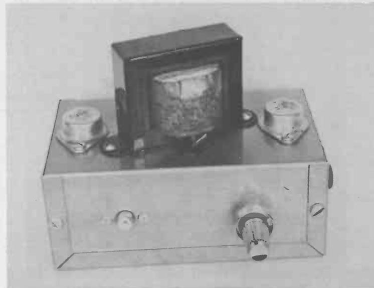
Fig. 6-16. Finished 5-watt modulator.
