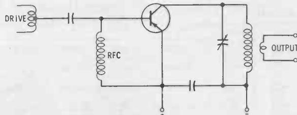
Fig. 4-3. Power amplifier with a tapped coil for input impedance matching.
