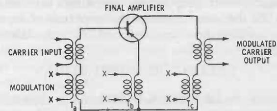
Fig. 6-3. Basic method of modulating an AM transistor transmitter. Only one of the three transformer connections would be used.
