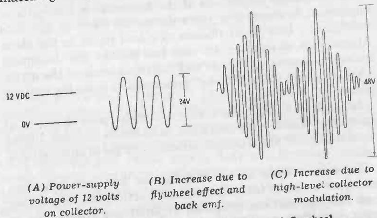
Fig. 1-9. Voltage increase due to back emf, flywheel effect and high-level modulation.
