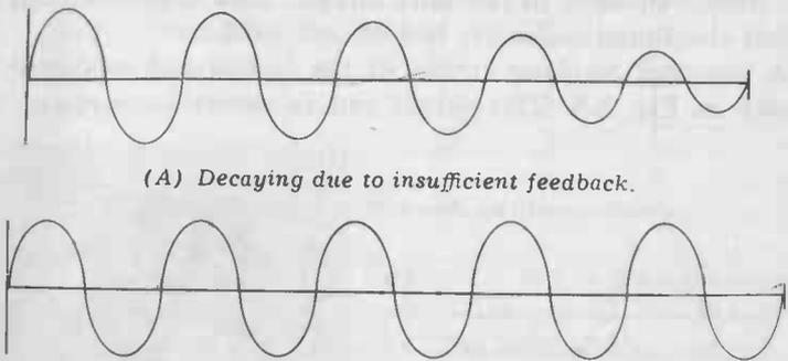
(A) Decaying due to insufficient feedback.
