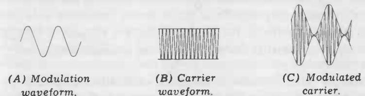
Fig. 6-4. The amplitude of the modulation waveform increases or decreases the carrier amplitude.
