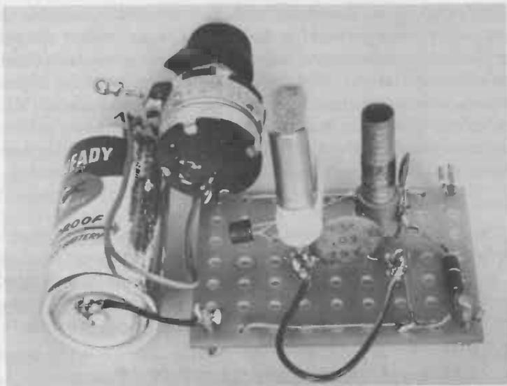
Fig. 7-7. The tunnel-diode transmitter.
