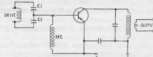
Fig. 4-4. Power amplifier with capacitive divider for input impedance matching.
