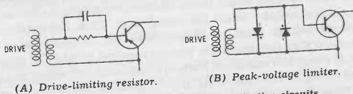
Fig. 1-10. Base-emitter breakdown protective circuits.
