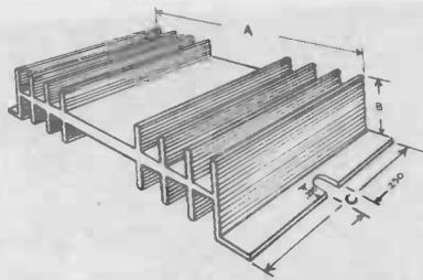
Fig. 1-4. Commercially built heat sink.
