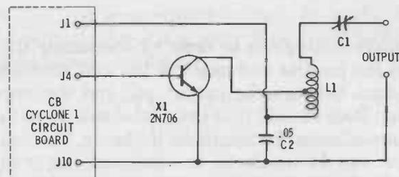
Fig. 4-11. Schematic for the "CB Cyclone II" power amplifier.
