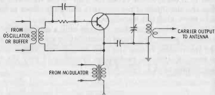
Fig. 6-5. Output circuit of a typical AM transistor transmitter.
