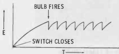
Fig. 7-3. Waveform generated by the circuit shown in Fig. 7-1.
