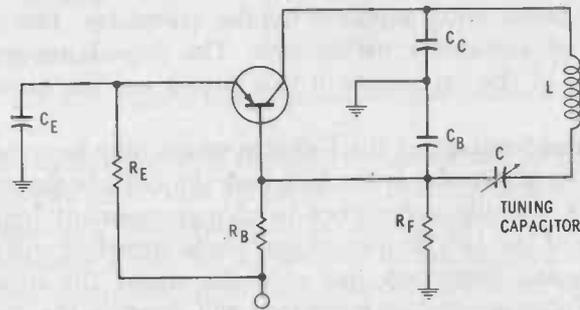
Fig. 2-14. Clapp oscillator configuration.
