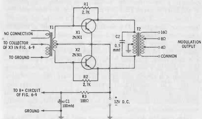
Fig. 6-15. Schematic diagram of the five-watt transmitter modulator.
