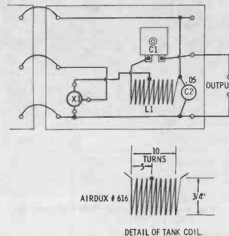
Fig. 4-12. Layout for the "CB Cyclone II."
