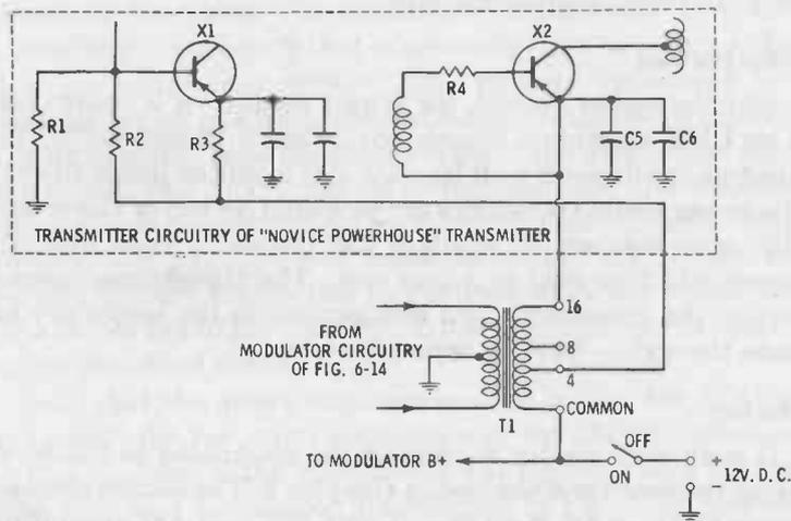
Fig. 6-18. Circuitry showing the method of connecting the modulator to the 80/40-meter transmitter project of Chapter 5.
