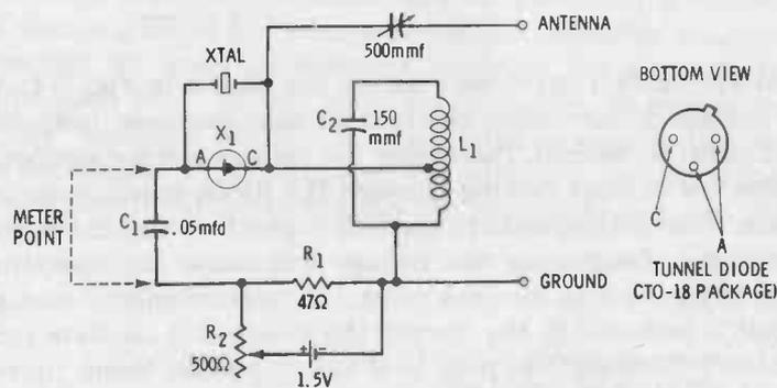
Fig. 7-5. The tunnel-diode oscillator.
