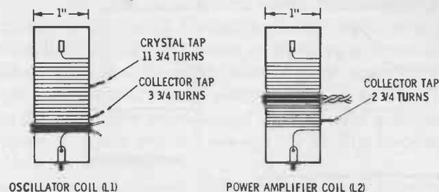
Fig. 5-5. Coil-winding detail.
