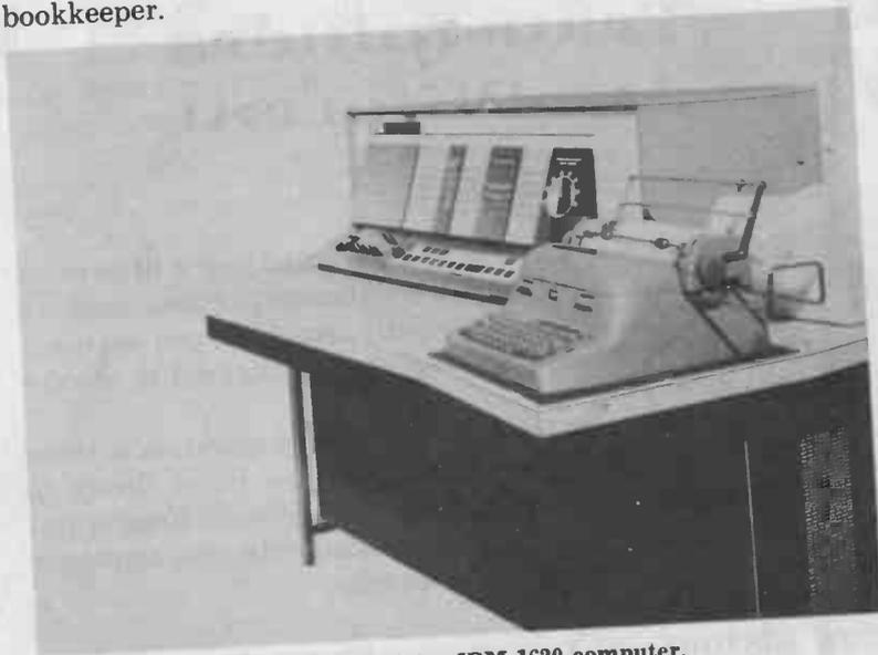
Fig. 1-1. Transistor IBM 1620 computer.
