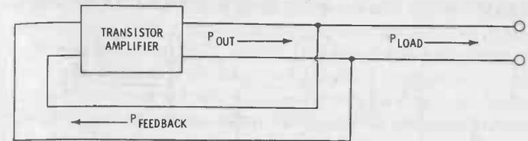
Fig. 2-3. Black box equivalent of an oscillator.
