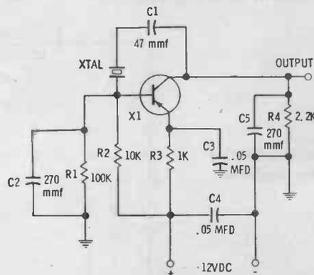
Fig. 3-2. Schematic of the crystal checker.
