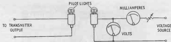
Fig. 1-17. System for estimating power output.
