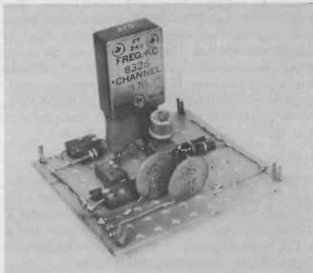
Fig. 3-4. Photo showing crystal socket.
