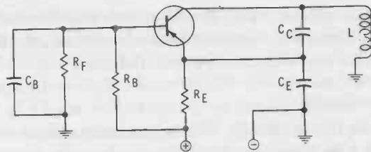
Fig. 2-11. Colpitts with capacitive-divider feedback.
