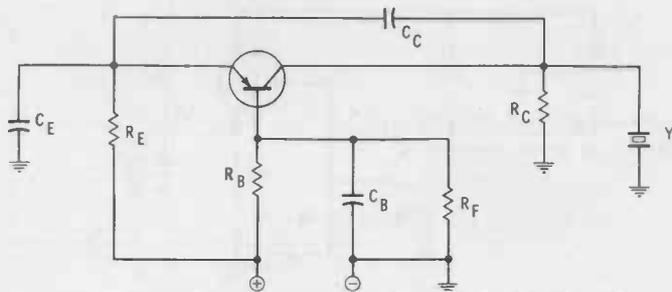
Fig. 2-22. Circuit of a Pierce oscillator.
