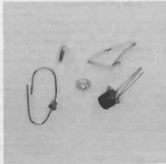
Fig. 7-1. Examples of tunnel diodes.
