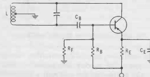
Fig. 2-8. Hartley-type oscillator.
