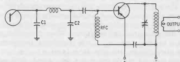
Fig. 4-5. Low-pass filter coupling system.
