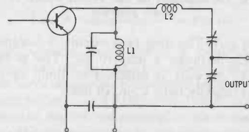
Fig. 4-7. "Sloppy-tuned circuit" for output impedance matching.
