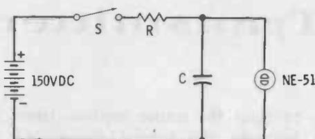
Fig. 7-2. A relaxation-type oscillator using a neon bulb as the negative-resistance device.
