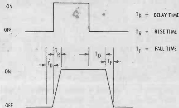
Fig. 1-2. Rise, fall, and delay time characteristics.
