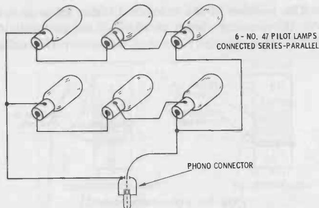
Fig. 5-6. Dummy-load bank for transmitter testing.
