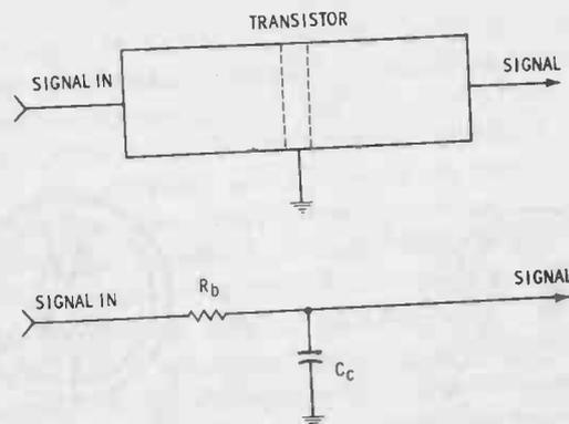
Fig. 1-6.  $R_b$  and  $C_c$  form low-pass filter.
