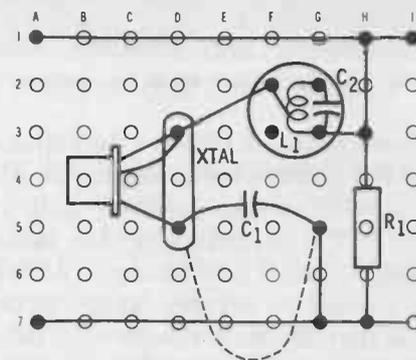
Fig. 7-6. Layout of the tunnel-diode oscillator.
