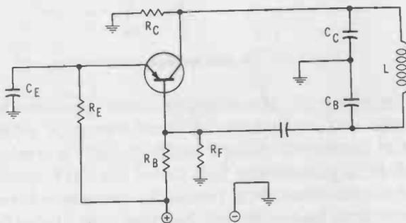
Fig. 2-12. Alternate Colpitts circuit.
