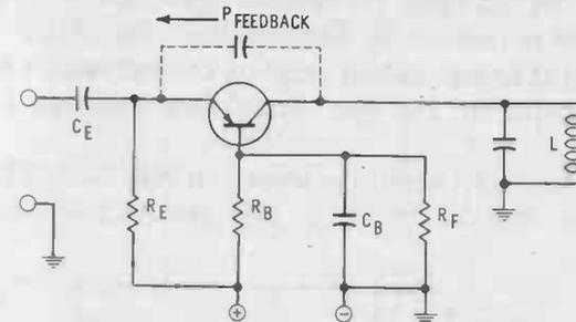
Fig. 2-10. Colpitts oscillator circuit.
