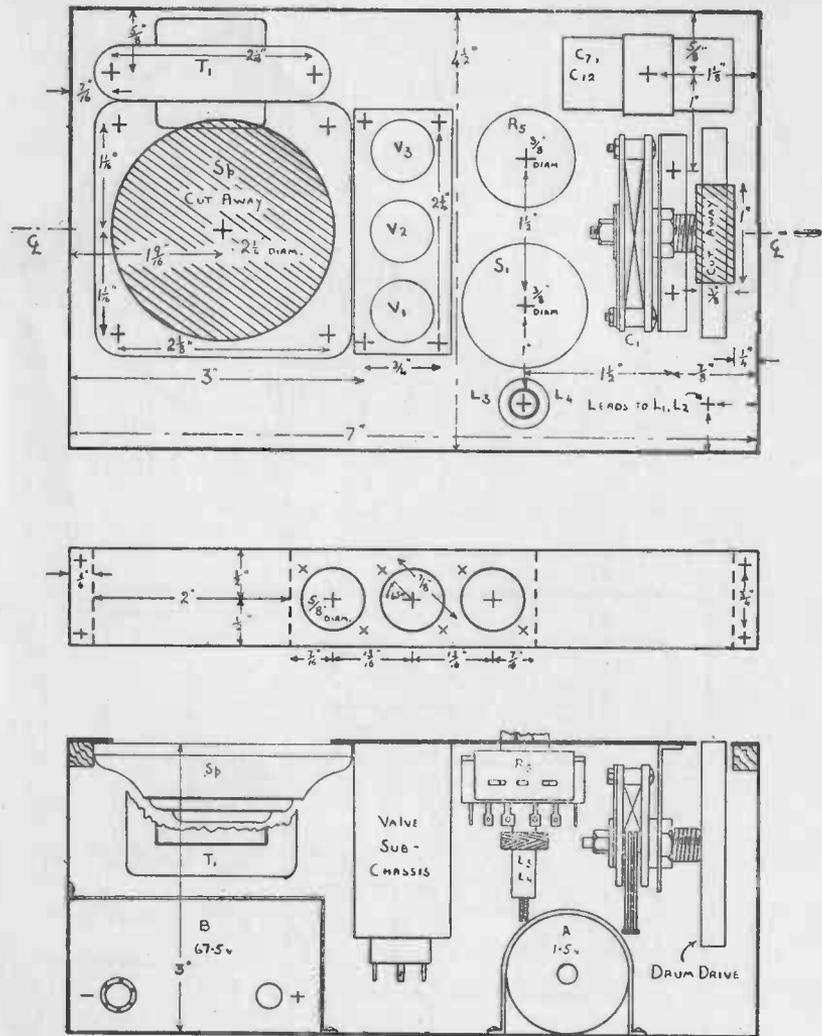
Fig. 2. Panel Dimensions, Sub-chassis and Side Constructional View of the "Minor"
