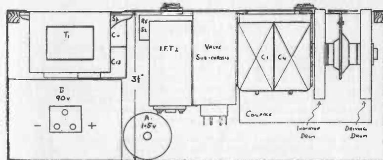
Fig. 15. Panel Dimensions, Brackets and Side Constructional View of the "Carri-Major"
