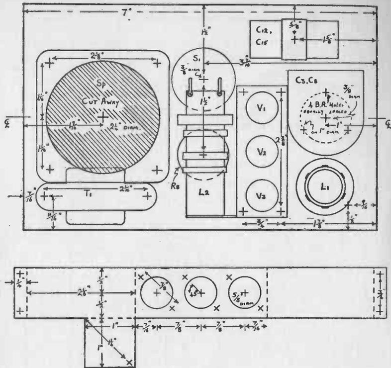
Fig. 6. Panel Dimensions, Sub-chassis and Side Constructional View of the "Carri-Minor"
