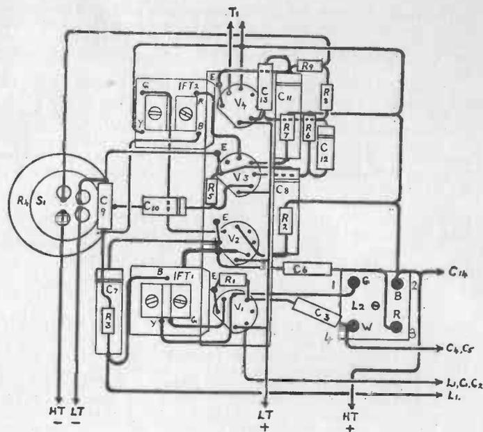
Fig. 10. Point-to-Point Wiring Plan of the "Simplest Super"
