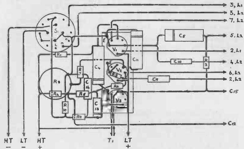
Fig. 7. Point-to-Point Wiring Plan of the "Carri-Minor"
