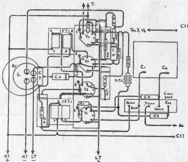
Fig. 16. Point-to-Point Wiring Plan of the "Carri-Major"
