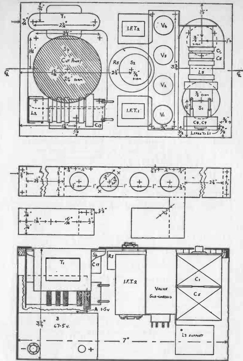
Fig. 12. Panel Dimensions, Bracket, Sub-Chassis and Side Constructional View of the "Two-Band Super"
