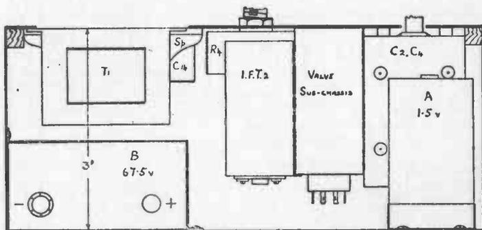
Fig. 9. Panel Dimensions, Sub-chassis and side Constructional View of the "Simplest Super"
