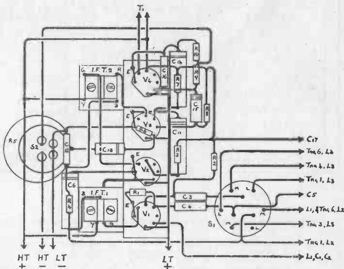
Fig. 13. Point-to-Point Wiring Plan of the "Two-Band Super"
