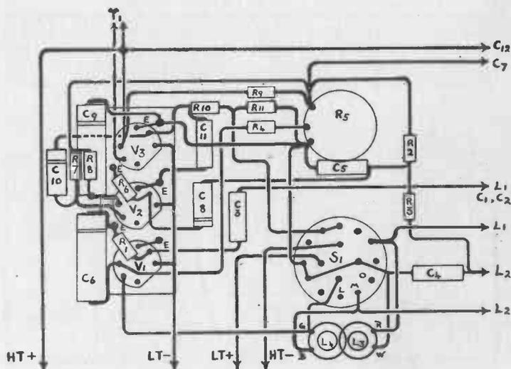
Fig. 4. Point-to-point Wiring Plan of the "Minor"
