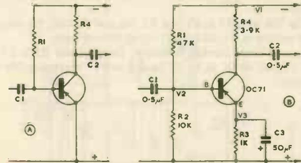
FIG. 93. Audio amplifier for low signal levels
