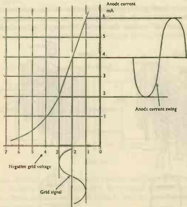
FIG. 18. Operation of class A amplifier
