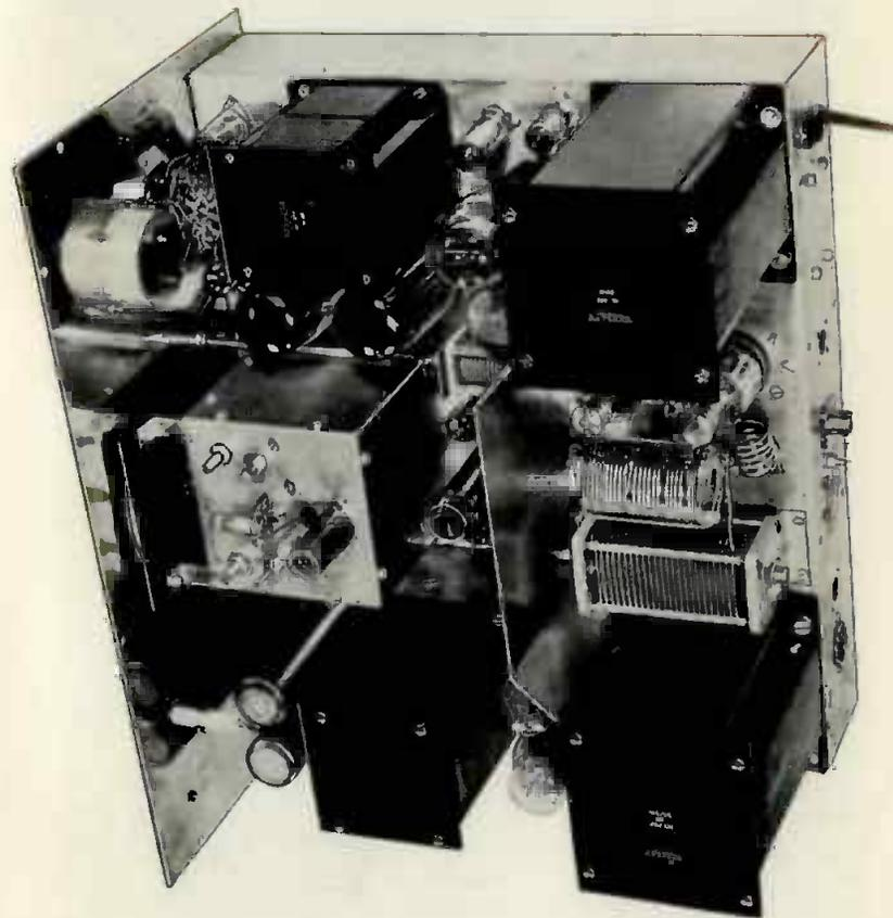
1. DX-100U 150 watt transmitter covering 160 to 10 metres. Left, power transformers, centre, screened VFO, right, push-pull modulator, PA two 6146's. (Heathkit, Daystrom Ltd., Gloucester.)
