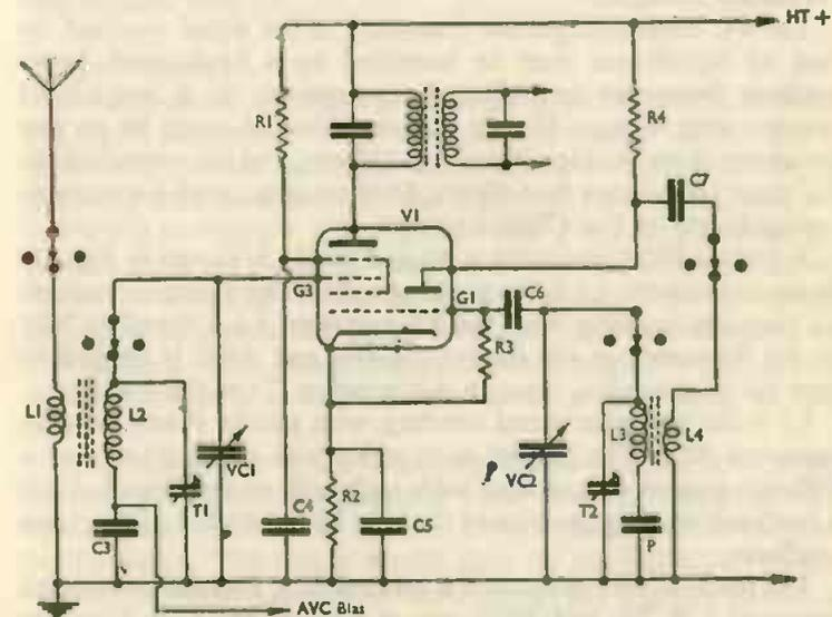
FIG. 28. Triode-hexode frequency changer
