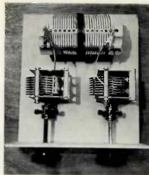
12. 10-80m. aerial tuner for Zepp, tuned doublet, or end-fed Hertz (see aerials chapter). Clips permit series or parallel tuning on any band.
