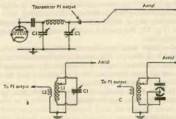
FIG. 74. Ways of connecting an end-fed aerial
