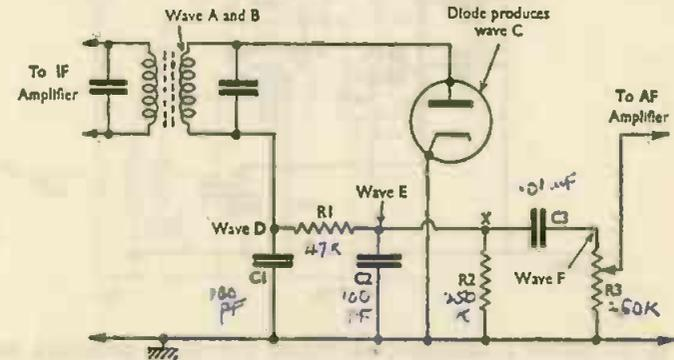
FIG. 25 Detector or Demodulator circuit
