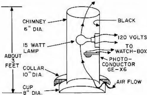
Figure H3.6 Cross-section view of smoke detector
