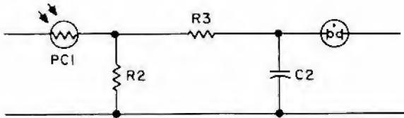
Figure E6.2 Inverted operation of 1000-watt flasher
