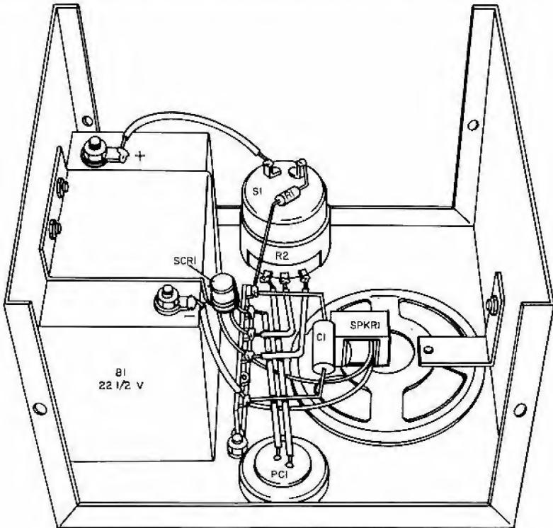
Figure H3.3 Watch box pictorial diagram
