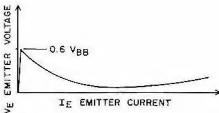
Figure 27. Unijunction transistor characteristic
