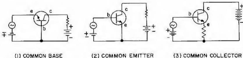
Figure 24. Transistor hook-ups
