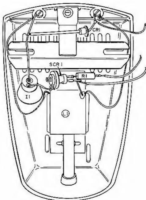
Figure A1.2 Battery-saver pictorial diagram (negative ground)
