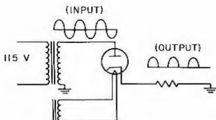
Figure 3. Diode connected for half-wave rectification
