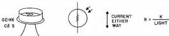
Figure 42. Typical photoconductor
