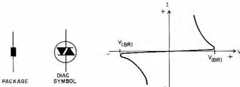
Figure 40. Symbol and characteristic of the Diac (GE-X13)
