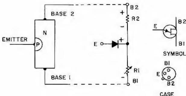
Figure 26. Unijunction transistor
