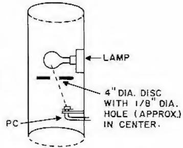
Figure H3.7 Alternate arrangement for smoke detector
