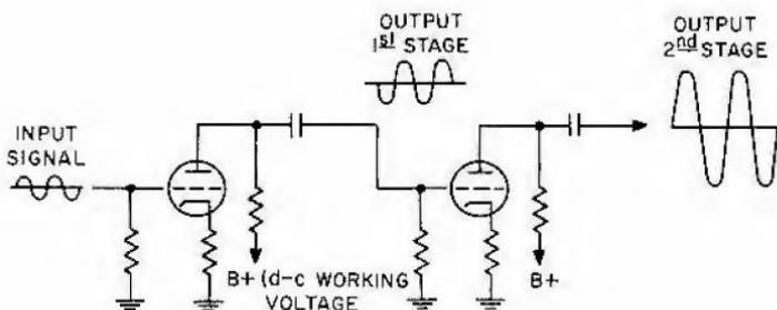
Figure 6. Two-stage triode amplifier
