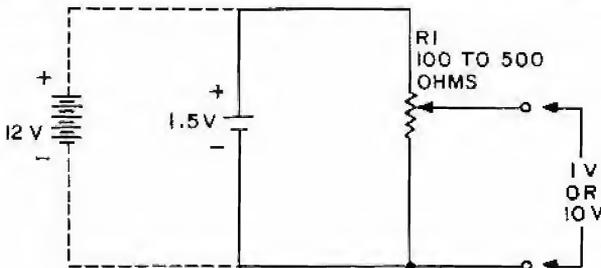
Figure W6.3 Voltage calibration source for adapter
