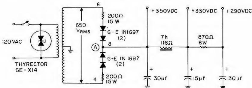
Figure W11.3 Alternate silicon rectifier replacement circuit—
