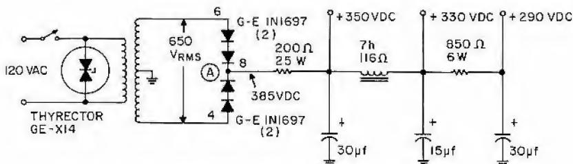
Figure W11.2 Alternate silicon rectifier replacement circuit—
