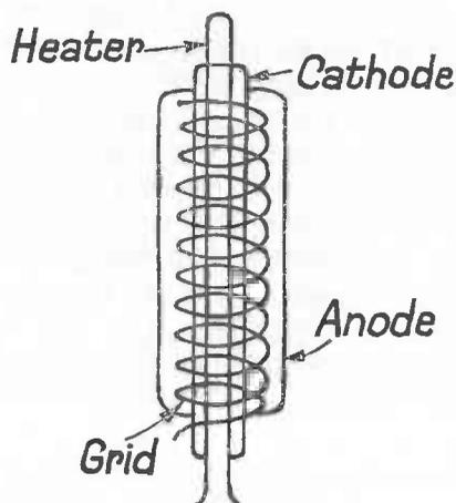
Fig. 14 An Indirectly Heated Triode
