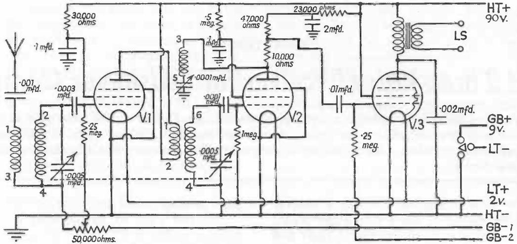
Fig. 11 Three-Valve Battery Receiver. Theoretical Diagram
