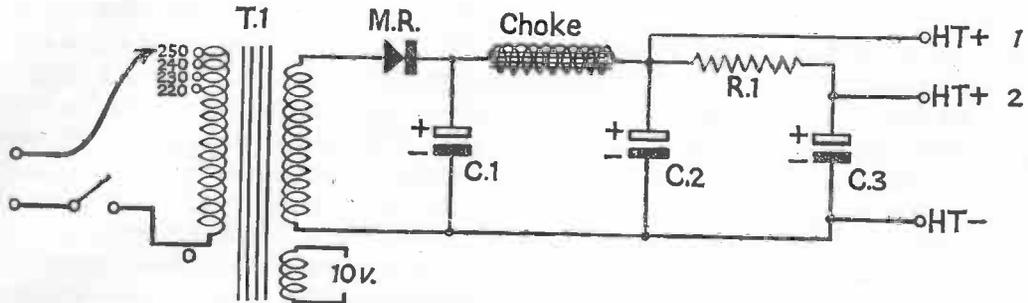
Fig. 16 Mains HT Unit. Theoretical Circuit
