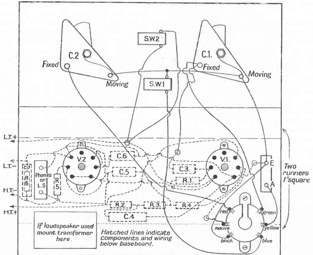
Fig. 10 Battery Two-valve Receiver
