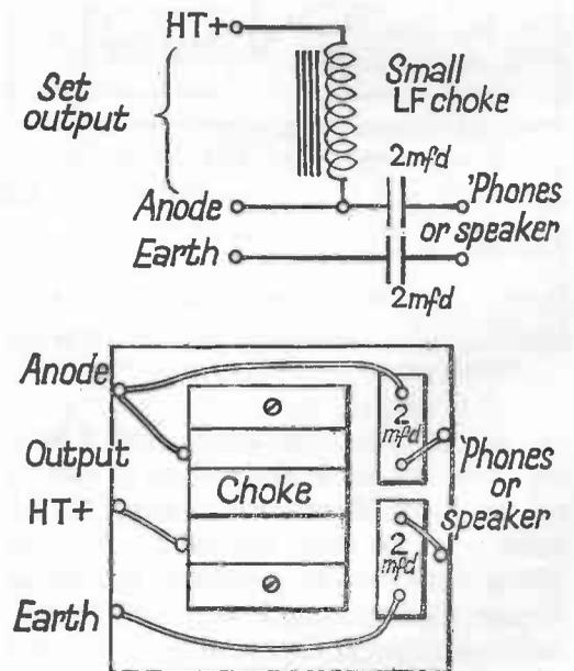
Fig. 18 Output Filter Circuit
