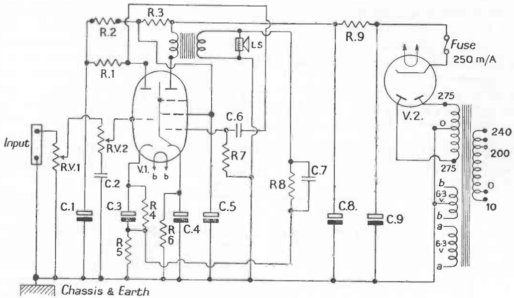
Fig. 23 Basic Diagram for 2-valve amplifier
