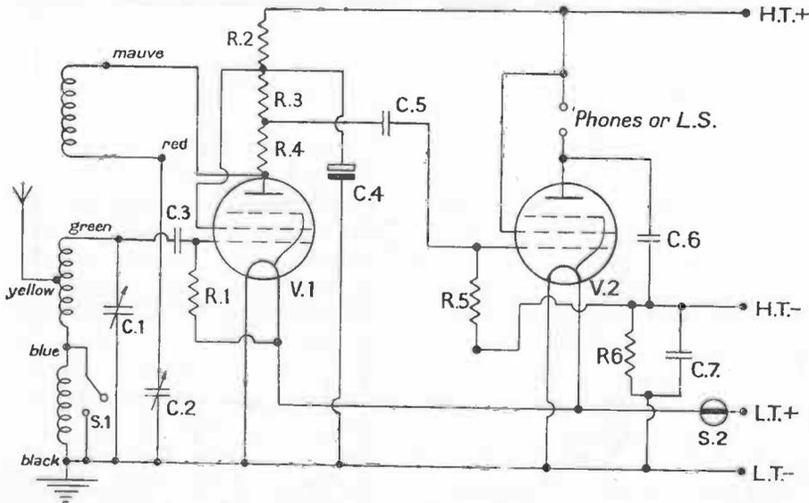
Fig. 9 Battery Two-valve Receiver
