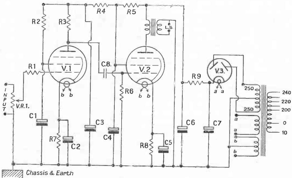
Fig. 24 Basic Diagram for 3-valve amplifier
