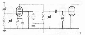
Fig. 17. The pentode as r.f. valve. The tuning capacitor of the detector circuit is connected direct to earth and the lower end of the tuning coil is connected to earth via a by-pass capacitor.
