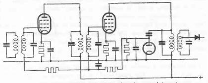
Fig. 29. I.F. amplifier with automatic gain control (a.g.c.).
