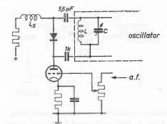
Fig. 86. Narrow band frequency modulation by means of a diode parallel to tuning circuit of the oscillator stage.
