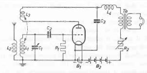
Fig. 12. Variable feedback by means of a variable series resistor. Headphones matched by means of a transformer.
