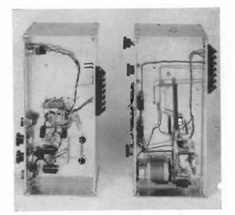
Photo 12. Underneath view of the transmitter and modulator. On the right the transmitter with the very robust oscillator coil visible at the bottom. To the right of this the trimmer of the permanently tuned 80-metre circuit. The wiring of the modulator (left) needs no further explanation.
