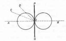
Fig. 101. Radiation pattern of halve-wave aerial  $(1 = \lambda/2)$ .
