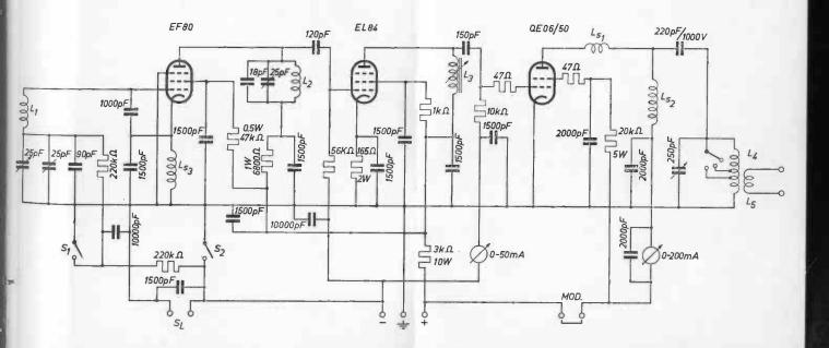
Modulation transformer :core diameter2.8 × 5 cmthickness of lamination0.5 mmair gap0.07 mmprimary2 × 1300 turns0.2 mm enamel wiresecondary1800 turns0.16 mm
