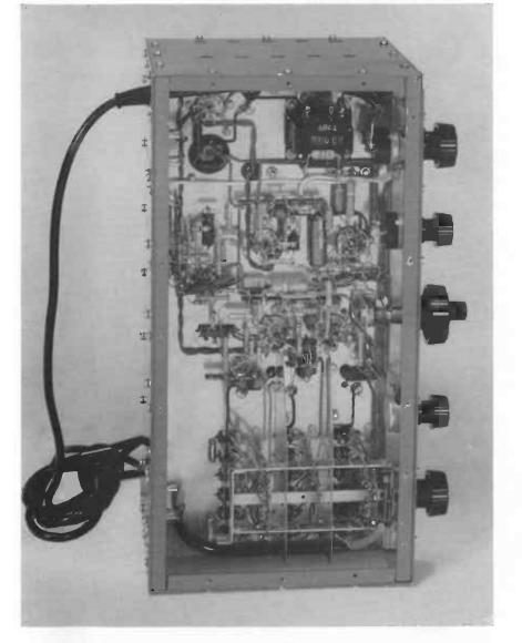
Photo 7. Underneath view of short-wave superheterodyne receiver. At the bottom the wave range switch with the two screens to separate the aerial circuit, the second tuned circuit and the oscillator circuit from each other. In the centre slightly to the left the screening over the valve holder of the i.f. valve. The loudspeaker transformer is at the top.
