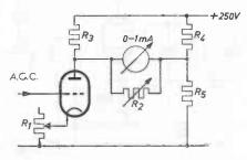
Fig. 31. Simple signal-strength meter.
