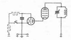
Fig. 67. Keying the screen-grid circuit with negative bias.
