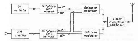
Fig. 88. Single-sideband modulation according to the phase-displacement system. By means of 90° phase-shift networks, the phases of both the carrier wave and the modulation are changed 90°. In the balanced modulators in which the carrier is suppressed again, the signals are combined in such a way that one sideband is suppressed.
