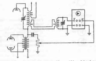
Fig. 123. Modulation depth measurement with an AM-modulated transmitter by means of an oscilloscope.
