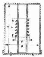
Fig. 129. Position of coil in screening can. The letters correspond to those in formula 5.
