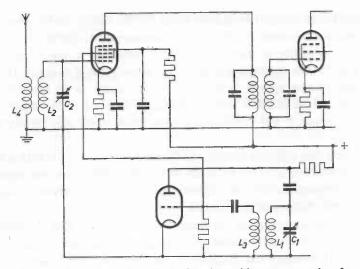
Fig. 20. Circuit diagram of frequency changing with separate valve for mixing and oscillating.
