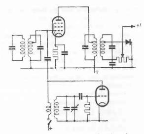
Fig. 28. I.F. amplifier with "beat-oscillator" for telegraphy reception.
