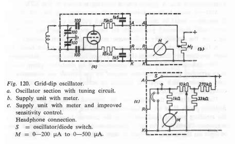
It is recommended that the grid-dip meter is provided with a connection for headphones as shown in the circuit diagram in Fig. 120c. Headphones also constitute a sensitive indicating medium and enable the correct signal to be selected in cases of doubt.
