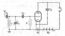
method of detection is similar to that shown in Fig. 8 and is therefore again accompanied by some damping in the tuning circuit. Compared to the amplification which is obtained this effect is negligible, however, provided that the values of the components have been chosen correctly.
