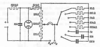
Fig. 117. Wheatstone bridge with a.c. voltage source, suitable for resistance and capacitance measurement. Headphones as indicator.
