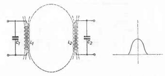
Fig. 24. Two circuits tuned to the same frequency. Coupling less than "critical".
