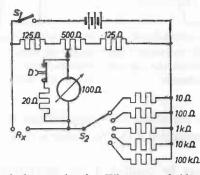
Fig. 116. Practical example of a Wheatstone bridge for resistance measurement. Switch  $S_2$  selects the measuring range. The sensitive meter position is obtained by means of push button D.
