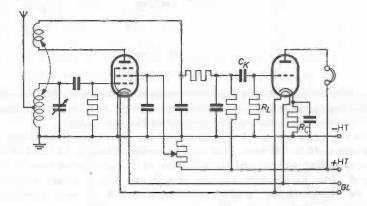
Fig. 14. Resistance-coupled detector and a.f. amplifier. An indirectly heated pentode is used as detector and an indirectly heated triode as a.f. amplifier.
