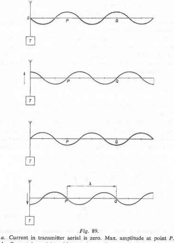
b. Current in aerial positive maximum. Zero-amplitude at point P.
