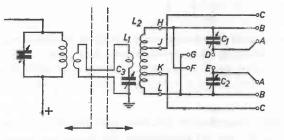
Fig. 100. Aerial coupling unit for matching to high and low-impedance.  $C_1 = C_2 = 200 \text{ pF.}$  $C_3 = 350 \text{ to } 500 \text{ pF.}$
