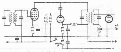
Fig. 30. Combined a.g.c. and manual control.
