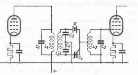
Fig. 27. I.F. band-pass filter with crystal filter for improved selectivity.
