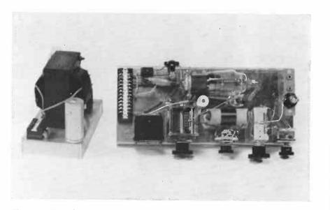
Photo 9. Top view of the telegraphy transmitter. The method of mounting the transmitter valve and associated chokes is clearly visible. The aerial connections are on the right.
