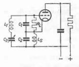
Fig. 42. Electron-coupled oscillator (ECO) with Hartley oscillator circuit.
