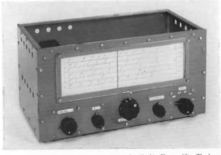
Photo 5. Short-wave superheterodyne receiver (described in Chapter 10). The large linear dial clearly shows the six bands. The knobs are (from left to right): a.f. gain control, b.f.o. switch, tuning knob, r.f. gain control, range switch.
