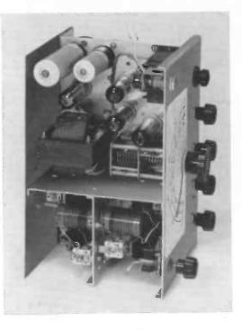
Photo 3. Top view of straight receiver. The two coil compartments are seen at the bottom of the photograph (detector on the left, aerial on the right). Each compartment contains three coils, one for each band, which are mounted perpendicularly to each other. Behind the twin capacitor is the mains transformer; the loudspeaker transformer is seen on the top r.h. side.
