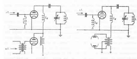
Fig. 72. Principle of Heising modulation, i.e. a form of anode modulation employing a choke. Fig. 73. Anode modulation with transformer coupling between transmitter and modulator.
