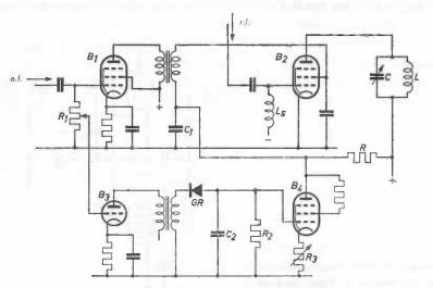
*Fig.* 79. Controlled carrier modulation. The clamp tube  $B_4$  is controlled according to the a.f. level.
