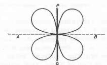
Fig. 102. Radiation pattern of full-wave aerial  $(1 = \lambda)$ .
