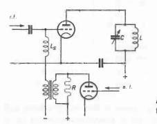
Fig. 74. Control-grid modulation. Transformer coupling.
