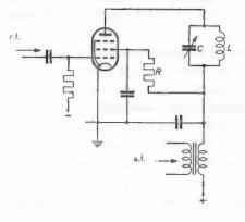
Fig. 76. Combined anode and screengrid modulation. The correct screen-grid voltage is obtained by means of resistor R. high enough to ensure that the screen-grid dissipation remains within certain limits. The transformer should match the value  $\frac{V_a}{I_a + I_{g_2}}$ .
