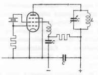
Fig. 50. Pierce oscillator with tuning circuit to increase the delivered r.f. voltage.
