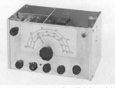
Photo 2. The straight receiver (described in Chapter 10). In the centre the large dial with the three ranges. The 5 knobs at the bottom are (from left to right): r.f. gain control, wave switch, feedback control, a.f. gain control + mains switch, fuse holder. The aerial capacitor is on the top l.h. side and the signal lamp on the top r.h. side.
