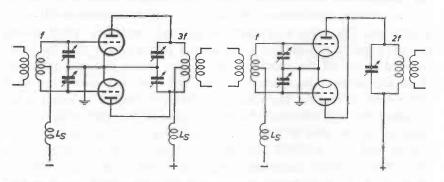
Fig. 53. "Push-pull" amplifier suitable as Fig. 54. "Push-push" amplifier specially "trebler". suitable as "doubler".
