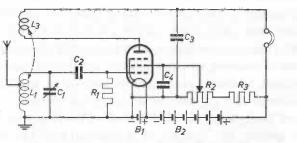
Fig. 13. The pentode as detector. Feedback from the anode, controlled by the screen grid voltage.
