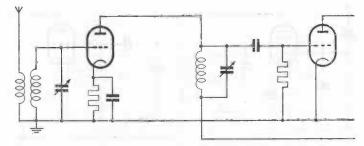
Fig. 16. Triode as r.f. amplifier with by-passed cathode resistor for correct adjustment of the negative bias. The heaters of the indirectly heated valves have been omitted in this and the next figures for the sake of simplicity.
