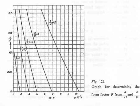
Assume that we use a former with a diameter of 3 cm and that the diameter of the copper wire is 1 mm, then:
