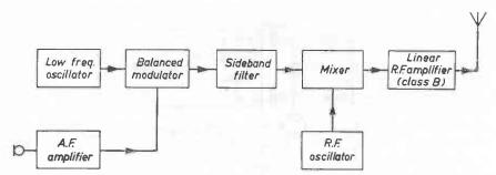
Fig. 87. Single-sideband modulation according to the "filter" system. The audio signal, together with an a.f. oscillator signal is fed into a balanced modulator, the carrier wave being suppressed. The sideband filter filters out one sideband. This is then transformed to the correct frequency.
