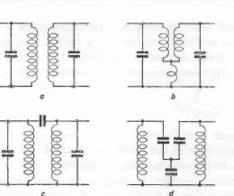
Fig. 4. Coupling methods with band-pass filters
