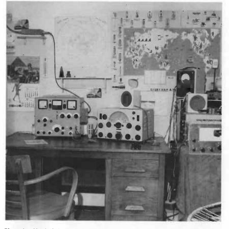
Photo 1. Shack belonging to PAOIB. The transmitter (left) and the receiver (right) are placed in convenient positions, plenty of space having been left for the morse key, microphone, log and other necessary attributes. On the right-hand side there is room for measuring instruments and for equipment which is being built. The aerial filter is seen in the left-hand top corner.
