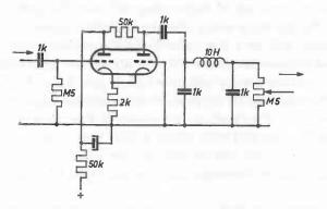
Fig. 85. Improvement of modulation by clipping the modulation peaks (speech clipping) and harmonic filter.
