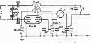
Fig. 121. Grid-dip oscillator with amplifier. Meter M = 0-2 mA to 0-6 mA.
