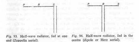
If the radiator is fed at point R, however, the impedance at that point will be low (low voltage, high current) and the feeders should be matched accordingly. This type of aerial is known as the "dipole" or "Herz" aerial.
