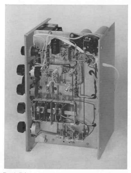
Photo 4. Underneath view of straight receiver. The wave-switch has four sections with a screen in the centre. This is in line with the screening on the top of the chassis between the aerial and detector circuits. The three trimmers for adjusting the feedback are seen at the bottom.
