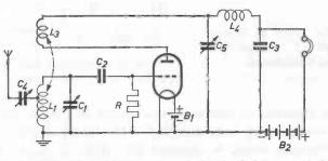
Fig. 11. The triode as detector with feedback by means of an extra coil. Adjustable with variable capacitor.  $L_4$  and  $C_3$ prevent r.f. voltages from reaching the headphones.
