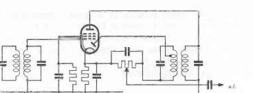
Fig. 22. Circuit arrangement where the germanium diode in Fig. 21 is omitted by using a diode-pentode.
