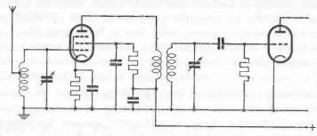
Fig. 18. The detector tuning circuit is earthed. The signal is received from the r.f. stage via a coupling coil.
