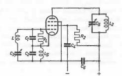
Fig. 44. Electron-coupled oscillator with Clapp oscillator circuit.
