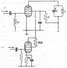
Fig. 78. Screen-grid modulation with the aid of a clamp tube.
