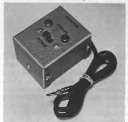
Fig. 212. Exterior view of the headphone amplifier.
