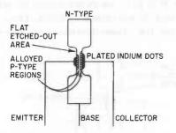
Fig. 608. This method can be considered as a combination of the surface-barrier and alloy-junction processes.
