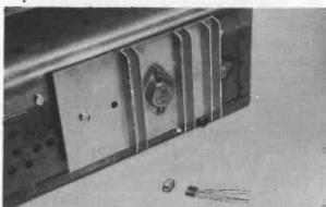
Fig. 704. Large cast or extruded aluminum heat sinks are used to help dissipate the heat by convection. If the heat sink is insulated from the chassis it is not necessary to use other insulators (Fig. 702). The aluminum can be anodized to form a very thin insulating coating.
