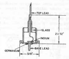
may be made of germanium, silicon, or various semiconductor compounds. If we ignore external appearances, variations in manufacturing technique, and differences in exact electrical specifications, there are basically two classes of diodes in current use: (a) signal handling types and (b) power rectifiers. Both operate in essentially the same fashion, except for the magnitude of currents handled, and both are identified with the same schematic symbol, as shown in Fig. 609.
