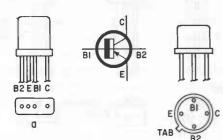
Fig. 210. Side views and basing diagrams for tetrode transistors (a, b), triode transistors with internal shield (c), and the Unifunction transistor (d). Like Figs. 208 and 209 this sketch is not to scale.
