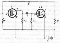
Fig. 412. Circuit of a transistor multivibrator. The schematic is essentially that of a two-stage amplifier with capacitive feedback between its input and output circuits.
