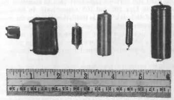
Fig. 202. Subminiature capacitors shown with "standard" sized units. From left to right . . . a pair of 0.1 µf ceramic capacitors, a pair 0.05 uf paper tubulars, and a pair of 50 uf electrolytics. Rule scale indicates sizes.
