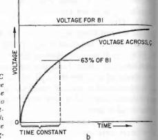
Fig. 413. Measuring the simple R-C circuit (a) to get the charging curve (b) is not usually practical. An infinite impedance voltmeter is required to prevent its current drain from affecting the charging curve. A very high value of resistance and capacitance would be needed to "time" the charging rate.
