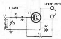
Fig. 611. Simple crystal detector and single transistor amplifier is a typical circuit for the beginning experimenter.
