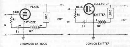
Fig. 307. The basic common-emitter transistor circuit configuration together with the analogous vacuum tube circuit arrangement. Often, the words "common" and "grounded" are used interchangeably . . . thus, a common-emitter stage might be specified also as grounded-emitter.
