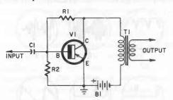
Fig. 402. The single-ended amplifier used for audio amplification is always operated "Class A". Distortion occurs when the bias is of a value that permits any portion of the signal to move the instantaneous bias point to a nonlinear portion of the operating curve. This distortion can be put to a practical use in special circuits not intended for the reproduction of sound.
