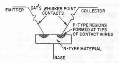
Fig. 602. This pictorial representation of the point-contact transistor shows the formation of p-type regions on the n-type base material.
