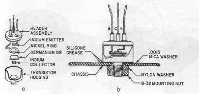
Fig. 508. An "exploded" view of a p-n-p alloy-junction power (multiwatt) transistor is shown at (a) . . . mounting details for this unit are given at (b). For maximum heat dissipation, most power transistors are mounted on a metal chassis or "heat sink."
