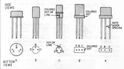
Fig. 208. Side view outlines and basing diagrams for typical low power transistors. This sketch is not to scale.
