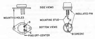
Fig. 209. Basing diagrams and outline sketches of power transistors.
