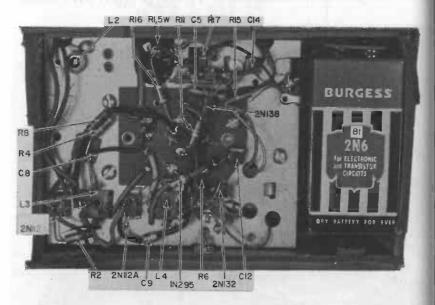
Fig. 217. "Below chassis" (back) view of the four-transistor receiver. Smaller electrical components are found here.
