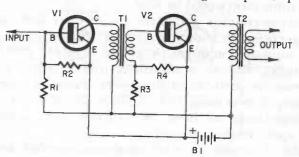
Fig. 407. Transformer-coupling gives greater gain. Higher cost of the transformer is offset by eliminating a transistor, coupling capacitor and bias resistors.
