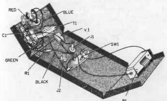
Fig. 214. Pictorial wiring diagram of the headphone amplifier. Compare this with the schematic given in Fig. 211 and the actual photograph of a wired model given in Fig. 213.
