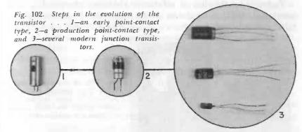
step in the transistor's evolution. Finally, with the invention of the junction transistor in 1951, a variety of new designs and types became possible, and manufacturers were able to introduce production techniques which eliminated most of the transistor's early faults. This last step is illustrated at 3, Fig. 102.
