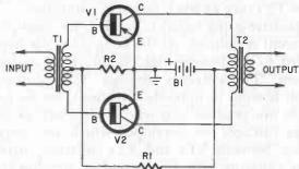
Fig. 403. The push-pull amplifier can be biased "Class A" for the least distortion or "Class B" for the greatest power output. Compromise amplifiers (like AB) are used for more power and have more distortion than those in Class-A operation. Class-C bias is used only with L-C tuned circuits.
