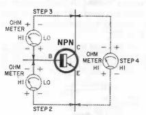
Fig. 707. Ohmmeter readings for n-p-n transistor tests.
