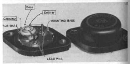
Fig. 509. Detail view of an uncapped (left) and capped multiwatt p-n-p transistor.
