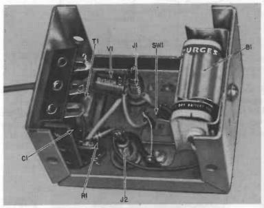
Fig. 213. Interior of the headphone amplifier, with major components identified.
