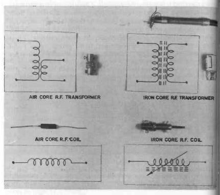
Fig. 204. Radio and intermediate frequency (rf and if) coils and transformers. Some of these use an air core, others employ a ferrite core to obtain greater inductance with fewer turns of wire. An adjustable core, indicated schematically by an arrow, permits the coil's inductance value to be changed.
