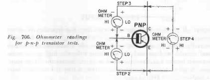
With a suspected transistor removed from its circuit, then, the test technique is a simple one.
