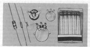
Fig. 201. Fixed and variable resistors. Three fixed resistors and two views of a small volume control are shown. The volume control is a subminiature type with built-in knob and switch. Compare this with the "standard" sized control. Bookmatches are included for size comparison.
