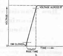
when dealing with circuits handling square-waves, pulses, and other step-like functions. This term can be explained quite easily if we refer to Fig. 414.
