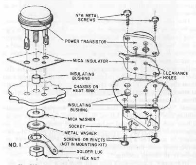
Fig. 702. Power transistor mounting must provide for heat dissipation. Mica insulators are coated with silicone grease for better conduction. (Motorola Semiconductor Prod. Inc.)
