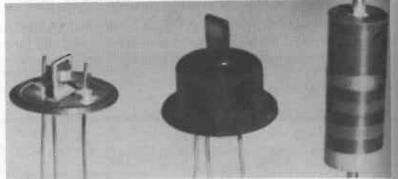
Fig. 506. Uncased (left) and cased views of an alloy-junction transistor . . . the small carbon resistor (right) is included to show relative sizes.
