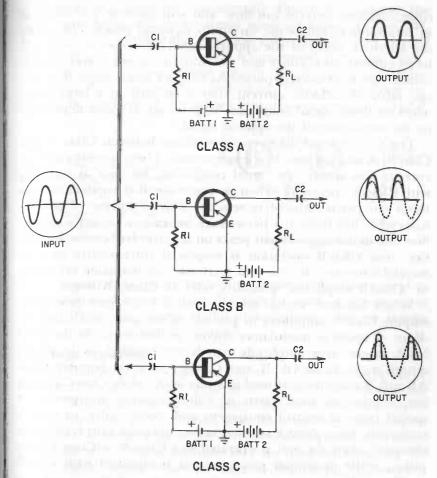
Fig. 404. The three basic arrangements of amplifier operation—Class A, Class B and Class C. In addition there is a fourth, intermediate between A and B—called, appropriately, Class AB.
