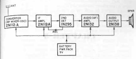
Fig. 218. Block diagram of the four-transistor receiver.
