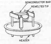
establishing a dominance of donor elements and forming a second n-type layer. Later, of course, the grown crystal is sliced into a three-layered "sandwich" of n, p and n semiconductors, then diced into n-p-n transistors.
