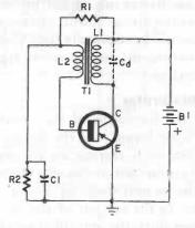
a piezo-electric quartz crystal may be incorporated into the feed-back circuit. Such a crystal is electrically equivalent to a high "Q"-tuned circuit (see discussion of coils in Chapter 2).
