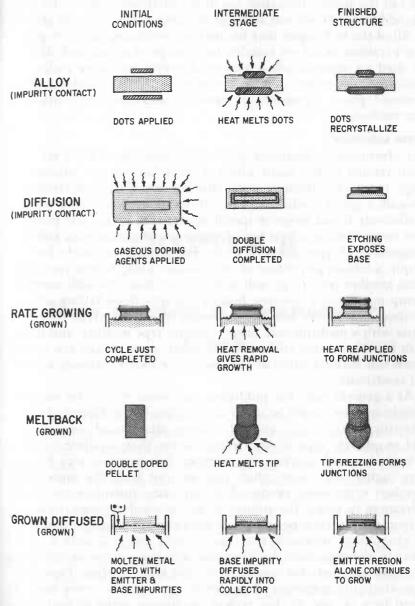
Fig. 510. Summary of important transistor production techniques. These methods, used to produce various types of junction transistors, represent the different techniques that may be employed. The important thing is that the production methods used permit the formation of two junctions having accurately controlled physical and electrical characteristics.
