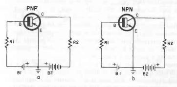
Fig. 306. Bias connections for p-n-p (a) and n-p-n (b) transistors. The dc polarities are generally referred to the electrode which is common to both the input and output connections . . . the emitter in this case.
