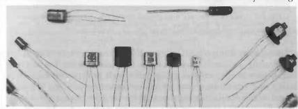
Fig. 104. Typical transistors. These are all low and medium power units, and demonstrate the variety of sizes and styles that are available. About 2,000 different types are being produced.
