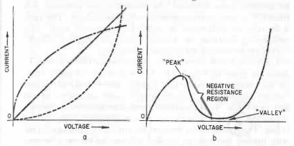
Fig. 616. The straight solid line in (a) is the linear characteristic of a resistor. Nonlinear devices may have curves like the broken and dashed lines. The Tunnel diode has a more complex curve (b) and the reverse slope (negative resistance region) allows the diode to oscillate.
