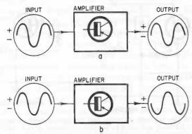
Fig. 310. What we mean by phase when speaking of an amplifier stage. At (a), the input and output signal waveforms are in phase. At (b), the two signals are out-of-phase. In the latter case, we say that phase reversal has taken place.
