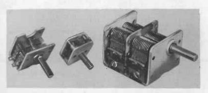
Fig. 203. Typical tuning capacitors. Miniature variable units used in transistor circuits are shown to the left, while the larger "standard" unit shows relative sizes. The very small capacitor uses a plastic film dielectric . . . the other two capacitors use air as a dielectric.
