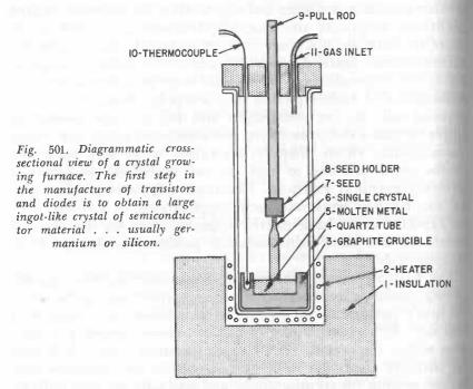
almost all rock and sand have silicon as one of their primary elements. Regardless of the original source of the raw material the semiconductor element is taken through a multistage refining and purification process which involves both chemical reactions and metallurgical techniques, resulting in ingots or bars of relatively "pure" metal.
