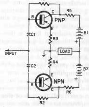
nected between the junction of the emitter resistors (R3 and R4) and the split-power supply, B1 and B2. The input signal is applied through dc-blocking capacitors C1 and C2 to both transistors simultaneously.
