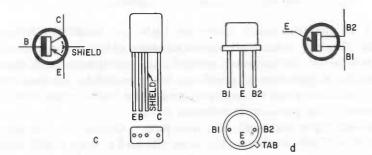
pattern or arrangement which serves to identify the leads, not actual dimensions, for these transistors are manufactured in a variety of physical sizes.
