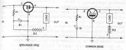
Fig. 308. The grounded-grid circuit is often used for circuit isolation. The common-emitter stage does not provide the isolation of its vacuum-tube counterpart.
