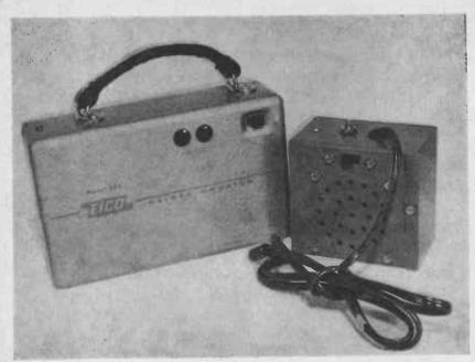
Fig. 7-11.—The Geigamp alongside a commercial Geiger Counter with which it can be used.
