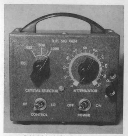
Fig. 9-5.—Author's model of the R.F. Alignment Generator.
