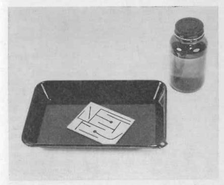
Fig. 13-4.—After the desired layout has been transferred to the copper-clad laminate as a pattern of resist, the board is etched in an enamel or plastic tray.
