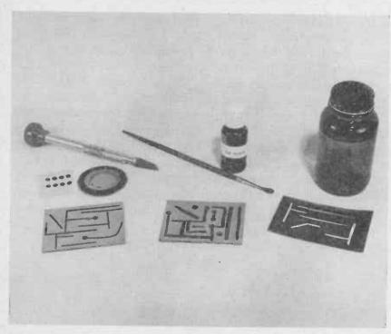
Fig. 13-3.—Three popular techniques used for making up "one-shot" etched circuits in the laboratory. Reading from left to right, the methods shown include tape resist, ink resist, and a photographic negative for a printed circuit layout.
