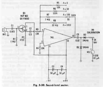
the high impedance of the microphone to the lower input impedance of the IC. The amplifier has four fixed levels of voltage gain ( $A_v = 1$ ,  $A_v = 10$ ,  $A_v = 100$ , and  $A_v = 1000$ ) set by switched-in feedback resistors R5, R6, R7, and R8. The output of the amplifier drives the rectifier-type meter circuit (C5, D1, D2, R9, M1).
