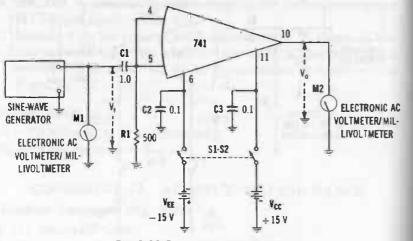
Fig: 2-22 Common-mode rejection.
