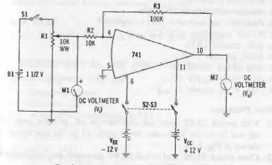
Fig. 2-18. Maximum dc output-voltage.swing.
