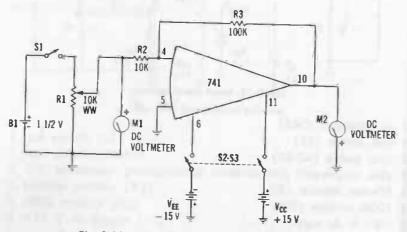
Fig. 2-11. Closed-loop dc voltage gain (inverting).
