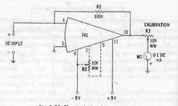
Fig. 3-23. Electronic dc microammeter.
