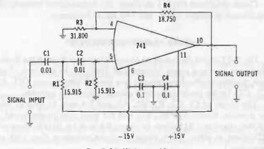
Fig. 3-14. High-pass filter.
