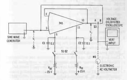
Fig. 2-24. Ac follower operation (noninverting).
