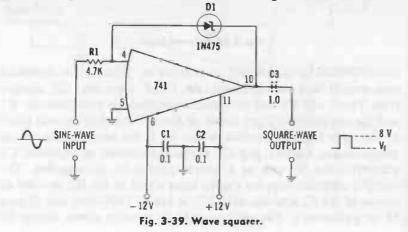
swings between that voltage and  $V_s$ , the forward voltage of the diode (this excursion is shown in the output-voltage waveform in Fig. 3-39). Output capacitor C3 is required only when strict ac coupling is desired.
