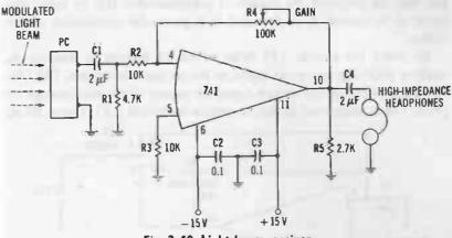
Fig. 3-40. Light-beam receiver.
