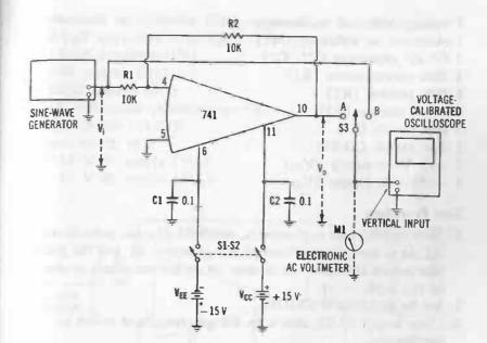
Fig. 2-25. Ac follower operation (inverting).
