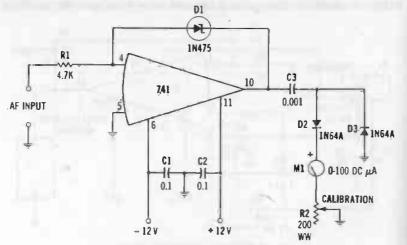
Fig. 3-29. Analog-type audio frequency meter:
