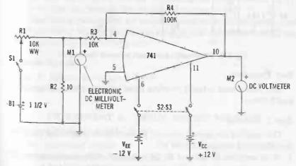
Fig. 2-7. Offset-null adjustment, external (method 1).
