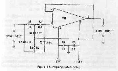
The values given in Fig. 3-17 actually result in a frequency of 994.7 Hz. For exactly 1000 Hz, trim resistors R1 and R2 to 15,915 ohms, and R3 to 7957 ohms. (It is easier to prune resistance than high capacitance.)
