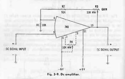
Check the circuit for (1) dc drain; and with gain potentiometer R3 at various selected settings, check (2) maximum input-signal voltage, (3) maximum output-voltage swing, (4) output/input linearity, (5) input resistance, and (6) output resistance.
