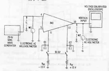
Fig. 2-13. Open-loop.ac voltage gain.
