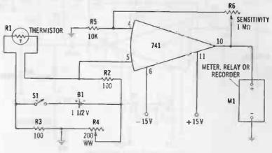
Fig. 3-28. Electronic thermometer.
