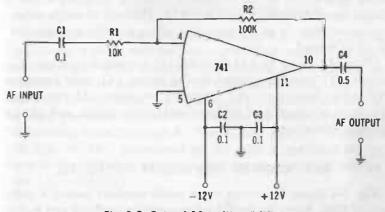
Fig. 3-2. Gain-of-10 audio amplifier.
