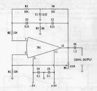
Fig. 3-10. Twin-T audio-oscillator.
