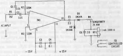
Fig. 3-34. Tuned ac relay-
