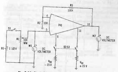
Fig. 2-12. Closed-loop dc voltage gain (noninverting).
