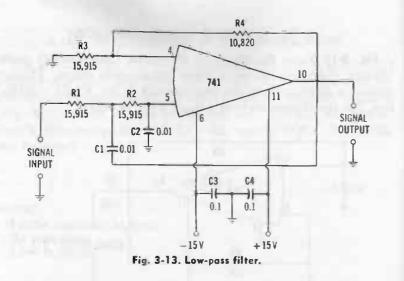
Check the circuit for (1) dc drain, (2) frequency response, (3) maximum input-signal amplitude, (4) maximum output-voltage swing, and (5) voltage gain in the passband.
