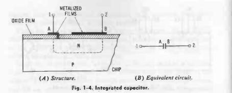
the film, which it penetrates through a hole to contact one end of the n region. Leads 1 and 2 are attached to these film-type contacts. The area of plate B is chosen for a desired capacitance (for a given oxide-film thickness, the greater the area the higher the capacitance).
