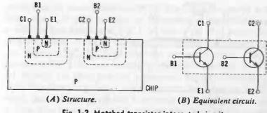
Fig. 1-2. Matched-transistor integrated circuit.
