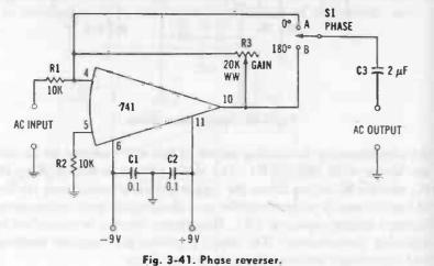
position B, and observe the phase of the output signal, which should appear rotated 180°. Adjust potentiometer R3 for an amplitude suitable for observation. (4) Repeat Steps 1 through 3 at various frequencies, noting the effect of frequency on phase reversal and on amplitude. (5) Check the dc drain at (a) zero-signal input and (b) maximum-signal input.
