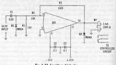
Fig: 3-33. Sensitive.af/rf relay.
