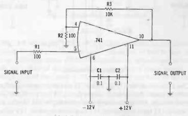
Fig. 3-5. Noninverting amplifier.
