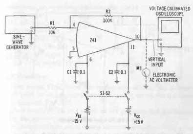
Fig. 2-19. Maximum ac output-voltage swing.
