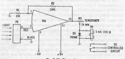
Fig. 3-35. Photorelay,
