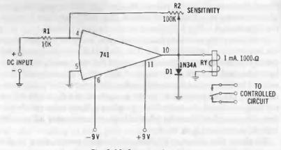
Fig. 3-32. Sensitive dc relay.
