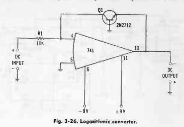
over a portion of its operating range is imparted to the IC. This type of converter finds application in instrumentation, control, analog calculating, and signal processing.
