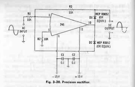
to operate at higher frequencies than it otherwise might reach. For efficient operation of the circuit, resistors R1 and R3 must be matched within 1 percent.
