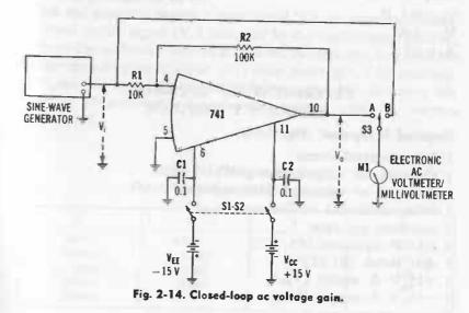
2 0.1- $\mu$ F capacitors (C1, C2) 1 dpst switch (S1-S2) 1 spdt switch (S3) 1 10K resistor (R1) 1 100K resistor (R2) 1 +15 V dc supply (V<sub>CC</sub>) 1 -15 V dc supply (V<sub>EE</sub>)
