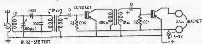
Fig. 818. Diode-type broadcast receiver with transistor a.f. amplifier.
