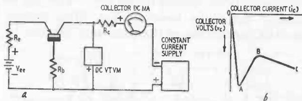
Fig. 914-a, -b. Circuit for testing collector negative-resistance characteristics.
