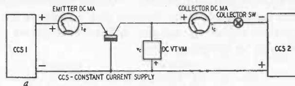
Fig. 905-a. Test circuit for measurement of forward characteristics.
