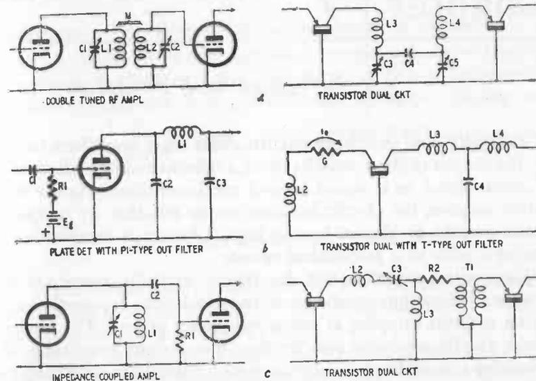
Fig. 602. Representative tube circuits with transistor duals.
