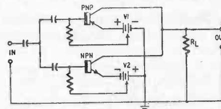
Fig. 408. Push-pull amplifier using complementary symmetry principle.
