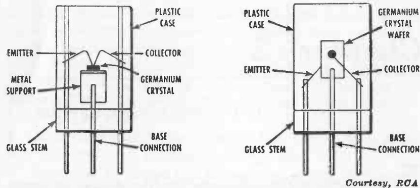
Fig. 201. Essential features of point-contact and junction transistors.
