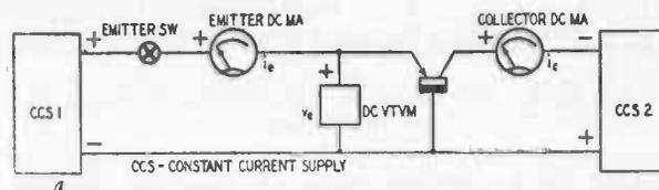
Fig. 904-a. Test circuit for measurement of feedback characteristics.
