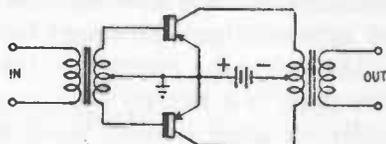
Fig. 407. Conventional push-pull amplifier.
