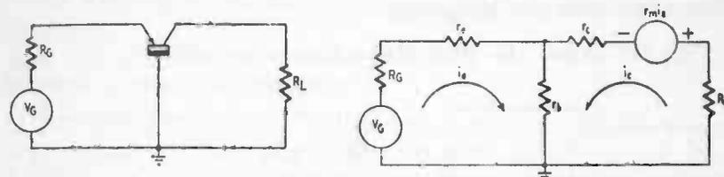
Fig. 302. Grounded-base amplifier and equivalent 3-terminal network.
