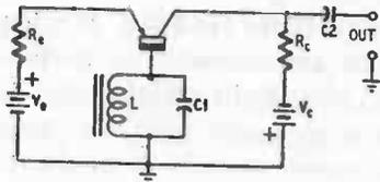
Fig. 501. Base-tuned oscillator.
