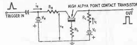
Fig. 701. Basic switching circuit using emitter negative resistance.
