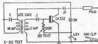
Fig. 812. Audio signal injector for amplifier servicing.
