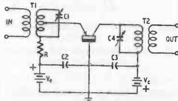
Fig. 413. Single-stage transformer-coupled r.f. amplifier.
