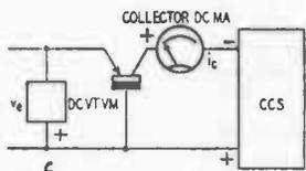
Fig. 907-c. Feedback resistance measurement.
