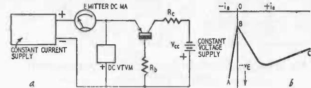
Fig. 913-a, -b. Circuit for testing emitter negative-resistance characteristics.
