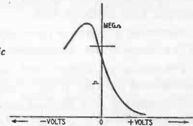
Fig. 107. Static resistance characteristic of a semiconductor diode.
