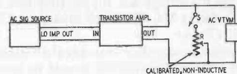
Fig. 911. Circuit for measurement of output impedance.
