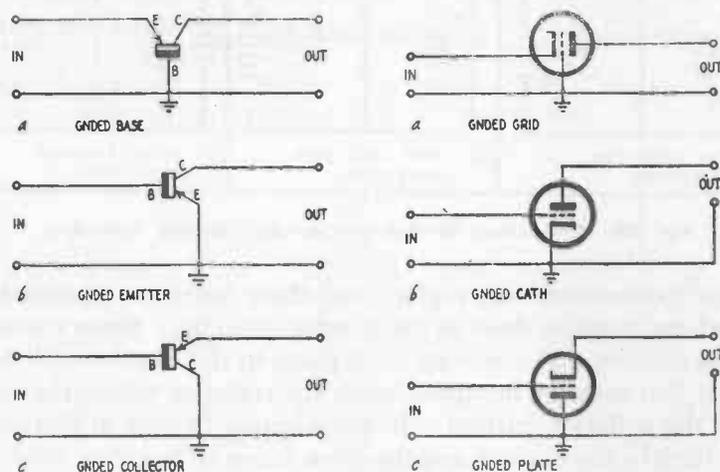
Fig. 210. Transistor amplifier configurations with equivalent tube circuits.
