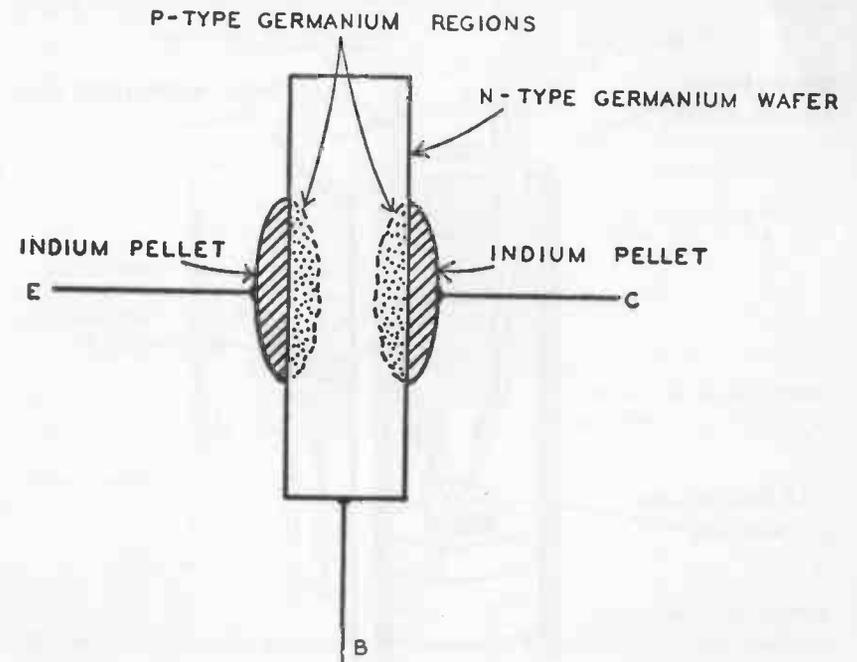
Fig. 203. Construction details of diffused P-N-P transistor junction.
