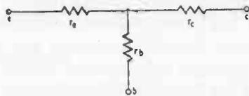
Fig. 212. Simplified equivalent 3-terminal resistance network of transistor.
