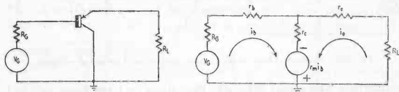
Fig. 304. Grounded-collector amplifier and its equivalent network.
