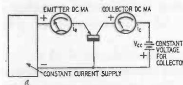
Fig. 908-a. Test circuit for current amplification, alpha.
