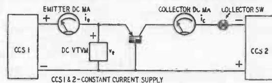
Fig. 902-a. Test circuit for measurement of input characteristics.
