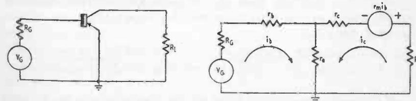
Fig. 303. Grounded-emitter amplifier and its equivalent network.
