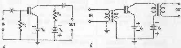
Figs. 402-a, -b. Grounded-emitter single-stage amplifiers.
