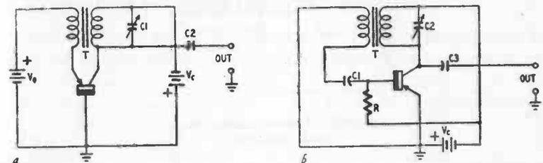
Figs. 502-a, -b. Grounded-base and grounded-emitter tickler-type oscillators.
