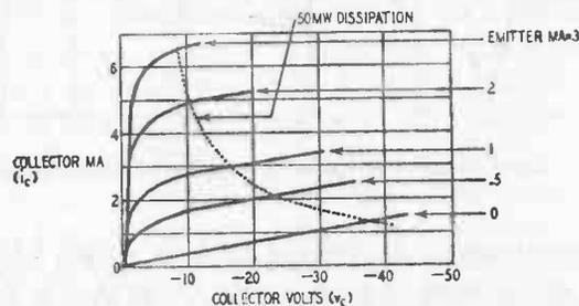
Fig. 216. Collector current vs. collector voltage curves.
