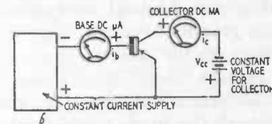
Fig. 908-b. Test circuit for current amplification, beta.
