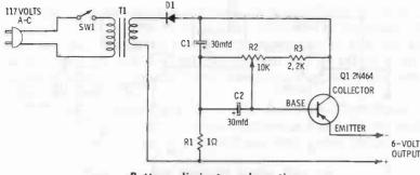
Battery eliminator schematic.
