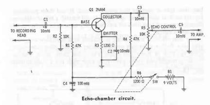
utilizes a negative-ground arrangement, do not hook this adapter in; it must be changed accordingly. To accomplish this, reverse the battery and capacitive polarities (so that the negative terminals go to ground), and change the transistor to an NPN 2N366.
