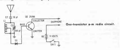
just drop in a tiny ceramic 60-pf capacitor and do all the tuning with L1. You can mount a small tuning knob on the screw-shaft of L1. The detector is a standard crystal diode, available for less than a dollar at most electronic parts stores.
