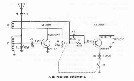
tuning slug of the loopstick antenna coil. In any case, adjust R1 for best regenerative kick-in (bringing with it the best of 2-transistor a-m reception), and leave it there. R1 is *not* a volume control.
