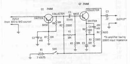
Transistor audio amplifier circuit.
