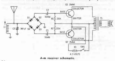
Note the bridge-like formation of four crystal diodes. This acts as the detector complex, leaving the transistors free to perform as fulltime push-pull amplifiers. Coil L1 is an ordinary vari-loopstick (untapped) antenna coil which is adjusted for calibration purposes only. When the plates of capacitor C3 are fully meshed, you adjust L1 so that the receiver is set at approximately 550 kHz on the broadcast band. After L1 is set, C3 is your tuning control.
