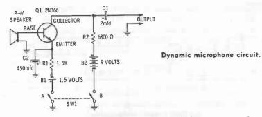
Actually, you can use any size speaker to build your own dynamic mike. Generally speaking, the larger the speaker, the greater the fidelity of the resultant output. Conversely, the smaller the speaker, the greater the loss in fidelity. In most applications, however, a small pm speaker from a discarded transistor radio makes a great microphone.
