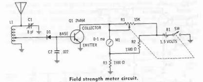
For greatest sensitivity for weak-signal sources such as low-power walkie-talkies, tune C1 to the exact operating frequency. This will be signaled by a definite and sudden rise on M1 when you hit this frequency. Once this has been preset, you can proceed with your tuneup as decribed previously. The coil is made from a prefabricated *Mini-ductor* form by cutting off a 12-turn section to use as L1.
