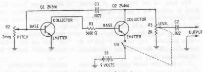
Signal generator schematic.
