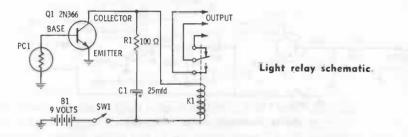
Construction is quite simple and straightforward. An aluminum housing makes a good enclosure, but this is not critical. A plastic parts box will do just as well. Watch battery and electrolytic capacitor polarities, and you should experience no trouble. The photocell can be mounted atop your light relay box, or wired remotely as far as 50 feet away without degrading performance. Just make certain you use good nonresistive copper interconnecting wires.
