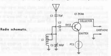
With the transistor antenna coil, tuning is accomplished by varying the capacity of C1, a 365-pf subminiature variable. The antenna itself can be any long wire, or just a piece of insulated hookup wire with an alligator clip in the end. The alligator clip can then be affixed to any large metallic object (window frame, bedspring, etc.) which can then serve as a large antenna.
