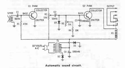
Here is how it works: Adjust potentiometer R2 to "hear" only the sound you want to trigger the circuit. Next, adjust R3 for the approximate "time-on" period, which can be anywhere from 1 to 20 seconds depending upon where you set the control. From here, everything is automatic. Nothing happens until the speaker hears the tone or voice signal it requires. Hookup can be in any fashion you want; just connect to the contacts you wish to use on K1.
