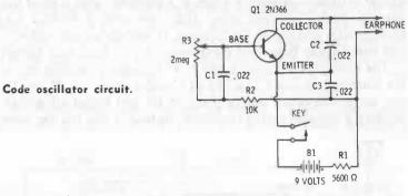
You can adjust the pitch of the C-W notes to any desired frequency by adjusting the setting of R3. No power switch is required, since, unless the key is momentarily depressed, the circuit is not functioning and consequently will not draw current from the battery. If you like, you can feed this oscillator into a headset-to-speaker-adapter circuit (such as is described in Project 8) and wind up with room-filling sound.
