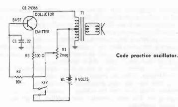
The entire affair can be built right into the speaker enclosure itself, although we obtained all the parts including the speaker, earphone jacks, and off-on-volume control from a discarded transistor radio. This left us with plenty of space for the battery and associated components. The "key" leads were fed to the earphone jack. When we want to practice CW, all we have to do is plug in the key. No off-on switch is required since the circuit draws no power until the key is depressed.
