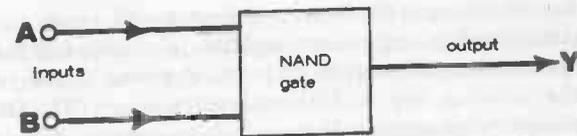
Fig. 13-3. The NAND gate shown in simple diagrammatic form.
