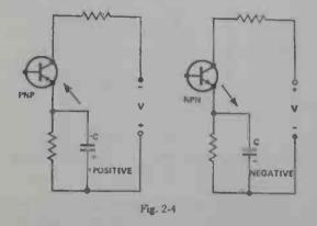
connect it the right way; that is, with correct polarity. Don't reverse the connections or you may damage the transistor permanently, possibly ruin it completely.
