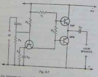
An important precaution with power transistors is the provision of heat-sinks where necessary. But you must be careful to bear in mind that the metal cases of transistors such as an AD140 are in contact with one active element of the tranastor-in this case, the collector-and it is imperative to insulate the case from the heat sink (in the electrical, not the thermal, sense), or else to have the heat sink in contact with the case (which gives better heat dissipation) and insulate 32
