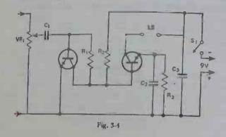
R1 can be about 6.8K, and R2 about 33K or 39K, but a little experimenting can be tried here, within limits. The input capacitor can be up to about 10  $\mu$ F electrolytic, but is not critical and tubular paper types sof lower capacity can be tried.
