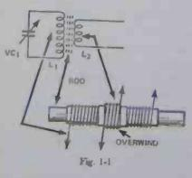
A ferrite-rod may have anything from one to four main windings (L1 in Fig. 1-1) parallel-tuned with a variable capacitor (VC1 in Fig. 1-1). These coils will be for medium; medium and long; trawler-band, medium and long; short, trawler-band, medium and long; or short, medium and long
