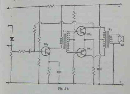
When selecting replacements for any set, always make sure about the polarity of the existing transistors. It is not always safe to trust entirely to the type-number of the transistor as sole evidence; if you have access to the maker's service data, check this also as confirmation. If the set has been tampered with or serviced carelessly or incompetently there is always the chance that someone has fitted a wrong type of replacement transistor! If you inadvertently copy their error you will prob-
