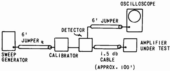
Fig. 13-8. VSWR test setup.
