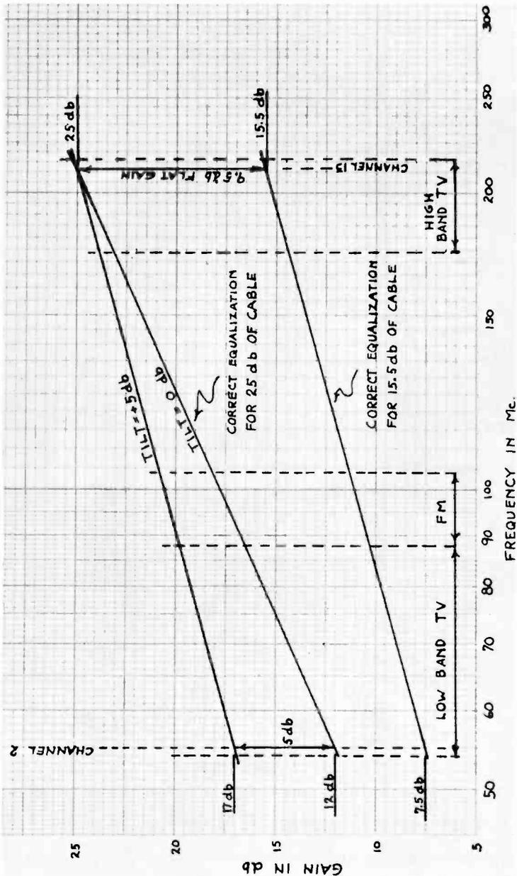
Fig. 10-3. Graph showing function of tilt control.
