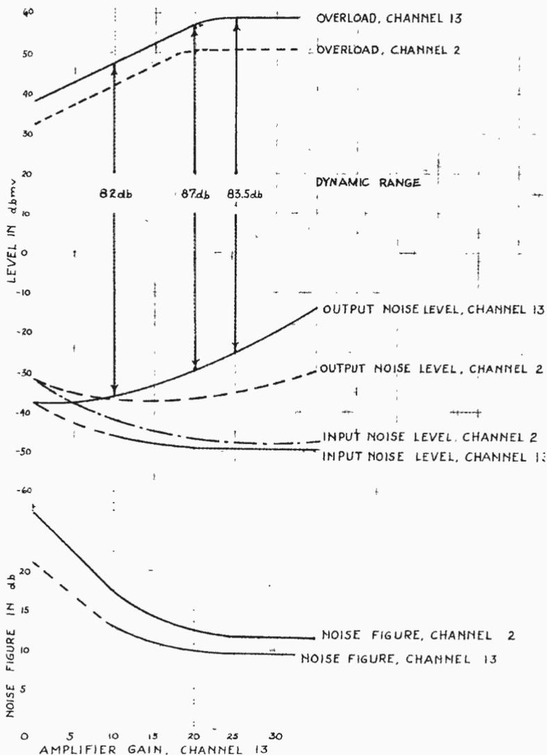
Fig. 7-1. Optimum amplifier gain chart.
