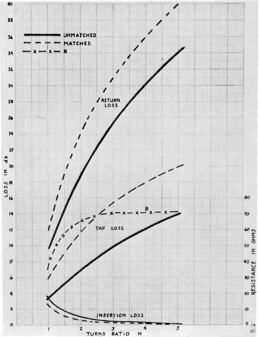
Fig. III-3. Transformer tap design graph.
