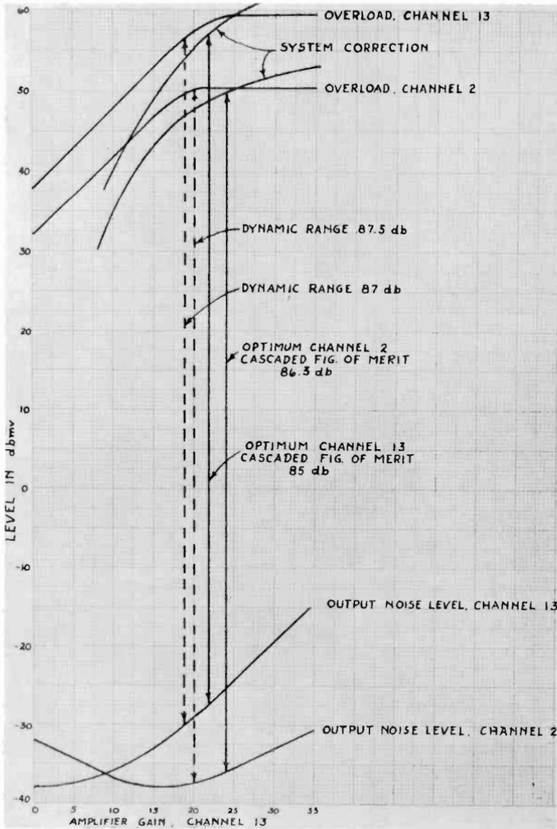
Fig. 7-2. Graphical analysis of amplifier dynamic range and cascaded figure of merit.
