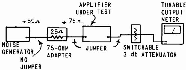
Fig. 13-11. Diagram of noise figure test setup.
