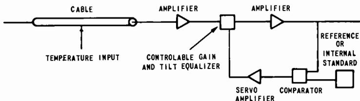
Fig. 11-2. Block diagram of a closed-loop AGC system.
