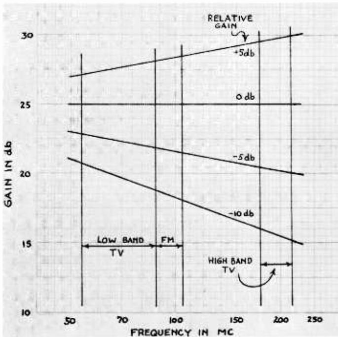
Fig. 10-2. Graph showing action of tilt-compensated gain control.
