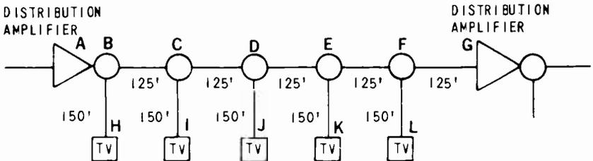
Fig. 8-4. Block diagram of a typical distribution system. Points of mismatch are indicated by letters.
