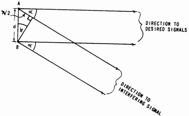
Antenna locations at A and B, spaced distance  $d$  apart. Spacing must be such, that signal at A is delayed by one half wavelength, hence  $d = \lambda/2 \sin \alpha$ . Read  $d$  in wavelengths of the interfering station for any angle from graph below.
