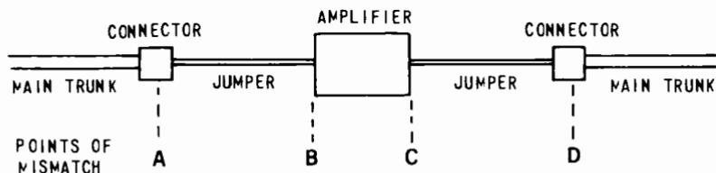
Fig. 5-1. Illustration of mismatches caused by jumper cables.
