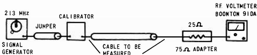
Fig. 13-6. Diagram of setup to measure cable loss.
