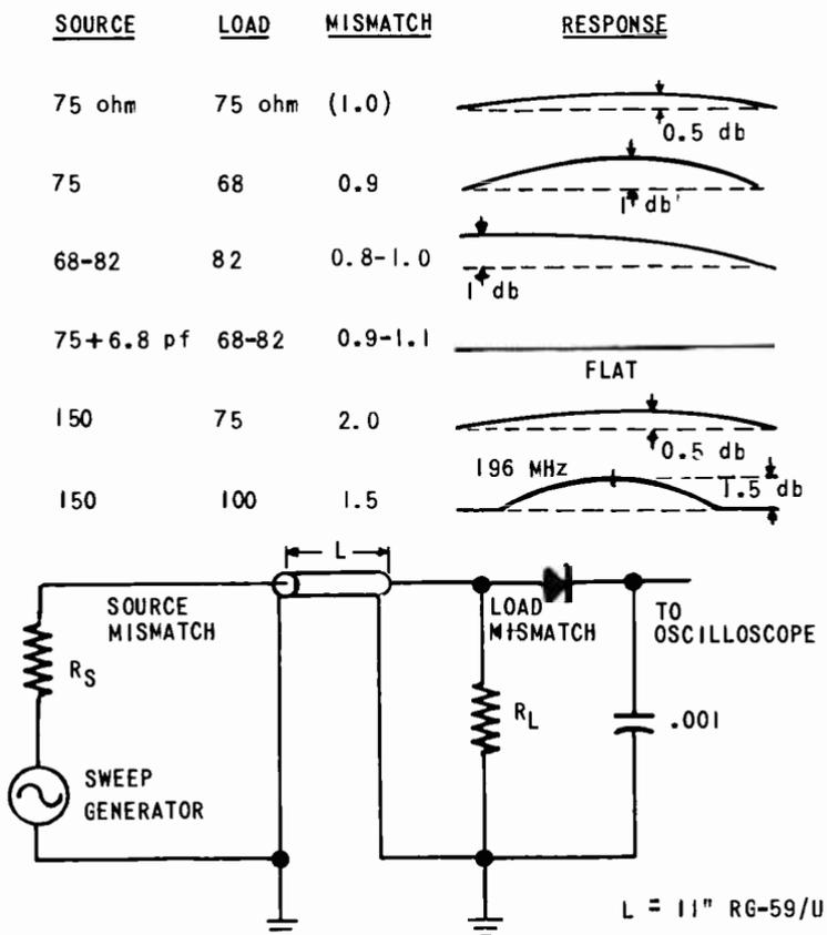
Fig. 5-3. Effect of input or output jumper cable.
