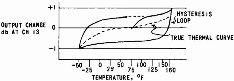
Fig. 13-14. Thermal hysteresis curve.
