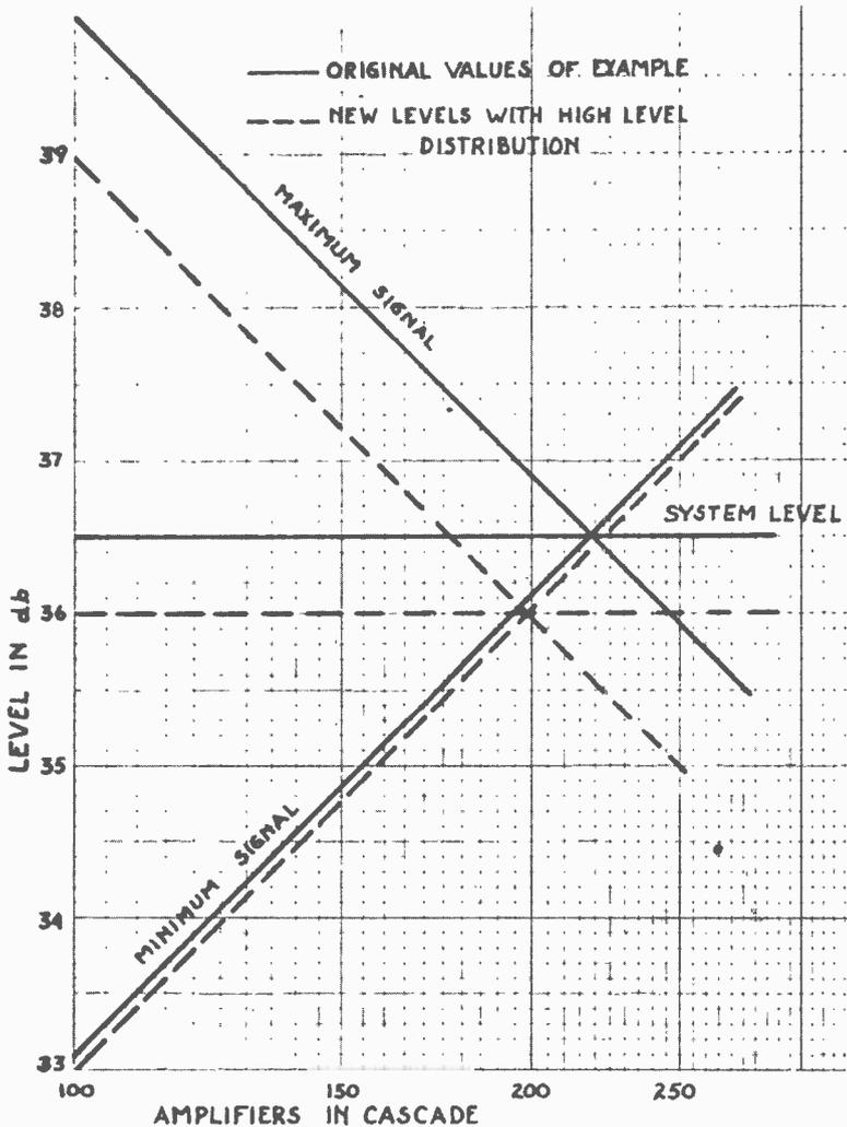
Fig. 9-2. Derating curve for high-level distribution. dynamic range. The calculation is readily performed using power addition,\* and we find for this example that the main trunk must be derated by 0.95 db. This main-trunk derating must be made from the combined overload level of the main trunk only, which is 36.7 dbmv, and is slightly higher than for the cascade including the distribution amplifiers. Thus, system level would have to be reduced to 35.7 dbmv.
