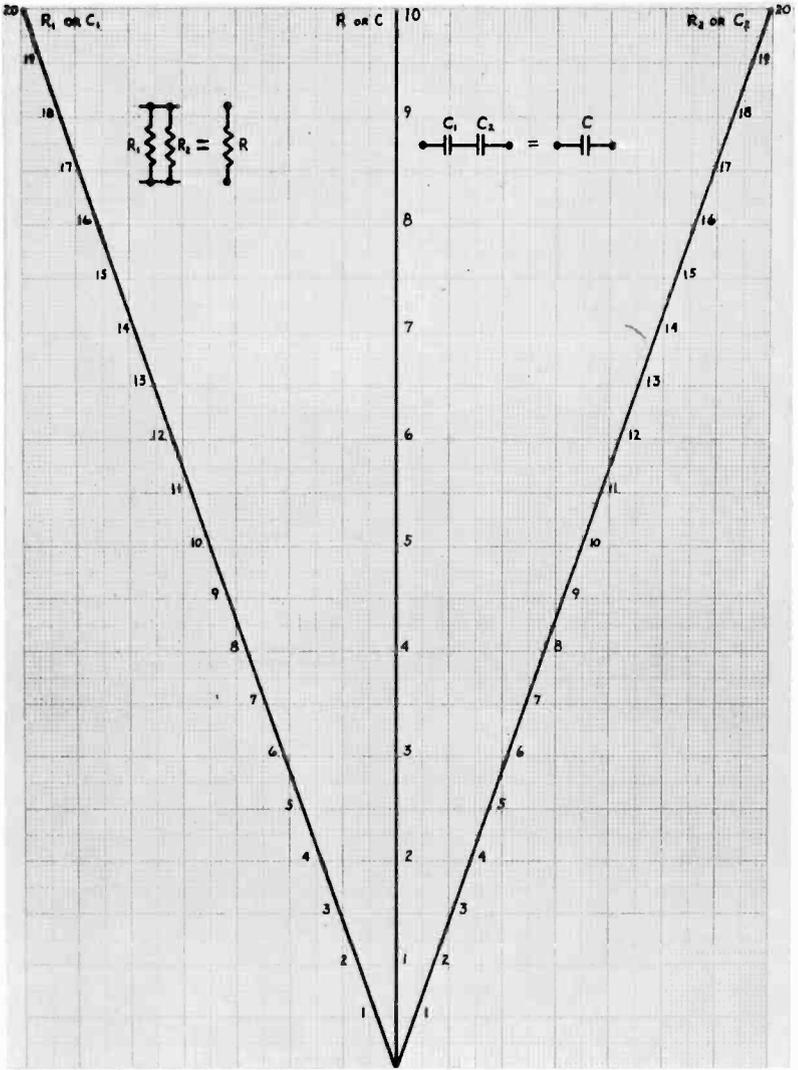
28. Parallel resistors or series capacitors.
