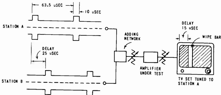
Fig. 3-5. Illustration of "windshield wiper" effect.
