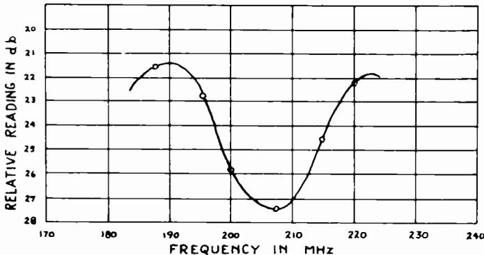
Fig. 10-1. Curve showing error with old-style 20 db test point.
