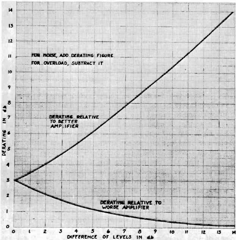
Fig. I-1. Cumulative noise or overload level curves.
