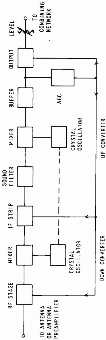
Fig. 2-2. Block diagram of a typical reconversion head end.
