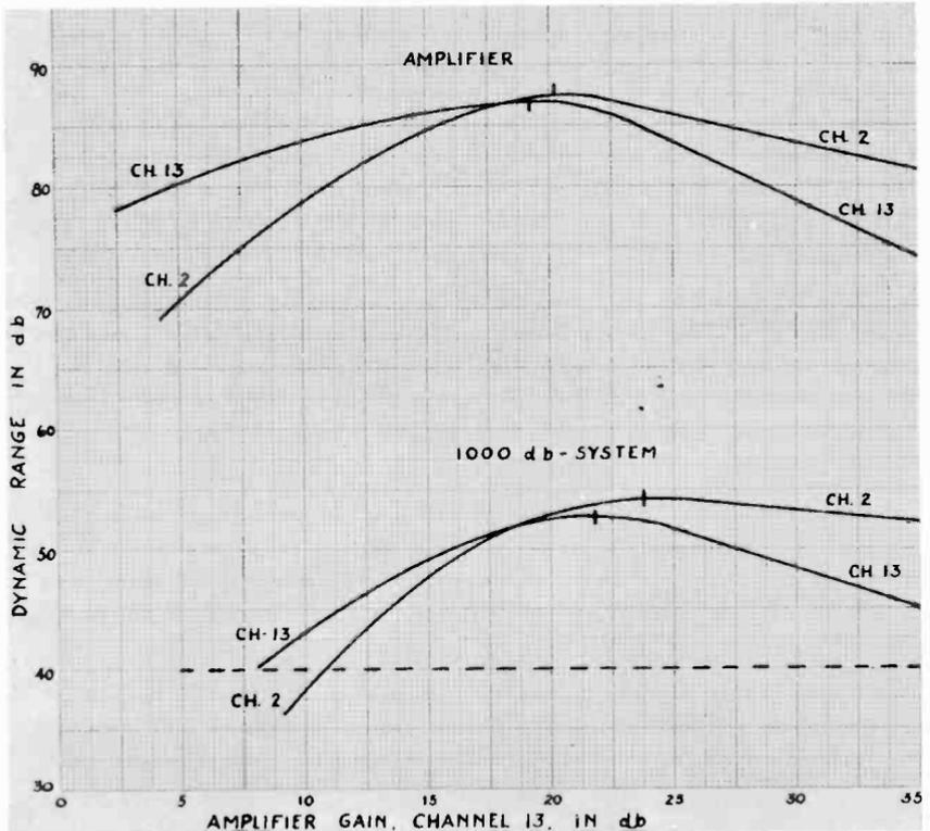
Fig. 7-3. Amplifier and system dynamic range curves. lems in the equalization of bridger amplifiers. Also, it necessitates even more the use of midspan bridgers with their difficult equalization problems. With lower gain amplifiers, midspan bridgers can be more readily avoided. Also, bridgers can be built into the same housing with the main trunk amplifiers, thereby avoiding special equalization problems.
