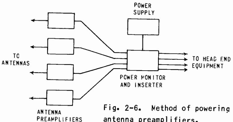
Fig. 2-6. Method of powering antenna preamplifiers.
