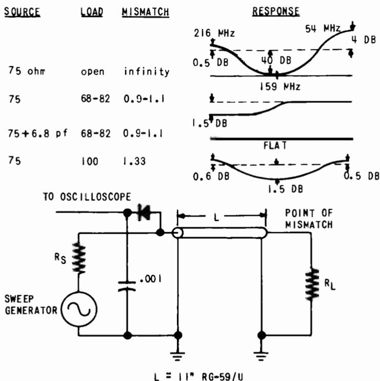
Fig. 5-4. Effect of jumper cable on taps or bridgers.
