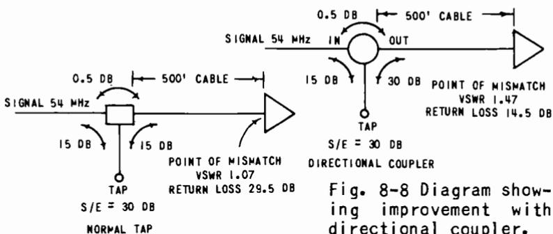
Fig. 8-8 Diagram showing improvement with directional coupler.
