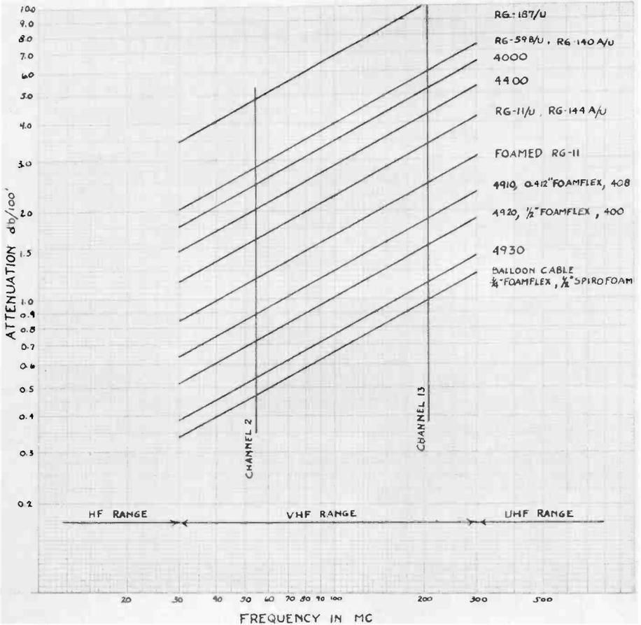
Fig. 3-1. Typical coaxial cable attenuation curves. 50 to 220 MHz, a straight-line approximation may be used. In CATV work, it is common practice to specify cable length in db attenuation at the highest channel in use (Channel 13, or 213 MHz, for modern all-band systems). Fig. 3-2 shows the attenuation characteristic of typical high-quality coaxial cable for 25 db cable length, a common spacing between repeater
