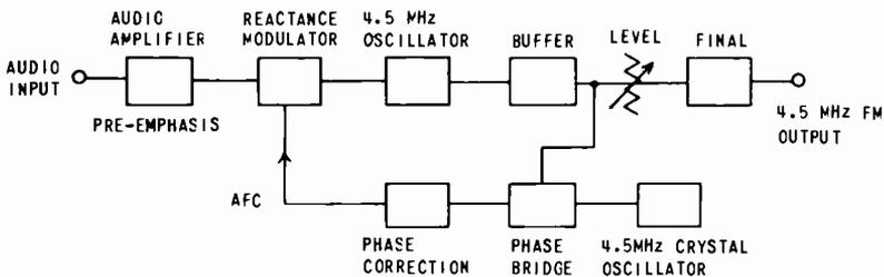
Fig. 2-5. Block diagram of a 4.5-MHz FM audio modulator.
