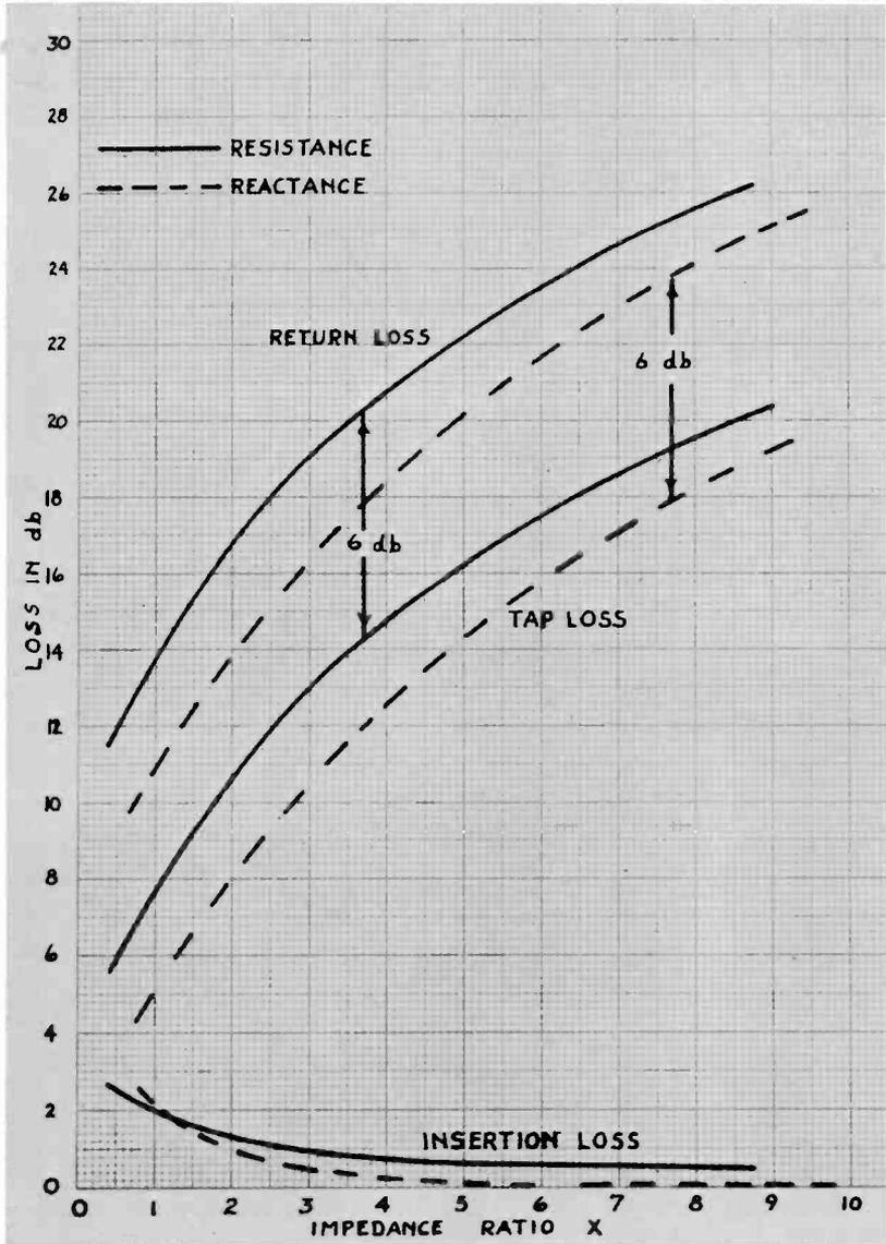
Fig. III-2. Series-impedance tap design graph.
