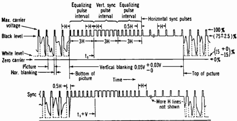
7. Composite TV waveform showing sync and blanking pulses.  $V = 1/60$  sec.  $H = 1/15,750$  sec.
