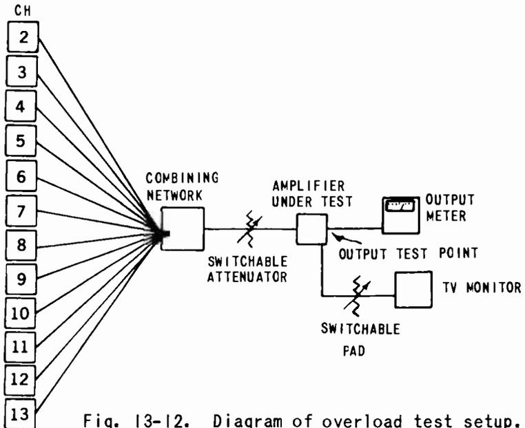
Fig. 13-12. Diagram of overload test setup.
