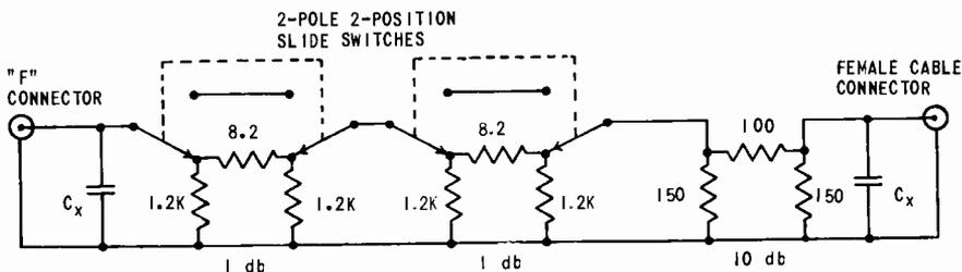
Fig. 13-2. Calibrator schematic.
