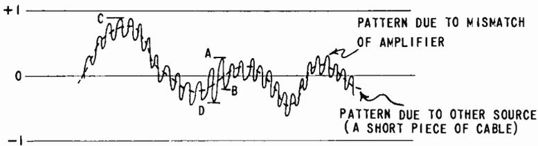
Fig. 13-10. Superimposed VSWR pattern caused by multiple reflections.
