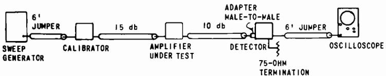
Fig. 13-7. Diagram of alignment and gain test setup.
