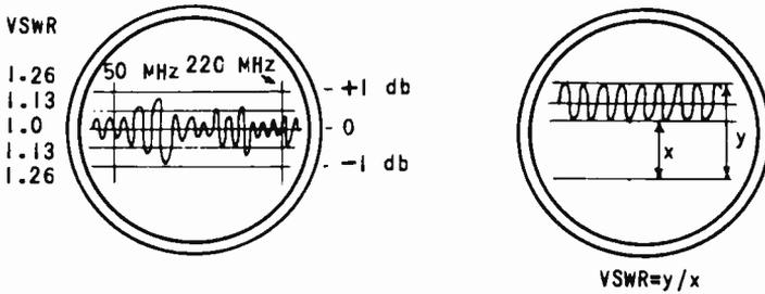
Fig. 13-9. VSWR oscilloscope patterns.
