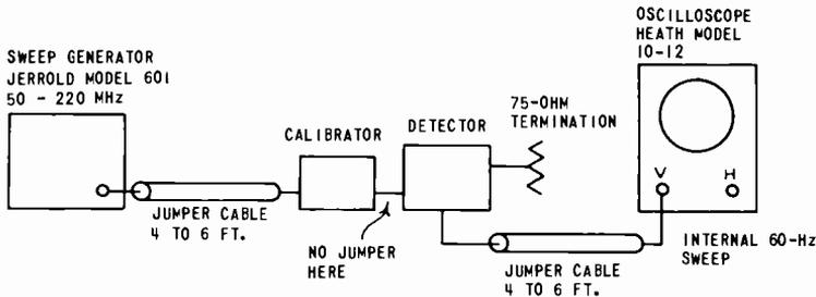
Fig. 13-1. Calibration setup diagram for amplifier alignment.
