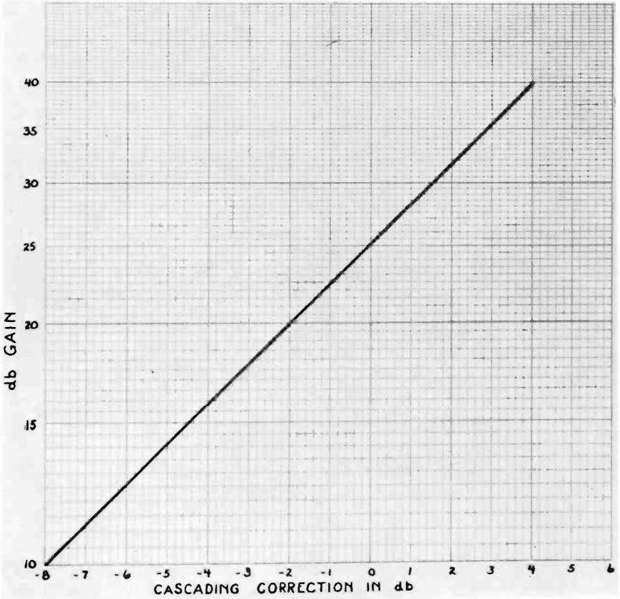
Fig. 3-7. Correction chart for cascaded amplifier figure of merit.
