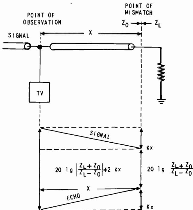
Fig. 8-2. Diagram showing echo generation.
