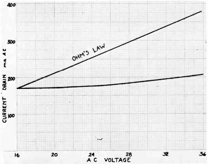
Fig. 12-1. Power characteristics of a typical CATV amplifier.
