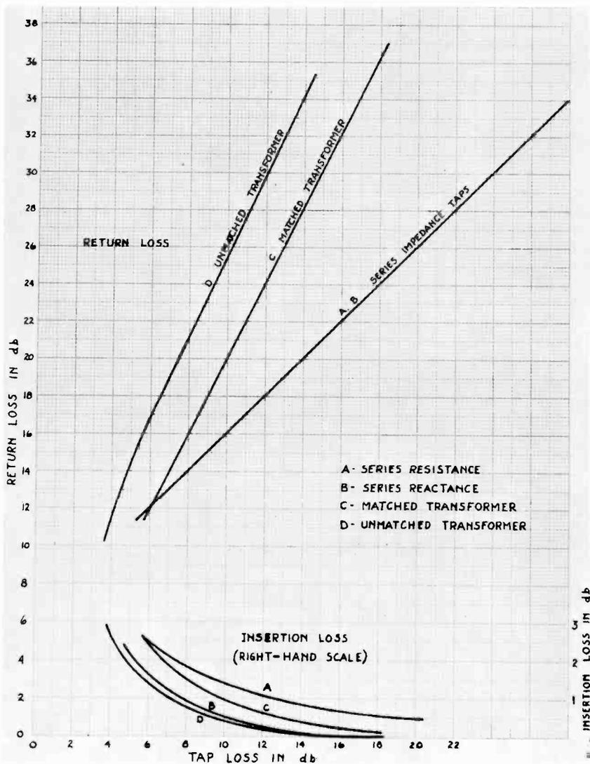
Fig. III-4. Graphical comparison of tap types.
