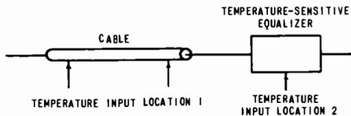
Fig. 11-1. Block diagram of an open-loop AGC system.
