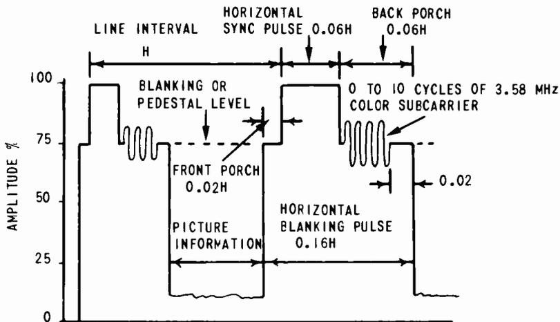
9. Detailed sketch of horizontal blanking and sync pulses.
