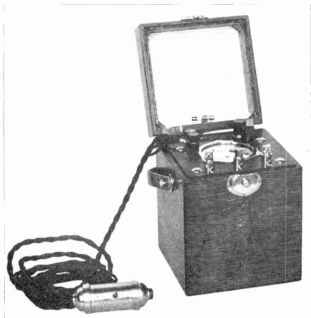
Fig. 66. Watthour test meter or rotating standard, used for calibrating watthour meters.
