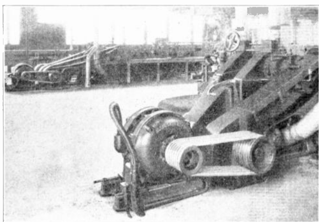
Fig. 155. An A. C. induction motor in use for driving a woodworking machine. The motor is connected to the machine by means of a special rope drive. (Photo courtesy Allis-Chalmers Mfg. Co.)
