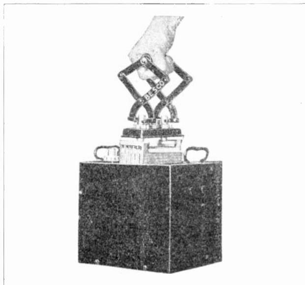
Fig. 36. This view shows a convenient type of cell puller used for lifting plate groups or elements from cell jars when taking down a battery for repairs.
