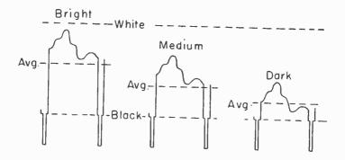
Fig. 14.—Picture signals for backgrounds which are bright, medium, and dark.
