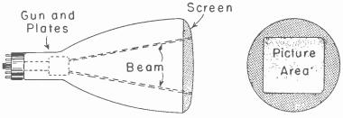
Fig. 7.—A typical picture tube.
