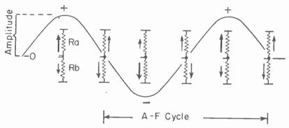
Fig. 9.—Audio-frequency potentials result from variations af electron flows and potential differences in the discriminator resistors.
