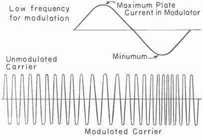
Fig. 20.—Effect of reactance modulator plate current on carrier frequency.
