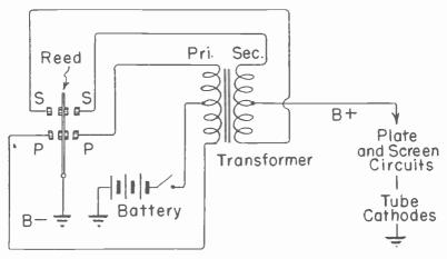
Fig. 13.-Circuit connections for a synchronous vibrator.
