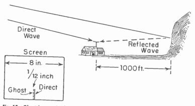
Fig. 15.—Ghost images in the reproduced picture may result from reflected waves.
