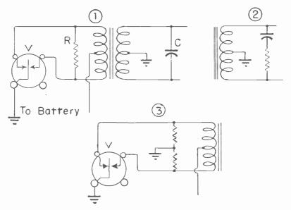
Fig. 12.-Methods of reducing sparking at vibrator points.
