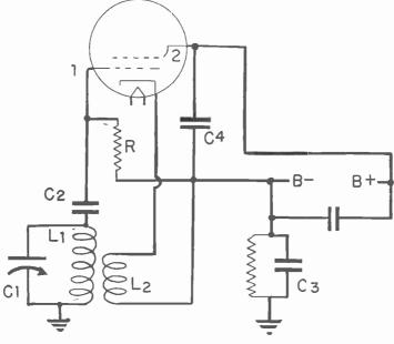
Fig. 6.—The oscillator circuit of the converter.
