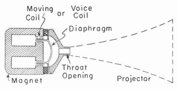
Fig. 22.—A loud speaker driver unit with rigid metallic diaphragm.
