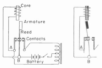
Fig. 10.—How the vibrator reed is made to swing by magnetic action.
