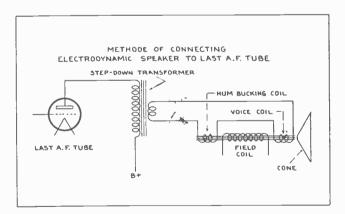
Fig. 23-14.—This figure shows a dynamic speaker connected to the last stage af a radio receiver. Note how the hum bucking coil is connected in series with the voice coil.
