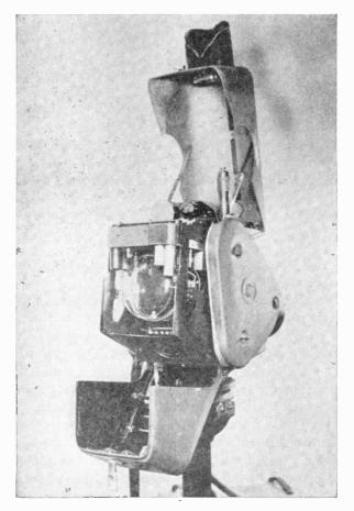
Fig. 2.—A Balaban and Katz television camera used at station WBKB in Chicago.
