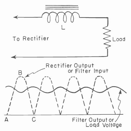
Fig. 21-12.-Choke filter; input and output waveforms.
