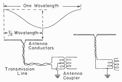
Fig. 14.—The doublet or half-wave dipole antenna.
