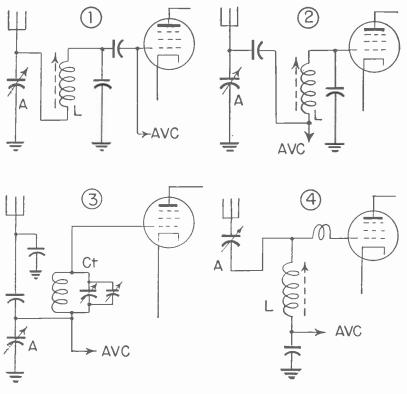
Fig. 3.—Typical auto-radio antenna circuits.
