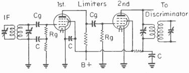
Fig. 6.—Circuits for two limiter stages in cascade.
