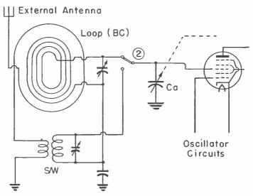
Fig. 2.—Antenna circuits with a built-in loop for broadcast reception.
