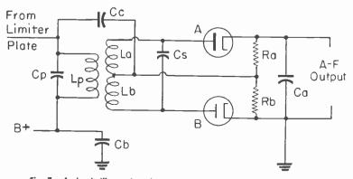
Fig. 7.—A circuit illustrating the general principles of the discriminator.
