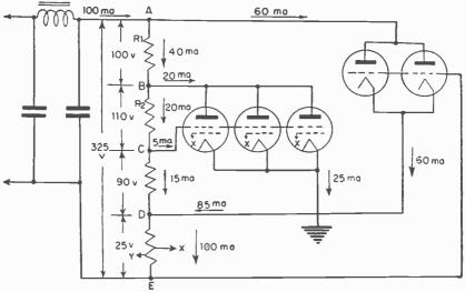
Fig. 21-15.—Typical voltage-divider circuit for receiver.
