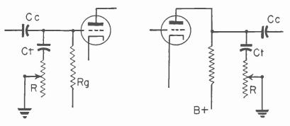
Fig. 19.—Tone control in a grid circuit (left) and in a plate circuit (right).
