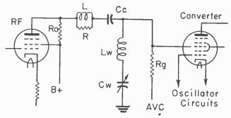
Fig. 9.—A typical untuned coupling between r-f and converter tubes.
