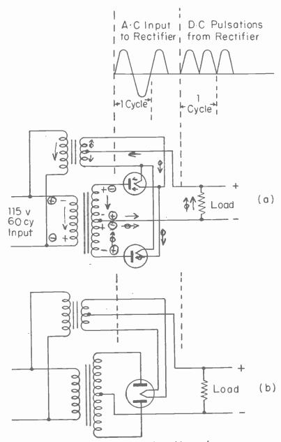
Fig. 21-5.—A full-wave rectifier and its waveforms.
