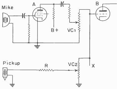
Fig. 20.—An additional amplifying stage for microphone input.
