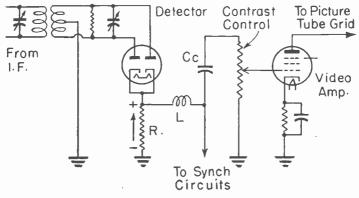
fig. 9.—A full-wave diode detector circuit.
