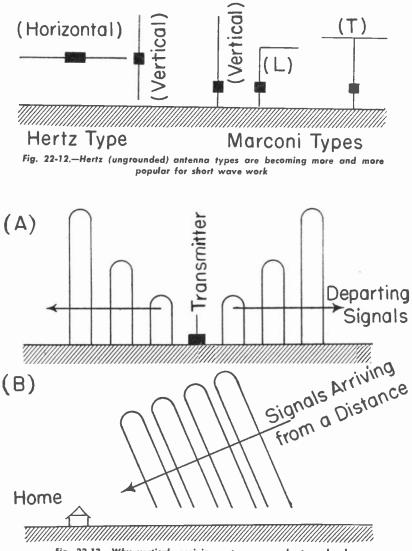
Fig. 22-13.—Why vertical receiving antennas are best on locals, while horizontal types favor distance.
