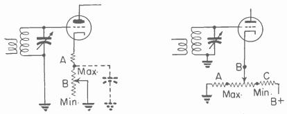
Fig. 4.-Volume control by variation of cathode potential and grid bias.
