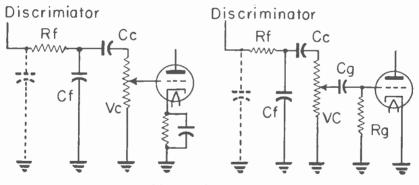
Fig. 19.—Circuits used between discriminator and first a-f amplifier.
