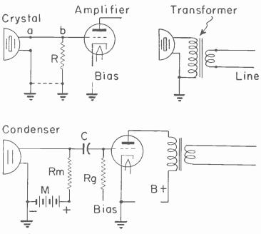
Fig. 12.—Output connections for high-impedance microphones.
