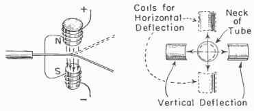
Fig. 8.-The principle of magnetic or electromagnetic deflection.
