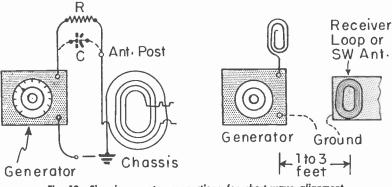
Fig. 13.—Signal generator connections for short-wave alignment.
