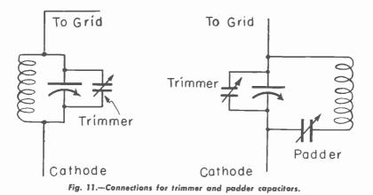
tuning capacitor, and is arranged for adjustment of its capacitance by means of a screwdriver or wrench. For a 360 mmfd tuning capacitor the trimmer may have a maximum capacitance of 15 to 25 mmfd. The trimmer capacitance is a small percentage of the maximum capacitance of the tuning capacitor, but is a large percentage of its minimum capacitance. Consequently, adjustment of trimmers has greatest effect at high frequencies where
