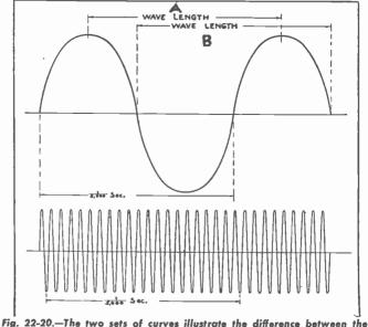
frequency of sound waves and radio waves.
