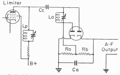
Fig. 18.—A discriminator circuit having phase displacement for only one of the rectifier lines.
