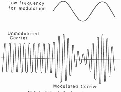
Fig. 2.—Amplitude modulation of a carrier wave.
