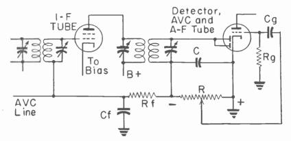
Fig. 9.—The elements of a simple automatic volume control circuit.
