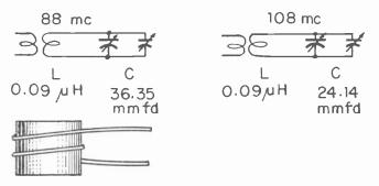
Fig. 12.—Inductances and capacitances for resonance in the f-m range.
