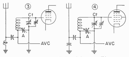
Fig. 4.—Antenna circuits feeding into radio-frequency amplifying tubes and converters.
