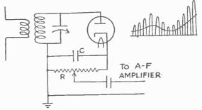
rig. 22-32.—Using a diode tube for a detector.
