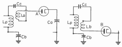
Fig. 10.—The diode rectifier circuits which include the primary of the transformer.
