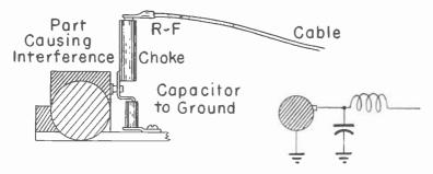
Fig. 18.—Connections of capacitor and choke coil to a part causing interference.
