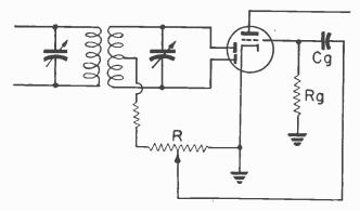
Fig. 8.-Volume control on a full-wave diode detector.
