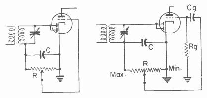
Fig. 5.—Volume controls in diode detector circuits.
