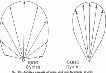
Fig. 25.—Relative spreads of high- and low-frequency sounds from a loud speaker.
