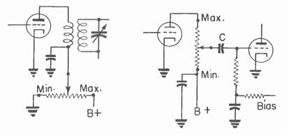
Fig. 3.-Volume controls in amplifier plate circuits.
