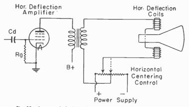
Fig. 22.-A magnetic horizontal deflection system for the picture tube.
