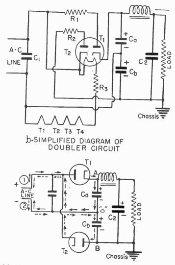
DOTTED LINE---->Indicates Direction of Charging Current Flow When(2) is Positive
