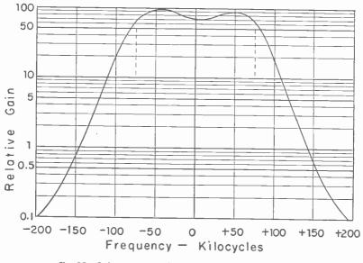
Fig. 15.—Gain at various deviations in a typical i-f system.
