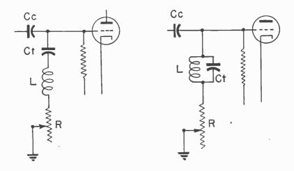
Fig. 22.-Tone controls employing tuned resonant circuits.
