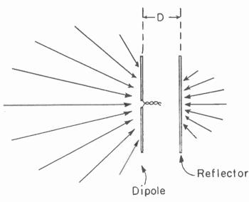
Fig. 16.—A reflector used with a dipole antenna.
