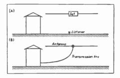
Fig. 22-14.—The theoretical ideal (A) and the practical substitute (B). extreme simplicity of this arrangement is evident. Its anti-noise action leaves little to be desired, it is easy to erect, the line can be of any convenient length upward of some 40 feet (be sure to use that much and coil up any you don't need inside the set cabinet) and strong wind does little damage.
