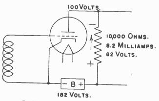
Fig. 23-6.—A load in the plate circuit of the tube.
