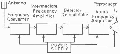
Fig. 1.—Principal parts of a superheterodyne receiver.
