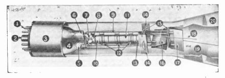
Fig. 4.—The electron gun in one type of DuMont cathode-ray tube. 1, 2 and 3; base collar, base pins, and locating key. 4, 5 and 6; glass stem, getter for gas removal, and glass press. 7 and 8; heater and cathode. 9; supports. 10; control grid. 11; focusing anode. 12; supporting collars. 13; accelerating anode. 14 and 15; supports. 16 and 17; plates for deflecting electron beam. 18 and 19; static shield and connection. 20; glass envelope of tube.
