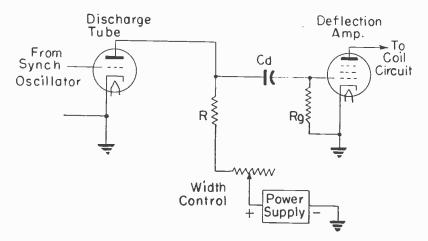
Fig. 19.—How a capacitor may be charged and discharged to produce a sawtooth wave of potential
