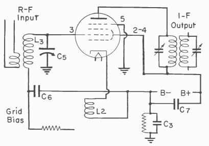
Fig. 7.-The mixer circuit of the converter.
