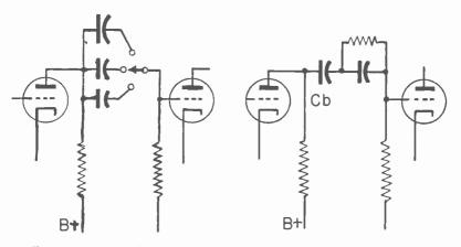
Fig. 21.-Tone controls which reduce the response at low audio frequencies.
