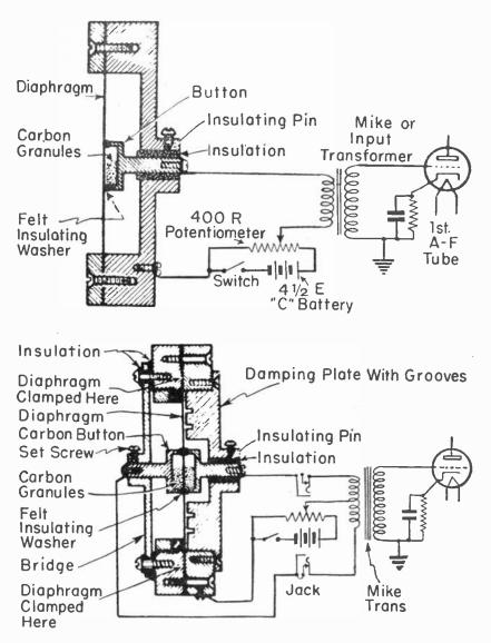
Fig. 11.—A single-button carbon microphone (top) and a double-button type (bottom).
