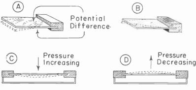
Fig. 7.—The flexing of a piezo-electric crystal produces potential differences between the crystal faces.
