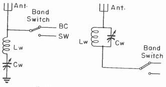
Fig. 11.—Wave traps in the antenna circuit.
