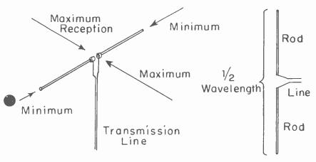
Fig. 7.—A half-wave dipole antenna.
