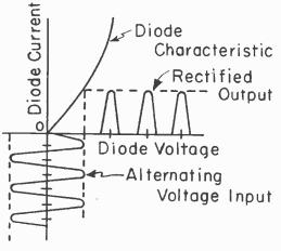
Fig. 21-2.—A diode as a rectifler with A-C on the plate.
