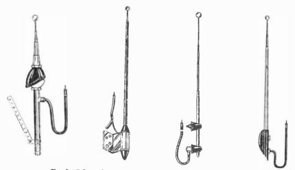
Fig. 1.--Telescoping types of auto-radio antennas. (Spirling)
