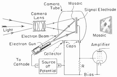
Fig. 3.—The relation of the lens and picture tube in a television camera.
