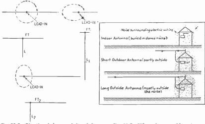
Fig. 22-8.—Directional characteristics of the "T" and inverted "L" antennas.
