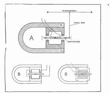
Fig. 23-11.—These sketches show the construction of the loudspeaker driving units or reproducers of the balanced armature type.
