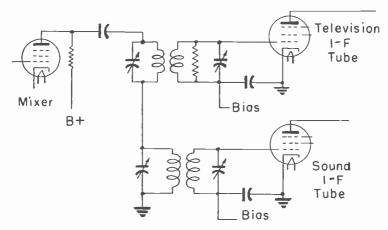
Fig. 5.—I-f transformers for television and for sound, with the primaries in series.
