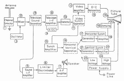
Fig. 2.—Paths followed by various signals through principal parts of a television receiver.
