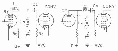
Fig. 10.-Wave traps in the plate circuit of an amplifier tube.
