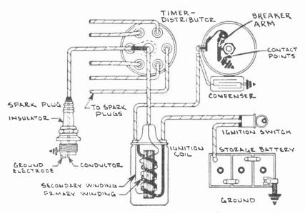
Fig. 17.—The parts and their connections in an automobile ignition system.
