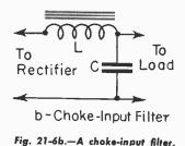
from the rectifier. Fig. 21-6a shows a condenser-input filter sometimes referred to as a *pi* section and Fig. 21-6b shows a chokeinput filter. Further subdivisions of these filters can be made according to the number of sections of filter elements used.
