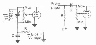
Fig. 2.--Volume controls in amplifier control grid circuits.
