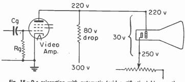
Fig. 15.—D-c reinsertion with automatic (grid rectification) bias on the video amplifier tube.
