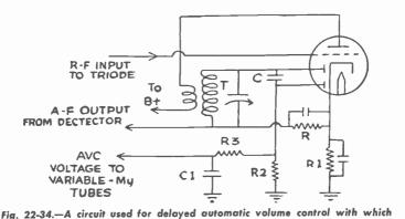
Fig. 22-34.—A circuit used for delayed automatic volume control with whic weak incoming signals are not affected by the automatic features.
