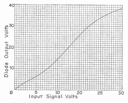
Fig. 6.—Output and signal voltages for a typical diode used for detection.
