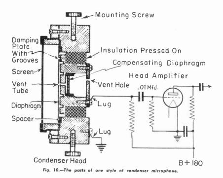
sound waves that reach the diaphragm. Separated from the diaphragm by an air space of about 1/1,000 inch is the stationary back plate or damping plate. The construction of one style of condenser microphone is shown by Fig. 10.
