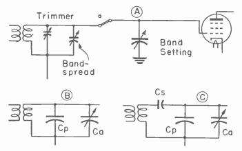
Fig. 6.—Arrangements of tuning capacitors for band spreading.
