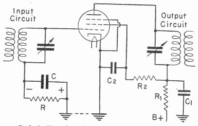
Fig. 5.—A grid capacitor and resistor at the grounded side of the limiter control grid circuit.
