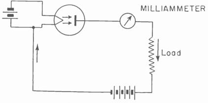
Fig. 21-1.—A diode as a rectifier.
