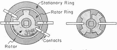
Fig. 3.—One unit of a rotary selector switch.
