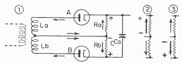
Fig. 8.--The direct-current circuits for the discriminator diodes.
