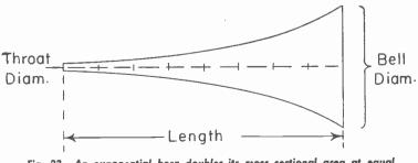
Fig. 23.—An exponential horn doubles its cross sectional area at equal intervals of length.
