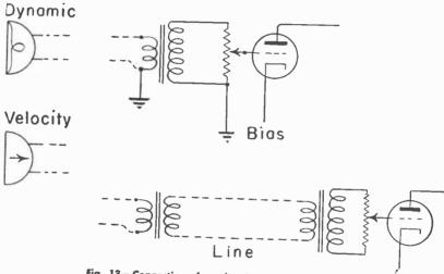
Fig. 13.—Connections from low-impedance microphones.
