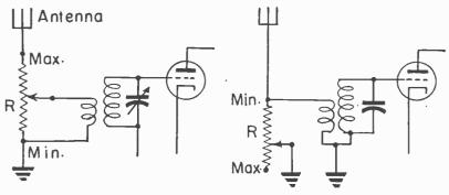
Fig. 1.-Volume controls in the antenna circuit.
