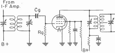
Fig. 1.—The circuit for a limiter stage.
