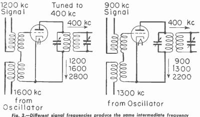
. 3.—Different signal frequencies produce the same intermediate frequency when the oscillator frequency is varied.
