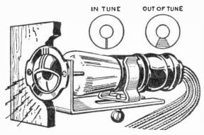
Fig. 15.—An electron ray tube for indicating correct tuning.
