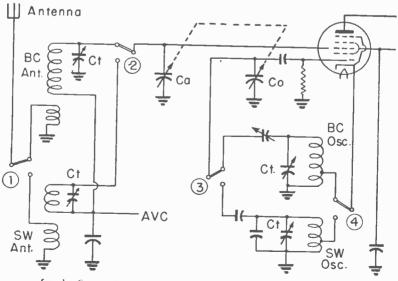
g 1.—Circuits from antenna to converter in a two-band receiver.
