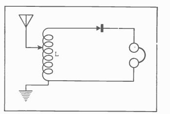
Fig. 22-24.—This sketch shows a circuit for a simple crystal detector radio receiver
