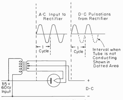
Fig. 21-3.—A half-wave rectifier circuit and its waveforms.
