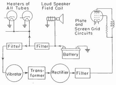
Fig. 7.—Principal units in the power supply system.
