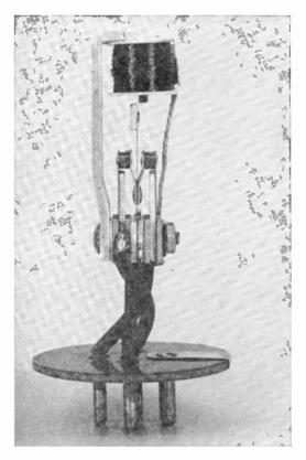
Fig. 11.—The internal construction of a vibrator.
