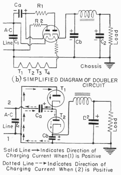
Fig. 21-19.-Common line or series feed of voltage doubler.
