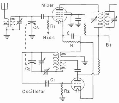
Fig. 14.—Circuits for separate mixer and oscillator tubes.
