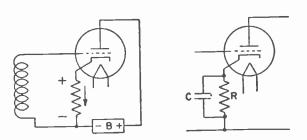
Fig. 23-5.—Negative bias for the grid may be obtained with a resistor in the cathode lead.
