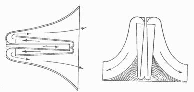
Fig. 24.—Sectional diagrams of folded exponential horns.
