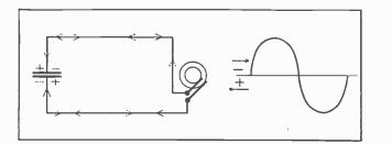
Fig. 22-5.—On the left is shown a curve for one cycle of alternating current. On the right is shown the manner in which the alternating charge a condenser and set up current flow in its circuit.
