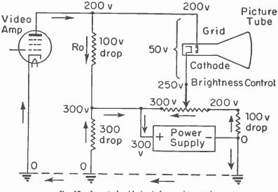
Fig. 13.—A control grid circuit for a picture tube.
