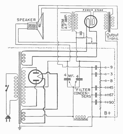
Fig. 23-13.—Diagram of a power supply unit, dynamic speaker, and the last stage of power amplification of a receiver. Note the field cail af the speaker is connected in series with the negative lead of the D.C. plate supply and serves as ane of the filter chokes. Also note the connection of the cone coil, or voice coil to the secondary of the output or speaker coupling transformer.
