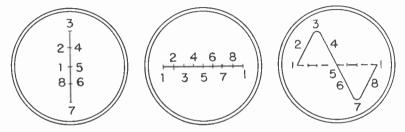
Fig. 7.—Vertical and horizontal deflections combine to trace a curve.
