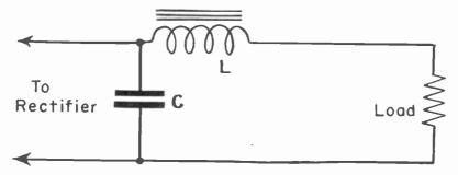
Fig. 21-8.—Choke added to simple capacitor filter to improve filtering action.
