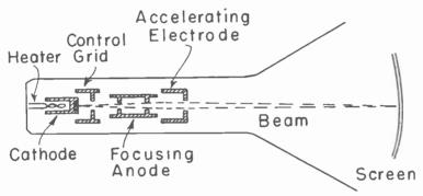
Fig. 9.—Electrostatic focusing of the electron beam in a picture tube.
