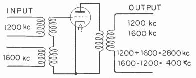
Fig. 2.—Output frequencies produced from two imput frequencies.
