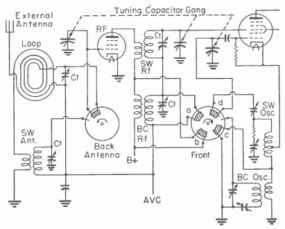
Fig. 7.—An r-f amplifying stage with tuned coupling between the r-f tube and the converter signal grid.
