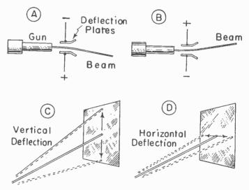
fig. 5.—How the electron beam is bent by electrostatic charges on deflection plates.
