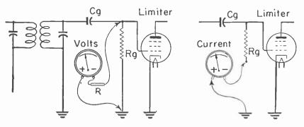
Fig. 2.—Output measurements at the grid resistor of the limiter tube.
