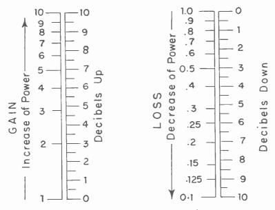
Fig. 4.—Relations between gain or loss and decibel measurements.
