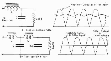
Fig. 21-13.—Single section and two-section choke-input filters, showing input and output waveforms.
