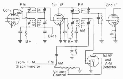
rtg. 17.-Employing the first i-f tube for amplification of both f-m and a-m signals.
