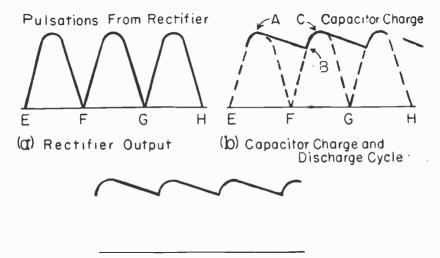
(C) Wave Form of Filter Output Fig. 21-9.--Waveforms of filter of Fig. 8.
