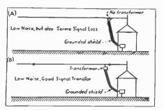
Fig. 22-10-A-B.—Shielded lead ins—poor (A) good (B).
