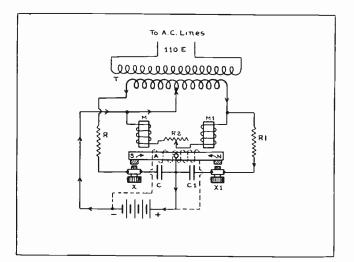
Fig. 2.5. The above diagram shows the parts and connections of a simple mehanical rectifier of the vibrating type. The synchronous operation of the contacts delivers pulsating D.C. to the battery circuit.
