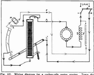
Fig. 127. Wiring diagram for a carbon-pile motor starter. Trace this circuit carefully.
