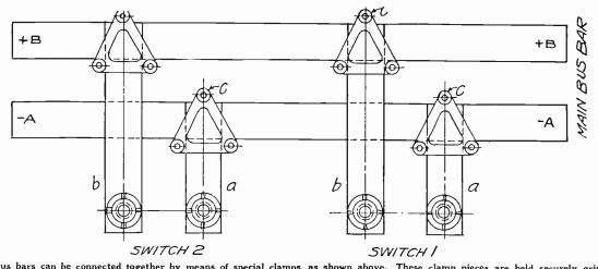
Fig. 72. Bus bars can be connected together by means of special clamps as shown above. These clamp pieces are held securely gripped to the busses by means of short bol's through the holes in their three corners. Clamps of this type save the trouble of drilling the copper busses.
