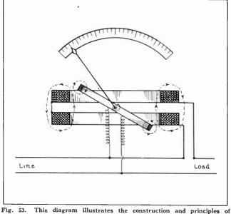
Fig. 53. Inis diagram illustrates the construction and principles of the dynamometer type instrument. Note the action between the flux of the moving and stationary coils.
