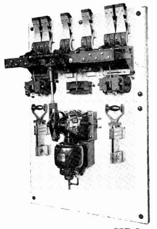
Fig. 63. Large, heavy duty circuit breaker equipped with a motor for automatic reclosing, after it has been tripped either by an overload, or by remote control.
