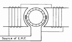
Fig. 110. Diagram of the connections for a simple shunt motor. 127. STALLING TORQUE OF SHUNT MOTORS
