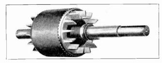
Fig. 200. Complete rotor of the double squirrel-cage type. Note that there are no open slots around the rotor core, the bars being cast into the rotor.
