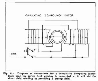
to lower the counter-E. M. F. sufficiently to allow enough current to flow to carry the load. The stronger the field of any motor, the lower will be the speed at which it can generate the normal counter-E. M. F.
