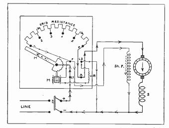
ig. 122. Wiring diagram of a 4-point starter for speed regulating. Observe the connections and operating principle carefully.
