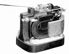
Fig. 59. This photo shows a meter element with part of the magnetic shield in place around it. These shields are made of soft-iron laminations and prevent magnetic flux from other machines or circuits from interfering with the accuracy of the meter. One-half of the shield is shown removed in this view.
