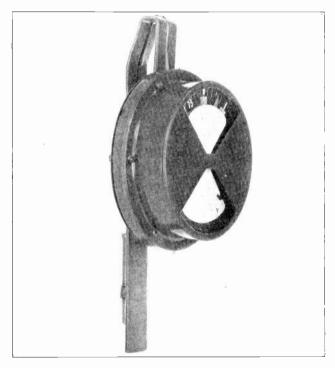
Fig. 112. This pho'o shows a temperature-indicating device for use with pole type transformers. This device is called a thermotel and indicates both excessive temperatures and overload of a transformer on which it may be installed.
