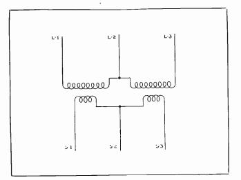
Fig. 131. Connections for using two single-phase transformers to provide three-phase service by what is called the "open-delta" connection.
