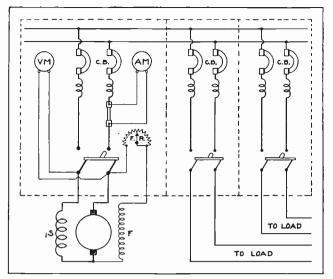
Fig. 74. The above diagram shows the wiring and equipment for a simple switchboard with one generator panel and two distribution panels.
