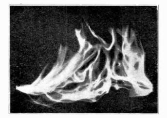
Fig. 2. The above view shows a high voltage arc created by passing current at a potential of several hundred thousand volts through air.
