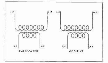
Fig. 117. This sketch shows windings of two transformers with their leads properly marked for subtractive and additive polarities.
