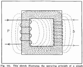
transformer and shows the manuer in which the primary flux passes through the core and induces voltage in the secondary winding.
