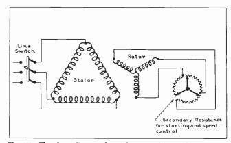
Fig. 183. The above diagram shows the connections of the stator and rotor of a slip-ring induction motor, and also the variable resistance used in the rotor circuit for starting and speed control.
