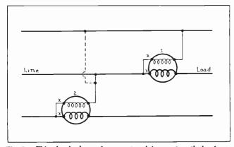
Fig. 38. This sketch shows the correct and incorrect methods of connecting one of the wattmeters when measuring three-phase power by the "two wattmeter method".
