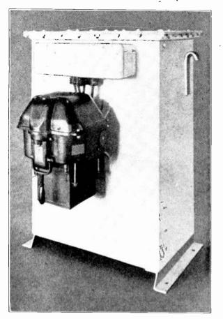
Fig. 217. This photo shows a static condenser enclosed in a moistureproof metal tank and equipped with an oil switch for breaking the circuit between the condenser and the line. These condensers are made for both indoor and outdoor service. (Courtesy Electric Machinery Mfg. Co.)
