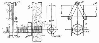
Fig. 73. Two views showing the method of connecting bus bars to the stude of switches and circuit breakers.
