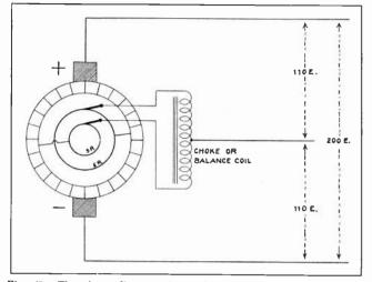
Fig. 45. The above diagram shows the commutator, slip rings, and balance coil of a three-wire D. C. generator.
