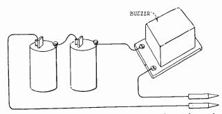
Fig. 155. A simple test set consisting of dry cells and buzzer is a very effective device for trouble shooting and locating of faults in electric circuits and machines.
