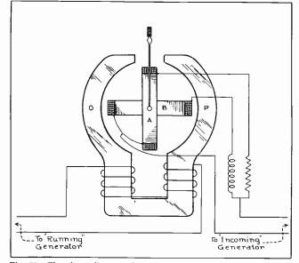
Fig. 75. The above diagram shows the important parts and illustrates the principles of a synchroscope. This diagram also shows the connections of the coils to the "running" and "incoming" generators.
