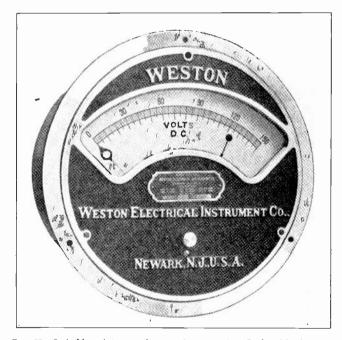
F.g. 77. Switchboard type voltmeter for mounting flush with the surface of the board. No e the stationary index pointer or marker, to indicate when full voltage is reached by the movable pointer.
