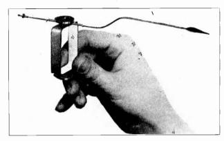
Fig. 76-A. An excellent view of the movable coil, pointer and spring of a D. C. meter.
