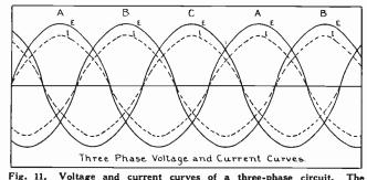
Fig. 11. Voltage and current curves of a three-phase circuit. The voltage is shown by the solid lines and the current by the dotted lines.
