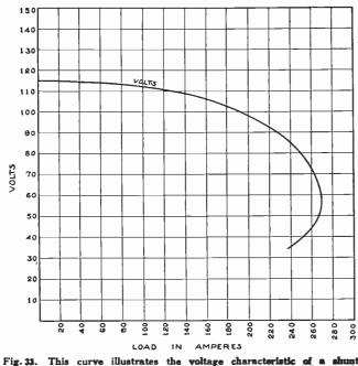
Fig. 33. This curve illustrates the voltage characteristic of a shunt generator. Note how the voltage drops as the load in kilewatts is increased. Full load in this case is 240 amperes.
