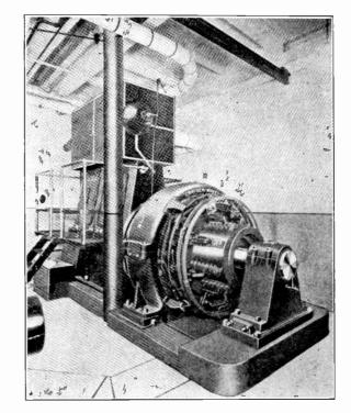
Fig. 42-A. Large D. C. generator driven by a vertical engine. If this machine is rated at 250 volts and 3000 amperes, what is its capacity and KW?
