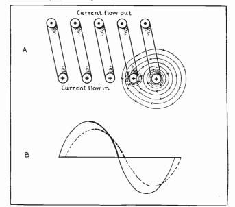
Fig. 18. This sketch shows the same coil as in Figs. 16 and 17 during a period when the current through the coils is decreasing from maximum to zero value. Note how the flux contracts and cuts across the turns of the coil.
