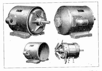
Fig. 209. Completely enclosed A.C. induction motor with special airjacket to direct the cooling air over the surface of the motor casing. These motors are ideal for use in extremely dirty locations or in places where there are explosive vapors or dust.
