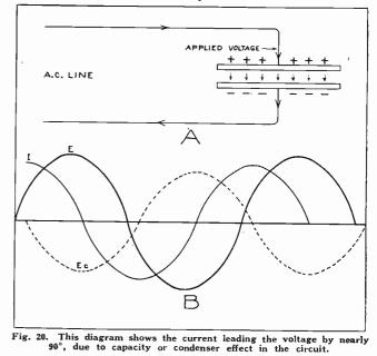
You will note at the first curve on the left that the current reaches maximum value just a little later than the applied voltage starts from zero value. Then, as the applied voltage keeps on increasing, the counter-voltage, Ec, of the condenser is building up and reduces the flow of current, until it reaches zero value just after the applied voltage reaches maximum.
