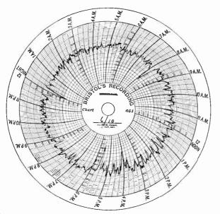
Fig. 94. Paper disk or chart from a direct acting recording meter. The irregular black line shows the voltage curve traced by the pointer and pen throughout each hour of the day and night.
