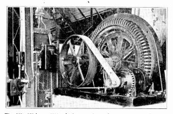
Fig. 192. 150-h. p., 2300-volt, low-speed, synchronous motor and exciter. The speed of the large motor is 144 RPM. (Photo courtesy Allis-Chalmers Mfg. Co.)
