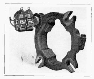
Fig. 20. Above are shown two brushes in their holders which are mounted on a brush rocker arm for a four-pole machine. Note the coil springs by which the brush tension on the commutator can be adjusted.
