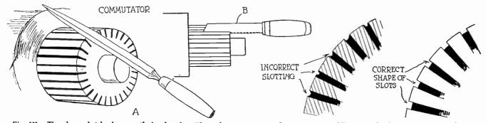
Fig. 151. The above sketch shows methods of undercutting mica segments on the commutator. Mica must be kept down even with, er below the surface of the commutator bars, or it will cause the brushes to make poor contact and cause severe sparking.
