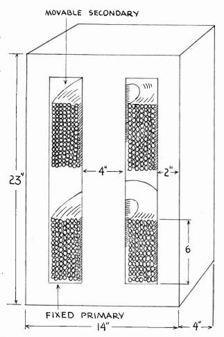
Fig. 153-D. A 10 Kv-a. welding transformer designed for operation on a 220 volt line.
