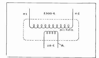
Fig. 119. The above sketch shows a schematic diagram of the primary and secondary windings of a single-phase transformer. This transformer has a step-down ratio of 20:1 and one side of the secondary is grounded, as is common practice.
