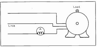
Fig. 33. Ammeter connected to measure the current in one phase of a three-phase motor.
