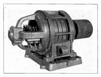
Fig. 182. This photo shows a complete slip-ring motor to which variable resistance can be connected for starting and speed-regulating duty. Note the slip rings and rotor connections on the left-hand end of the machine. (Photo courtesy General Electric Co.)
