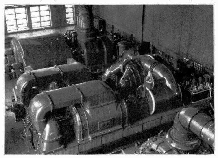
Fig. 3. Modern steam generators of the above type produce many millions of h. p. of electrical energy, for use in lighting and the operation of power machinery. The generator shown in this photo is of 165,000 kw. capacity and is driven by steam turbines. (Photo courtesy of American Brown Bovery Co.)
