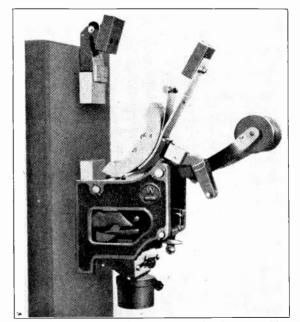
Fig. 66-B. This view shows the same circuit breaker as in Fig. 66-A, except that it is now in open position. Again note carefully the construction and position of the main contacts and arcing contacts. Also note the trip adjustment on the bottom of the breaker.
