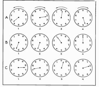
Fig. 92. The above sketches, A, B, C, show the dials of a kilowatthour meter in three different positions. If you will practice reading each set of these dials with the instructions here given, you will be able to easily and accurately read any KW-hour meter.
