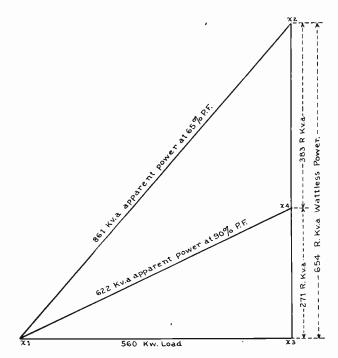
Fig. 121. This diagram also shows the reduction obtained in the apparent power and wattless power by improving the power factor of a system. By carefully measuring the top section of the vertical line in the diagram we can find the size of the condenser required to correct the power factor.
