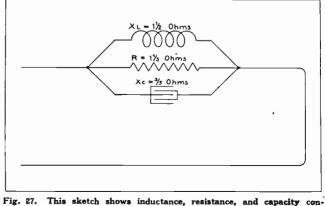
Fig. 27. This sketch shows inductance, resistance, and capacity connected in parallel. The method of determining the impedance of such a circuit is thoroughly explained on this page.
