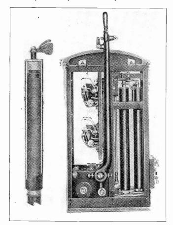
Fig. 126. Carbon-pile rheostat for starting D. C. motors very gradually. On the left is shown one of the carbon resistance elements used with such starters.
