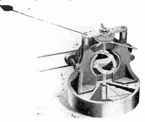
Fig. 49. Another dynamometer type meter with slightly different arrangement of the coils. Note the damping vane attached to the bottom end of the shaft so that it rotates in the damping chamber under the meter element.
