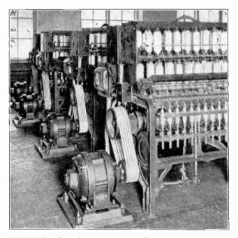
ig. 154. This photo shows a group of machines in a textile mill. each of which is driven by an individual A. C. motor.
