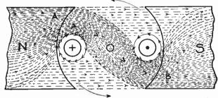
Fig. 167. The above diagram illustrates the manner in which the reaction between the lines of force from the armature and field windings set up the torque or turning effort in a motor.
