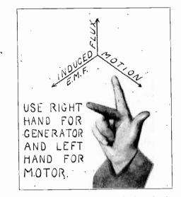
Fig. 22. This figure shows a method of holding the fingers to use the right-hand rule for determining direction of induced voltage in generators.
