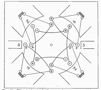
7. 56. This simple sketch illustrates the manner in which two interpoles can be used to neutralize self-induction in the coils of a four-pole machine. Fig. 56.
