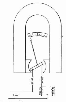
Fig. 105. This diagram shows a meter designed for reading two different voltages.
