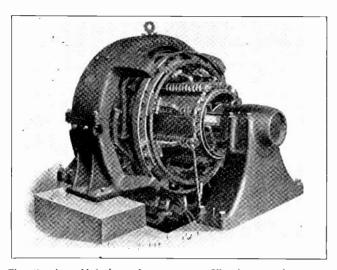
Fig. 46. Assembled three-wire generator. Slip rings can be seen at the right-hand end of the commutator. If this machine is rated at 500 KW, what should the maximum load in amperes be on both of the 110 volt circuits it supplies?
