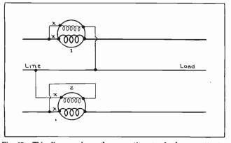
This diagram shows the connections to the lower Fig. 37. wattmeter reversed to obtain proper readings on circuits with low pov factor.
