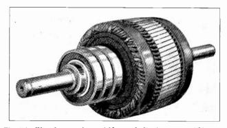
Fig. 181. Wound rotor of a variable speed slip-ring motor. This rotor has windings of insulated copper wire similar to those in D. C. armatures.
