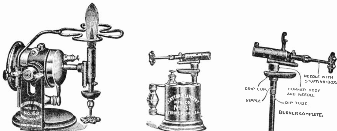
Fig. 25. This view shows the important parts of a blow torch on the right, and at the left the method of using a blow torch in a special stand for heating a lead melting pot.
