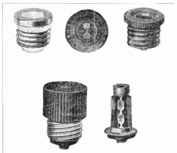
Fig. 106. The three fuses in the upper row are of the ordinary plug type with fusible windows to show when the link is blown out. The lower view shows a refillable plug fuse and one of its refill elements.
