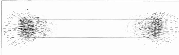
Fig. 5. Sketch of bar magnet showing how iron filings are attracted almost entirely at its ends or poles.
