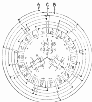
Fig. 82. This diagram shows a six-pole, three-phase winding with the six poles of each phase connected two in series and three in parallel, and then the three phase groups connected star.
