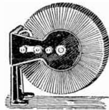
is formed into a nearly closed circle, the ends of the winding being brought together to form the coil into a large ring. See *illustration*.
