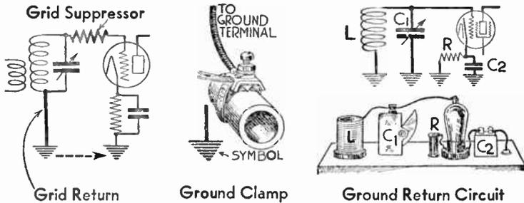
connected to it in a radio device. 2—A connection to such a framework or a short circuit to it. 3—The lower portion of a *capacity antenna*. 4—The earth and all parts conductively connected to it.
