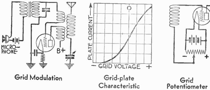
*grid voltage* and *plate current* in a vacuum tube. The mutual characteristic. See *illustration*.
