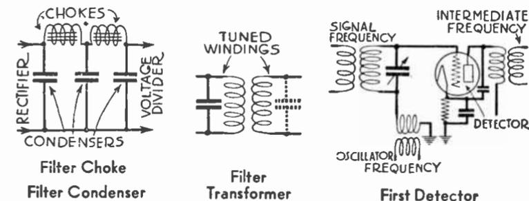
**filter choke.**—An inductance used in a *filter system* to retard the flow of currents at higher frequencies and permit passage of low frequencies or direct current. *See illustration.*
