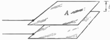
FIG. 2-10. Parallel-plate capacitor.
