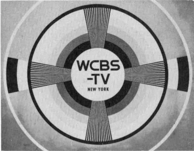
Fig. 107. *Ideal test pattern. Adjust sweep size and linearity for a pattern that most closely resembles the one shown. Don't expect perfection.*
