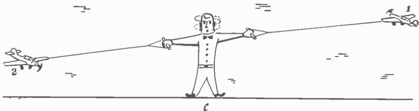
Fig. 1305. Control-line airplanes are used in this analogy of in-phase (a),  $90^\circ$  (b) and  $180^\circ$  phase shift (c).
