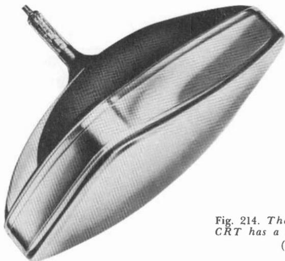
Fig. 214. *The 110° deflection CRT has a short, thin neck.*
