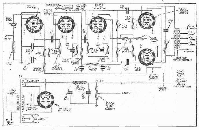
Considering the number of condensers used in isolating circuits from each other, the underchassis wiring is clear and uncomplicated. Resistance-capacity networks are inserted not only in the pre-amplifier plate circuit. but also in the high-voltage lead to the inverter stage. These working in conjunction with the "balanced" inverter circuit, produce an amplifier with remarkable stability.
