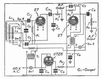
Abave: Wiring diagram for signal generator.
