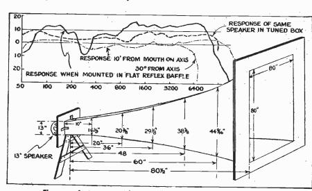
The seven-foot exponential horn. All necessary dimensions are given.
