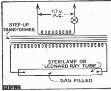
Basic circuit of the Sterilamp, the widely used bactericide.
