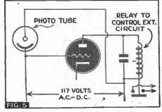
Phototube controls a relay circuit.
