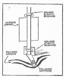
The rounded sapphire tip, which supplants the usual, less-unyielding steel needle, rides in the record groove with a pressure said to be only about 0.9-oz.; its side-to-side motion in a lateralcut record groove wobbles the mirror at audio frequency (\*and can be operated into the supersonic region, it is said), the resulting changes in light intensity on the light-sensitive cell generating a voltage which is then amplified.
