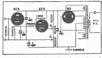
The Electronic Voltmeter above dispenses with expensive meters, using an ordinary 665 electron-ray tube as indicator. If proper care is exercised in its calibration and use, it should be accurate enough for all radio service applications.
