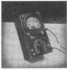
The Ya Mei multimeter. Test leads are shown in the DrC. jacks.
