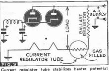
Current regulator tube stabilizes heater potentia when A.C. supply fluctuates.
