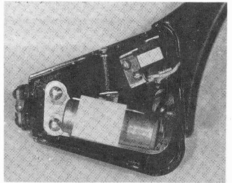
The Photoelectric Pickup. It is said to be 40% to 60% more sensitive than preceding types. The light from a high-intensity argon-filled filament-type exciter lamp fed by a radio-frequency current is reflected from a mirror, about ½-x ¾-in. high, and paper-thin to a selenium ''electric eye.''
