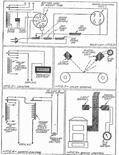
using the meter as for grading will register the relative density of the smoke passing through the chimney breach. LIGHTING CONTROL
