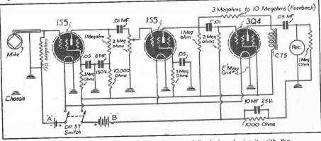
The ultra-small hearing aid tubes and a carefully-designed circuit with the application of inverse feedback are combined in a very effective instrument which compares well with commercial devices
