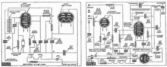
Schematic circuits of 2 of the Phono-Oscillators described in the accompanying article, and illustrated at top of page pictorially.
