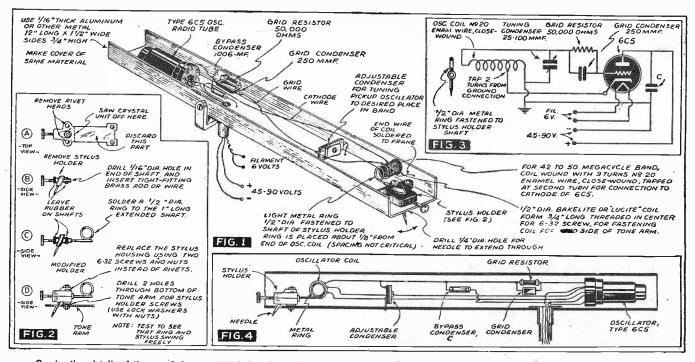
Construction details of the new Frequency Modulation Phono Pickup system. The circuit of the accompanying F.M. oscillator is given in Fig. 3.
