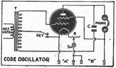
may be any available of about 30 ohms resistance and is used to drop, the "A" battery voltage to the required tube filament voltage. The "on and off" switch (Sw) may be on the rheostat or it may be separately mounted. In most cases the 'phones may be substituted by a P.M. speaker with a suitable speaker transformer. The key is placed as it is in the circuit to eliminate "key-clicks."
