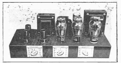
The amplifier at the left uses a double triode as inverter, to make an amplifier without a driver transformer. A second double triode is used to permit two inputs, low-gain for phonograph, and high-gain, from a pre-amplifier stage, for use with a low-level microphone. The combination makes for both simplicity and fidelity. The three controls are: Microphone, phonograph and tone.
