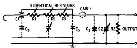
Fig. 806. Circuit diagram of the frequency-compensated probe.
