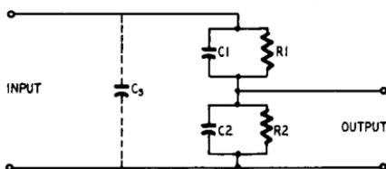
Fig. 805. *Electrical arrangement of the frequency-compensated probe.*
