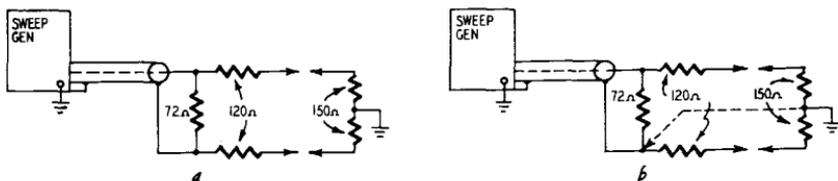
Fig. 418-a, b. These two illustrations show one technique that can be used for getting balanced output from a sweep generator. This method does not give a perfect impedance match.
