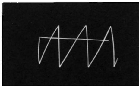
Fig. 515. Photo of current waveform in horizontal yoke.
