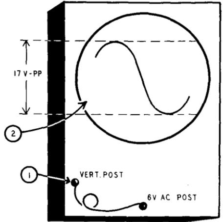
For example, with the vertical sensitivity switch set to  $\times 1$  position, adjust the vertical sensitivity control until a 17 volts peak-to-peak pattern occupies a total of 17 squares. Remove the jumper.
