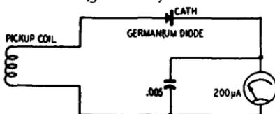
Fig. 812. R.f. detector probe circuit.
