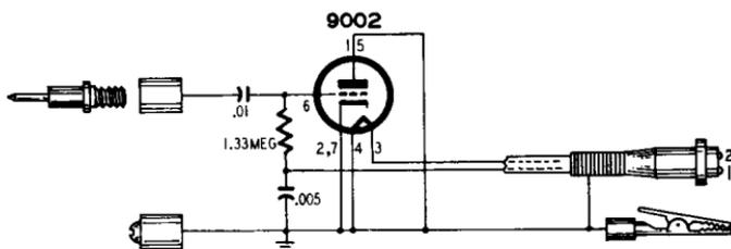
Fig. 1002. *Peak-indicating high-frequency probe (r.f. probe).
