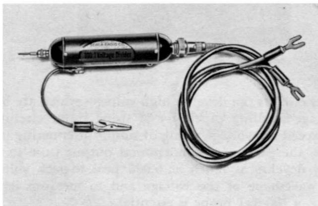
Fig. 601. Photo of a high-voltage, capacitance-divider probe.
