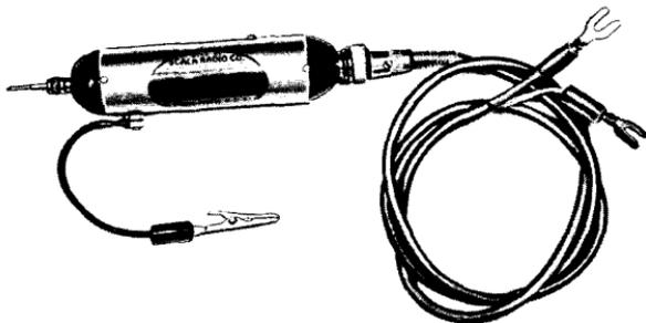
Fig. 501. A 10-to-1 low-capacitance signal-tracing probe.
