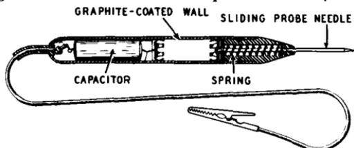
Fig. 804. *Cross-sectional view of capacitor-tester probe.*
