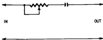
Fig. 803. Circuit diagram of capacitor-tester probe.
