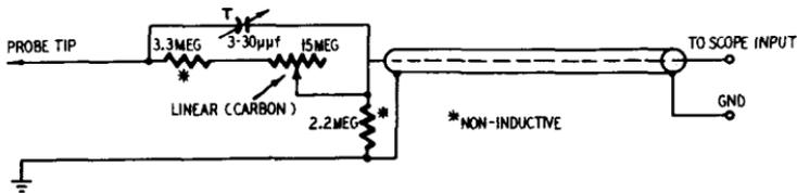
Fig. 503. Component values for a typical low-capacitance probe.
