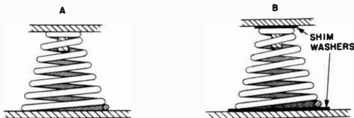
Fig. 509-a, b. If one or more corners of the chassis are not high enough (a) shim washers can be added (b).
