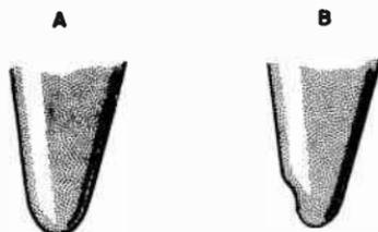
Fig. 522-a,-b. Good needle (a) and worn needle (b).
