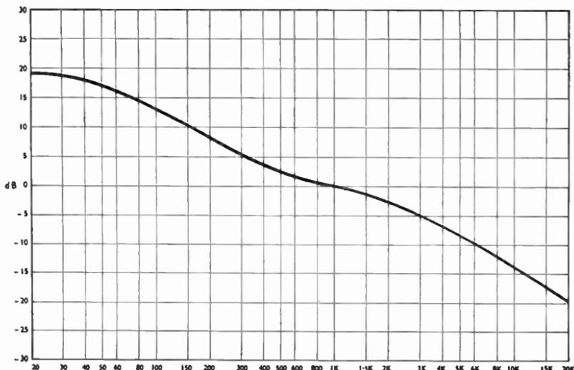
FIG. R/15. *Standard replay characteristic for microgroove records in U.S.A. and Great Britain (R.I.A.A. and B.S.S. 1928/1955).*
