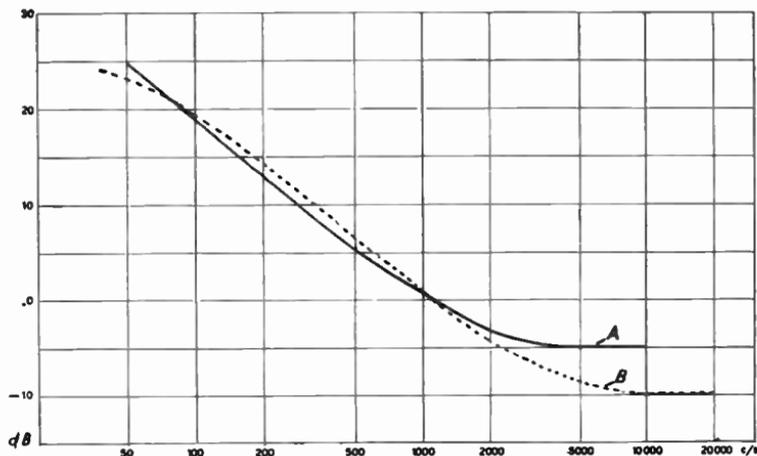
FIG. T/3. *Standard replay characteristics for 7½"/sec tapes*
