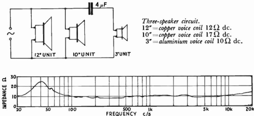
FIG. 1/2. Unusually level impedance curve achieved by parallel working.
