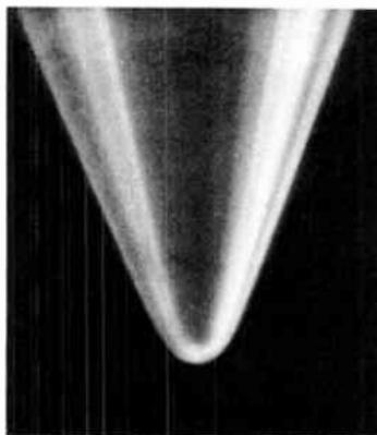
FIG. S/12. Typical  $\frac{1}{2}$  mil sapphire for stereo. Mag. 250x.
