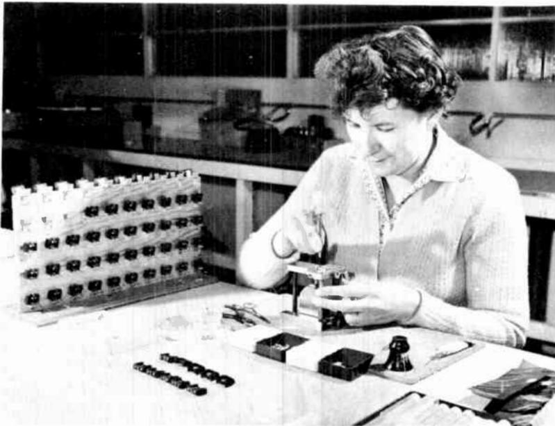
FIG. P/7. *Mounting armature in Decca pickup head.
