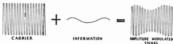
FIG. A/1. *Amplitude modulation.*
