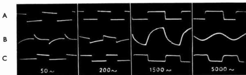
FIG. S/4A. Square waves at 50, 200, 1,500 and 5,000 *c/s*.
