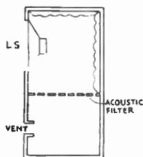
FIG. A/5. Reflex enclosure with Acoustic Filter. Ordinary saw-cuts  $1\frac{1}{2}$ " apart make suitable slits. Absorbent lining in upper section only.
