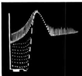
FIG. I/3. *Picture of combined effect of motor-boating and parasitic oscillation on steady tone at 1,500 c/s, showing severe intermodulation.*
