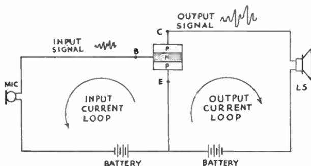
FIG. T/12. *The transistor as an amplifier.*
