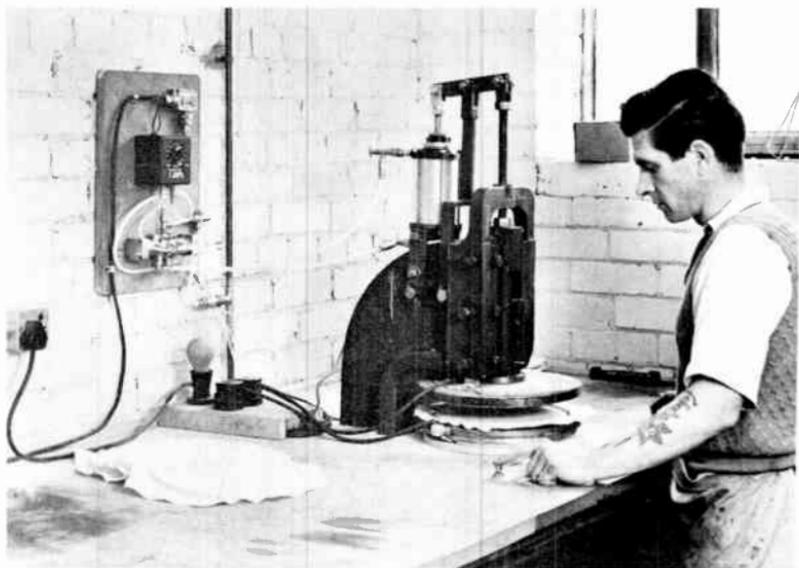
FIG. R/19B. *Pneumatically operated and timed moulding press.*
