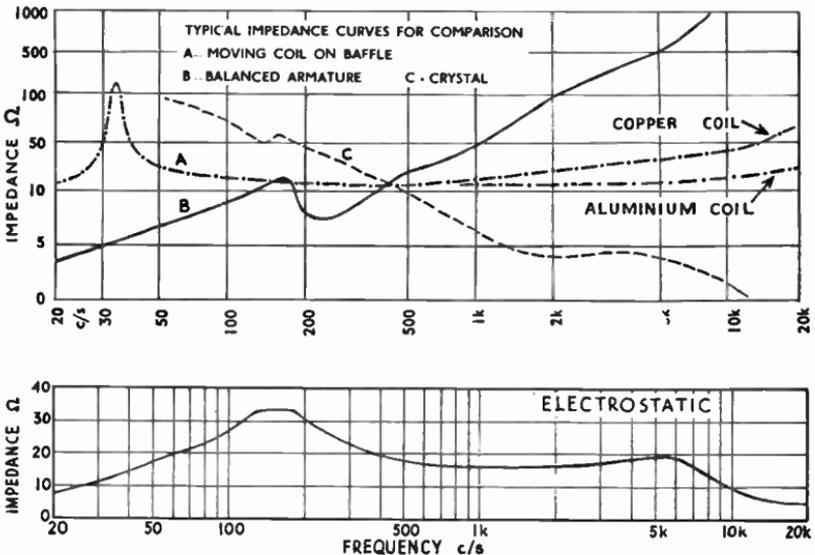
FIG. 1/1. Typical impedance curves.
