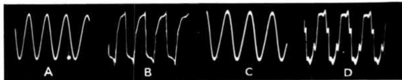
FIG. N/2. *Distortion caused by injudicious use of bass and treble lift in high-class amplifier.*
