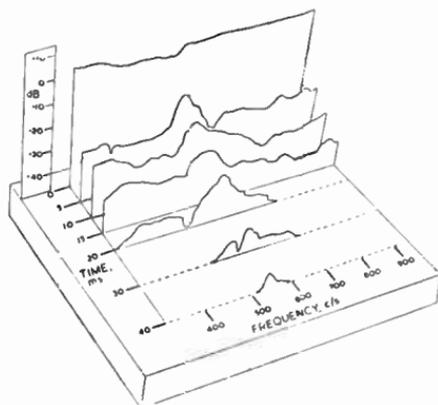
FIG. D/4. Interrupted tone test of loudspeaker. The rear portion represents the steady state response, and the others indicate different resonances which show up at intervals up to 40 milliseconds after termination of signal.
