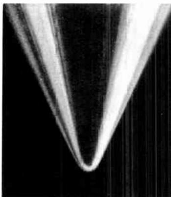
**STYLUS-HOT** When cutting microgroove and stereo discs it is now universal practice to use a stylus tip which is heated to a temperature of approximately  $100^{\circ}\text{C}$  by means of a small electric heating coil surrounding the shank.
