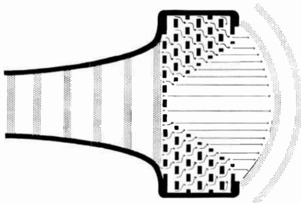
FIG. D/7. Sectional diagram of acoustic lens with perforated plates showing time-lag and wider dispersion.
