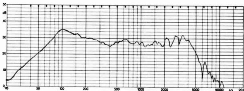
FIG. L/7. Axial response of 1930 model. Bass resonance 90 c/s.
