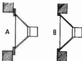
FIG. C/1A. To avoid cavity resonance use arrangement B.
