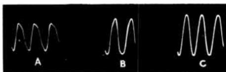
FIG. N/1. *Non-linearity at A and B at 40 c/s with 1 watt input to 10" unit.*
