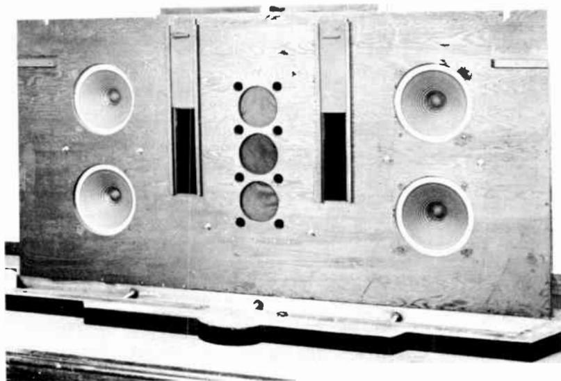
FIG. O/1. Loudspeaker system for electronic organ.
