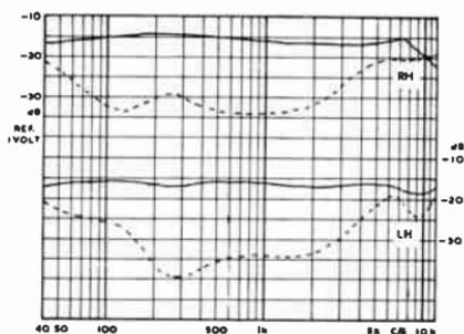
FIG. C/2. *Typical response curves and separation between channels of crystal pickup.*
