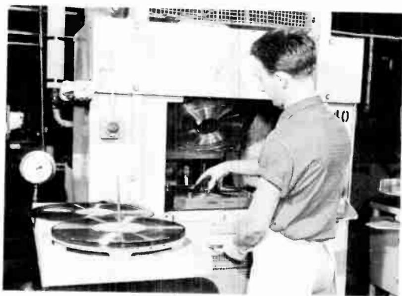
FIG. R/13. *Pressing the final record.*
