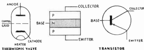
FIG. T/11. *Valve and Transistor symbols.*
