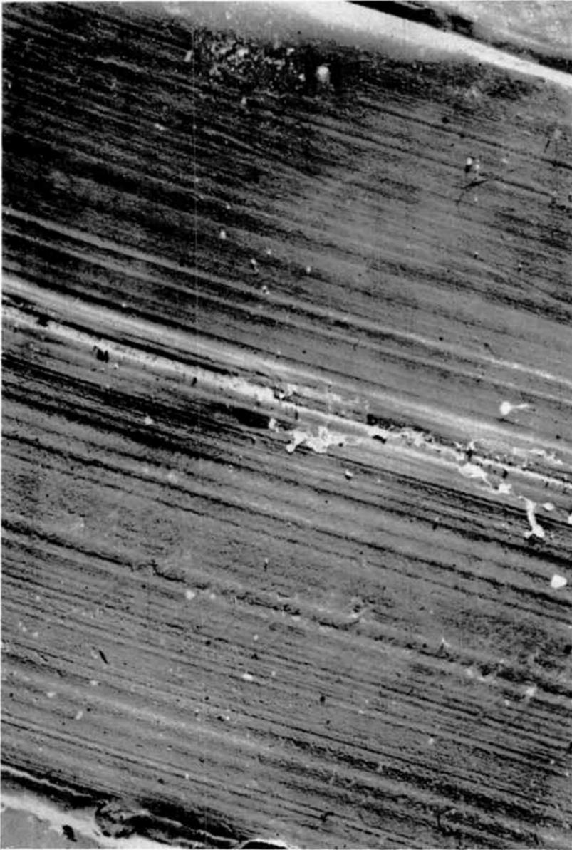
FIG. E/6A. *Part of unplayed microgroove as revealed by Electron Microscope.
