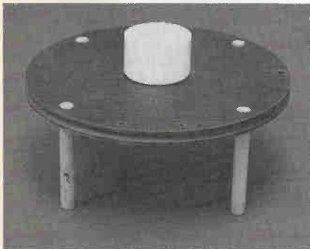
Shown here is the 9-inch circular deck supported by four dowel rods, and an end cap positioned at its center.
