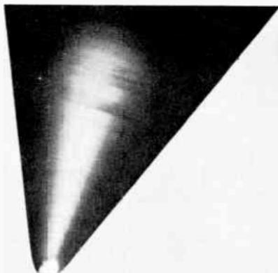
FIG. 18 (b).—EXCESSIVELY WORN STYLUS
