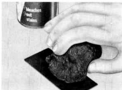
Fig. 705. *Cleaning a copper-clad phenolic board.*
