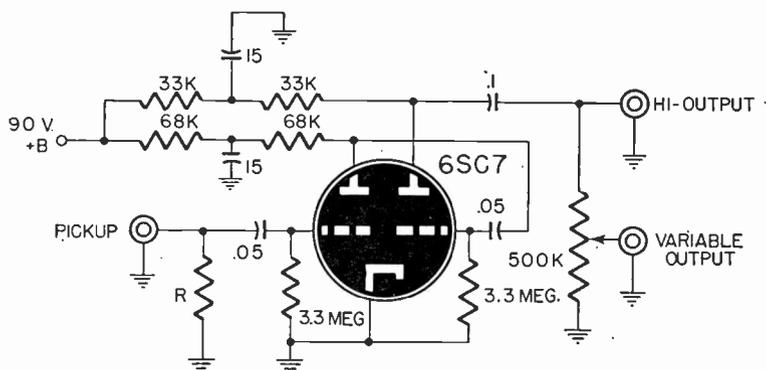
Fig. 1306—Typical unequalized preamplifier for low-level magnetic pickup.
