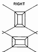
Fig. 1204—Right and wrong ways to place two ribbon microphones for best pick-up.
