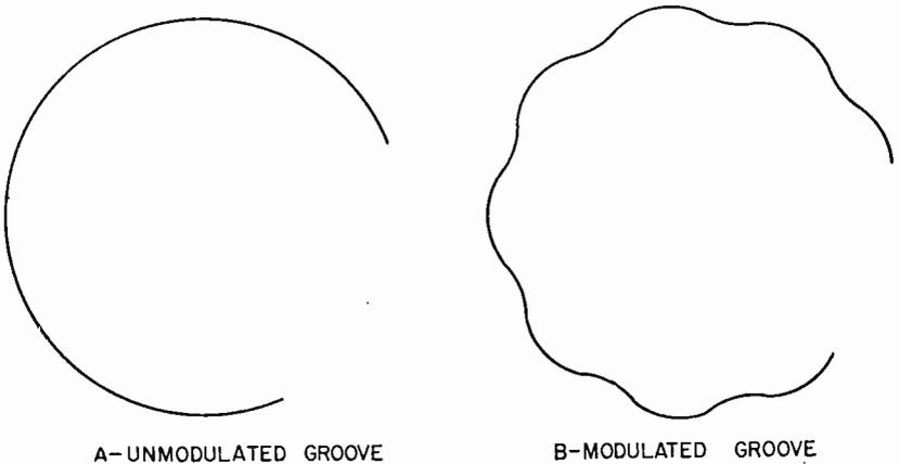
Fig. 101—*a*—Grooves without signal recorded; *b*—with signal recorded.
