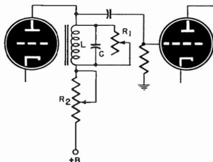
Fig. 1114—A resonant equalizer circuit.
