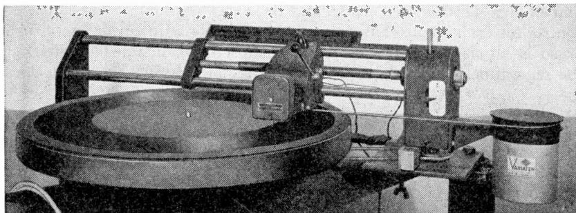
Fig. 1111—One type of automatic diameter equalizer mounted on overhead lathe. The cutter pulls the string which regulates the equalizer setting.
