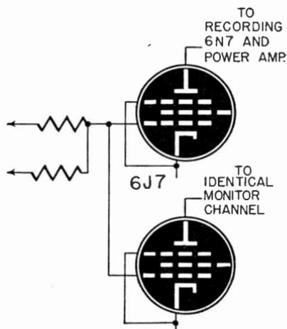
Fig. 902—Coupling monitoring stage for recording amplifier.
