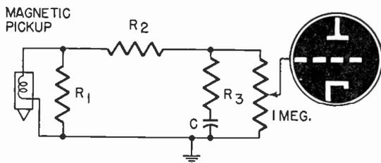
Fig. 1305—Bass booster for magnetic pickups.
