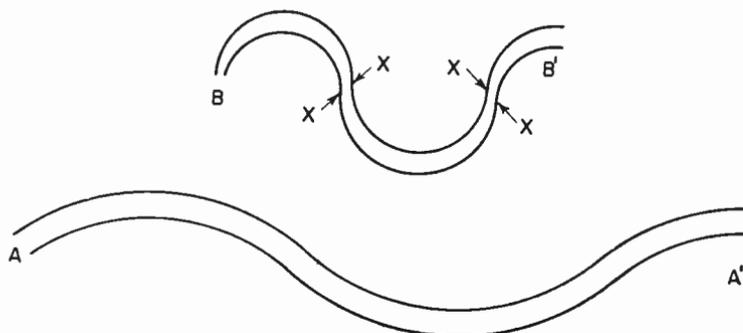
Fig. 1109—Grooves of same frequency at different disc diameters; note pinching of groove at points X-X.
