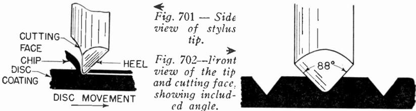
is the same as the stylus cutting face; and second, that the entire cutting face is not used. Fig. 702 shows that as the stylus cuts a deeper groove it cuts a wider groove. This bears directly on the matter of cutting pitch or number of lines per inch.
