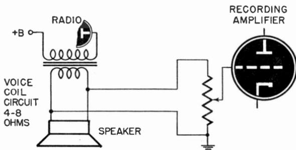
Fig. 1207—One method of coupling radio receiver to recording amplifier.
