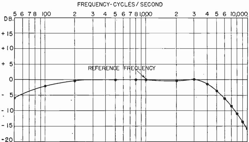
Fig. 1102—Typical response curve of a poor amplifier.
