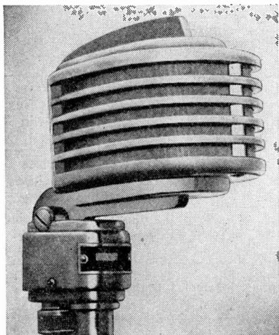
Fig. 802—Typical diaphragm type crystal microphone.
