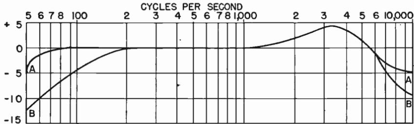
Fig. 1104—Output of standard frequency record (curve A) and output of recorded test disc (curve B).
