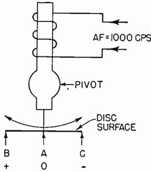
Fig. 602-b—Stylus moves back and forth, through point A, following voltage changes of Fig. 602-a.
