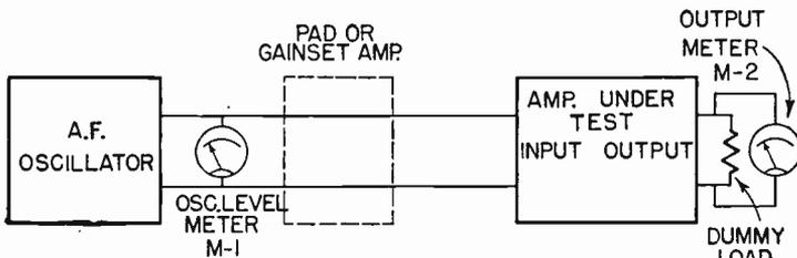
Fig. 1101—Frequency run setup. Oscillator output should not be high enough to overload the initial amplifier stages, but sufficient to give a reading on meter M-1.
