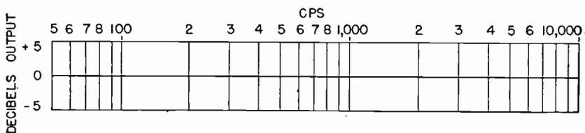
Fig. 608—Perfect crystal cutter response. This is NOT a comparison with the standard C-V curve.
