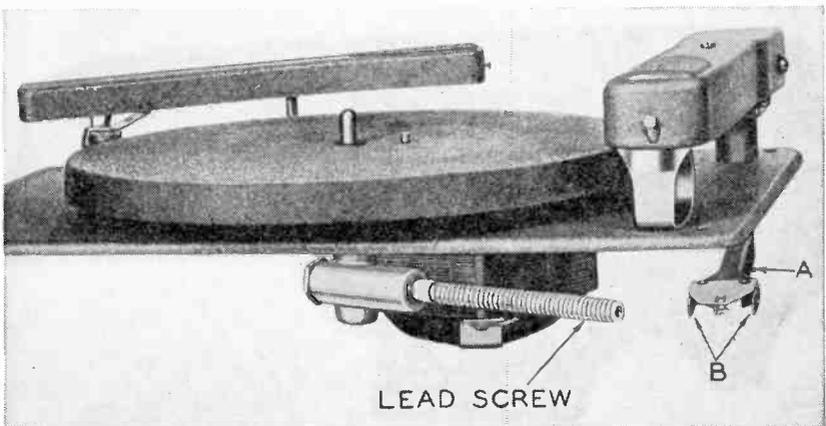
Fig. 403—A swinging-arm recording chassis
