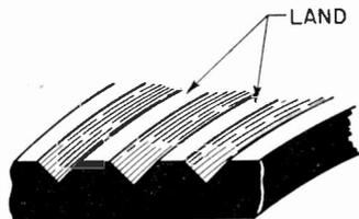
Fig. 703 — Several adjacent grooves, showing "land" between grooves.
