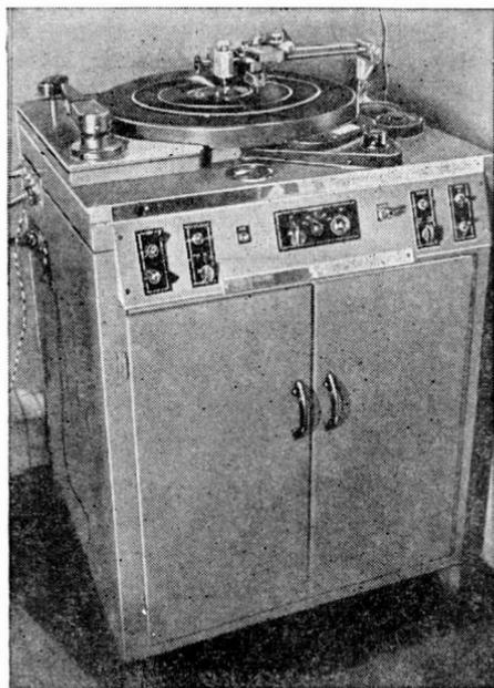
*Fig. 905—A fairly elaborate homemade recording and playback console used in a small professional recording studio.*
