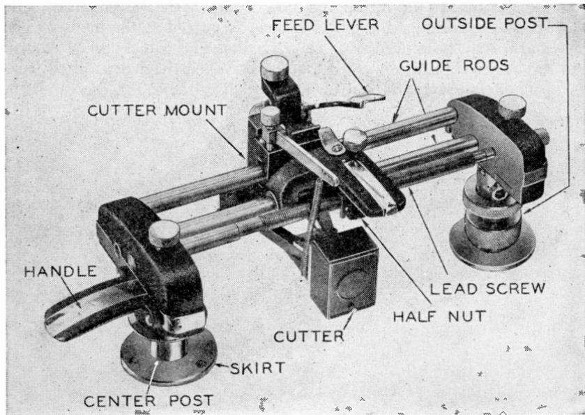
Fig. 405—An overhead lathe mechanism.
