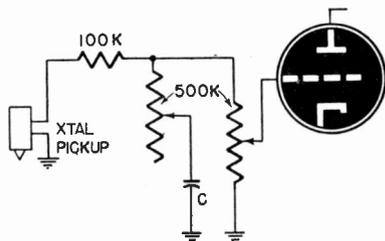
Fig. 1304—Basic high-attenuator for crystal pickups.
