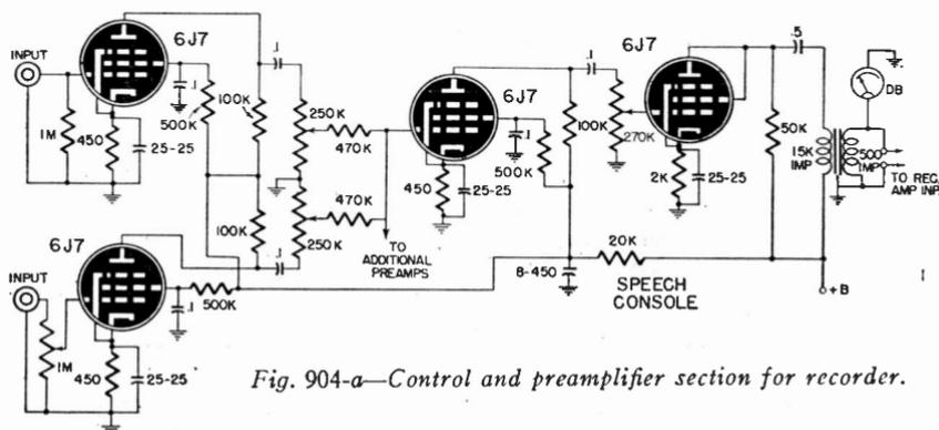
Fig. 904-a—Control and preamplifier section for recorder.
