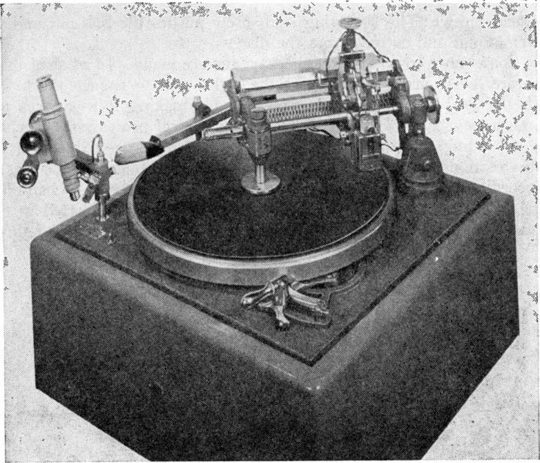
Fig. 406—A fairly elaborate overhead lathe recording table.
