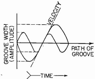
width at one octave above that frequency is 2 to 1. We can evaluate the groove widths in terms of voltage. A voltage ratio of 2 to 1 is equal to a decibel gain or loss of 6. We can now be exact when speaking
