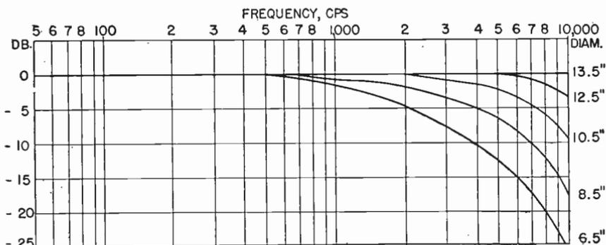
Fig. 1110—Approximate attenuation in playback due to "pinch effect" at various diameters.
