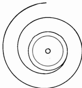
Fig. 1206—Appearance of lock groove at center of disc.
