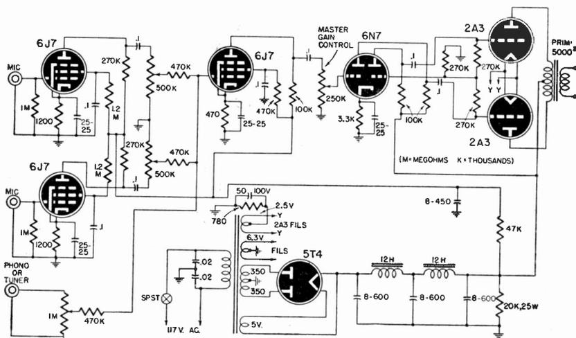
Fig. 901—Schematic diagram of a recording amplifier.
