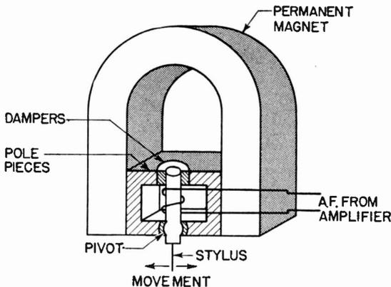
Fig. 501—Simplified sectional view of magnetic cutting head.
