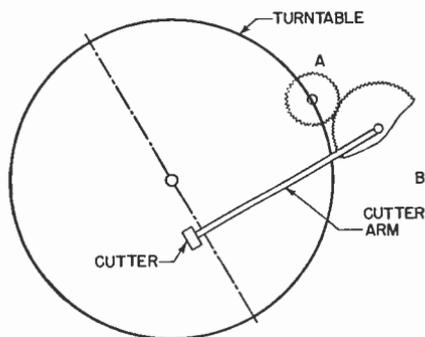
Fig. 404—Swinging-arm feed; Gear A driven by motor or turntable; gear B, on cutter arm, meshes with A, causing the arm to swing.
