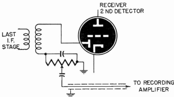
Fig. 1208—Another radio connection, which bypasses receiver audio system.
