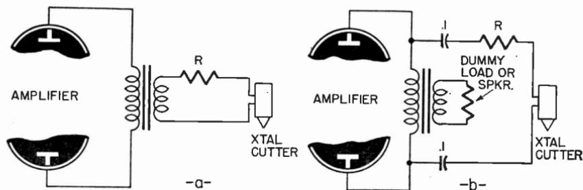
Fig. 1107—Crystal cutter connections for modified constant-velocity recording.
