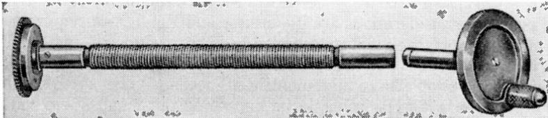
Fig. 401—Lead screw, with spiraling crank.
