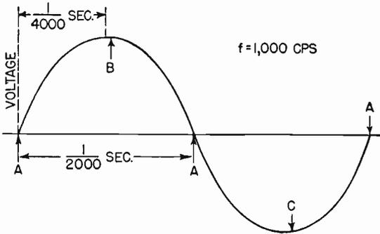
Fig. 602-a—A 1,000-cycle sine wave, showing time relations for  $\frac{1}{4}$  and  $\frac{1}{2}$  cycle.
