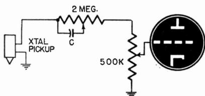
Fig. 1303—Basic high-booster for crystal pickups.
