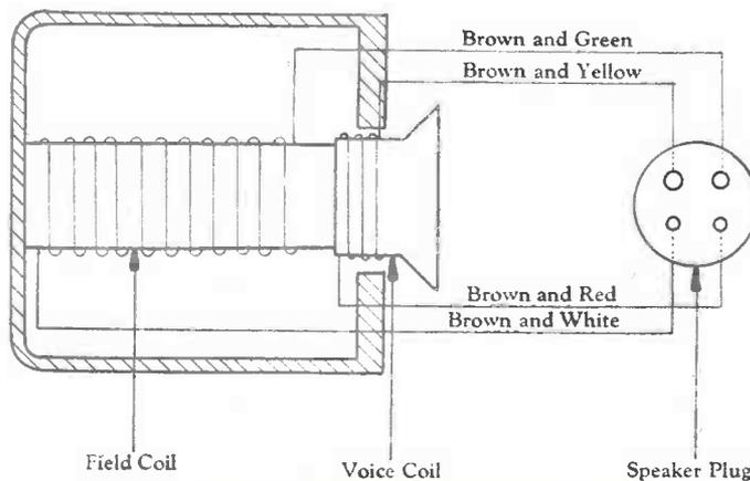
Fig. 6. Circuit of Dynamic Reproducer
