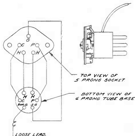
SKETCH OF CONNECTIONS FOR ADAPTER TO PLUG INTO SET.
