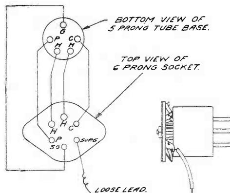
SKETCH OF CONNECTIONS FOR ADAPTER TO PLUG INTO ANALYZER.
