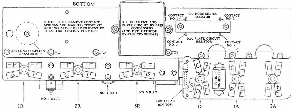
FIG. 113. TEST CHART FOR MODEL 43, 46 AND 53. Model 47 chart is similar except that it has four separate R. F. sockets.
