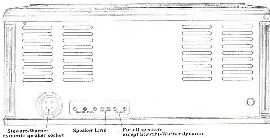
Fig. 2—Rear View, Showing Terminal Layout
