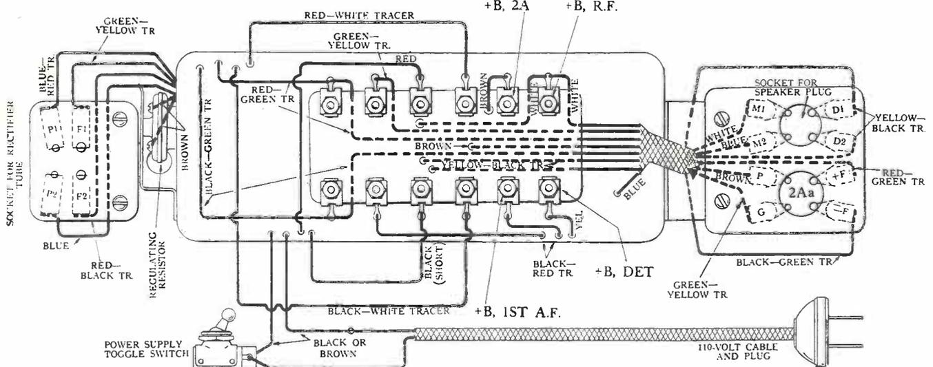
FIG. 114. SHOWING CONNECTIONS AND APPROXIMATE POSITION OF LEADS FROM SEALED CONTAINER IN MODEL 43 POWER UNIT. In early type of power unit for Model 43, two brown leads from the primary-shunt condenser connect to the +B, 2A terminal and to the brown P2Aa lead respectively. In later models these connections are made internally.
