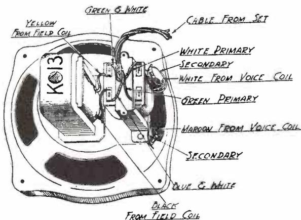
Fig. 1—Single Speaker Connections—121 Code.
