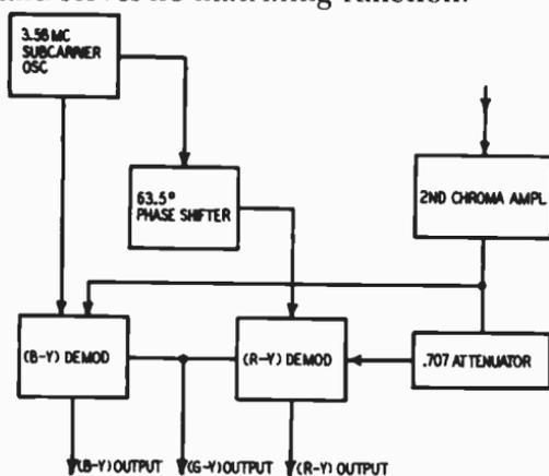
Fig. 504. Arrangement of the (R - Y) (B - Y) demodulation system to accomplish simultaneous (G - Y) matrixing.
