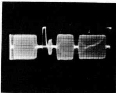
Applied color signal; this output from the color bar generator consists of horizontal sync, burst, I and Q voltages. It is very useful in determining whether the color subcarrier is being applied in exact quadrature and whether the color subcarrier is being applied with I at  $57^\circ$  from burst.
