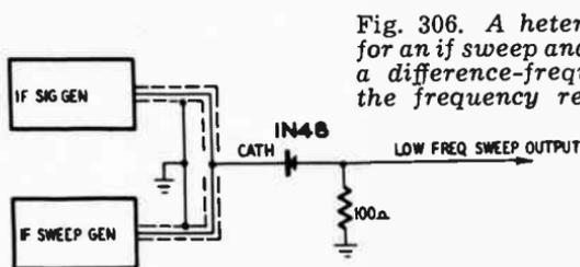
Fig. 306. A heterodyne output arrangement for an if sweep and signal generator to provide a difference-frequency output for checking the frequency response of video-frequency circuits.
