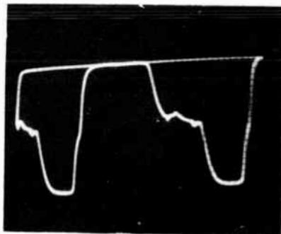
Output from Q detector; again, considerable contamination of Q output with I output. The Q bar is the longer of the two downward excursions. Contamination is caused by misadjustment of the color phasing control.
