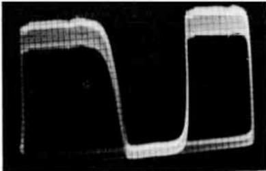
If the output from the I detector appears as shown here, with strong interference from the Q signal, the color subcarrier is not arriving at the I detector in required quadrature relation. Check the  $90^\circ$  phase-shifting network in the output circuit of the color subcarrier oscillator.
