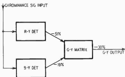
The (G - Y) matrix operates by mixing  $-0.51$  (R - Y) with  $-0.19$  (B - Y) to form (G - Y). Thus, positive output from the (R - Y) or (B - Y) detectors results in negative output from the (G - Y) matrix, or negative output from the (R - Y) and (B - Y) detectors results in positive output from the (G - Y) matrix. Negative output from a detector or matrix results in less beam current from the associated electron gun, while positive output results in increased beam current.
