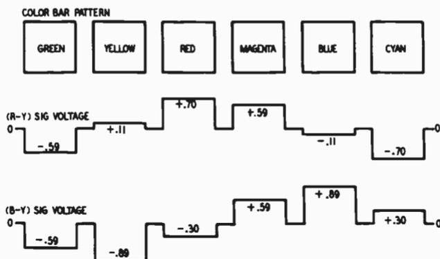
Fig. 422. Relative signal levels when the (B - Y) gain control is set correctly.
