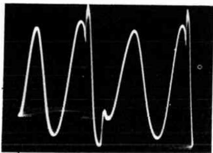
Fig. 809. Boost pulse at bandpass amplifier appears in demodulator output.
