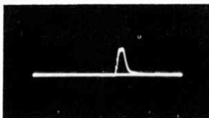
Fig. 330. Small distorted feedthrough obtained when attempting to sweep the Y and Q channels through the chroma bandpass amplifier with a 0-2-mc sweep signal. Since the passbands of the two circuits are staggered, a sweep test cannot be obtained by conventional sweep checks. (A) Feedthrough, I channel, from chroma amplifier. (B) Feedthrough, Q channel, from chroma amplifier.
