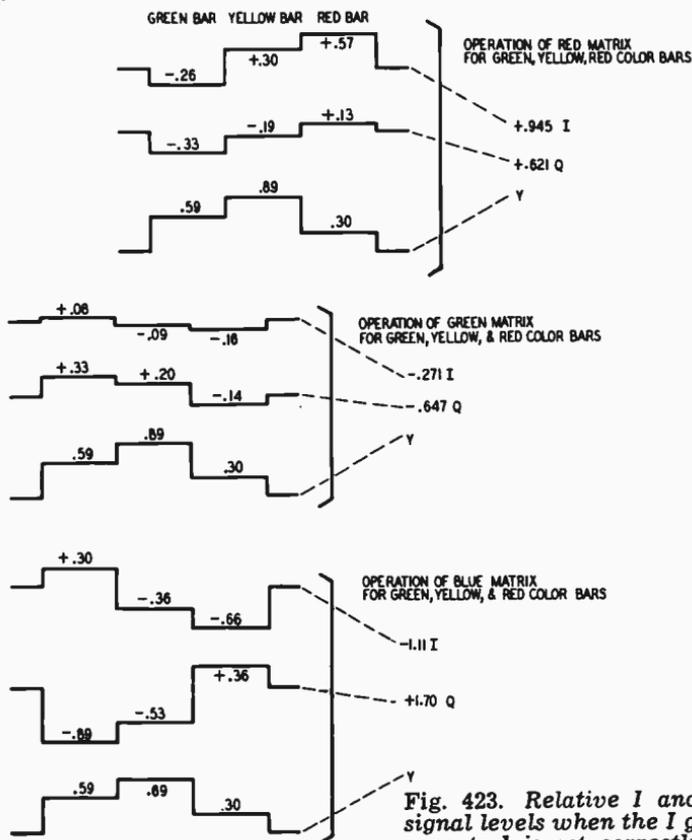
Fig. 423. Relative  $I$  and  $Q$  signal levels when the  $I$  gain control is set correctly.
