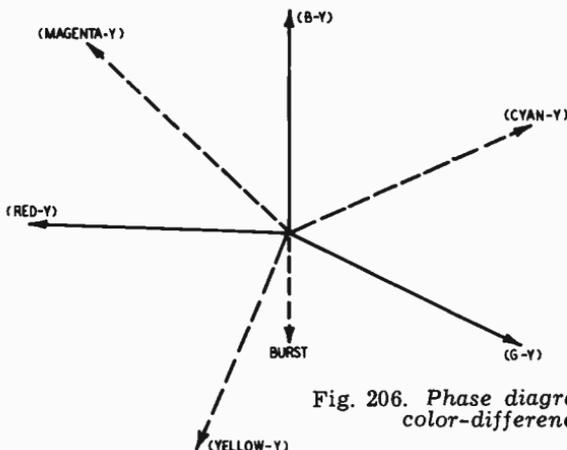
Fig. 206. Phase diagram of the chief color-difference signals.
