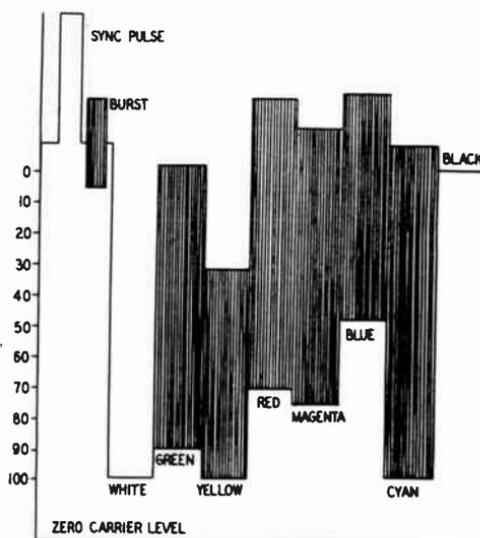
Fig. 611. The color signal places a greater demand on the dynamic range of the if amplifier than a black-and-white signal because the 3.58-component extends into the blacker-than-black region.
