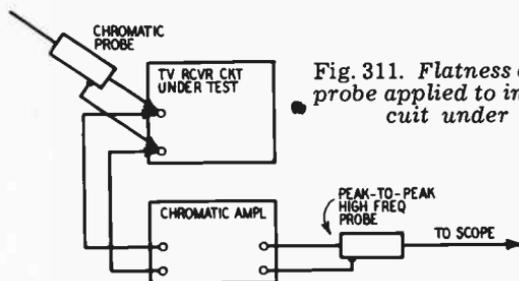
Fig. 311. Flatness check with probe applied to input of circuit under test.
