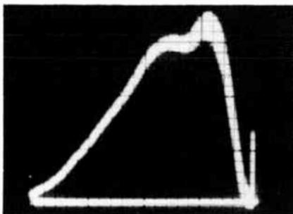
still remains the interleaved monochrome signal in this band from 2.1 to 4.2 mc. The output from the chroma bandpass amplifier accordingly consists principally of the mixed I and Q signal voltages.
