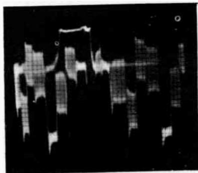
Sync circuits can be checked, if desired, with a horizontal sync pulse and burst signal, in the absence of any chrominance or luminance information. This photo shows the output from a color bar generator with only sync pulse and burst present.
