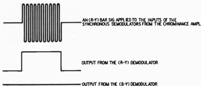
Fig. 417. Application of a wide-band scope at the (R - Y) detector output should indicate that an (R - Y) test signal produces maximum envelope output but that a (B - Y) signal produces zero output.
