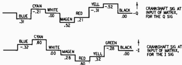
Fig. 419. A typical pair of cranks shaft patterns obtained at the outputs of I and Q demodulators when a color bar signal is applied to the receiver.
