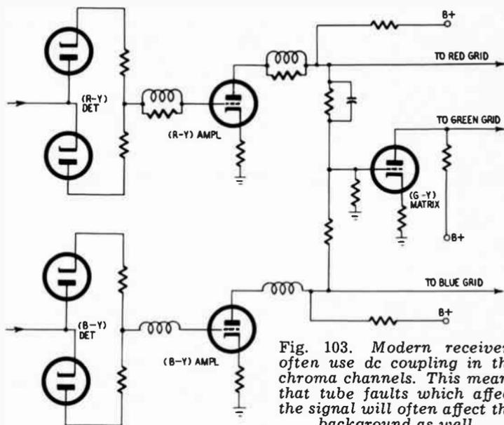
Fig. 103. Modern receivers often use dc coupling in the chroma channels. This means that tube faults which affect the signal will often affect the background as well.
