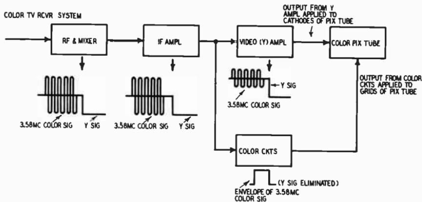
Fig. 604. Progress of the complete color signal through a color TV receiver.
