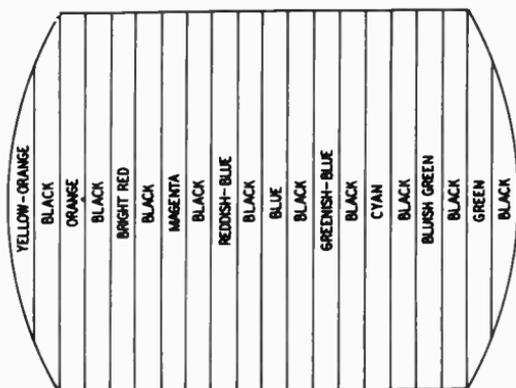
Fig. 117. In a keyed rainbow generator, the spectrum is broken up into stripes by black bars.
