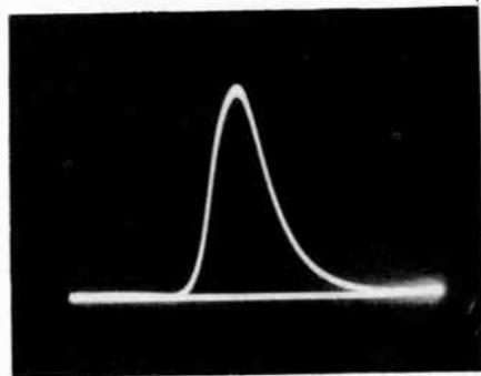
reference waveform drops to a small fraction of its former value (Fig. 813) and we conclude that, although the test with the signal-tracing probe suffices to show whether the signal is present or absent at this point, the test does *not* serve to show the stage gain.
