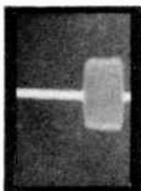
This is the appearance of an (R - Y) signal, as seen on the screen of a wide-band scope. A (B - Y) or a (G - Y) signal appears the same because it is only the phase of the chrominance signal which is varied to cause the matrix to develop various color signal voltages.
