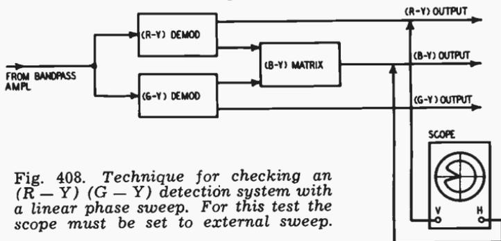
Fig. 408. Technique for checking an  $(R - Y)$   $(G - Y)$  detection system with a linear phase sweep. For this test the scope must be set to external sweep.
