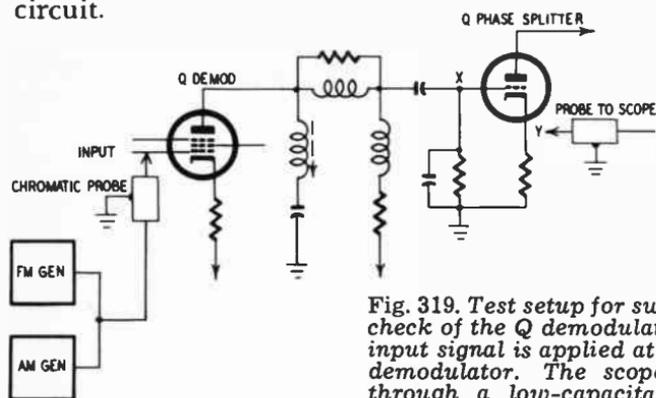
Fig. 319. Test setup for sweep-frequency check of the Q demodulator. The sweep input signal is applied at the grid of the demodulator. The scope is connected through a low-capacitance probe for low-frequency tests, or through a peak-to-peak demodulator probe for high-frequency checks. It is essential to apply the scope probe at point Y in the circuit and not at point X.
