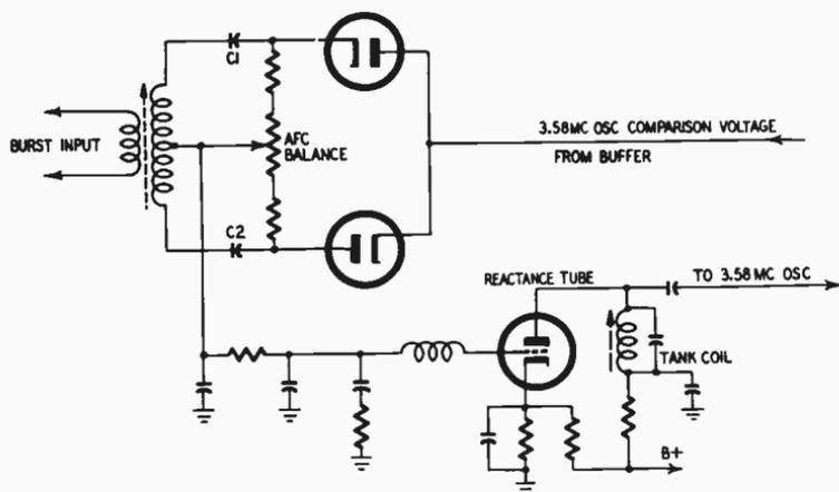
Fig. 217. Defects in the color afc phase detector and in the reactance-tube circuit can cause failure of the 3.58-mc oscillator. Sometimes a defective buffer stage is also responsible.
