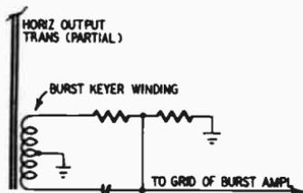
The gating pulse arrives too late, in some cases, due to changed values of resistors in the pulse-delay network, to faulty capacitors (Fig. 221) or, in some receivers, to "pulling" in the horizontal oscillator. The remedy is to check the waveforms in the horizontal oscillator circuit with a scope and low-capacitance probe. The slugs in the tuned coils should be adjusted to provide the waveforms specified in the service manual.
