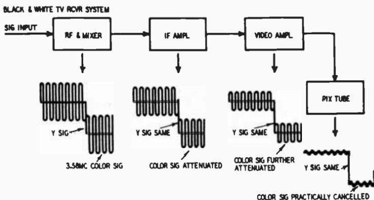
Fig. 603. Progress of the complete color signal through a black-and-white receiver.
