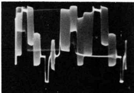
In adjusting bar widths, the controls may be set on the basis of a pattern observed on the screen of the color picture tube. (See photos 6 and 7).
