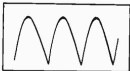
Fig. 712. Typical parabolic voltage across the convergence coil. (Courtesy of Motorola, Inc.)
