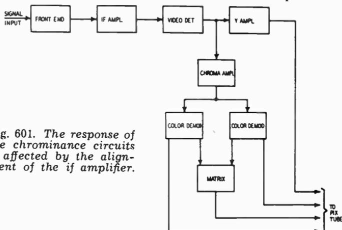
Fig. 601. The response of the chrominance circuits is affected by the alignment of the if amplifier.
