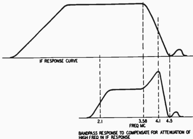
Fig. 610. Bandpass response compensates here only for the high-frequency if attenuation. Single-sideband compensation is subsequently provided in the I demodulator response.
