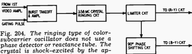
Fig. 204. The ringing type of color-subcarrier oscillator does not use a phase detector or reactance tube. The crystal is shock-excited by the applied burst voltage.
