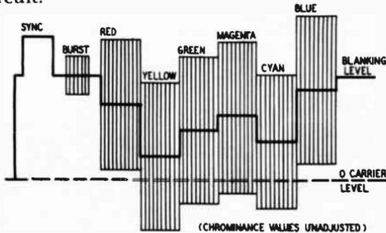
Fig. 803. Color signal corresponding to 100%-saturated color bars.
