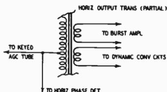
Fig. 701. Typical branch circuits which may load the horizontal-output transformer.
