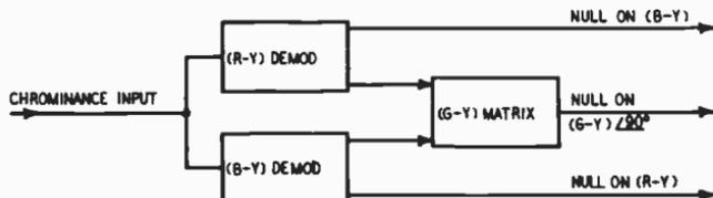
Fig. 418. Illustration shows the null checks that can be made on the three color difference signals.
