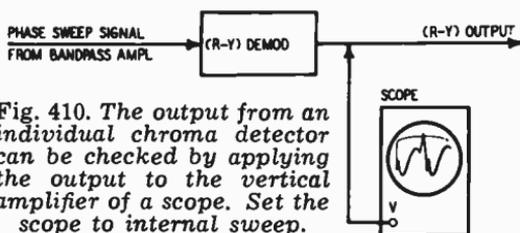
Fig. 410. The output from an individual chroma detector can be checked by applying the output to the vertical amplifier of a scope. Set the scope to internal sweep.
