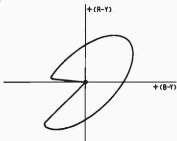
Fig. 406. Misadjustment of quadrature transformer produces elliptical pattern.
