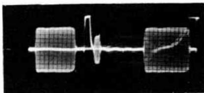
lators will display a crankshaft pattern (Fig. 419). The various levels of the crankshaft waveform indicate the values of chrominance voltage passed by the detector under test for each of the applied
