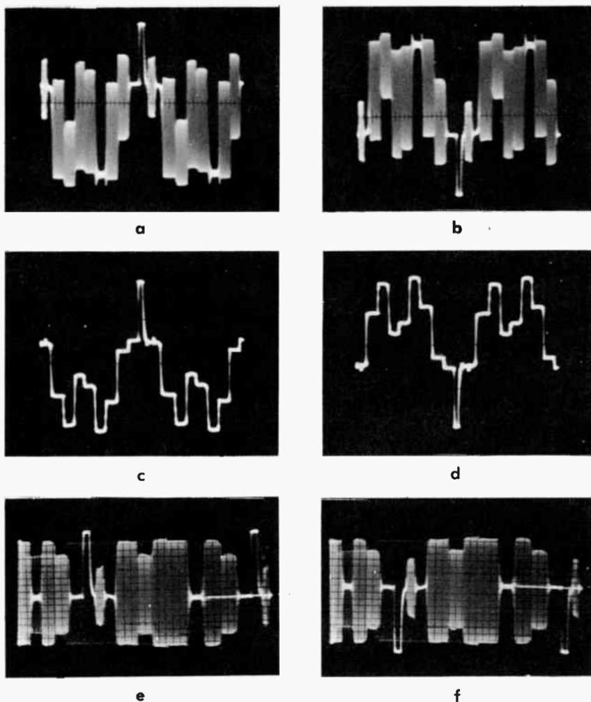
Fig. 211 (a to f). Typical video-frequency outputs from an NTSC color-bar generator.
