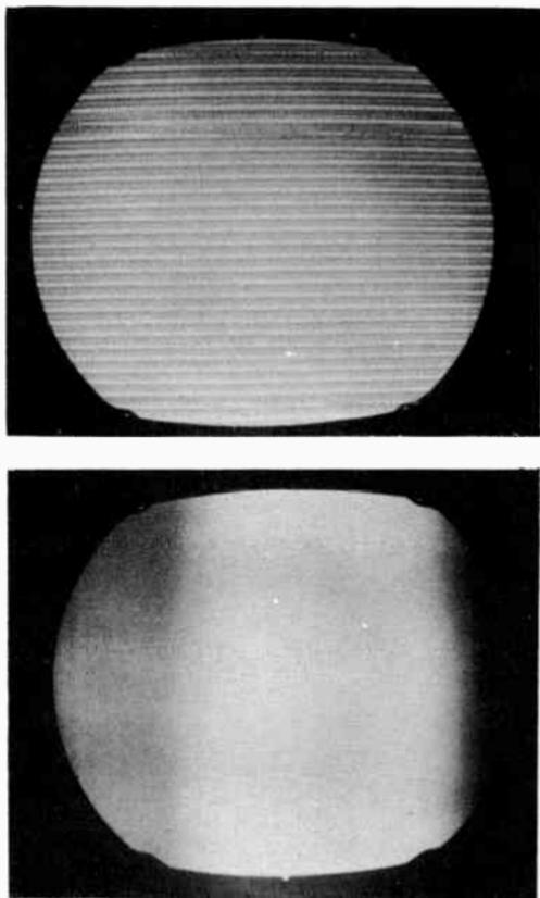
Fig. 220. Color subcarrier oscillator operating off frequency. (Above) Oscillator off frequency by 1,800 cycles. (Below) Oscillator off frequency by 15,750 cycles
