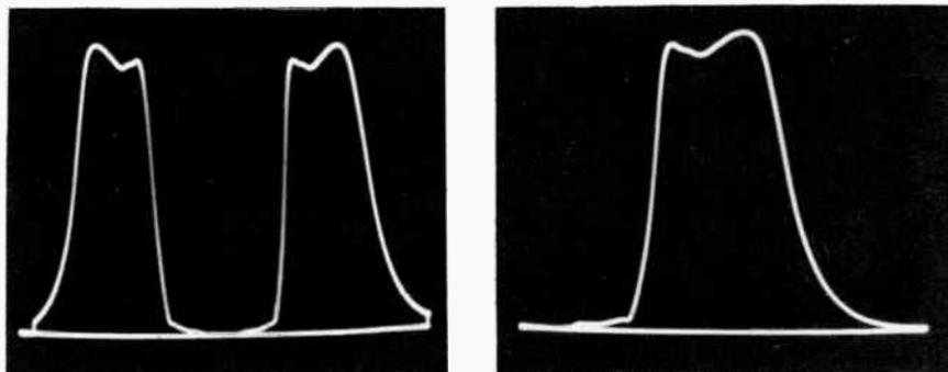
Fig. 334. (A) When the sweep generator is tuned with zero frequency appearing in the center of the display, there is considerable blank space between the twin responses from the chroma bandpass amplifier since the circuits cut off below 2.1 mc. (B) To obtain the standard form of curve, the zero-frequency point is tuned to the left-hand end of the base line.
