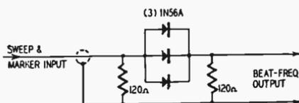
a marker generator is mixed with the swept signal. The signals are applied to the input of the Chromatic Probe. The probe modulates these signals and generates an upper and a lower sideband. The lower sideband sweeps from (nominally) 0 to 5 mc and is the signal that interests the color-TV technician. It is the signal output used to sweep-check the Y amplifier, I, Q, chroma amplifier and chrominance circuits.
