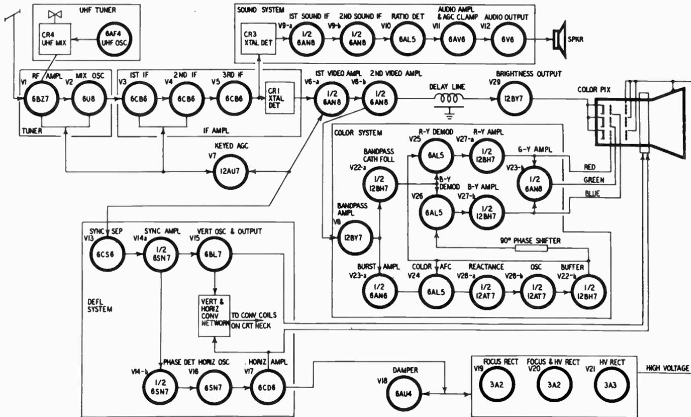
Fig. 101. Block diagram showing the various sections of a color TV receiver. (Courtesy of Motorola, Inc.)
