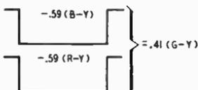
To obtain a saturated green hue on the screen of the color picture tube, the chrominance signal consists of  $-0.59$  (R - Y) and  $-0.59$  (B - Y), from which the green matrix forms  $+0.41$  (G - Y). With a Y signal of  $+0.59$ , the green gun runs "wide open" while the red and blue guns are cut off.
