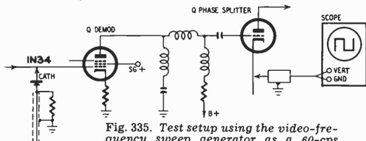
Fig. 335. Test setup using the video-frequency sweep generator as a 60-cps square-wave generator. The scope is connected at the cathode of the phase splitter through a low-capacitance probe, or the scope can be applied directly at this point. The sweep generator is set to some if frequency with a sweep width of 0.1 mc or less.
