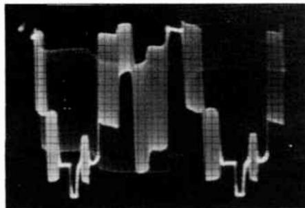
Effect on pattern of adjusting the overall Y gain control.
