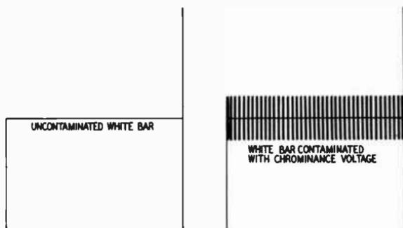
Fig. 342. Result of unbalance of primary signal voltages.
