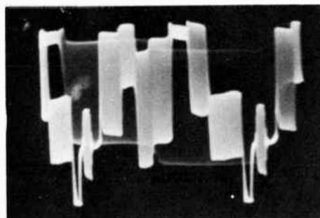
In the better color bar generators, the phase of the primary colors is set accurately with precision delay lines. The amplitude of the subcarrier for each primary color is set by three service controls: green, red and blue bar saturation. To produce white, the three primaries are added. (See photos 15, 16 and 17).
