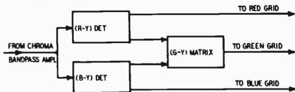
Fig. 102. A common (R - Y) (B - Y) (G - Y) arrangement.
