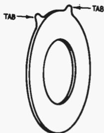
imum strength of field which provides good purity. The rings can also be rotated as a pair. This is another of the essential features of the purity adjustment.
