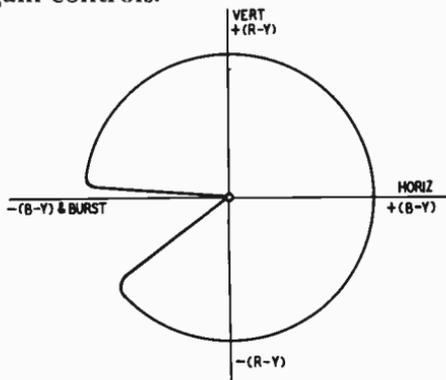
Fig. 404. The "pie cut" appears for the duration of the horizontal blanking interval. The illustration shows the proper relation of the cut to the horizontal base line for an  $(R - Y)$   $(B - Y)$  detection system.
