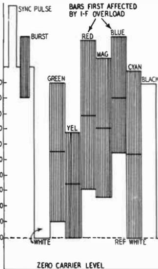
Fig. 341. Overload in if amplifier first distorts bar signals extending into black region.
