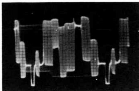
These photos (39, 40 and 41) show the effect on the pattern of adjusting the overall Y gain control.
