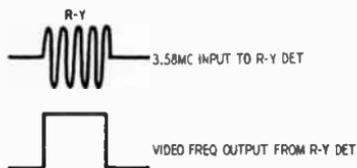
The input signal voltage to the matrix system has a frequency of 3.58 mc, but the output voltage from the (R - Y) and (B - Y) detectors has a square-wave shape, as shown. The output from the detectors has the shape of the envelope of the 3.58 mc signal. The square-wave signal voltages are applied to the input of the (G - Y) matrix.
