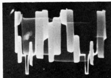
If the phase and amplitude of each of the primaries are correct, the subcarrier of the white bar will disappear. Since the phase is accurately and permanently set (for the example cited) with delay lines, the only other variables are the saturation controls. Hence, to set the amplitude of each of the primary color bars accurately, the technician needs only to vary simultaneously the three color-bar saturation controls and to cancel the subcarrier on the white bar.
