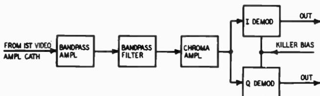
demodulators but the burst amplifier derives its signal prior to the bandpass amplifier. Thus, in Fig. 210, a fault in the bandpass amplifier does not affect operation of the color sync circuits but will affect color reproduction. In Fig. 209, a fault in the bandpass
