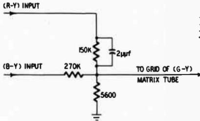
Fig. 420. Typical R-C network for matrixing the  $(R - Y)$  and  $(B - Y)$  signals to form the  $(G - Y)$  signal. (Courtesy of Motorola, Inc.).
