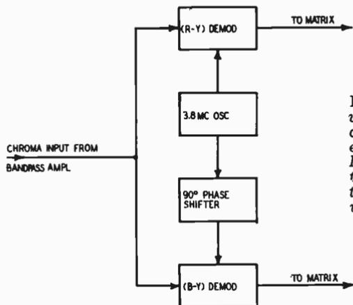
Fig. 405. The subcarrier voltages to the two chroma demodulators should be exactly  $90^\circ$  out of phase. If the phase is more or less than this, a circular pattern cannot be obtained with a linear phase sweep.
