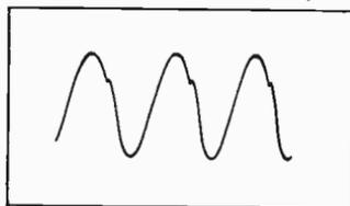
Fig. 710. *Horizontal convergence waveform at coil plug.*
