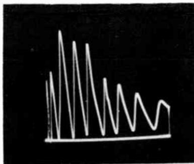
Fig. 304. *Very severe ringing of the Y amplifier caused by a short in the delay-line branch.*
