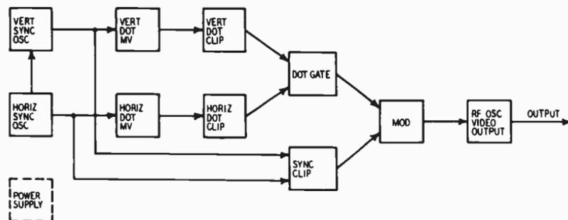
Fig. 901. Block diagram of a white dot generator. (Courtesy of Simpson Electric Co.).
