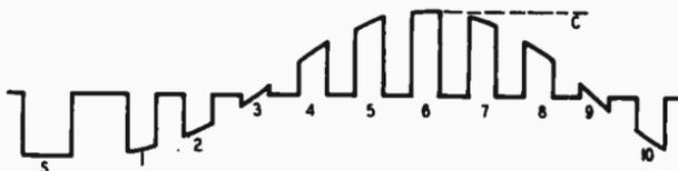
Fig. 507. How to check the ratio of luminance to chrominance voltages, using a rainbow generator. When the p-p voltage of the chrominance output from the generator is set equal to the p-p voltage of the sync pulse, the scope may be applied to the blue grid of the picture tube. The amplitude of the blue (6th) bar (see dotted line marked C) should then equal the amplitude of the horizontal sync pulse.
