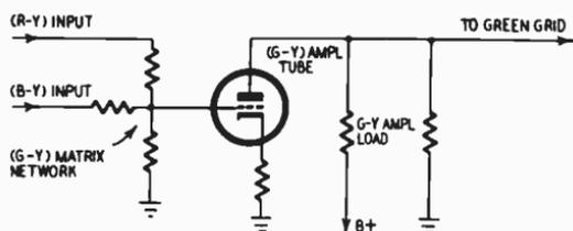
Fig. 503. The (G - Y) matrix network is in the grid circuit of the (G - Y) amplifier. The gain of the amplifier is controlled by values of cathode and plate load resistors.
