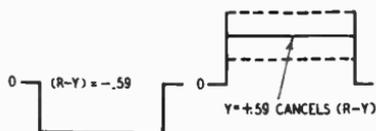
It is apparent that the green gun can operate at 100% output and the red and blue guns can be cut off to produce the saturated green hue only if the Y voltage is correct. If the Y voltage is greater than 0.59, the green hue will be contaminated with red and blue. If the Y voltage is less than 0.59, the green hue will be dimmed, with the green gun producing less than 100% output.
