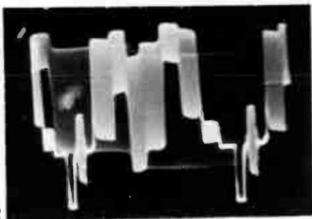
Another photo showing the result of varying the blue bar saturation control.
