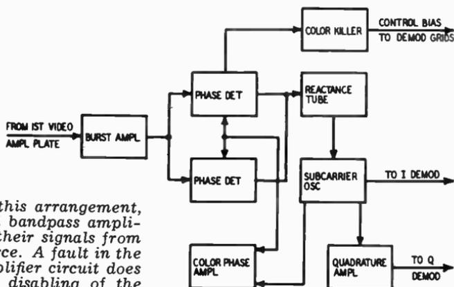
Fig. 210. In this arrangement, the burst and bandpass amplifiers receive their signals from the same source. A fault in the bandpass amplifier circuit does not result in disabling of the color-sync system, as is the case in the arrangement shown in Fig. 209.
