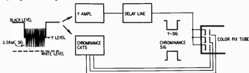
Fig. 337. The operation of the delay line is checked by the signal. The crankshaft signal passes through the Y amplifier and the chrominance signal through the chrominance circuits. If the delay is correct, the edges of color bars and black bars will meet exactly.
