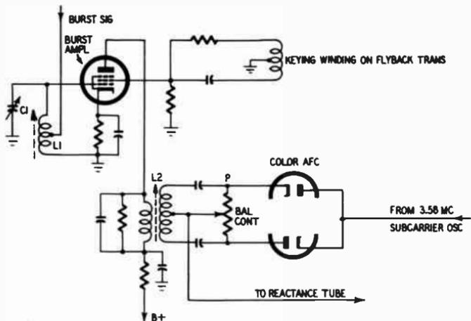
Fig. 208. Burst amplifier and color afc circuits.
