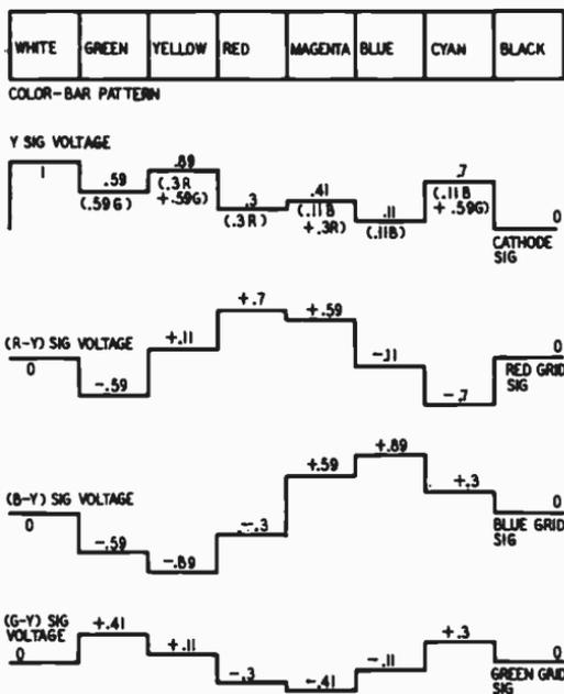
Fig. 502. The relative voltages applied to the electrodes of the picture tube when a 100%-saturated NTSC color bar signal is applied to the luminance and chrominance circuits.
