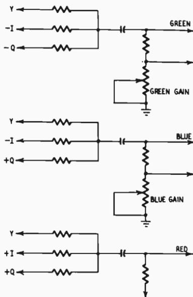
In a small number of sets  $(R - Y)$  and  $(B - Y)$  detectors are used, with a  $(G - Y)$  matrix, but the matrixing of the color-difference signals with the Y signal is not accomplished in the picture tube but in a separate resistive matrix similar to the I-Q matrix. When checked for proper matrix action, the scope is applied at the matrix input terminals instead of at the grids and cathode of the picture tube. The signals found in normal operation are the same as those of Fig. 502.
