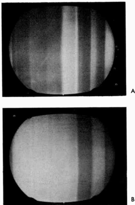
*Fig. 215. The photo at the top shows a color-bar pattern with Y and chroma both in sync. The lower photo shows a color-bar pattern with loss of color sync and retention of Y sync.*
