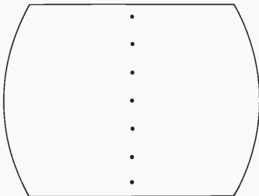
Fig. 112. To make the vertical dynamic convergence adjustments, focus your attention on the vertical column of dots down the center of the screen.
