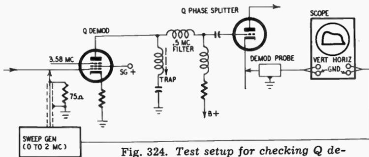
Fig. 324. Test setup for checking Q demodulator response.
