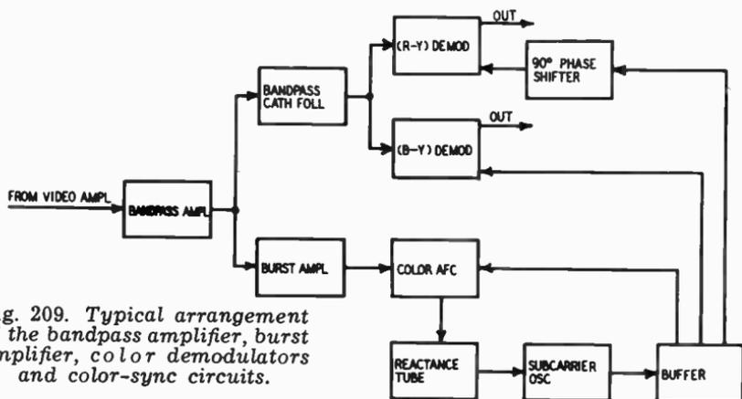
Fig. 209. Typical arrangement of the bandpass amplifier, burst amplifier, color demodulators and color-sync circuits.
