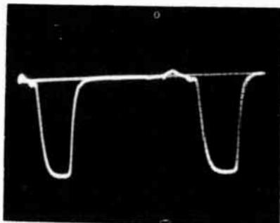
Output from Q detector, I signal nulled satisfactorily. Residual I signal is seen only as a small irregularity in the base line. The corners of the Q bars are rounded because of the relatively narrow bandpass of the Q demodulator circuit.
