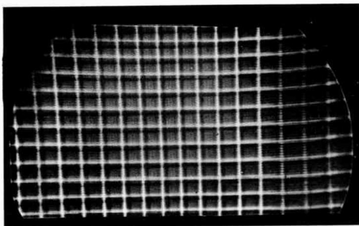
Fig. 111. *Crosshatch pattern displayed on misconverged picture tube.*
