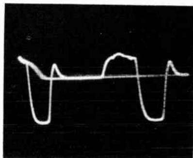
Output from Q detector; considerable contamination of Q bar with voltage from the I bar; I bar extends upward in photo; Q extends downward. Contamination is caused by misadjustment of color phasing control.
