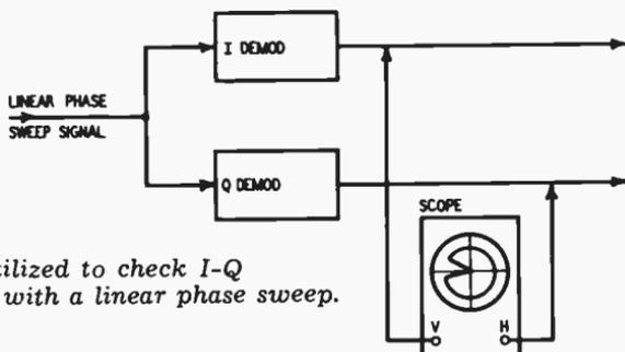
Fig. 407. Test setup utilized to check I-Q demodulators with a linear phase sweep.
