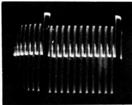
Fig. 411. *Keyed output of linear phase sweep generator.*
