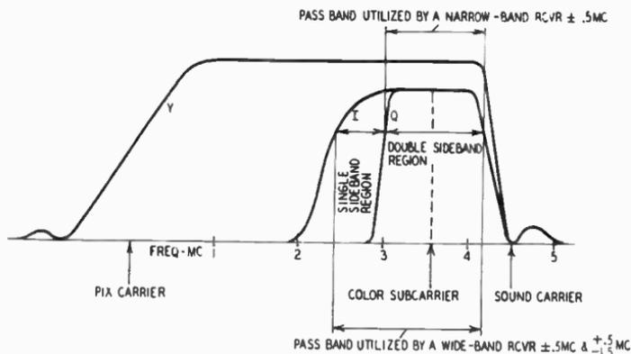
Fig. 602. Complete color signal has double- and single-sideband components within the chrominance region. Wide-band receivers utilizing the single-sideband chrominance signal must be aligned to take the half-voltage level of the single sideband into consideration.
