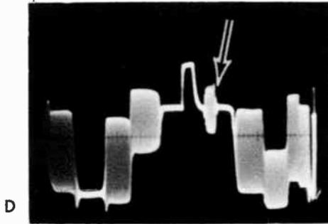
Compare the size of the burst signal with the photos in B and C.
