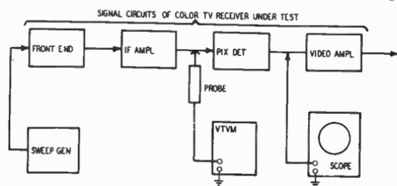
Fig. 811. *Demonstration setup to display probe loading effects.*
