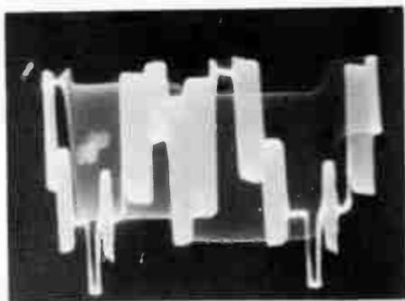
The next step (photos 24, 25 and 26) is to adjust the burst amplitude.
