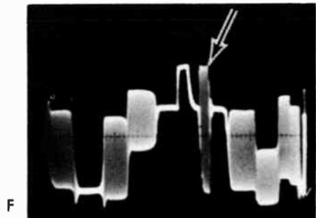
Maximum burst signal amplitude.
