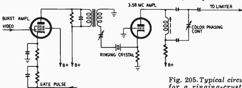
Fig. 205. Typical circuit for a ringing-crystal subcarrier oscillator.
