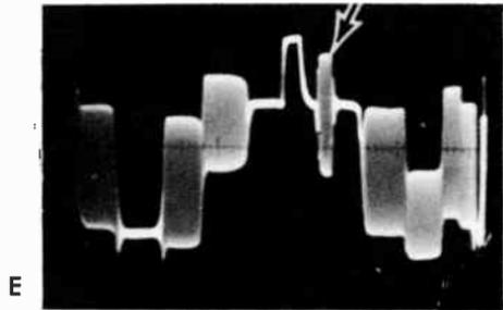
The burst now has a greater amplitude than that of the photo marked D.
