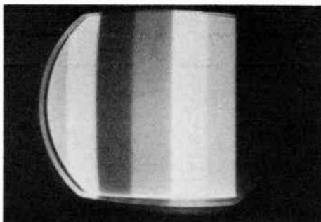
The controls can also be set on the basis of a chrominance signal as observed on the screen of a wide-band scope. However, some service technicians prefer the picture-tube display and believe that it provides a closer check on bar widths than does a scope.
