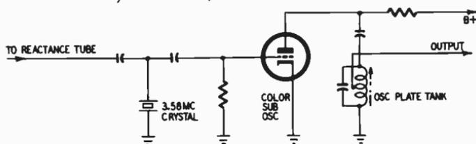
Fig. 216. Typical color-subcarrier oscillator. Low plate voltage indicates a non-oscillating circuit.
