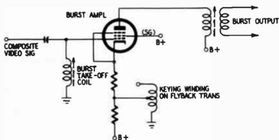
Fig. 203. The burst amplifier is keyed by a gate pulse from the sweep section.
