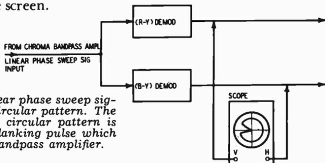
Fig. 403. The linear phase sweep signal produces a circular pattern. The "pie cut" in the circular pattern is formed by the blanking pulse which is fed to the bandpass amplifier.
