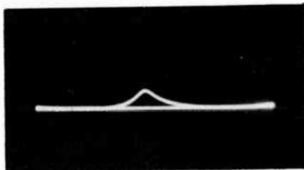
Fig. 814. Lesser attenuation of if signal by vtvm signal-tracing probe.
