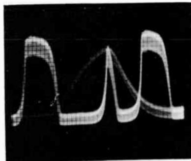
A complete color bar signal as seen when the signal is applied to the antenna input terminals of the receiver and a wide-band scope is applied at the output of the picture detector. This pattern shows some attenuation of 3.58-mc signal (burst should have same peak-to-peak voltage as the sync pulse). Overshoot of bar signals is also evident. These faults can be corrected by careful realignment of rf and if circuits.
