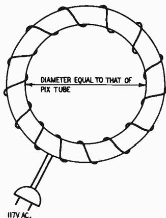
Fig. 108. A degaussing coil has the appearance of a large doughnut. The diameter of the coil is about the same as the rim of the picture tube. It provides an ac field for demagnetizing the picture-tube shield.
