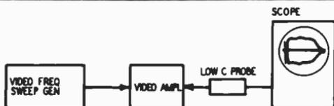
Fig. 301. When a video-frequency circuit is checked with a sweep-frequency signal, the scope displays the outline of the circuit's frequency response.
