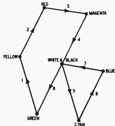
A vectorscope check of the color demodulators against a color bar signal is very informative and supplies a large amount of operating data in convenient form. When a color bar signal is applied to the receiver and the color demodulators are connected to a scope with the output from the  $(R - Y)$  demodulator energizing the vertical amplifier and the output from the  $(B - Y)$  demodulator fed into
