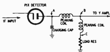
Fig. 801. Three possible test points are shown at A, B and C.
