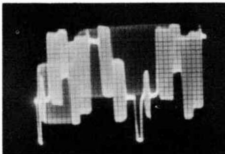
The bar sequence observed here is: green, yellow, red, magenta, white, cyan and blue. The bars have been adjusted to have approximately equal widths. To produce yellow, the green and red bars are overlapped. Magenta is obtained by overlapping red and blue. Cyan is produced by overlapping green and blue. White requires three colors—red, green and blue. (See photos 8, 9 and 10).
