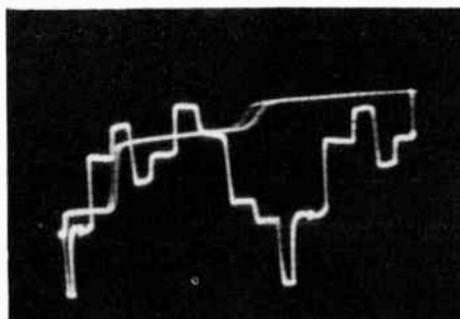
Since the amplitude of the green-bar Y component is 0.59, it is convenient to adjust the vertical gain of the scope so that the green bar occupies 59 squares. See photos 30, 31 and 32.
