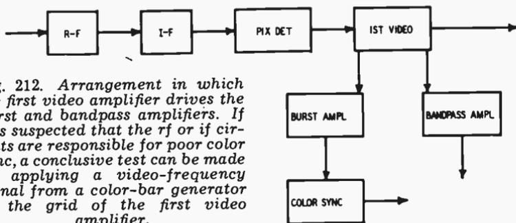
Fig. 212. Arrangement in which the first video amplifier drives the burst and bandpass amplifiers. If it is suspected that the rf or if circuits are responsible for poor color sync, a conclusive test can be made by applying a video-frequency signal from a color-bar generator to the grid of the first video amplifier.
