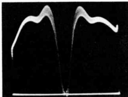
each square indicates an interval of 0.1 mc. Frequency points are then determined at any desired point along the response curve by counting squares and multiplying by 0.1 mc.
