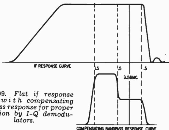
Fig. 609. Flat if response curve, with compensating bandpass response for proper utilization by I-Q demodulators.
