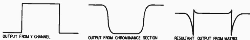
Fig. 511. Waveforms cancel, but have transient residues.
