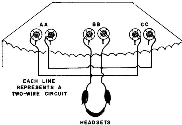
Fig. 202. Diagram of the stereophonic pickup system used at the Berlin Opera House in 1925.
