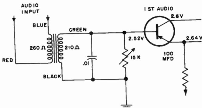
Fig. 603. In this circuit the volume control is placed across the secondary of the audio driver transformer.
