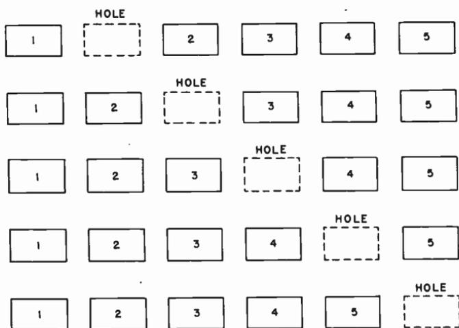
Fig. 109. Each block represents a freight car. The vacant space or "hole" can be made to move back by changing the positions of the cars.
