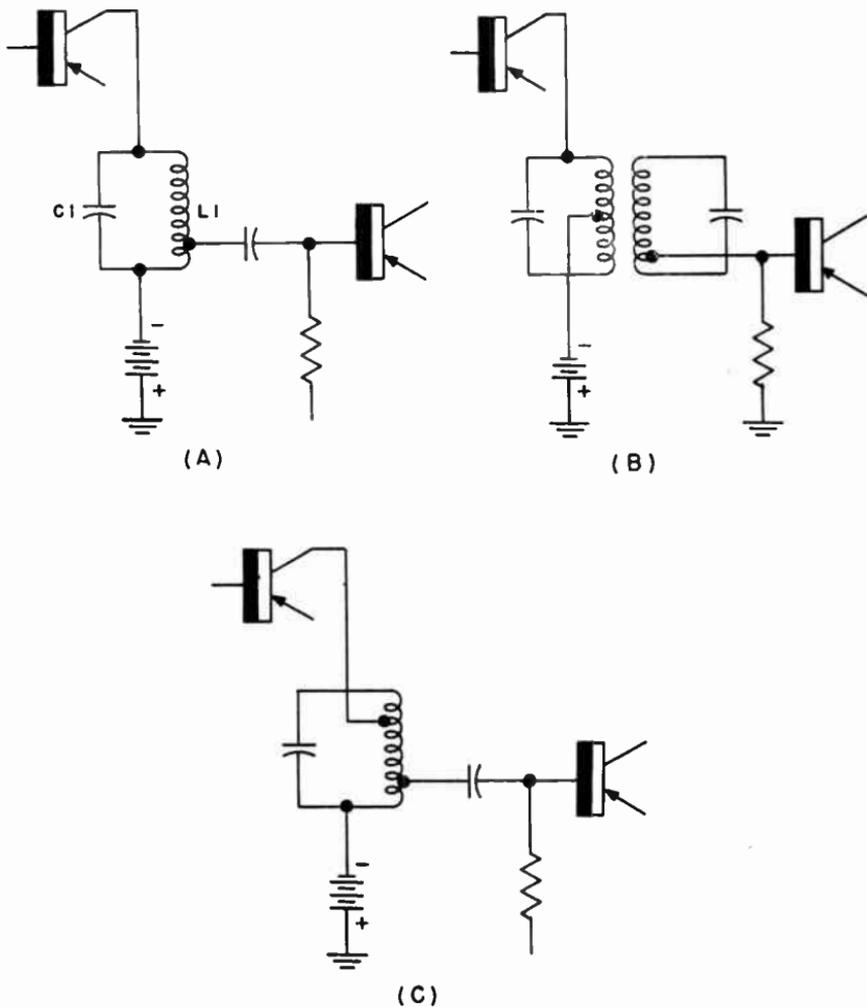
Fig. 419. Other methods used in coupling if stages.
