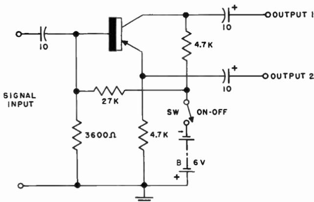
Fig. 614. A single transistor can be used to supply two outputs.
