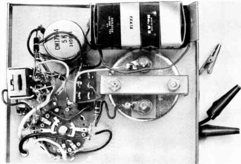
Fig. 219. *Factory-wired transistor tester uses a calibrated potentiometer. Clip leads supplement transistor socket.*
