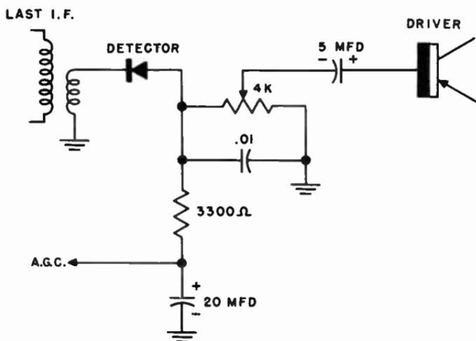
Fig. 601. Volume control circuit. Note the large-value coupling capacitor between the volume control and the base input circuit of the driver stage.
