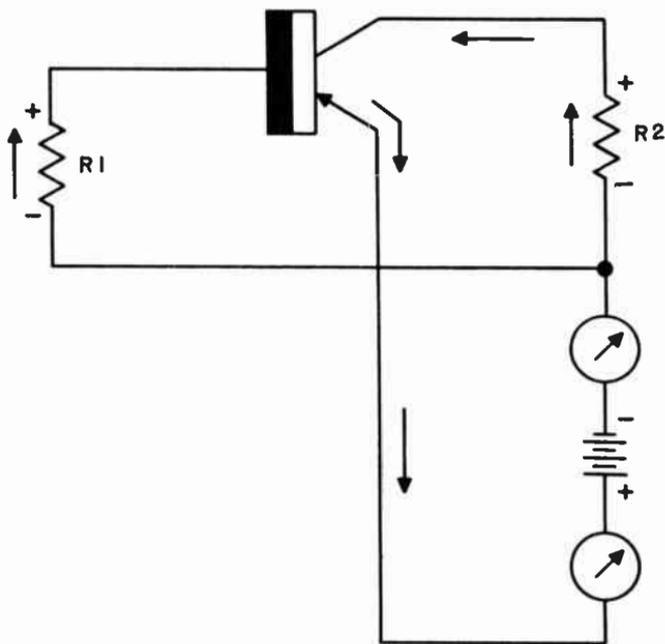
Fig. 306. *The electron flow out of the battery is identical to the electron flow into the battery.*
