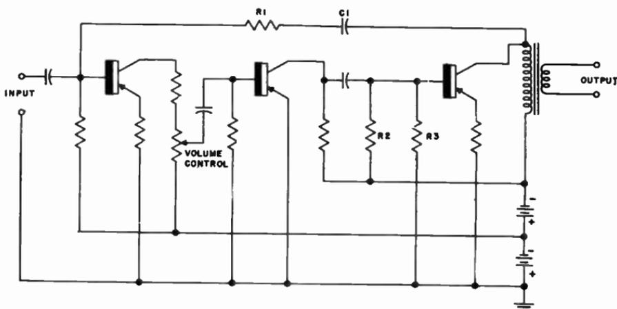
Fig. 321.  $R_1$  and  $C_1$  represent the negative feedback circuit. The amount of voltage fed back depends upon the values of  $R_1$  and  $C_1$  and also upon the output signal voltage.  $R_2$  and  $R_3$  form a voltage divider across the battery supply and place the correct amount of bias voltage on the input circuit of the last transistor.
