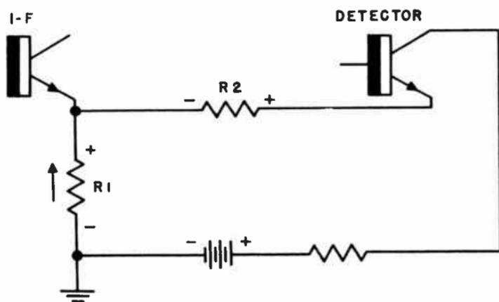
Fig. 507. Basic arrangement of an agc circuit.
