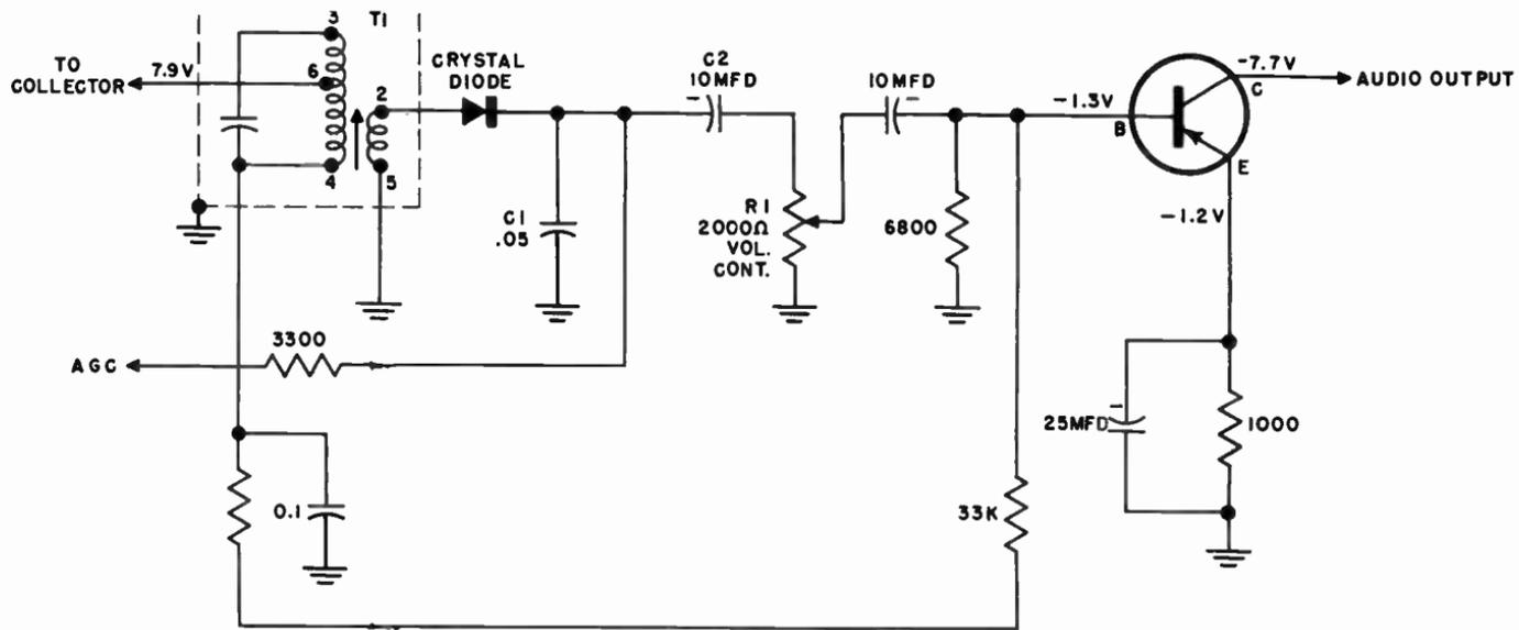
Fig. 503. Typical crystal detector circuit. The agc bus is taken from the output of the detector.
