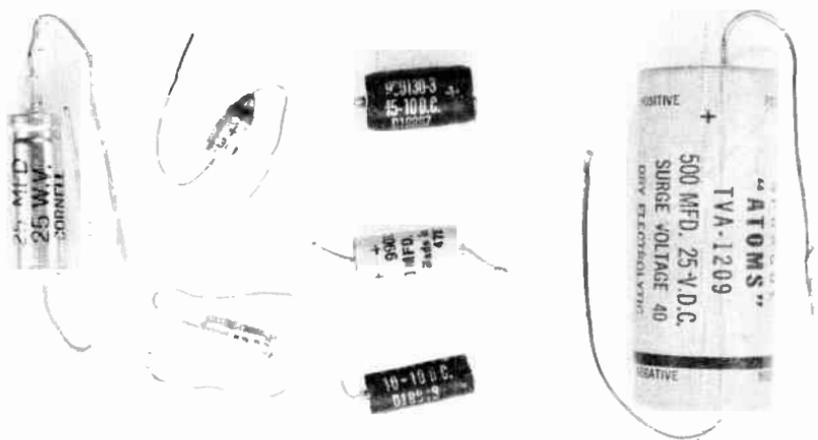
Fig. 427. These electrolytic capacitors are approximately one-half actual size.
