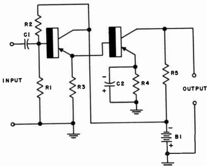
Fig. 319. *Direct-coupled transistor amplifier.*
