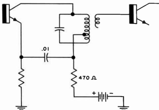
Fig. 416. Because of the presence of the  $.01 \mu\text{f}$  capacitor, the tap on the primary of the if transformer is at signal ground potential. Tapping down is a widely used method of obtaining a suitable impedance match.
