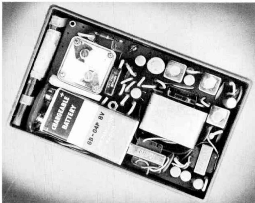
Fig. 425. Circuitry for six transistors fits compactly in the same space used by the receiver in Fig. 424.
