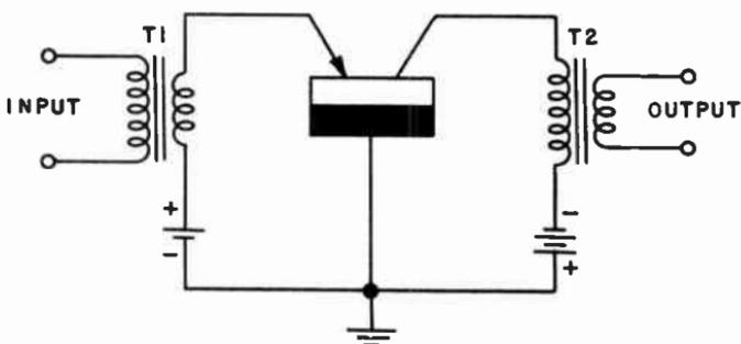
Fig. 215. Resistance- and transformer-coupled grounded-base amplifiers.
