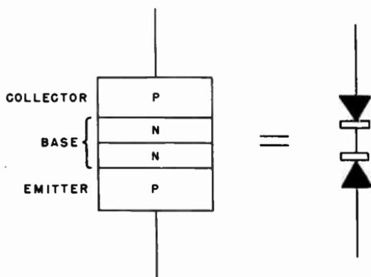
Fig. 203. If the n-region of the transistor is sliced in half (theoretically), it will form two diodes placed back to back.
