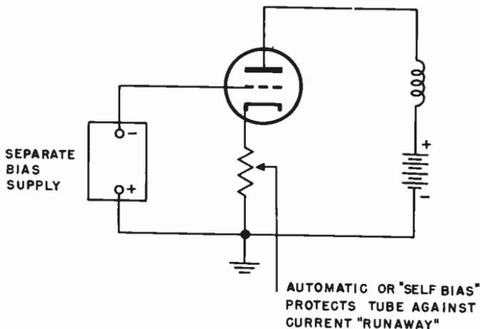
Fig. 304. *The cathode resistor helps keep the plate current within reasonable limits.*
