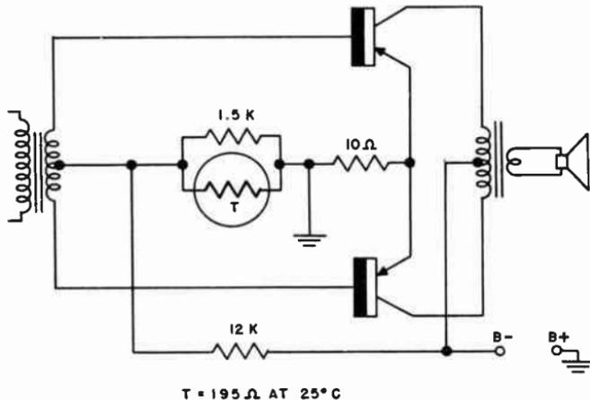
Fig. 607. The thermistor is placed in shunt with the common-base resistor of the two transistors.
