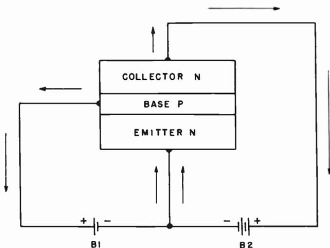
Fig. 207. Electron flow in the n-p-n transistor circuit.
