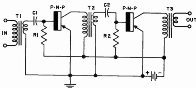
Fig. 315. Two-stage transformer-coupled amplifier using p-n-p units. A single battery supplies collector bias. Resistors R1 and R2 furnish fixed bias for the base-to-emitter input circuits.
