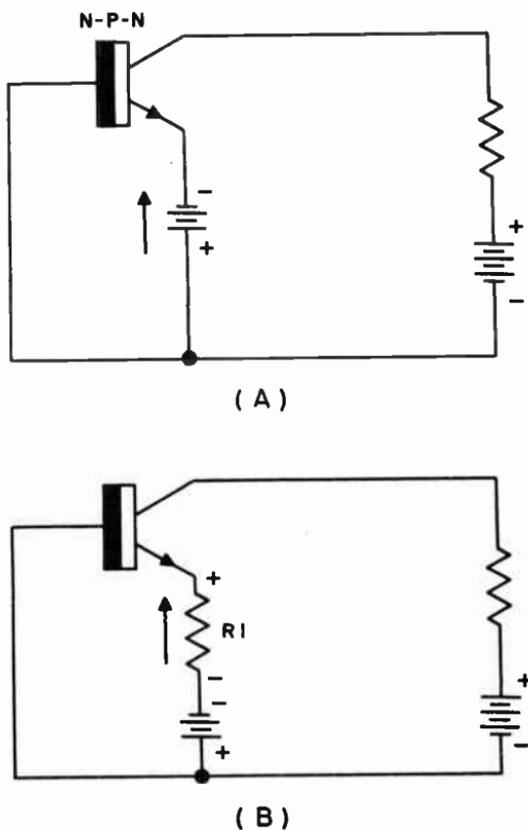
Fig. 506. Fundamental operation of an agc circuit.
