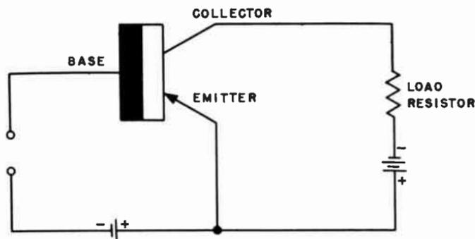
Fig. 211. Technique for connecting the load resistor to the transistor.
