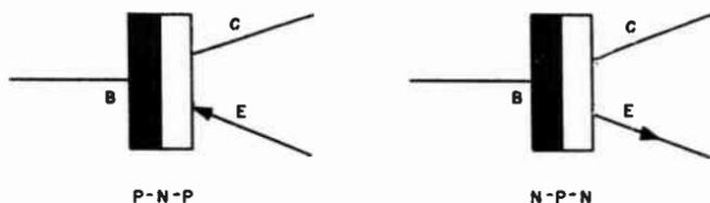
Fig. 209. Electronic symbols for p-n-p and n-p-n transistors.
