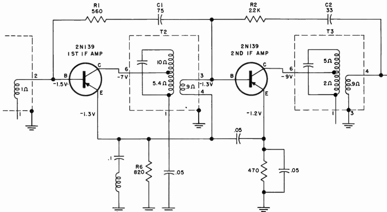
Fig. 421. Neutralization of transistor if stages.
