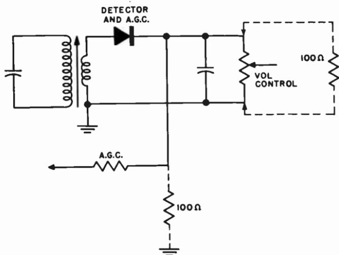
Fig. 513. To disable the agc, connect a 100-ohm resistor from the agc bus to ground.
