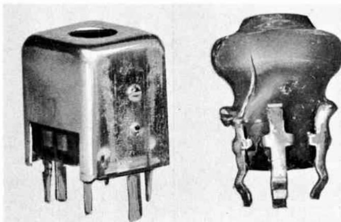
Fig. 422. Oscillator coil (left) and if transformer are attached to the printed-circuit boards by terminal lugs that are designed for easy insertion. (Thordarson-Meissner.)
