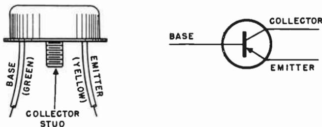
Fig. 606. Power transistors come in various shapes. The electronic symbol for all three-element transistors is the same.
