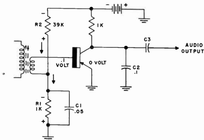
Fig. 505. Schematic showing a transistor used as a detector. The transistor has an advantage over the crystal diode in that it supplies gain.
