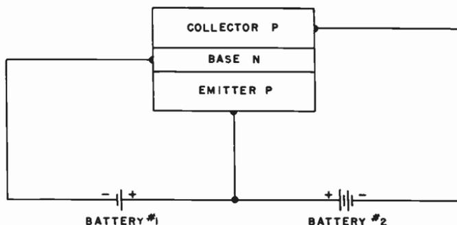
Fig. 202. *The transistor consists of an emitter, base and collector.*
