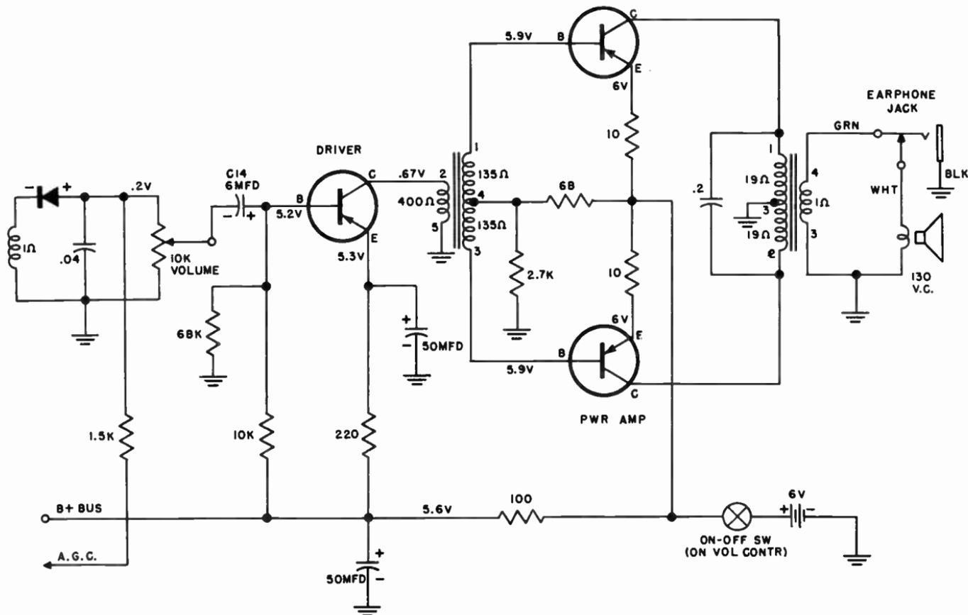
Fig. 609. Transistor audio amplifier using push-pull output.
