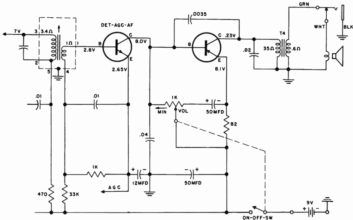
Fig. 605. Simple audio amplifier using two transistors. The detector transistor also supplies some audio gain.
