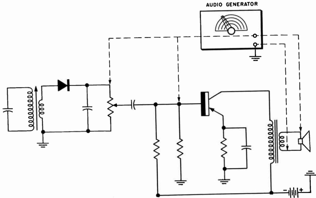
Fig. 220. There are a variety of connections that can be used for the audio generator signal-injection technique in finding a defective audio transistor. The practical applications of this system will be explained more fully in Chapters 7 and 8 in Vol. II.
