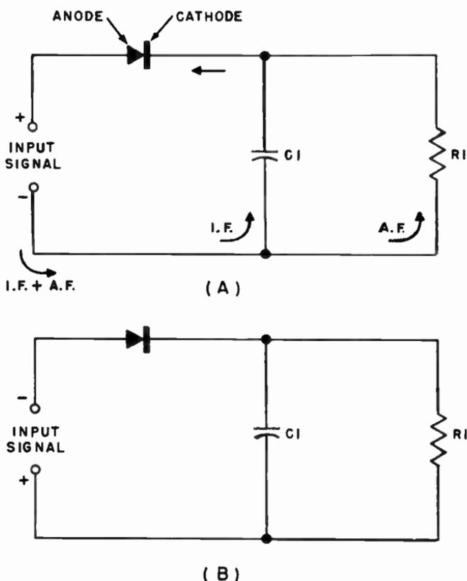
Fig. 501. When the input signal is of the proper polarity, current will flow through the diode, as indicated in A. When the input signal is reversed, practically no current will flow B.
