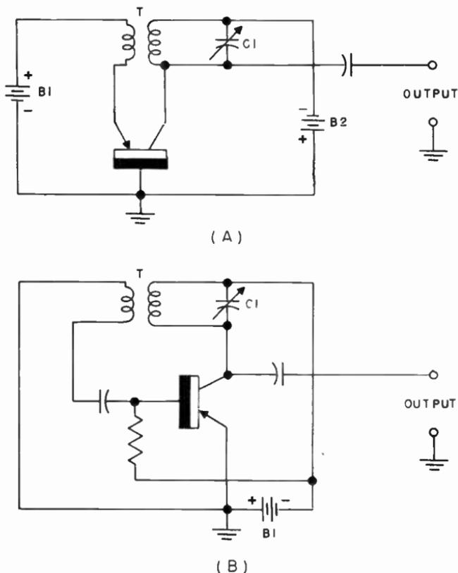
Fig. 413. *Grounded-base and grounded-emitter oscillators using a transformer for feedback.*
