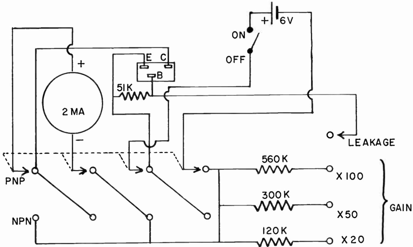
Fig. 218. Circuit used in a transistor tester kit. A meter, three switches, four resistors, a battery and a socket are all housed in a neat prefinished cabinet. (Electronic Measurements Corp.)
