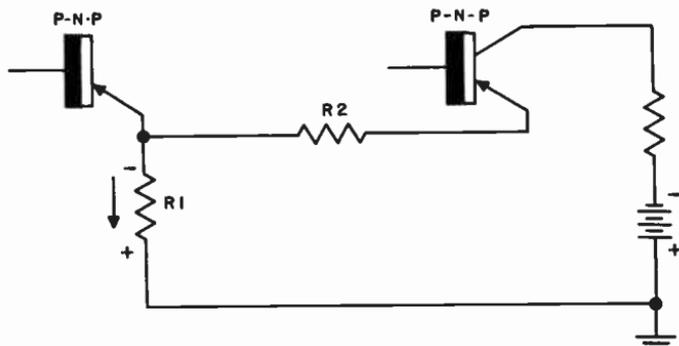
Fig. 510. Agc bias network for p-n-p transistors. Note that the voltage across bias resistor  $R_1$  is in opposition to the emitter bias voltage. Current flowing from the emitter through  $R_1$  reduces the forward bias, thereby lowering the gain of the transistor stage.
