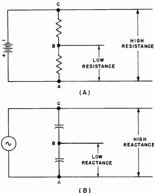
Fig. 417. Resistors and capacitors can be used as voltage dividers.
