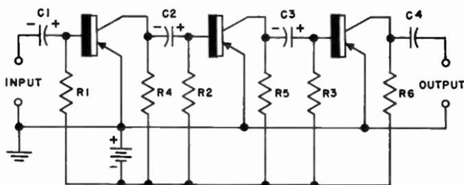
Fig. 318. R-C-coupled transistor amplifier using p-n-p units. Fixed bias is used throughout. The coupling capacitors can be  $2\text{-}\mu\text{f}$  tantalum electrolytics.
