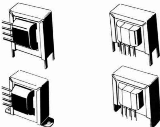
Fig. 316. Transistor transformers are small compared to those used in vacuum-tube receivers.
