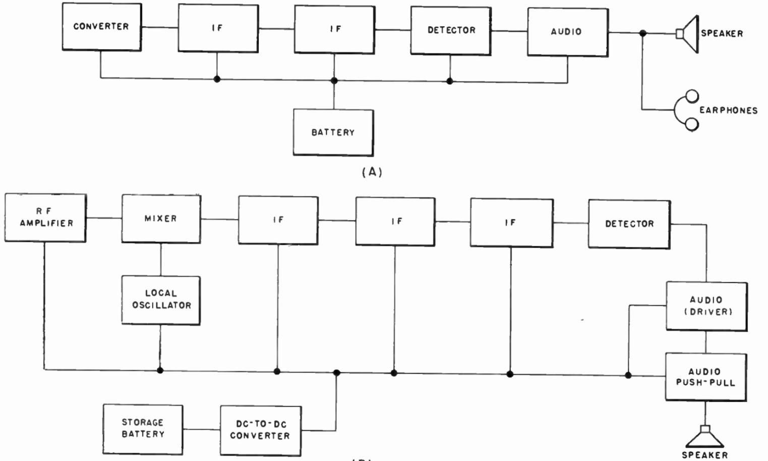
Fig. 406. Block diagram of a portable or home receiver (A) and a diagram of an auto radio (B). The automobile receiver is more complicated.
