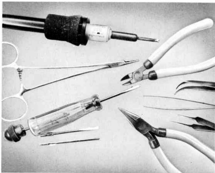
Fig. 401. Typical tools used in servicing transistor receivers.
