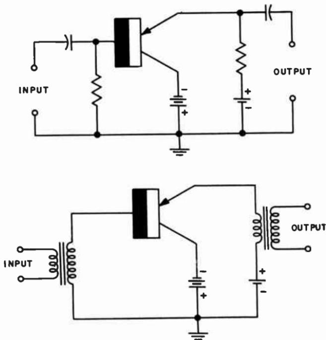
Fig. 217. Resistance- and transformer-coupled grounded-collector amplifiers.
