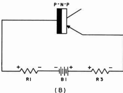
Fig. 307. The voltage across R1 supplies fixed bias. This bias remains fairly constant. The voltage across R3 supplies self-bias. The value of self-bias depends primarily upon the amount of collector current.
