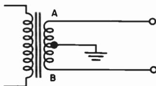
Fig. 613. An easy way to get out-of-phase voltages is to use a tapped transformer.
