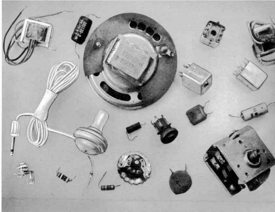
Fig. 118. A 2½ inch speaker is shown with many of the major components of a transistor receiver.
