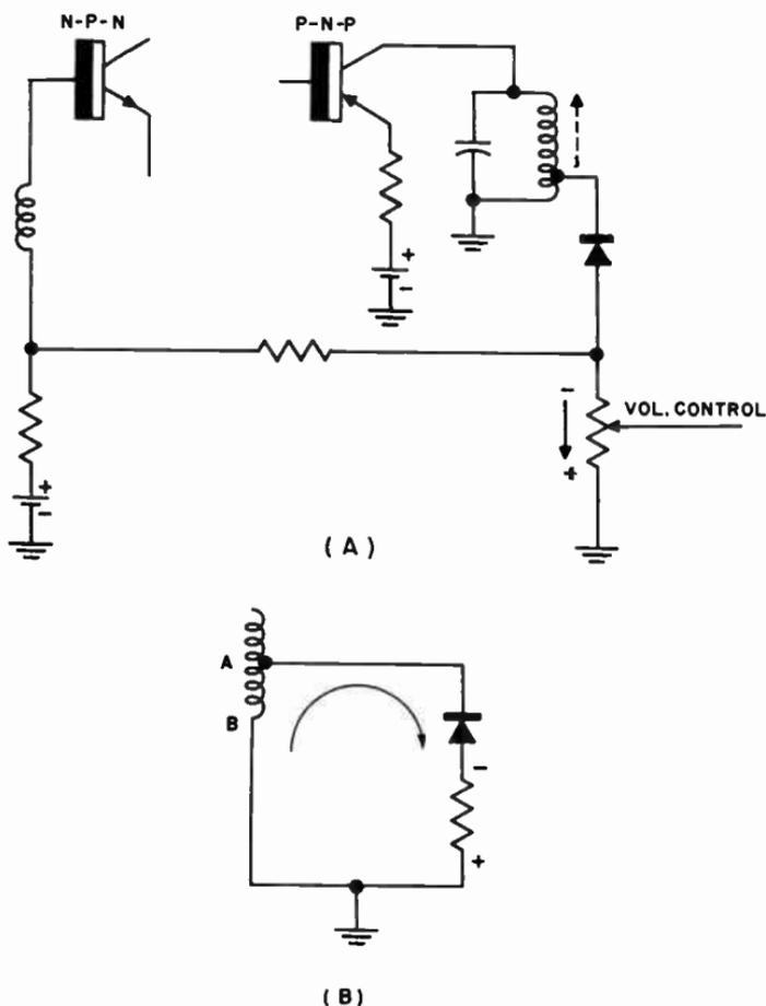
Fig. 511. Agc bias circuit for receivers using both n-p-n and p-n-p transistors. The agc voltage is used only by the n-p-n transistor.
