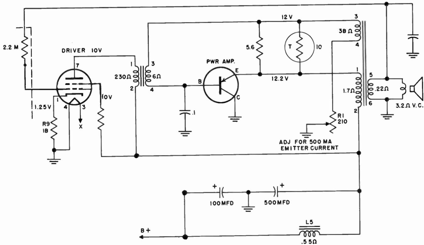
Fig. 611. Hybrid circuit using a vacuum-tube driver and power transistor for the output.
