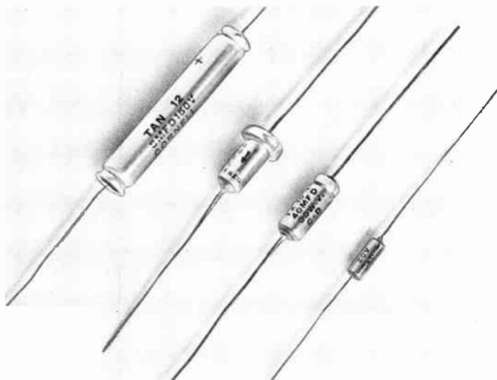
Fig. 314. The photo shows typical electrolytics used in transistor receivers. These are very small compared to the units you will find in vacuum-tube receivers.
