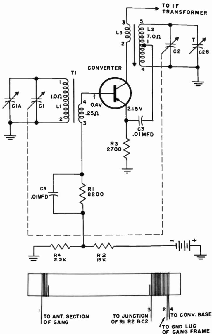
Fig. 409. Typical converter circuit. A Hartley oscillator is used. L3 is a feedback coil and is in series with the if transformer.
