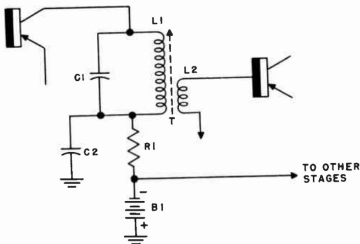
Fig. 415. The if transformer is a stepdown type. The collector circuit has a higher impedance than the base circuit of the following stage.
