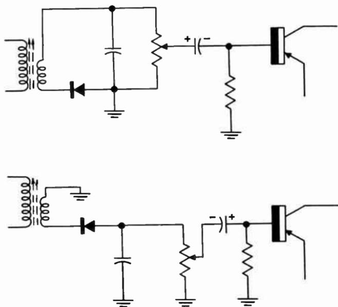
Fig. 504. Circuit arrangements using crystal diodes.
