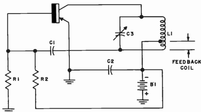
Fig. 412. Hartley oscillator. Oscillator action is the same as in a vacuum-tube type.
