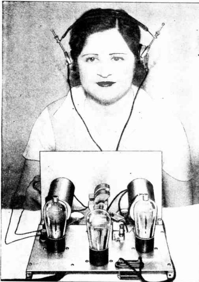
Here's a 3-tube short-wave receiver that you will derive a lot of pleasure from—it is up to the minute, with all controls mounted on the front panel, while switches change the wave bands.
