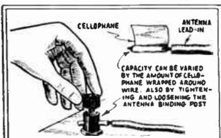
cially in experimental hook-ups. Capacity can be varied by the amount of Cellophane wrapped on the wire and also by tightening or loosening of the antenna binding post screw.—E. E. Thayer.
