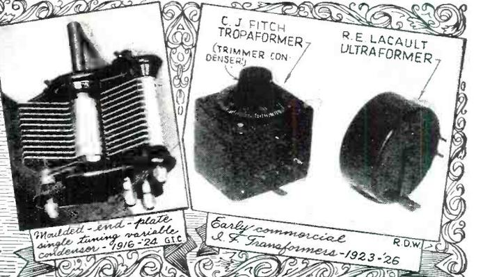
Milled-end-plate single tuning variable condenser, 1916-24 G.I. C.J. FITCH TROPAFORMER (TRIMMER CONDENSER) R.E. LACAULT ULTRAFORMER Early commercial S.F. Transformers, 1923-26 R.D.W.
