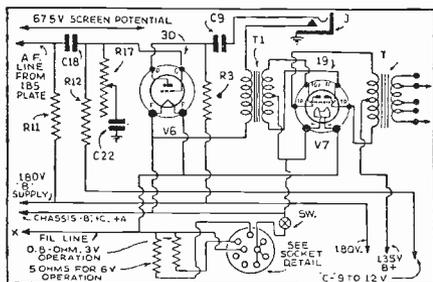
Fig. 43C—Audio channel of the battery super-heterodyne tuner shown in Fig. 43A.
