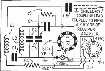
Fig. 91—Shows a circuit of a beat frequency oscillator that may be attached to any worthwhile receiver. Its purpose is to aid in bringing in distant stations.
