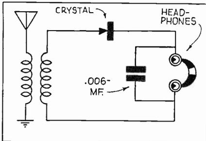
Students will find this simple crystal of great interest inasmuch as it uses a conventional tuner consisting of a solenoid and variable condenser to cover the broadcast band. A fixed crystal .006 MF mica condenser, and a pair of phones complete the balance of parts needed.
