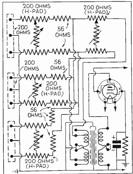
Fig. 67B—Mixer and input circuits with provision made for three microphones.
