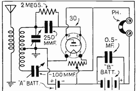
Regeneration by capacitive coupling. Feedback is controlled by the 100 MMF condenser.
