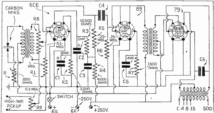
Fig. 54—A public address system for a carbon microphone and a high impedance pickup for portable use. It is battery operated, Class B output, capable of delivering from five to eight watts of power.
