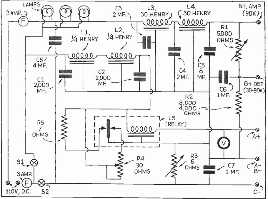
Fig. 75—An A-B-C Power Pack for D.C. Lines. Line voltage limits the output potential. With this power supply, frequent examination of the relay L5 is required. File the points if they become corroded or pitted, in order to insure stable operation; for, if this is neglected, varying output voltages will interfere with the radio reception.
