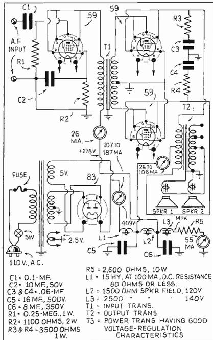
Fig. 69—A typical Class B audio frequency amplifier with an output of twenty watts.
