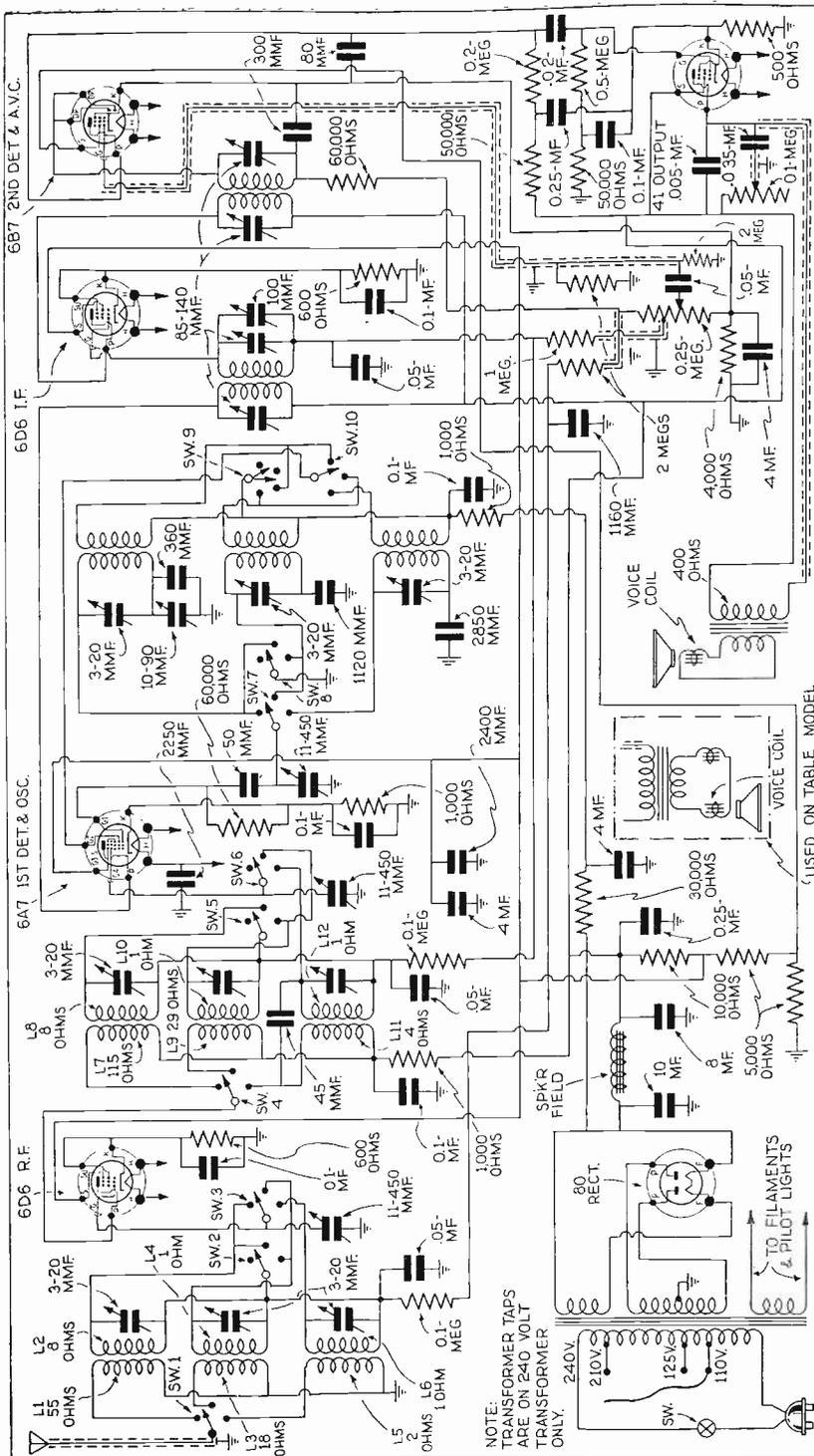
Fig. 38—RCA Victor Model 128. This circuit contains some very interesting features. This is a three-band 6 tube superheterodyne receiver with a stage of RF ahead of the first detector and oscillator, a 6D6 IF stage, a second detector, and AVC 6B7, and a 41 output tube. The 6B7 tube differs from most diode detectors inasmuch as it contains a screen grid element.
