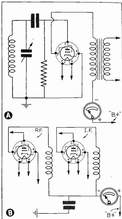
In Non-AVC receivers resonance does not cause a noticeable change in the plate current of any of the tubes except the detector. Therefore, the tuning meter should be connected in series with either the plate or cathode circuit of the detector. The plate circuit is preferable as the resistance of the meter need not be considered.
