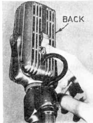
The output is comparable with the condenser type microphone and therefore requires a two stage preamplifier. This builds up the level to approximately -30 DB.
