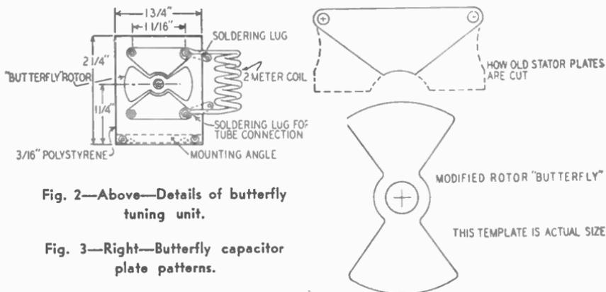
Fig. 2—Above—Details of butterfly tuning unit.
