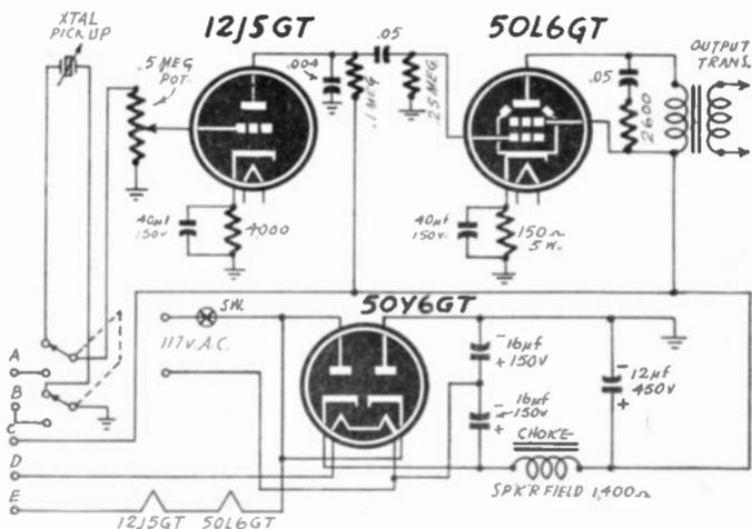
an inexpensive rim-drive phono motor. Then the mechanical reproducer was discarded and replaced by a crystal pickup. The next problem was to design an efficient amplifier small enough to fit the limited space and still leave room for a speaker. The minimum requirement appeared to be a two stage unit with a transformerless power supply and on consulting the tube manual we decided the most suitable lineup of available tubes to be a 12J5GT driving a 50L6GT, with a 50Y6GT rectifier.
