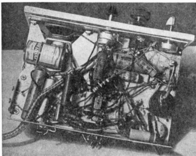
tinuous range from  $4\frac{1}{2}$  to 10 meters; but the additional coils required can easily be constructed. The coils are connected to the receiver by means of a three-terminal strip mounted on an adapter unit which is plugged into the coil socket. The r.f. choke, mounted in the adapter base, consists of about 20 turns of number 28 d.s.c. wire wound upon a  $\frac{1}{4}$ -inch wooden dowel. The coil and dowel should be carefully doped.
