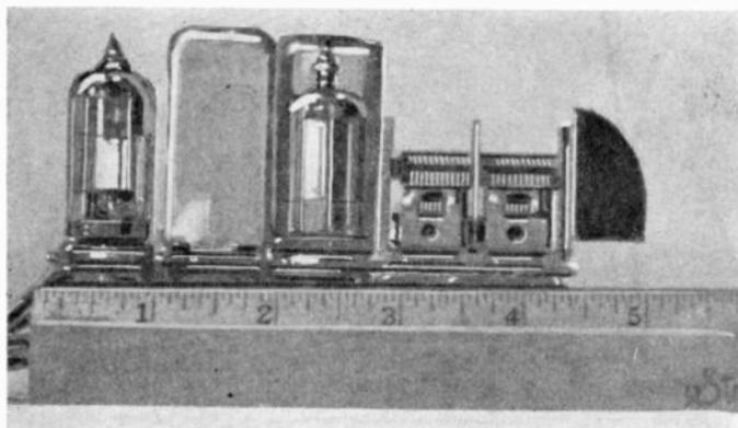
Chassis of the receiver — less than  $4\frac{1}{2}$  inches long.
