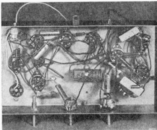
iron-core high-gain coils. As with the r.f. stage, no grid bias other than the a.v.c. is applied to the single 6K7 i.f. tube.
