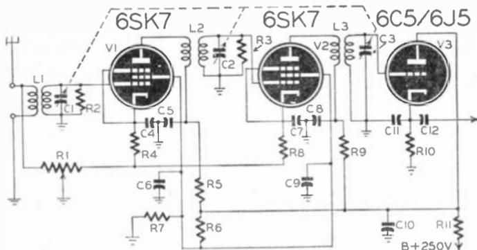
Fig. 5—Tuner is a 3-tube t.r.f. with infinite-impedance detector.
