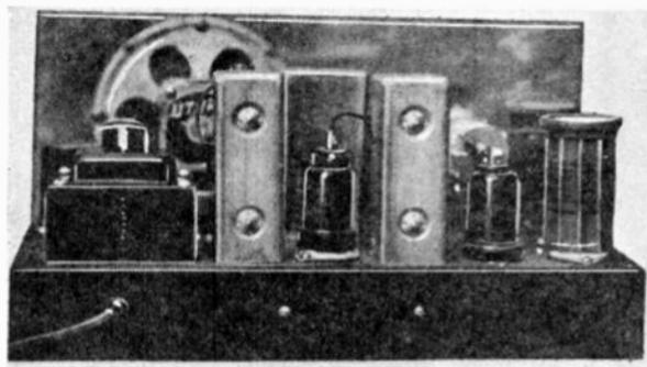
former. It was necessary to mount one of the small filter chokes above the chassis and at an angle to make room for the small speaker.
