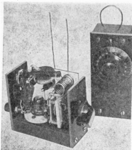
Front view of 955 receiver and wavemeter.
