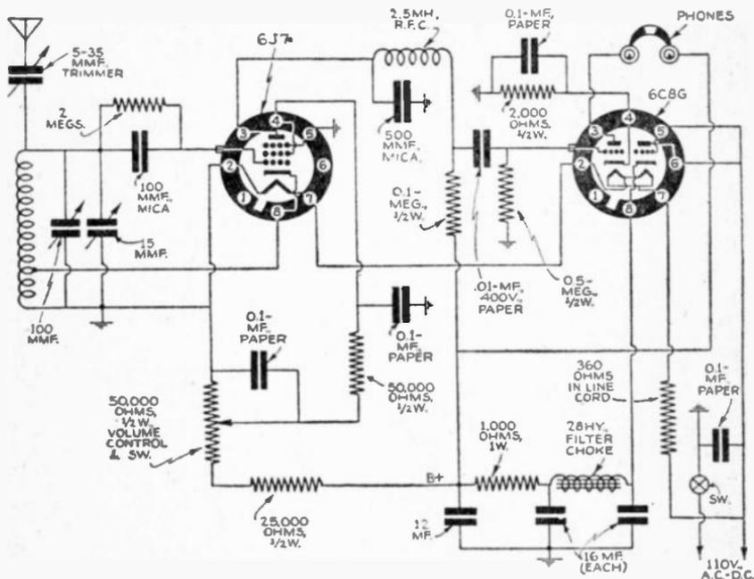
Fig. 1—Circuit of 2-tube beginner's receiver.
