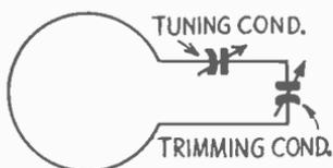
Fig. 5—Absorption wavemeter circuit.
