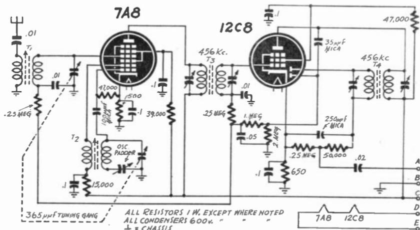
Schematic. The connections between the two sections of the diagram are keyed A-A, B-B, etc. Consider these solid connections when tracing circuits from one section to the other.
