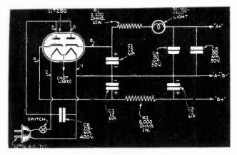
Diagram of Power Supply for operating battery-portables on A.C.-D.C. light lines.
