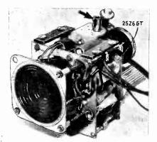
Fig. C. Chassis lying on its side shows the relationship of the speaker to the rest of the set. The arrow points to the shaft coupling which fastens the wheel to the tuning condenser shaft,
