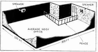
Fig. 6. A call system speaker placement was solved as shown above.
