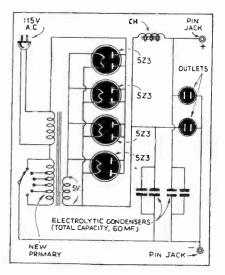
Fig. 1. Four 5Z3's in parallel deliver enough D.C. from 110 V. A.C. to operate a standard 110-V. D.C. radio set.
