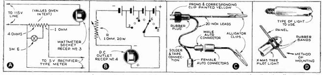
Fig. 2. The simple wattmeter circuit . . Hookup of the D.C. outlet . . Details of the D.C. cord . . Mounting the pilot lights 1940 RADIO-TELEVISION REFERENCE ANNUAL just pass the current through a known resistor and measure the voltage drop, calibrating the meter directly in watts. I use a 5-volt A.C. meter.
