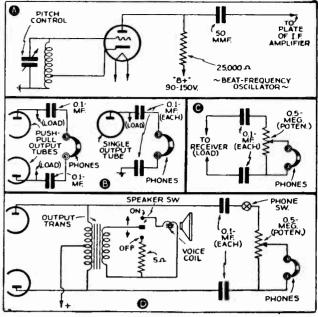
Fig. 2. B. F. O., headphone and loudspeaker connections.
