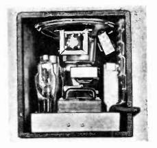
Fig. A Fig. B Fig. C View of the complete 3-tube A.C. superhet- View of the compact chassis. The entire View looking inside the cabinet. Note how erodyne receiver. Note that the speaker grille width is only 6 ins. The rectifier tube is compactly everything is mounted and how is on top of the case. The top knob is volume, combined with the output tube in one en-velope, a 12A7. components.
