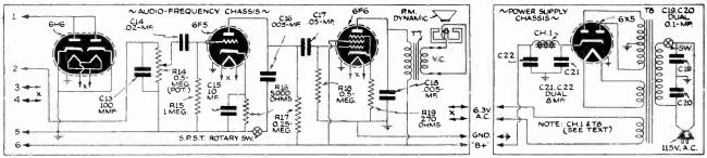
Fig. 3. Circuit arrangement of the A.F. unit.
