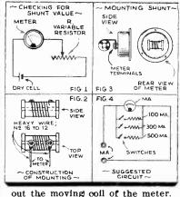
The resistor must be large enough to reduce the voltage to the amount needed to give full-(Continued on following page)
