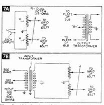
Fig. 7. (A) Push-pull input and push-pull output of a direct-coupled amplifier system. (B) Push-pull input connection,
