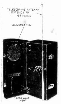
Fig. B. The selectivity of this little receiver is surprising. We were able to receive numerous stations in the editorial offices of Radio-Craft, located in a modern steel building in New York City, without interference., The "A" battery is located with the speaker where the thermos bottle is usually contained—in the cover.
