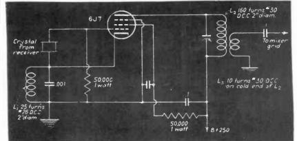
Fig. 1-Using crystal oscillator to check communication receivers.
