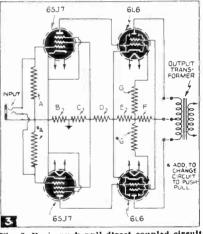
Fig. 3. Basic push-pull direct-coupled circuit. Note that only 2 extra resistors are required to change the circuit from a basic single to basic push-pull.
