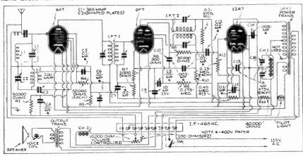
Fig. 1 Complete schematic diagram of the 3-tube A.C. superheterodyne receiver. The set is designed exclusively for the broadcast band. This circuit affords splendid reception even to the ex-tent of DA-ing Californian stations.
