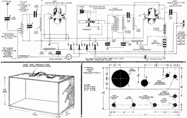
Diagram of connections for the 2½ meter Transceiver. A single 4-pole double-throw switch converts the circuit from "Talk" to "Listen" 1940 RADIO-TELEVISION REFERENCE ANNUAL Page 53
