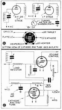
Fig. 6. A shadovgraph or tuning meter is attached to a superhet, as shown in A. Section B gives the socket connections for a visual tuning tube; and C, its circuit connection,
