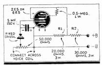
db. or watts. It may be found necessary to reverse the connections on the fixed crystal which is used as a rectifier. The supply voltages may be taken from the radio receiver or amplifier on which the device is to be used. A type 2E5 should be used if 2.5 V. is available and if 6.3 V. is available a 6E5 should be used. The regular high voltage of the amplifier may be used.
