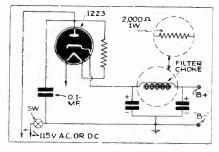
Fig. 4. The rectifier and filter circuit.
