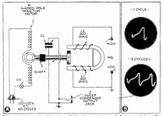
Fig. 2. Schematic diagram of the frequency modulator and impulse generator, and (15) the waveform of 1 and 2 cycles of the impulse generated
