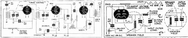
Fig. 2. Typical power-supply circuits of A.C.-D.C. sets.
