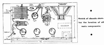
have low resistance to keep the voltage up and still have adequate filtering properties. About 400 ohms or less is satisfactory for the choke.
