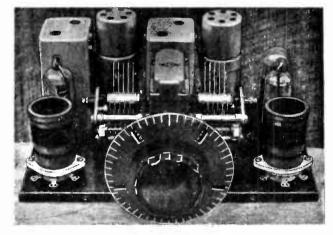
Front view of the superhet chassis, showing the National precision band-spread dial.
