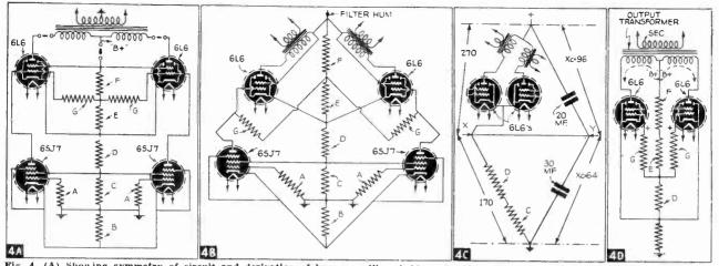
Fig. 4. (A) Showing symmetry of circuit and derivation of hum-cancelling bridge circuits. (B) Showing complex hum-balancing and voltage-balancing circuits. (C) Hum-balancing filter network. (D) Showing how hum is balanced in push-pull output transformer.
