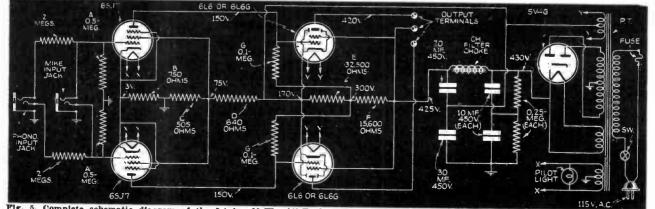
Fig. 5. Complete schematic diagram of the 5-tube, 10-W., All-Push-Pull Direct-Coupled Amplifier illustrated on the previous page. Page 42 1940 RADIO-TELEVISION REFERENCE ANNUAL
