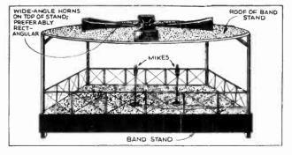
Fig. 4. A typicat park bandstand's arrangement of speakers is shown above.
