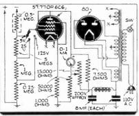
circuit requires no special switches or resistors, the range switch I used is an old 3-point tone control switch.
