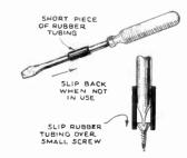
• A VERY simple means of preventing a screw-driver from slipping out of the slits of the screws in out-of-the-way places and for holding screws for placement in hard-to-reach spots. When not in use, the rubber may be slipped up the screw-driver shaft.
