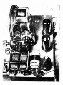
View of the completed chassis, showing placement of the more important units which comprise the Com-Rad
