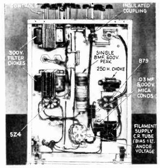
Fig. B. Under view of top power-pack pan. The under pan, hinged to it, is used only as a support and shield.
