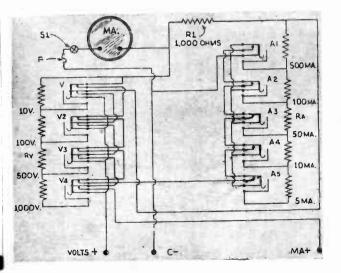
Fig. 1. Schematic diagram of the foolproof beginners' volt-milliameter.
