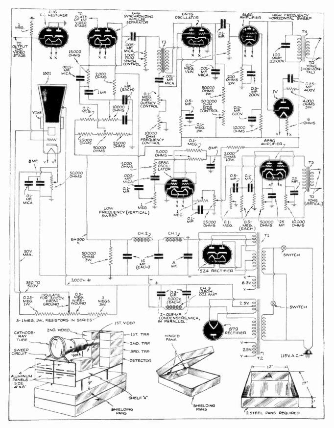
Schematic diagram of the 441-line T.R.F. Television Beceiver and complete dimensions for building the 2 required steel pans. The layout of all the main components is also shown.
