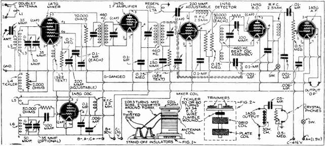
Schematic diagram and coll specifications for the superheterodyne receiver
