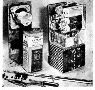
Fig. A. The "innards" of the Lunchbox Portable. One No. 6 drycell will run the set for months. Note the P.-M. dynamic speaker above the cell; and note the telescoping fishpole-type antenna which plugs into the front punch and extends to 45 ins.
