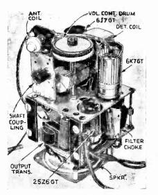
Fig. B. Front view of the compact 2-deck chassis. Two of the tubes are mounted on the top deck; the other 2 (one does not show here), on the lower deck—but protruding through the upper. Placement of parts is not very neat since all the parts, with space at a premium had to be eranmed in wherever they fitted.
