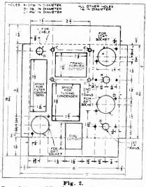
Fig. 2. Complete specifications for making and dril-ling the chassis for the 3-tube superheterodyne broadcast receiver
