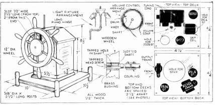
Fig. 3. Details for the lamp, volume-control drum and chassis.
