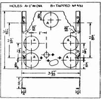
Fig. 2. Sub-chassis dimensions.
