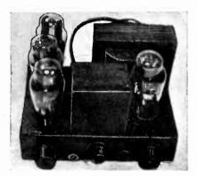
Top view of the A.C. to D.C. Power Supply,
