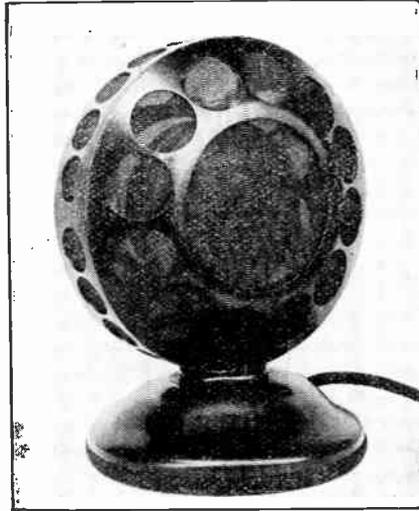
A microphone transmitter as used in radio broadcast stations.
