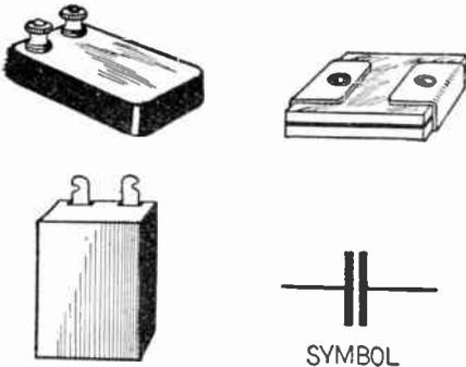
Fig. 28 (Test No. 33). Various types of fixed condensers used across the phoner in a radio receiver.
