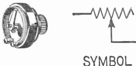
Fig. 18 (Test No. 17). Rear view of rheostat showing resistance wire and contact arm.
