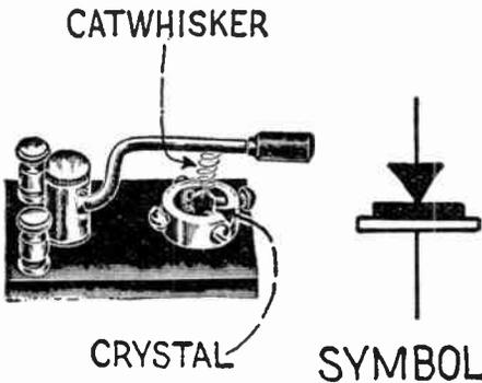
Fig. 29 (Test Nos. 34 and 35). A typical crystal detector.
