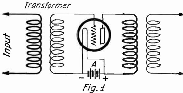
In the case of the detector this was taken advantage of to rectify the oscillations and make them audible in the telephone circuit. The relay action of the vacuum tube is used in the amplifier as we shall now explain.
