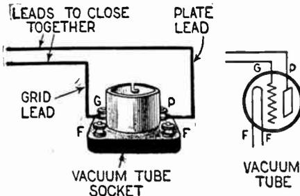
Fig. 23 (Test No. 27). Grid and plate leads from tube socket should be well separated.
