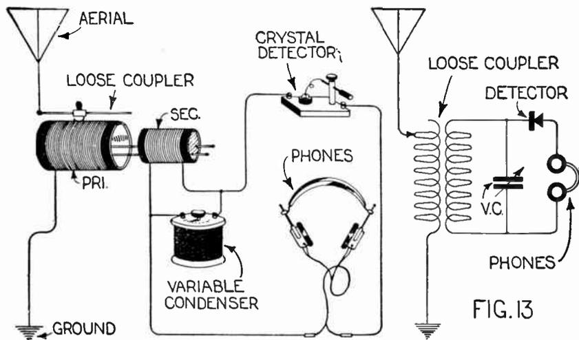
inductive circuits (Fig. 13), a considerable advancement over the preceding systems, as regarding selectivity and efficiency, has been made possible. However, in receiving, the inductive coupled method
