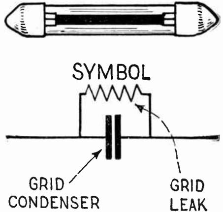
Fig. 22 (Test Nos. 21 and 22). A tubular type of grid leak.
