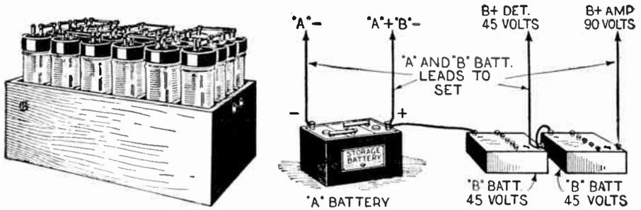
Fig. 9 (Test No. 4). At the left is shown a type of storage "B" battery, and at the right is indicated manner of connecting "A" and "B" batteries to a receiver.
