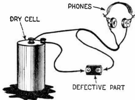
Fig. 5 (Test No. 1). Method of testing parts for defects.
