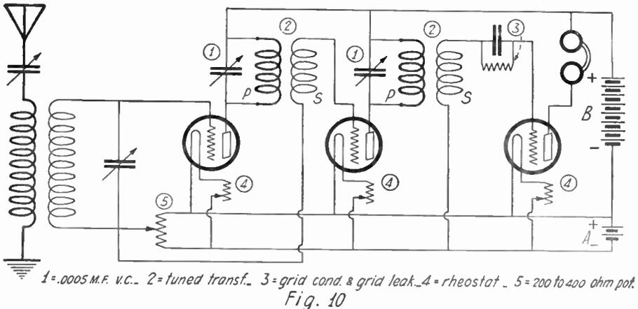
which cover a wide band of wave length. Generally the transformers used in short radio frequency amplifiers respond much better to a certain wave length than to some others, on account of the natural period of the windings. For short wave lengths it is therefore best to use some means of coupling between the tubes which may be ad-
