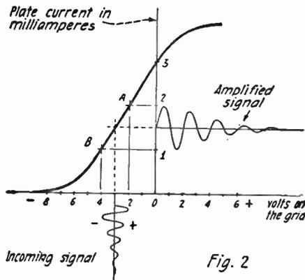
to operate it along the parts of the characteristic curve which is straight. In the case of Fig. 2 the incoming oscillation varies the grid potential from 1 to 3 volts negative producing a variation in plate current of 1 milliamperere. As may be seen, the greatest amplitude of the incoming wave train varies the point of operation from A to B along the characteristic curve which is straight, and therefore we
