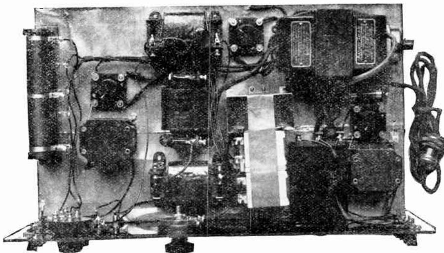
A combined power amplifier and "B" battery eliminator.
