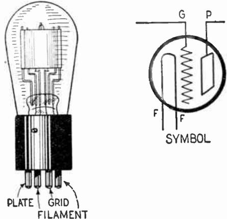
Fig. 27 (Test No. 81). A modern type of radio vacuum tube.
