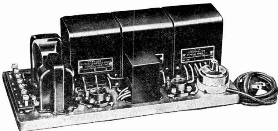
Another type of eliminator, combining a "B" power supply with a power amplifier and out-put filter as a last stage of audio for extremely loud signals.
