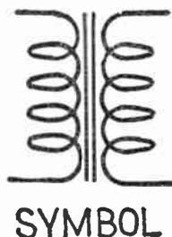
Fig. 20 (Test No. 19). An audio frequency transformer.
