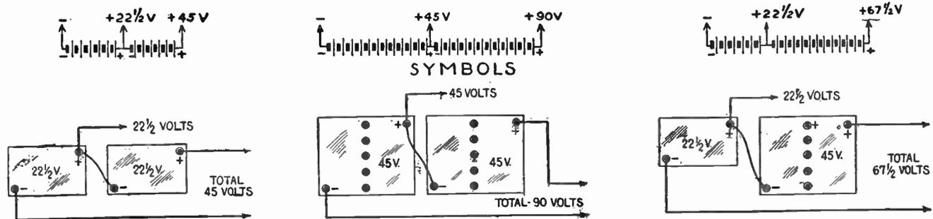
VARIOUS METHODS OF CONNECTING "B" BATTERIES
