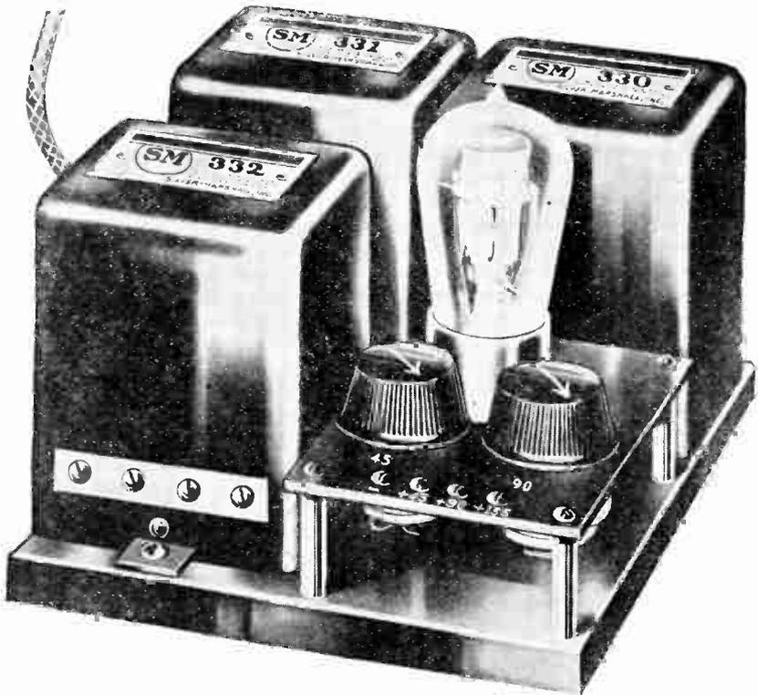
A modern "B" eliminator of the double wave vacuum tube rectifier type, which is being widely used by radio listeners of today. This tube is known as Raytheon.
