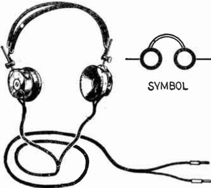
Fig. 26 (Test No. 80). Headphone much used in radio reception.
