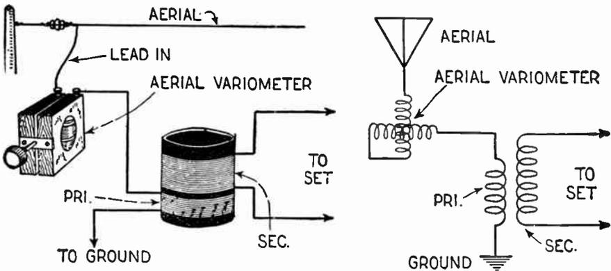
Fig. 12 (Test No. 10). Some sets use a variometer to tune the aerial circuit. The location of this variometer is shown above.
