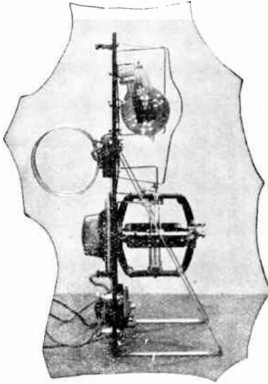
Side view of a short wave 5 meter transmitter showing the method of mounting the tube to keep down internal capacity.
