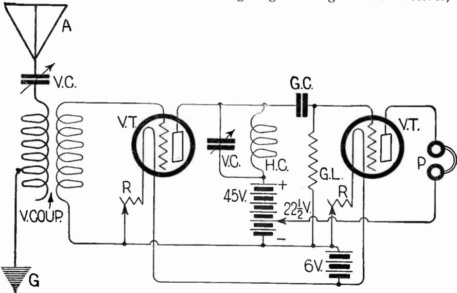
radio frequency amplification may be used ahead of it. Fig. 9 shows how this is accomplished. A single coil and variable condenser tune the antenna circuit and two tubes coupled by means of a radio fre-
