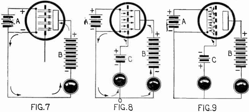
it will be seen that a current flows in the grid circuit because a certain number of electrons are stopped by the positively charged grid and allows the current of the battery B to flow in the circuit, in which case we have a grid-filament current.
