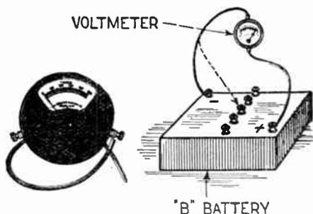
Fig. 8 (Test No. 4). Method of testing "B" battery voltage by means of a voltmeter.
