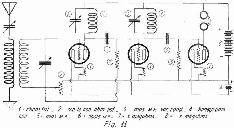
justed, or tuned to respond about equally well to a wide band of frequencies. Tuned circuits may be used and give, of course, best results since each stage may be adjusted so as to produce maximum amplification at the wave length which it is desired to receive, but one is soon limited along these lines on account of the number of
