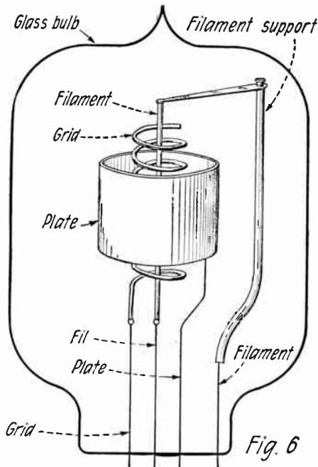
elementary one, it will function fairly well. In some cases, however, an additional set of batteries are used in the plate circuit with better results. The action of this circuit is a rectifying one; that is to say the incoming radio oscillations which represent the signals are rectified where but one-half of their alternations (that is their positive side) is permitted to pass through to the filament circuit and thence to the phones as previously mentioned in the graphs of Fig. 4.
