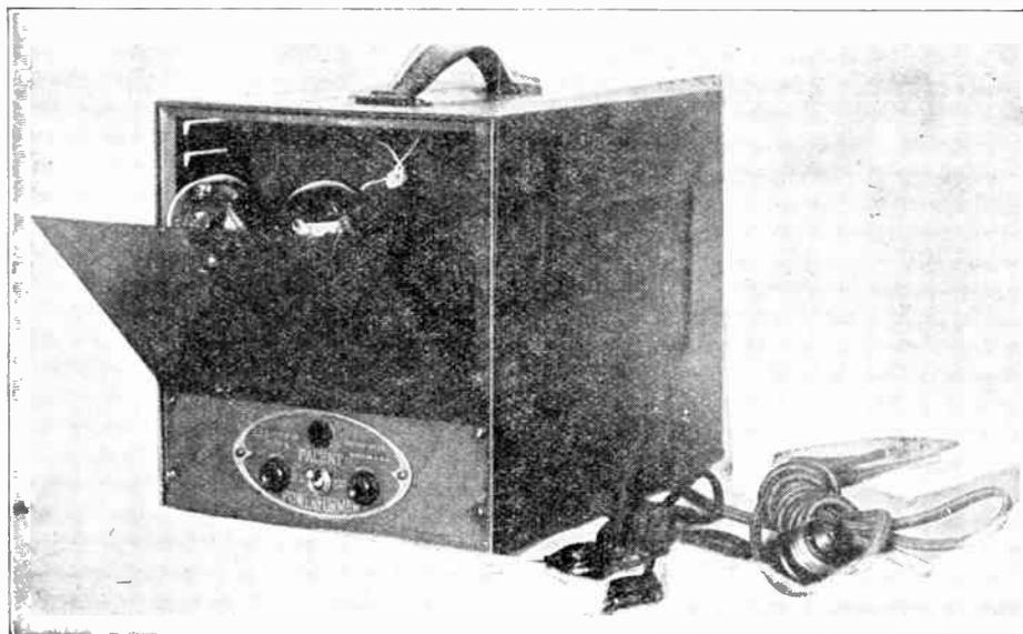
Another type of tube rectifier "B" eliminator and power amplifier.
