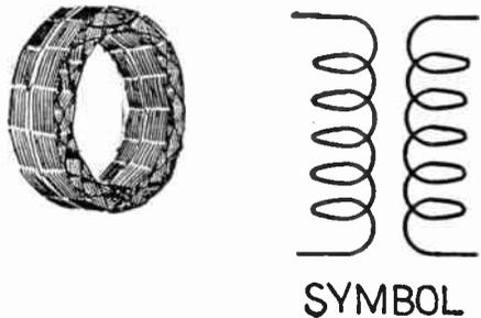
Fig. 30 (Test No. 37). A type of radio frequency transformer in common use.
