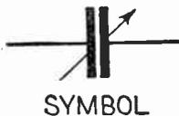
Fig. 15 (Test No. 14). A type of variable condenser.
