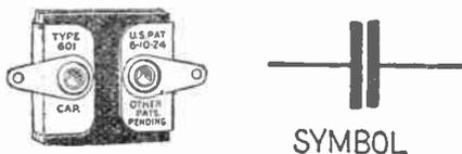
Fig. 14 (Test No. 18). A conventional type of fixed condenser
