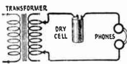
TEST FOR OPEN CIRCUIT
