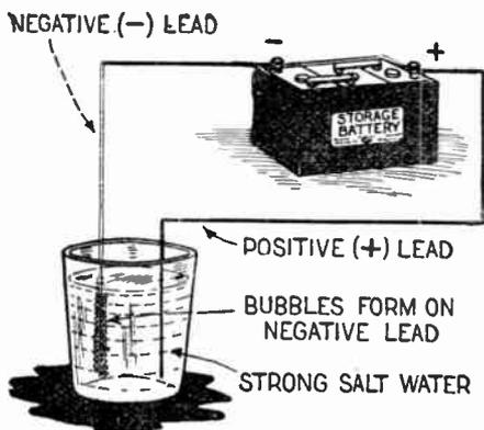
Fig. 7 (Test No. 3). How to determine positive and negative poles of an unmarked battery.
