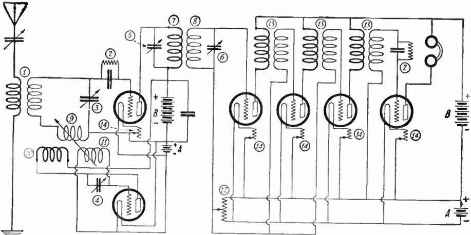
1 = vario coupler... 2 = grid leak & condenser... 3 = .0005 M.F... 4 = .001 M.F... 5 = .001 M.F... 6 = .001 M.F... 7 = L 500 honeycomb coil... 8 = L 600 honeycomb coil... 9 = 6 turns # 20 D.C.C. on 3" tube... 10 = 20 turns # 20 D.C.C. on 3" tube... 11 = 20 turns # 20 O.C.C. on 3" tube wound closely to 10... 12 = potentiometer... 14 = rheostat
