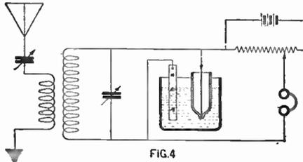
action of a current of electricity is called electrolytic action. When the plates are coated with gas bubbles they are said to be polarized. This polarization not only increases the resistance of the circuit but also sets up a difference of potential between the plates which acts in the opposite direction to the applied voltage and has a value of almost 1.5 volts. Therefore when polarization takes place the cur-
