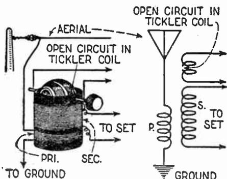
Fig. 18 (Test No. 12). In a regenerative circuit using a tickler coil, this coil may develop an open circuit. The tickler coil of a 8 circuit tuner is indicated above.
