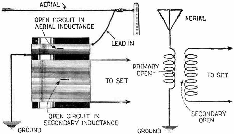
Fig. 10 (Test Nos. 7 and 8). Open circuit in aerial inductance and secondary inductance shown above. The diagram at left is in perspective and that on the right is in schematic form.
