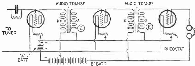
A.F. TRANSFORMER AMPLIFIER & DETECTOR
