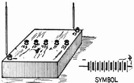
Fig. 25 (Test No. 29). A dry cell "B" battery. Fig. 9 shows a storage "B" battery and Fig. 1 the "B" battery connections for various voltages.
