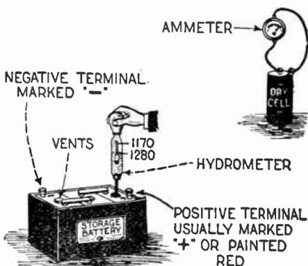
Fig. 6 (Test No. 2). Testing "A" battery voltage.
