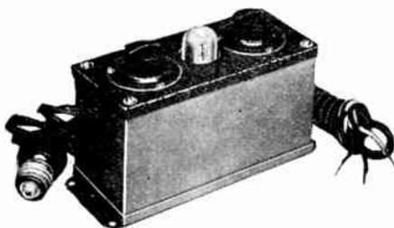
An eliminator for supplying "C" battery current for the up-to-date radio receiver.
