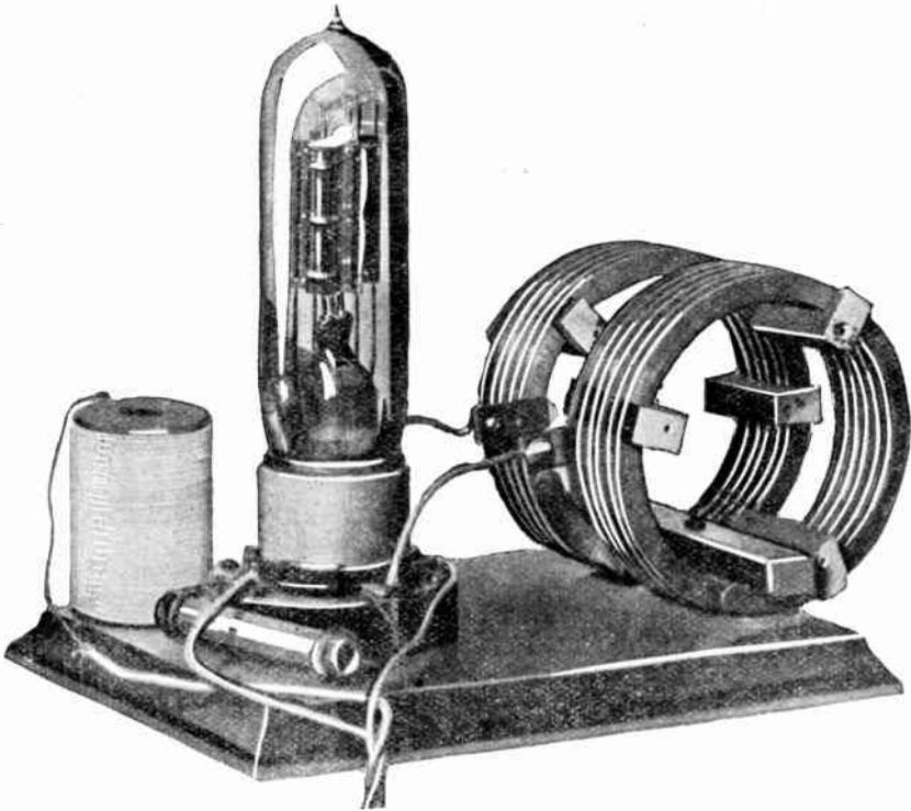
A twenty-meter transmitter used in a modern amateur station.
