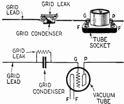
Fig. 24 (Test No. 28). The location of the grid condenser is shown in the illustration.
