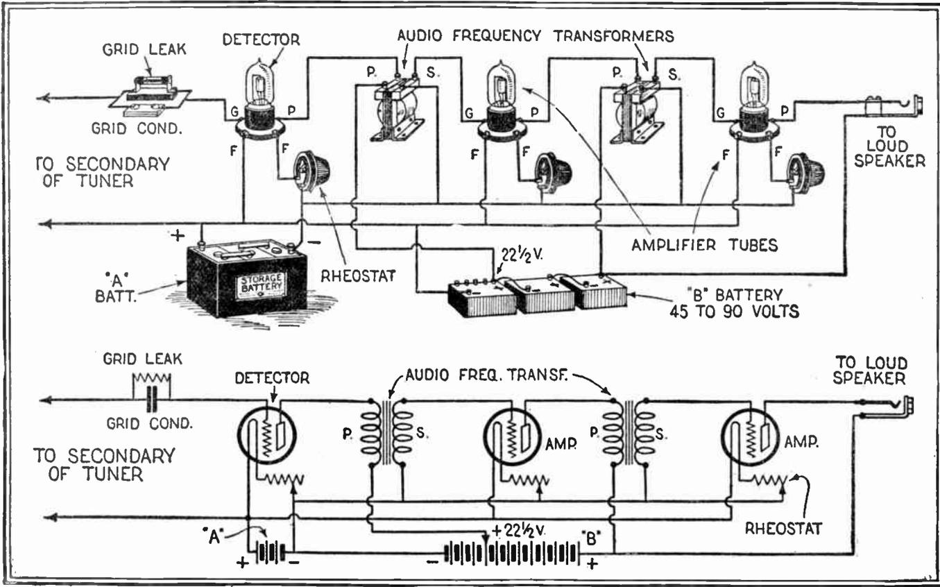
A vacuum tube detector and two stage audio frequency amplifier.
