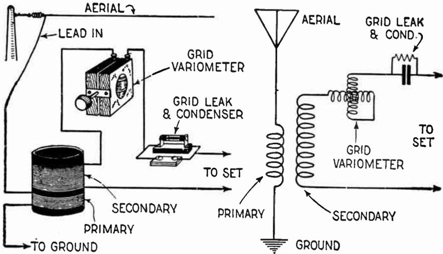
Fig. 11 (Test No. 9). The above diagrams show in both perspective and schematic forms the location of a grid variometer in a regenerative circuit.
