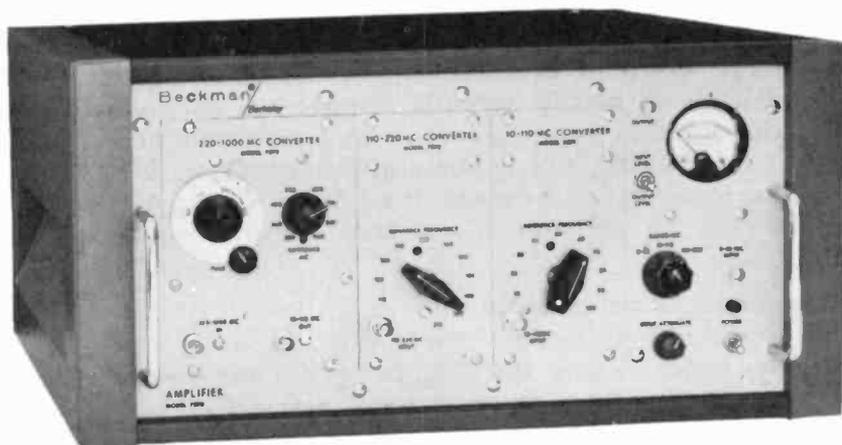
Fig. 604. It is necessary to heterodyne a high frequency that is not within the frequency range of a counter. Stable oscillators can be included in the same case. (Beckman, Inc.)
