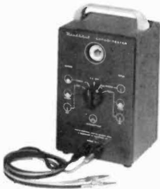
Fig. 1215. *This in-circuit capacitor checker only indicates open or shorted conditions. Actual capacitance and leakage values are not normally indicated as such. (Heath Co.)*
