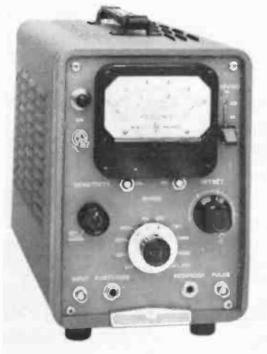
Fig. 1214. *Direct-reading frequency meter needs no adjustment or interpolations to determine frequency. Counters are also used for this type of measurement.*
