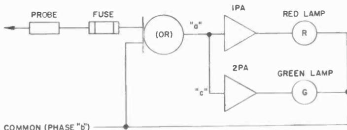
Fig. 828. Phase detector made from or unit and two preamplifiers.
