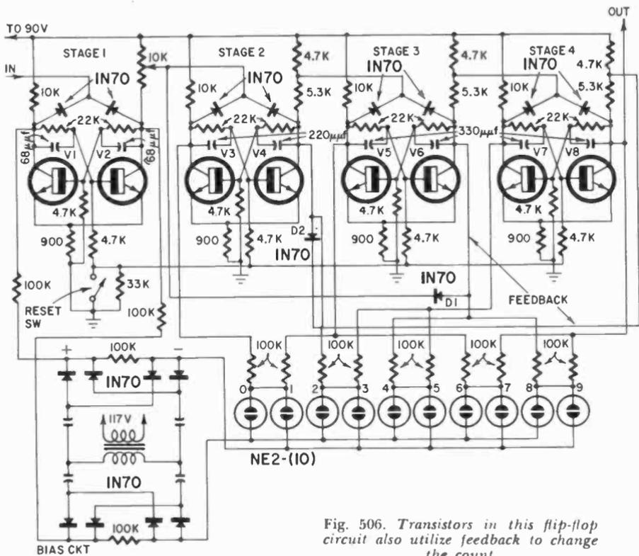
Fig. 506. Transistors in this flip-flop circuit also utilize feedback to change the count.
