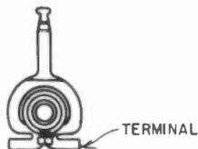
Fig. 705. The two-motion Strouger switch is actuated by two series of digital pulses which select from several hundred contacts.
