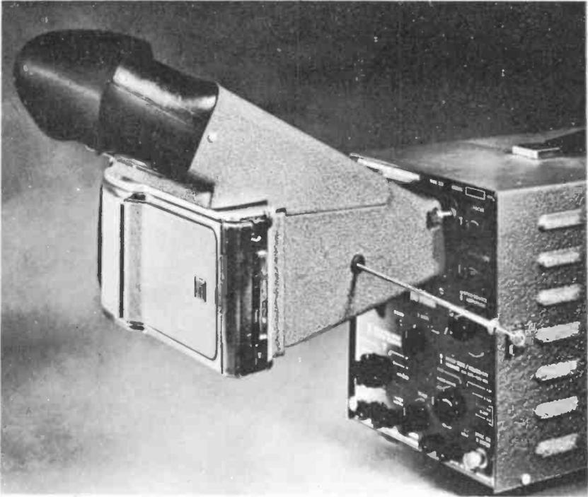
Fig. 1025. Oscilloscope camera shown here uses Polaroid-Land film.
