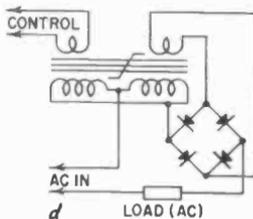
Fig. 805. Bridge-rectifier magnetic amplifier with shunt feedback and ac load.
