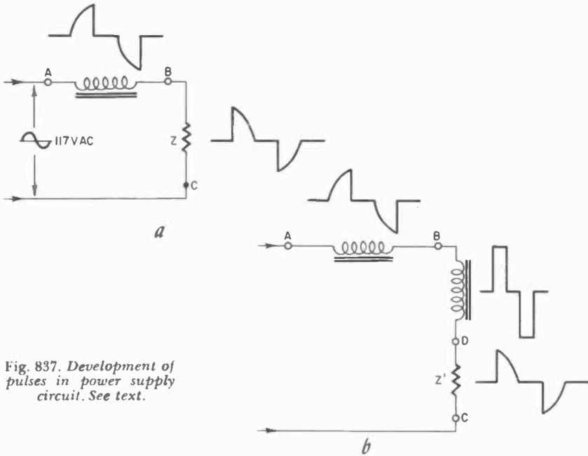
Fig. 837. Development of pulses in power supply circuit. See text.
