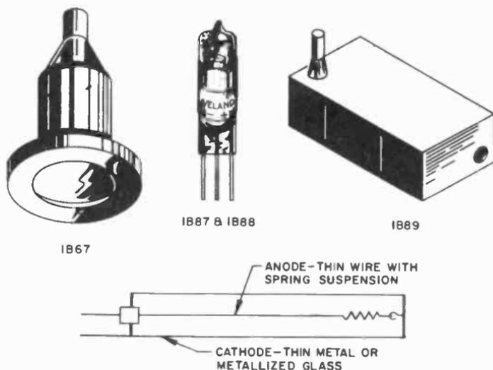
Fig. 213. Geiger-Muller tubes have a variety of shapes. The basic internal construction is shown. (Victoreen Instrument Co.)
