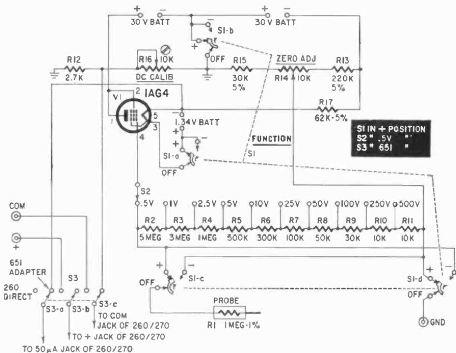
Fig. 1206. Schematic of vtm adapter shows single tube and switching circuit that allow vom operation without removing adapter.
