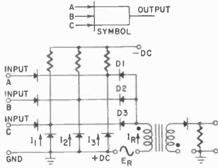
This is the basic Ramey switching unit. From this, various other logic units can be built by adding input circuits, etc., to obtain the desired function. Thus, in Fig. 816 we have added in effect, three diodes. Of course, each one must be blocked by an input signal or the reset current will flow. Thus the unit becomes an AND unit, and all three inputs must be present to obtain an output. A similar circuit can be designed with a different number of inputs, so long as each bias path is blocked.
