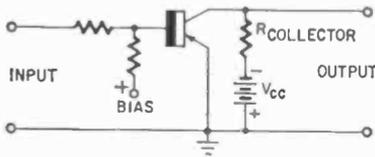
Fig. 901. Basic common-emitter transistor switch circuit.
