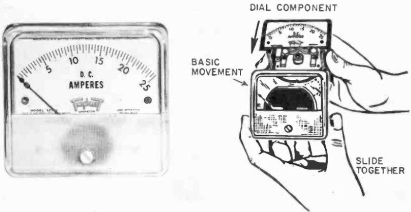
Fig. 1204. Handy for laboratory and bench test setups, the interchangeable units are useful in industrial electronics servicing. (Triplet Electrical Instrument Co.)
