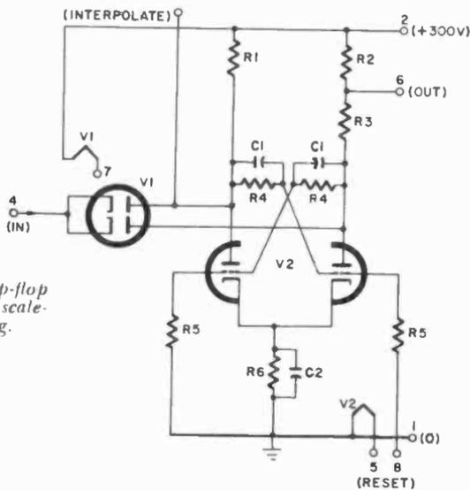
Fig. 501. Basic flip-flop circuit is used for scale-of-two counting.
