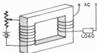
Fig. 801. Basic saturable reactor.
