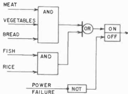
Fig. 808. The basic idea of logic operation is illustrated here.
