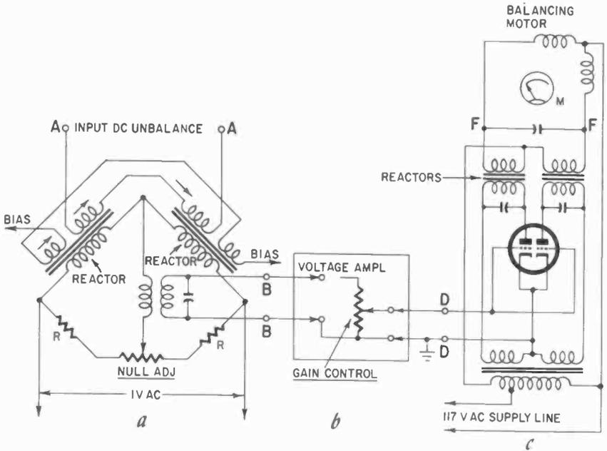
Fig. 1017. Another recorder circuit makes use of saturable reactors as input and control elements.
