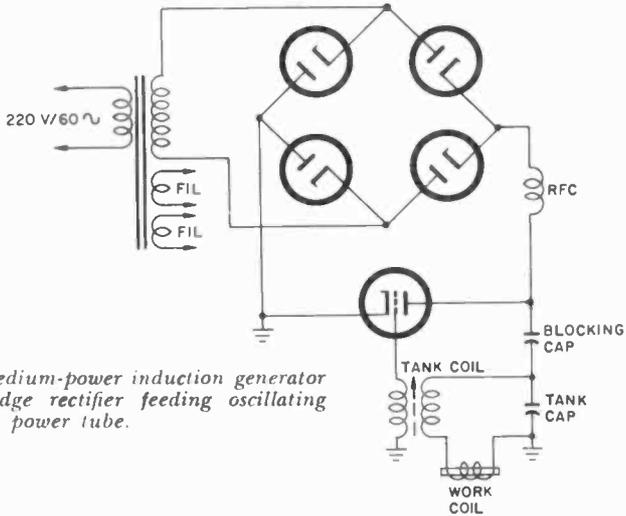
Fig. 305. Simple medium-power induction generator has unfiltered bridge rectifier feeding oscillating power tube.
