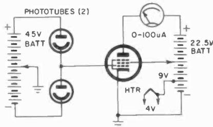
Fig. 718. This comparison circuit measures relative light intensities.
