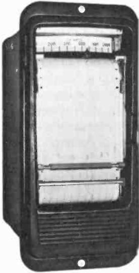
*Fig. 104. Industrial recorder of the single-channel type. This unit supplies a record of power consumption. (Westinghouse Electric Corp.)*
