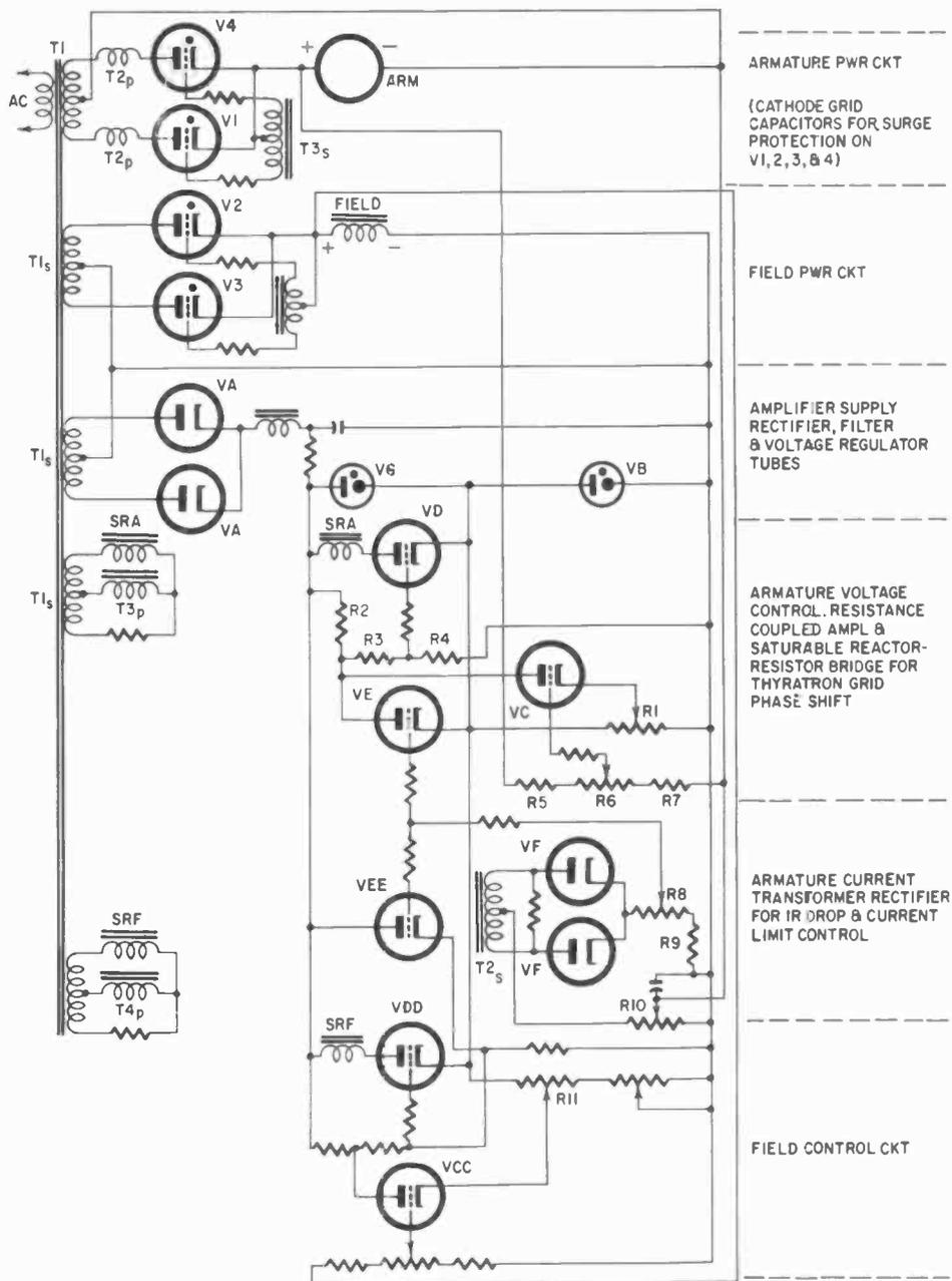
Fig. 728. Simplified schematic of G-E Thyrotrol constant-speed motor control. See text for explanation.
