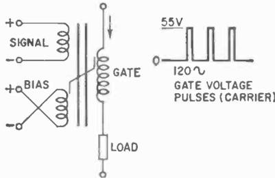
diagram, the bias winding is shown in reverse, indicating that it opposes the action of the signal winding. If we apply a pulse to the gate winding, with the core unsaturated, a constant voltage on the bias winding and no signal applied, this pulse will start to drive the core in to positive saturation, but it will not succeed very well, and the effect at the output will be negligible, due to the bias. However, with signal applied, the pulse will now go toward
