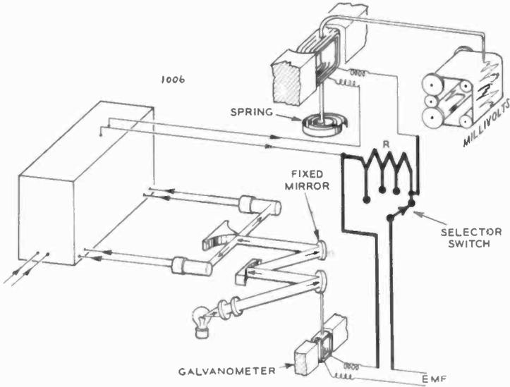
Fig. 1006. Mechanics of the potentiometer type photoelectric recorder are similar to the deflection type. Added circuitry is shown in heavy lines.
