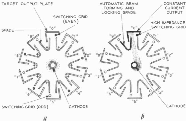
Fig. 511. During the CLEAR condition (a) there is no current flow. Electron beam indicates zero. Design causes beam to switch to the next highest number.
