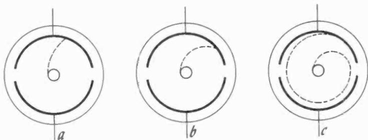
Fig. 1126. Three conditions of electron path in magnetron. Variations are due to changes in magnetic field or applied voltages.
