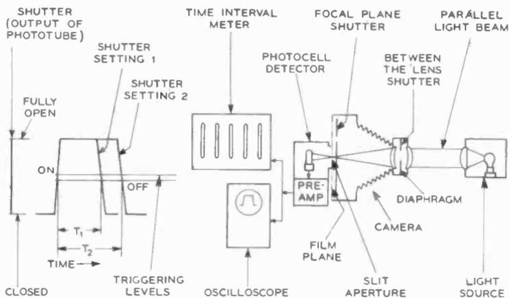
Fig. 610. A photocell connected to a time-interval meter will check camera shutter speed.
