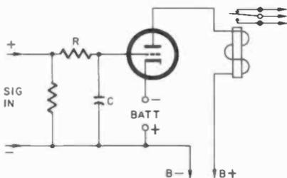
Fig. 710. Simple electronic delay circuit depends on charging time of capacitor C.
