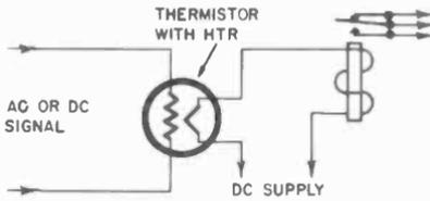
Fig. 713. Basic thermistor time-delay circuit.
