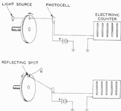
Fig. 605. Pulses of light can be converted into rpm with a counter.
