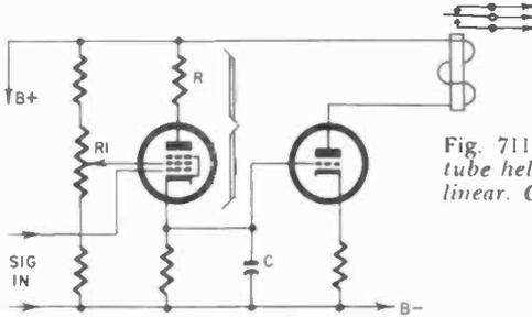
Fig. 711. Pentode charging tube helps make time delay linear. Charging rate is set by R1.
