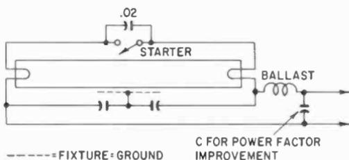
Fig. 405. Capacitor across switch reduces one type of interference while the capacitors grounded to fixture remove most of the hash.
