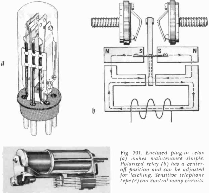
Fig. 701. Enclosed plug-in relay (a) makes maintenance simple. Polarized relay (b) has a center-off position and can be adjusted for latching. Sensitive telephone type (c) can control many circuits.
