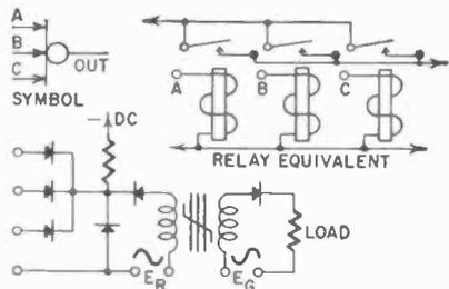
If input rectifiers are added, but only one bias rectifier (Fig. 817), any one of these inputs could block the bias rectifier current, and give us an OR unit. Again, the number of inputs is variable – there could be two, three (as shown) or more.
