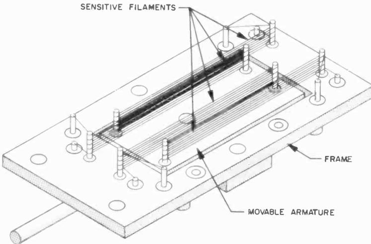
Fig. 1104. Unbonded strain gage is made of wire wound on pins. Resistance change is relative to the movement of the two plates. It can be attached to a diaphragm to measure pressure.
