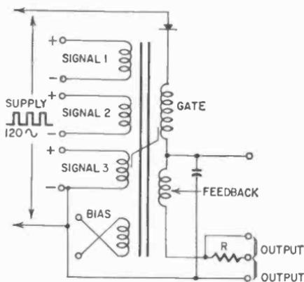
Fig. 833. Pulsed or circuit.
