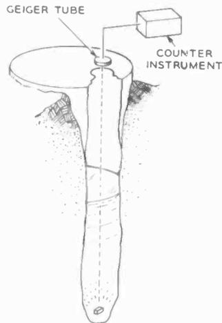
Fig. 1111. *Radioactive level measurement uses low-grade radioactive source, measures absorption by column of liquid.*
