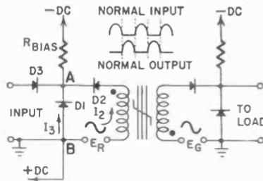
To match this unit to other similar units several conditions must be met. First, the reset winding must have a low impedance in order to assure positive reset. But to avoid loading the previous stage, a high impedance input is necessary. Therefore, the unit is equipped with rectifiers and a dc bias source (Fig. 815). The bias
