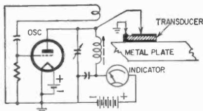
Fig. 319. Basic circuit for an ultrasonic thickness gage.
