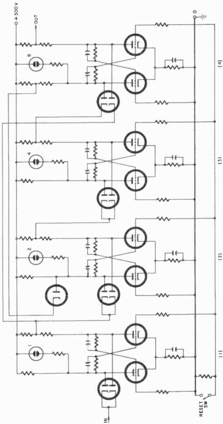
Fig. 502. Four scale-of-two flip-flops will count to sixteen.
