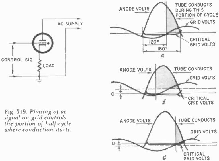
Fig. 719. Phasing of ac signal on grid controls the portion of half-cycle where conduction starts.
