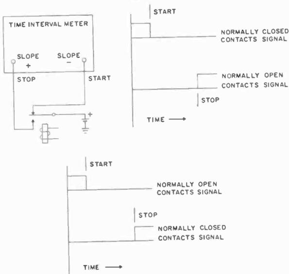
Fig. 607. Simple circuit measures relay transition time.
