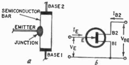
Fig. 904. The symbol for the Unijunction transistor and its internal construction.
