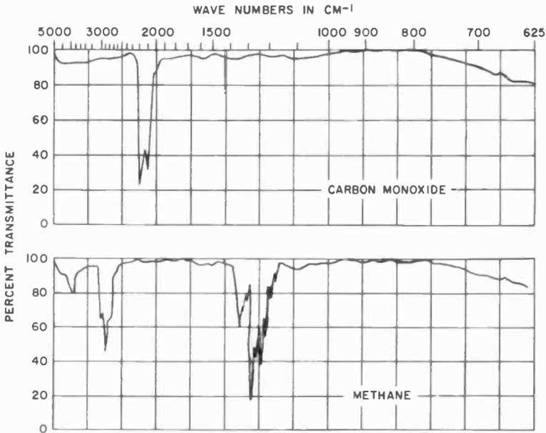
Fig. 1117. Infrared spectra can identify a great number of substances accurately. This is particularly true of hydrocarbon gases and vapors. Many other substances have characteristics in the microwave and ultraviolet spectrums.
