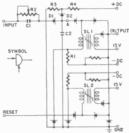
Fig. 821. Time-delay circuit made from Ramey units. Varying C2 and R2 will change timing.
