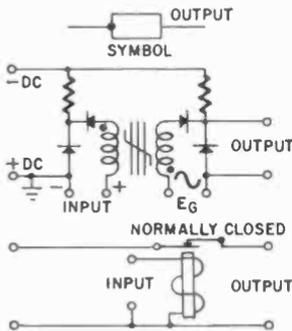
Fig. 818. Ramey not circuit with symbol and relay equivalent. As in the relay circuit, if an input is present, there is no output.
