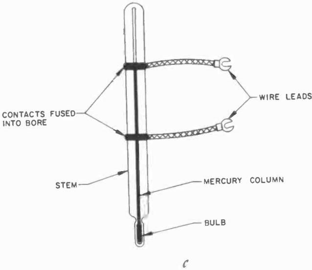
Fig. 1107-c. Contacts inserted through the glass during the manufacture of this highly accurate thermostal complete the circuit through the mercury column.
