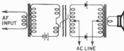
Fig. 807. Magnetic amplifier has been used to amplify audio frequencies. Unless a supersonic ac source is used, the carrier is heard.
