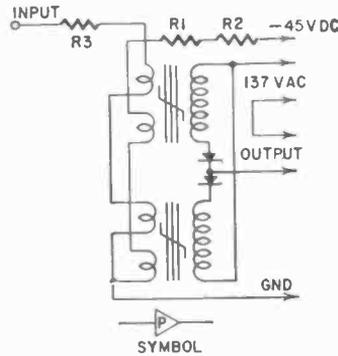
Fig. 823. Basic magnetic output amplifier circuit for Cypak system has extra windings to allow the two inputs to be circuited in series while the outputs are paralleled.
