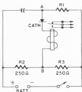
Fig. 709. Delayed make relay. See text for description of operation.
