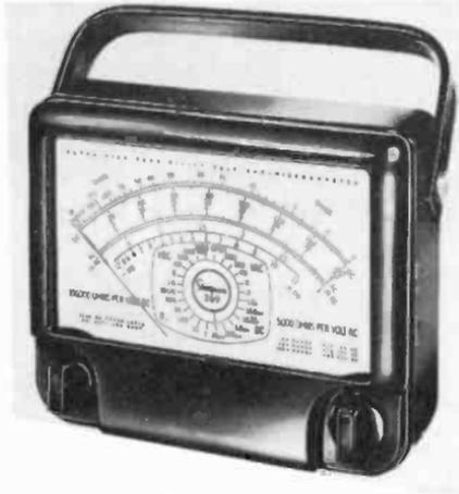
Fig. 1203. The 100,000-ohms-per-volt sensitivity of this instrument allows it to be used for tests that would normally require a vtvm. (Simpson Electric Co.)
