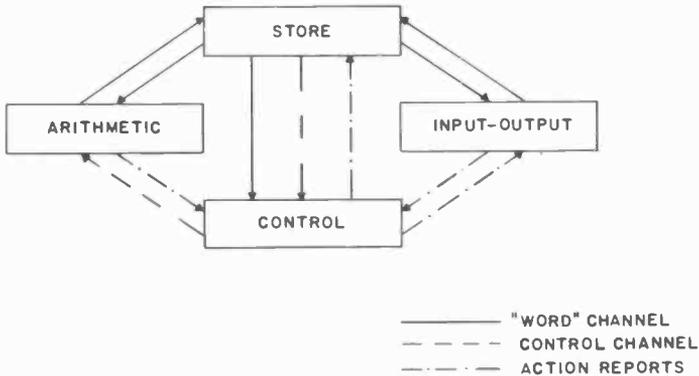
Fig. 922. Block diagram of basic digital computer.
