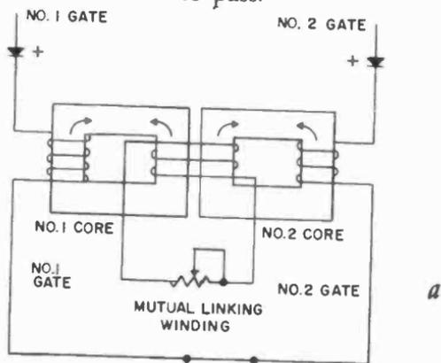
Fig. 838. Physical arrangement of pulsed delay unit is shown at (a) while the schematic is given at (b).
