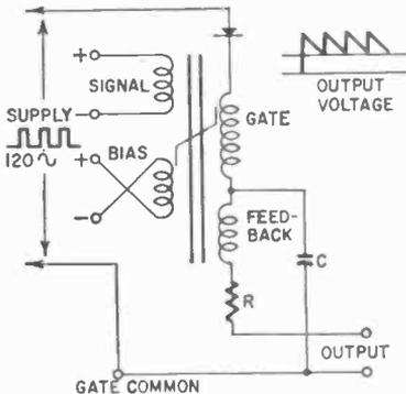
Fig. 831. Adding feedback makes the pulsed magnetic amplifier suitable for logic functions.
