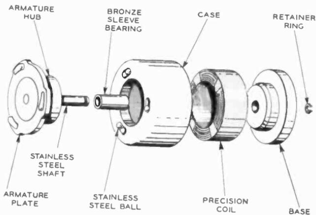
Fig. 704. Rotary solenoid can be used to drive many rotary switch decks.
