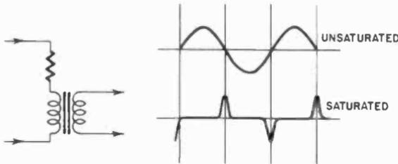
Fig. 725. A peaking transformer is saturated and produces secondary voltages only when changing from one state of saturation to the other. The low impedance of the saturated transformer requires a series current-limiting resistor.
