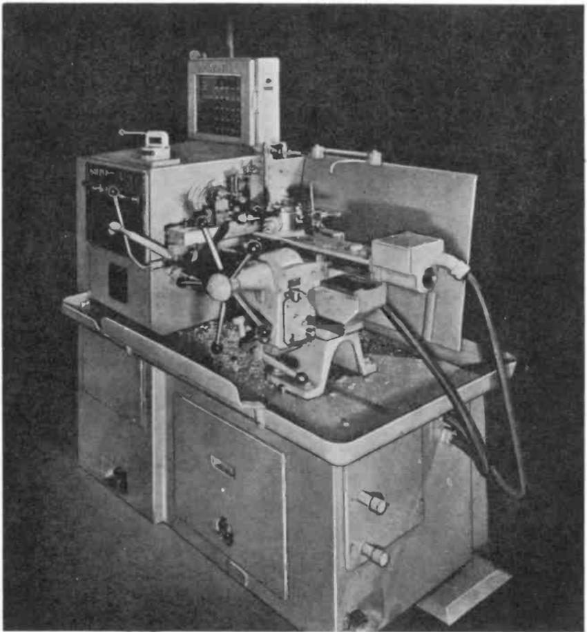
Fig. 822. This turret lathe has sequential operation control with a Cypak system.
