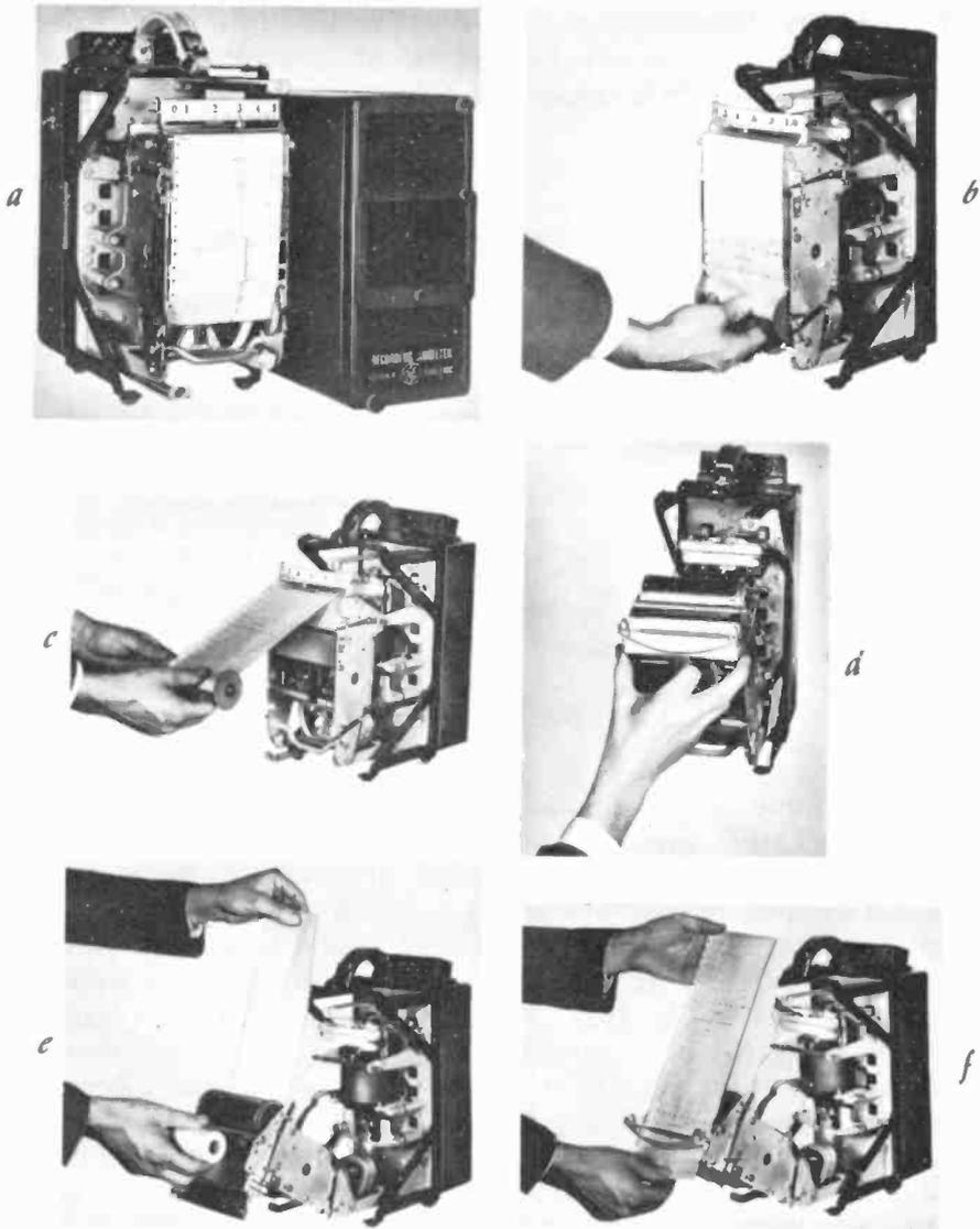
Fig. 1020. The chart-removal sequence: remove case (a), pull out take-up spool (b), remove unused chart paper (c), remove empty spool (d), start new roll (e), thread new paper through guides (f). Procedure is similar for most recorders and is detailed in their individual maintenance manuals. (General Electric Co.)
