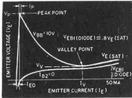
If we apply a voltage smaller than this emitter-junction voltage from an external supply, the junction will remain reverse-biased. But if we apply a larger voltage, holes will be injected into the
