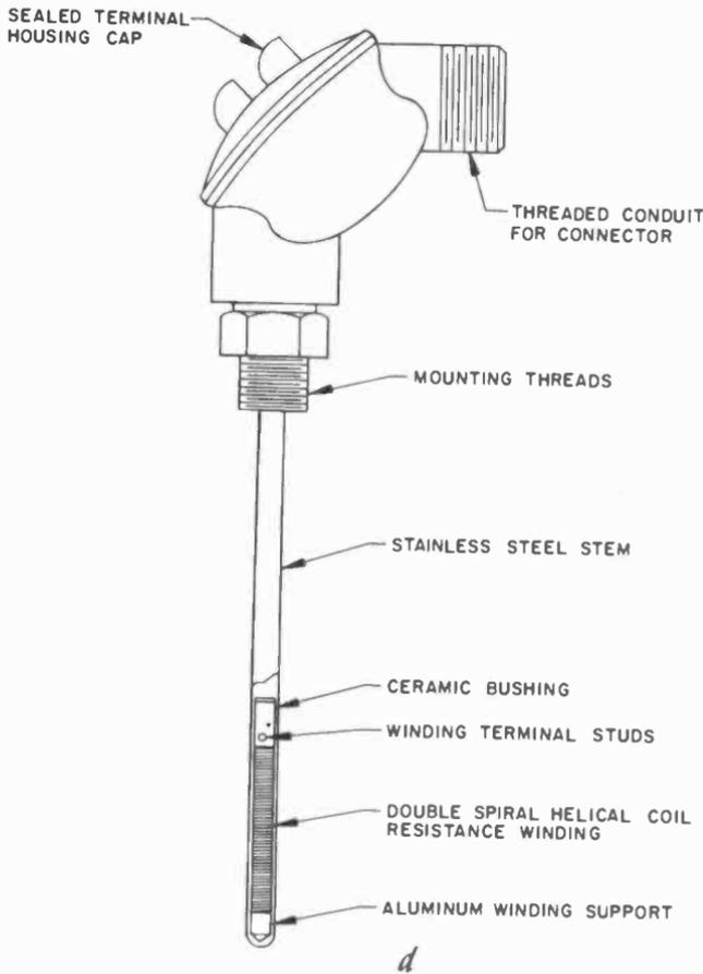
Fig. 1107-d. Resistance-change readings indicate the temperature in this sensing element.
