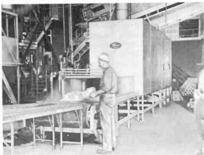
Fig. 102. *Large dielectric generator being used for the baking of foundry cores. (The Girdler Company.)*
