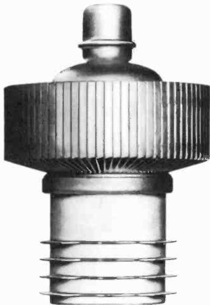
*Fig. 206. Forced air conducts heat away from the radial heat dissipating fins.*
