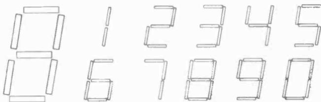
Fig. 613. Numerals of this type are displayed by neon tubes or electroluminescent display devices.
