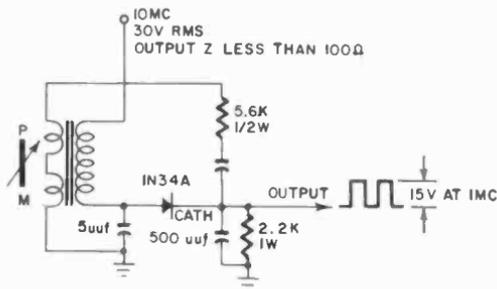
Fig. 516. Pulse feedback makes a freerunning multivibrator of the basic ferristor circuit.
