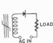
Fig. 812 (left). Hipernik core with winding, rectifier and applied ac can be self-saturating.
