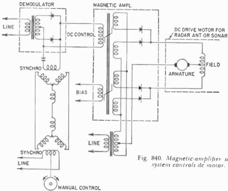
Fig. 840. Magnetic-amplifier servo system controls dc motor.
