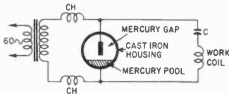
Fig. 304. Mercury under pressure prevents vapor from forming and making the arc uncontrollable.
