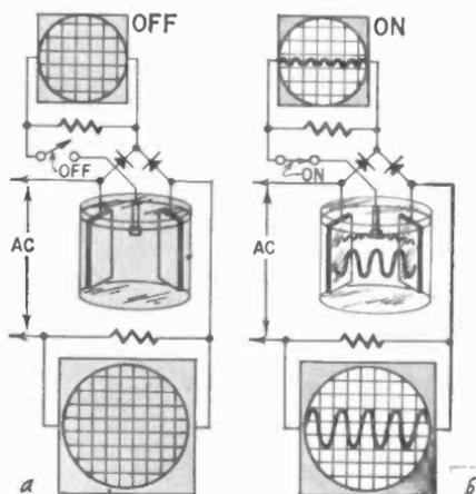
Fig. 910. Both the cryostat (a) and the electrochemical switch (b) must be housed in special containers.
