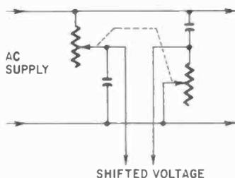
Fig. 722. Phase-shifted voltage output from this dual circuit is quite constant.
