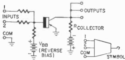
so long as we have one NOT without a signal. It takes a signal on both NOT's to get one from the NOR. Thus we get the AND function. We can add as many inputs to the NOR as we wish and, by adding more NOT's, we can make an AND circuit for more than two items.
