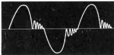
*Fig. 404. Waveform generated by repeated extinction and striking of arc within the fluorescent lamp is at frequency much higher than that provided by the power line.*
