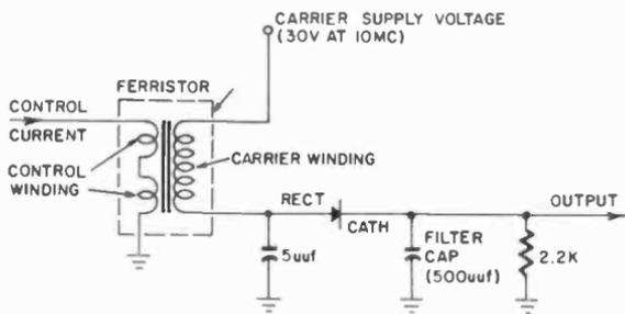
Fig. 514. Basic ferromagnetic amplifier. High-frequency ac is used for a carrier.
