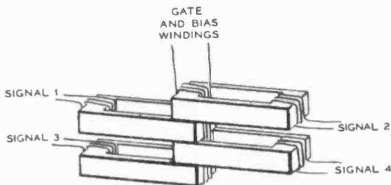
Fig. 835. Stacked cores for AND unit have common gate and bias winding but separate signal windings.
