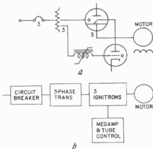
Fig. 204. Block diagram and single line diagram are different ways to show the same circuit.
