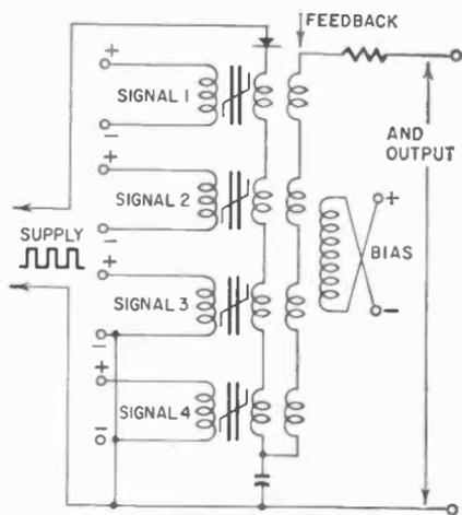
Fig. 836. Schematic of four input and units.
