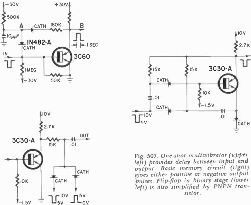
Fig. 507. One-shot multivibrator (upper left) provides delay between input and output. Basic memory circuit (right) gives either positive or negative output pulses. Flip-flop in binary stage (lower left) is also simplified by PNPN transistor.
